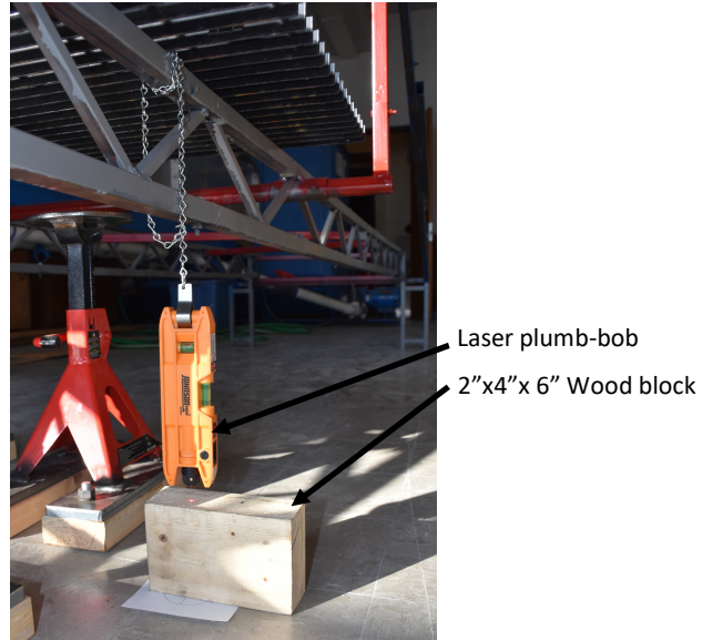
Figure 9. Laser plumb-bob position.
