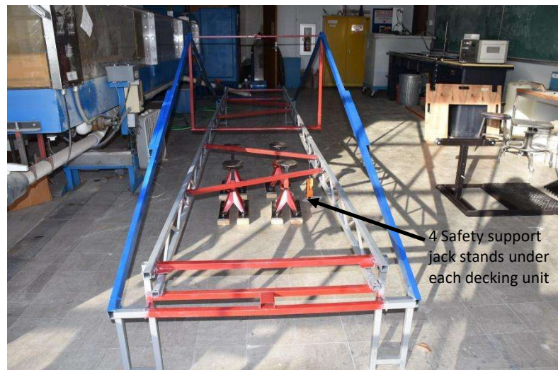
Figure 2. Jack stands under bridge at load location.
