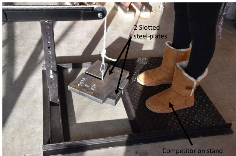
Figure 8. Load applied to lateral load stand.
