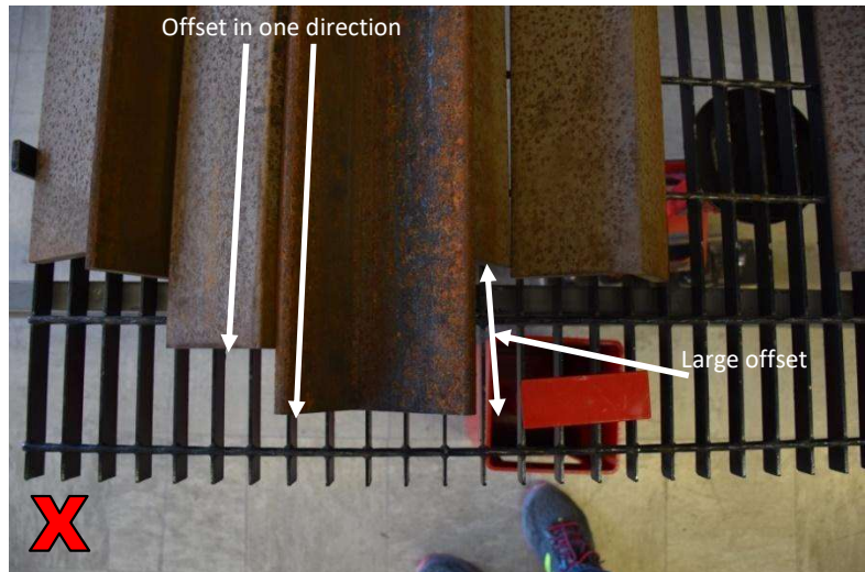
Figure 15b. Improper stacking of loading angles.
