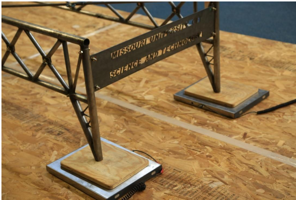
Bridge positioned on scales to measure weight
