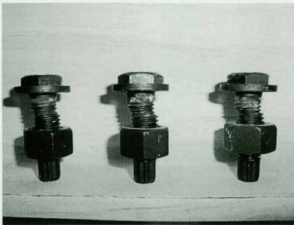
Test 3A – Connection Bolts at End of Test (fit back together)
