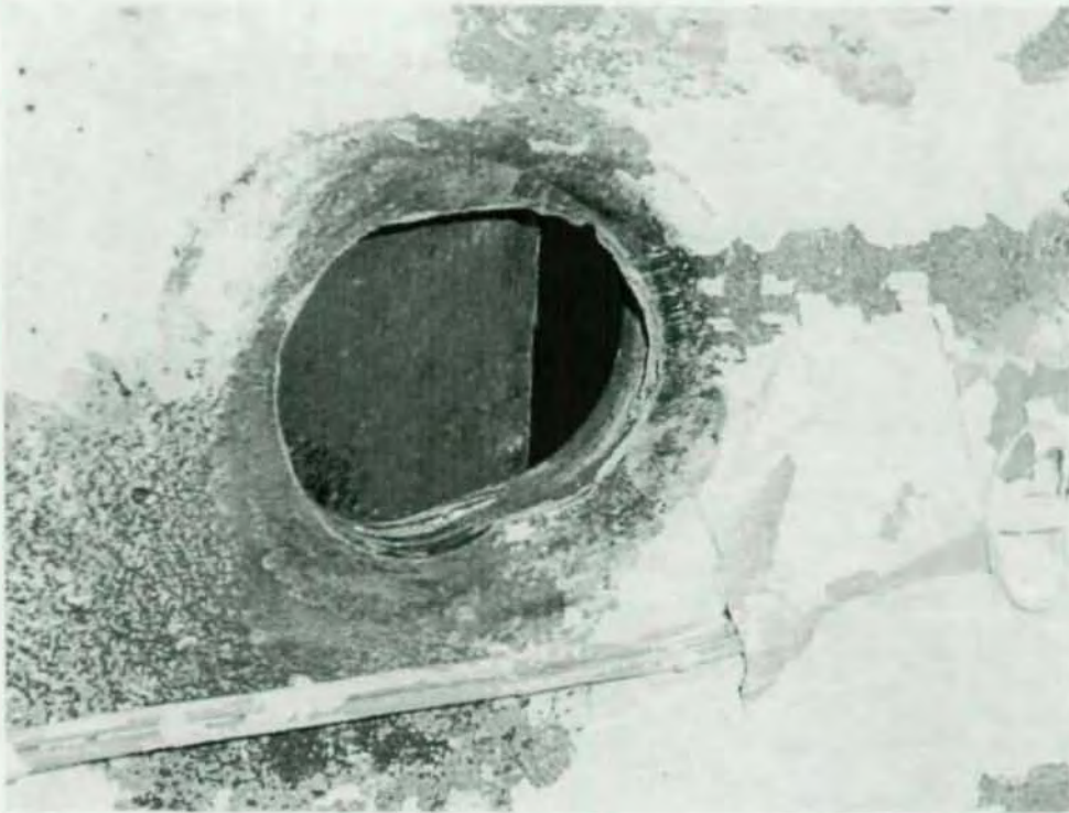
Test 3A – Bottom Bolt Hole in Shear Tab After Test
