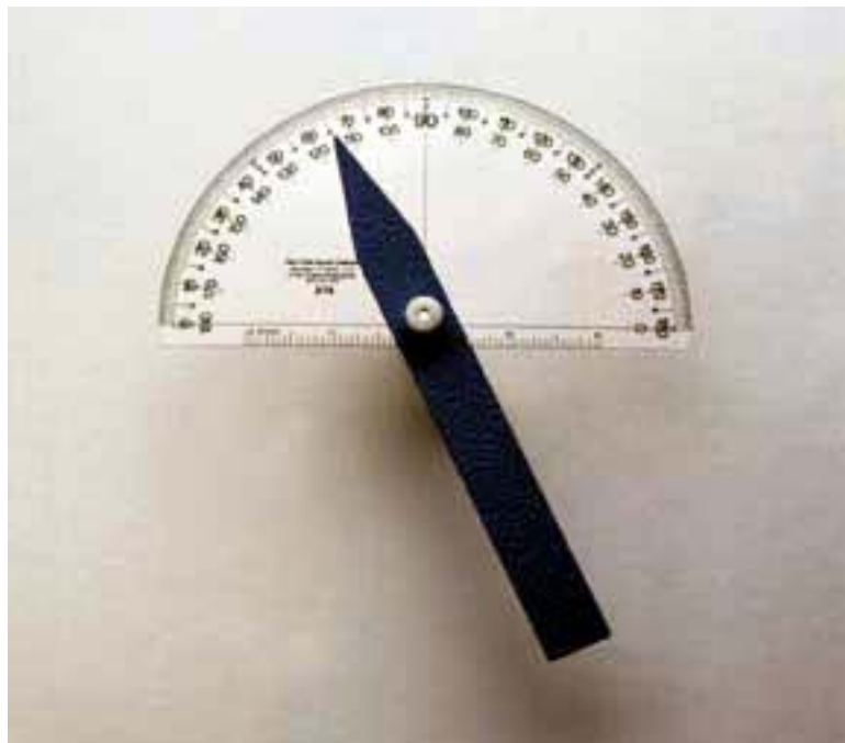
Figure 3.13 – Protractor used for measuring fracture angle
