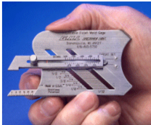
Figure 3.9 – Photograph of fillet weld gage
