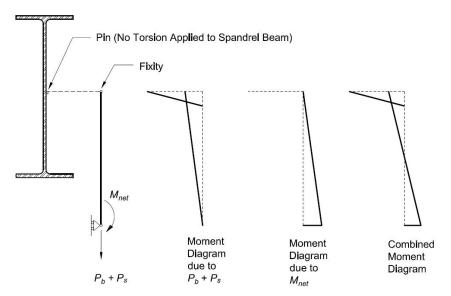
Fig. 7-28. Hanger assembly moment diagram with pin at spandrel beam web.
