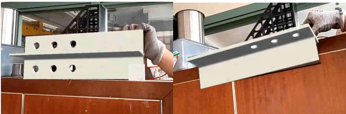
Figure 5: AR model overlaid on the sideways (left) and upside down (right) steel tee
