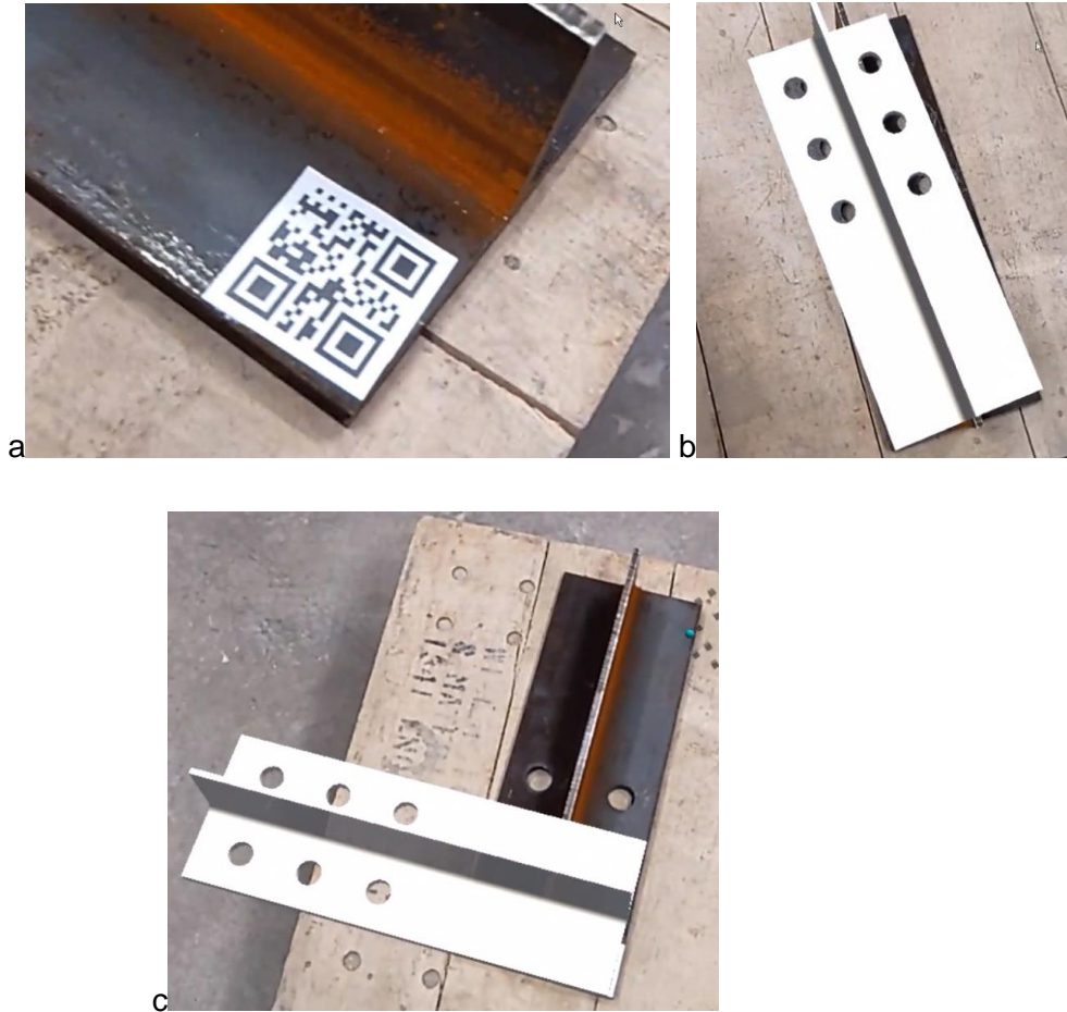
Figure 2a-c: Fig. a (Top Left) - Misaligned QR code, not flush with the corner of the steel tee Fig. b (Top Right) - Resulting model from Figure 2a orientation with QR code slightly misaligned Fig. c (Bottom) - Model with QR code placed on the incorrect side of the steel tee and rotated
