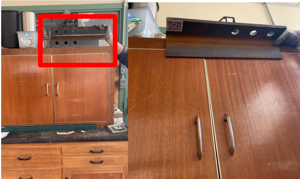
Figure 4: Setup of the steel tee to test when the QR code is sideways (left) and upside down (right) both at approximately eye level
