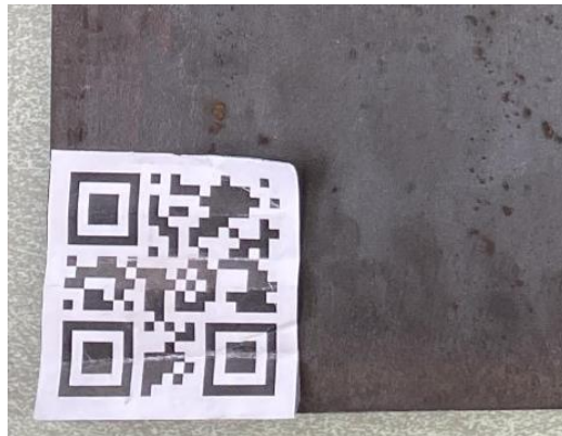
Figure 3: A wrinkled QR code that the HoloLens program could still recognize
