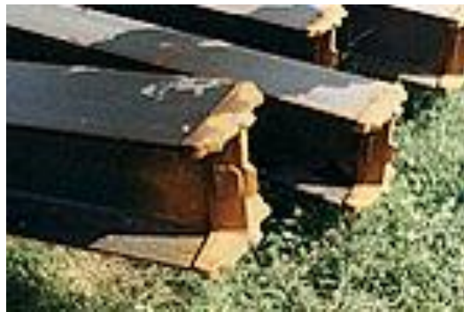
Figure 5 Example of pile tips.
