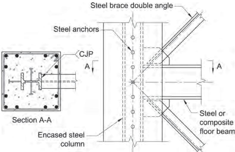
Fig. C-H1.1. Reinforced concrete (or composite) column-to-steel concentric brace.
