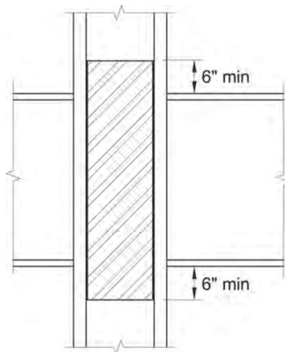
Fig. C-E3.7. Doubler plates used without continuity plates.
