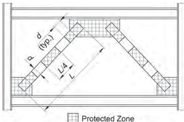
Fig. C-F2.14. Protected zone of inverted V-braced frame.
