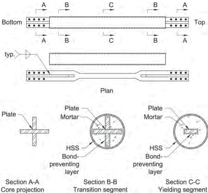
Fig. C-F4.1. Details of a type of buckling-restrained brace (courtesy of R. Tremblay).
