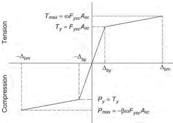
Fig. C-F4.3. Diagram of brace force-displacement.
