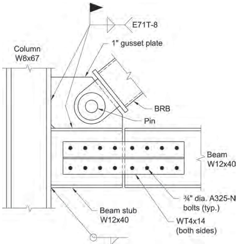
Fig. C-F4.6. Detail of connection with hinge
