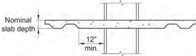
Fig. C-G4.3. Solid slab to be provided around column.
