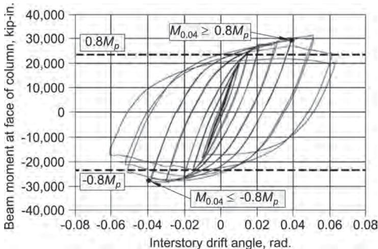
Fig. C-E3.2. Acceptable strength degradation, per Section E3.6b.
