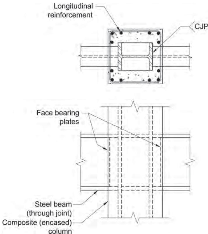
Fig. C-G3.1. Encased composite column-to-steel beam moment connection.
