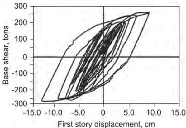
Fig. C-F2.21. Base shear versus story drift of an SCBF.
