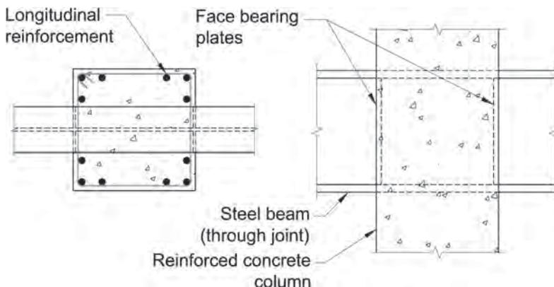
Fig. C-D2.10. Reinforced concrete column-to-steel beam moment connection.
