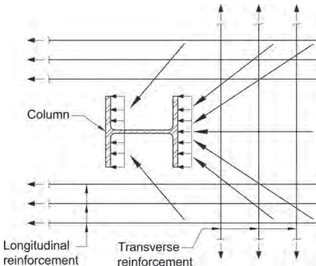
Fig. C-G4.2. Concrete slab bearing force transfer.
