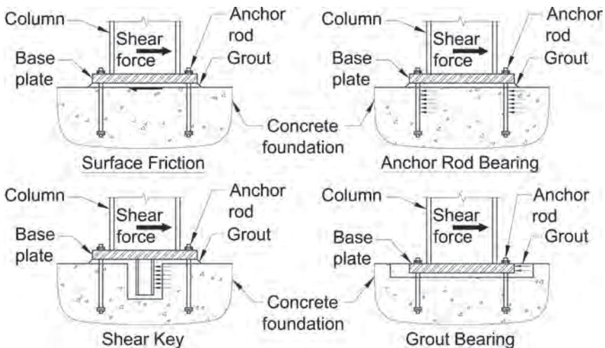
Fig. C-D2.5. Shear transfer mechanisms—column supported by foundation.
