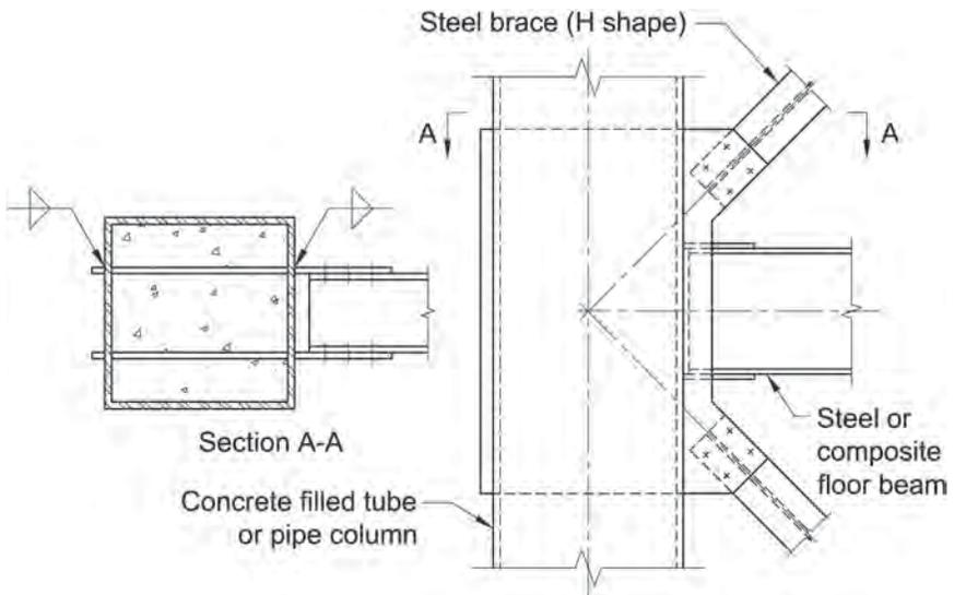
Fig. C-H1.3. Filled HSS or pipe column-to-steel concentric base.
