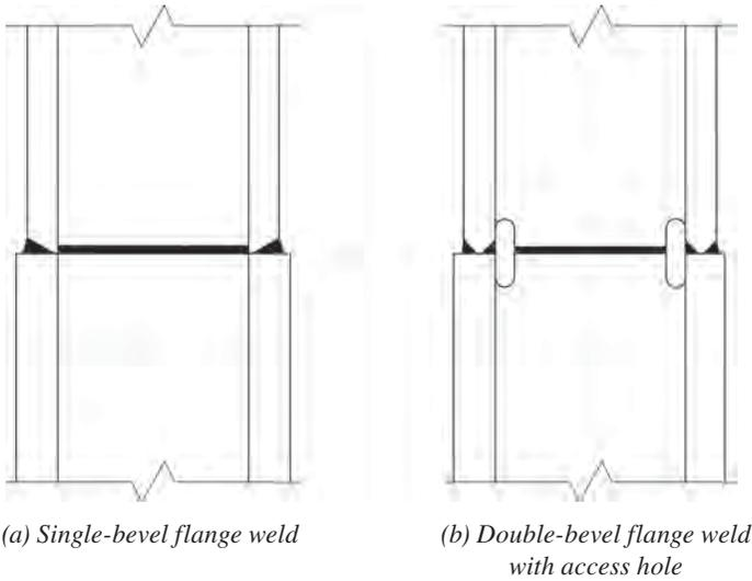
Fig. C-E3.10. Splice details with partial-penetration-groove welds.
