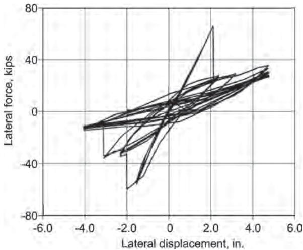
Fig. C-E4.1. Strength degradation in undetailed truss girder.
