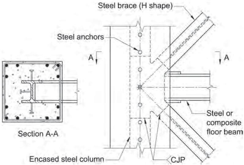
Fig. C-H1.2. Reinforced concrete (or composite) column-to-steel concentric brace.
