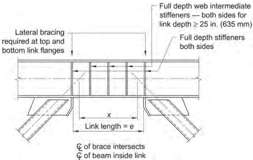
Fig. C-F3.6. EBF with HSS bracing ( $x < e$ ).
