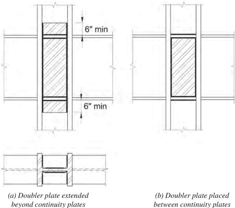
Fig. C-E3.8. Doubler plate used with continuity plates.
