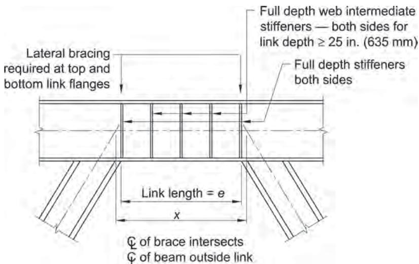
Fig. C-F3.7. EBF with W-shape bracing ( $x > e$ ).
