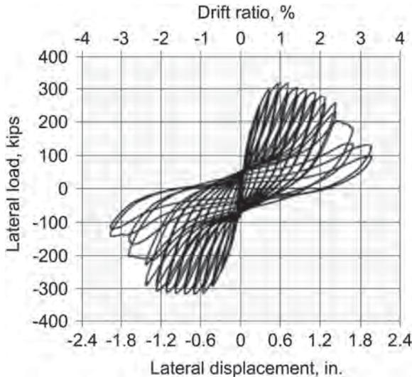
Fig. C-H7.4. Cyclic behavior of C-PSW/CF without boundary elements
