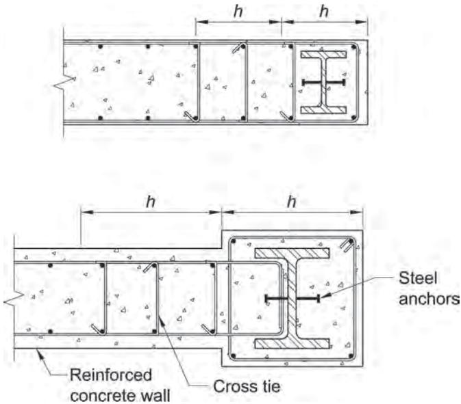
Fig. C-H4.1. Reinforced concrete walls with composite boundary element.
