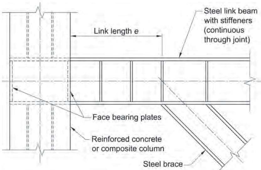
Fig. C-H3.1. Reinforced concrete (or composite) column-to-steel eccentric brace.
