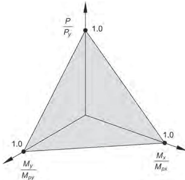
Fig. C-E3.1. Linear yield surface for bi-axial bending.
