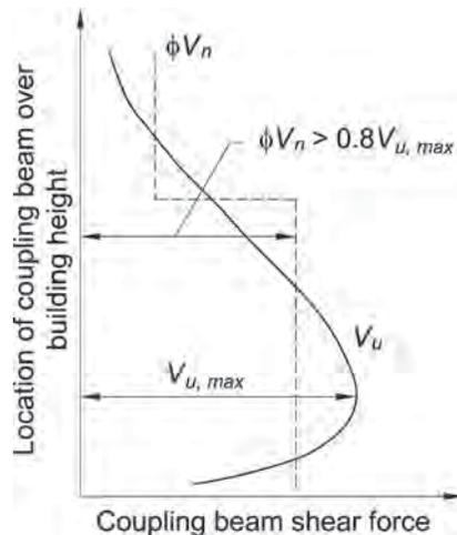
Fig. C-H4.4. Vertical distribution of coupling beam shear.
