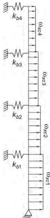
Fig. C-F5.3. Elastic VBE model with HBE springs.
