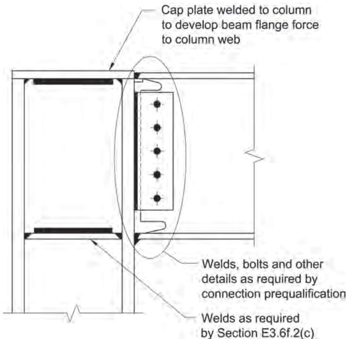
Fig. C-E3.9. Cap plate detail at column top.
