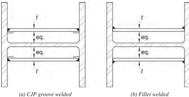
Fig. C-E3.5. Doubler plates spaced away from the web.
