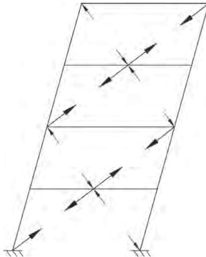
*Fig. C-F2.3. Anticipated braced-frame mechanism.*
