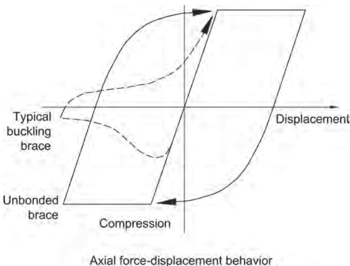
Fig. C-F4.2. Typical buckling-restrained (unbonded) brace hysteretic behavior (courtesy of Seismic Isolation Engineering).
