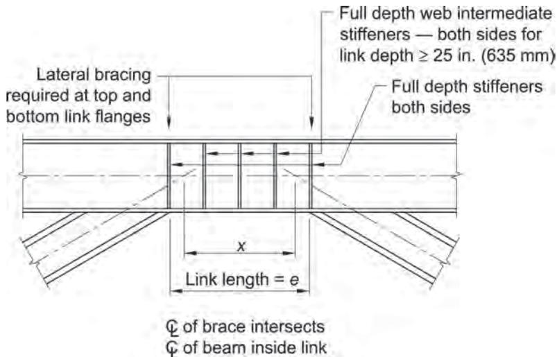
Fig.C-F3.5. EBF with W-shape bracing ( $x < e$ ).
