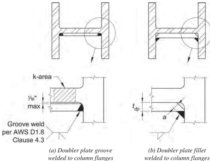
Fig. C-E3.6. Doubler plate in contact with column web.
