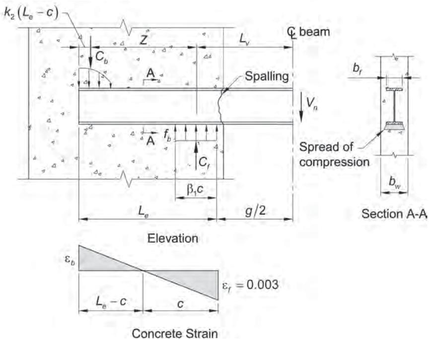
Fig. C-H4.5. Method for computing the embedment capacity.
