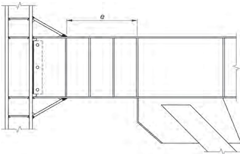
Fig. C-F3.10. Example of a reinforced link-to-column connection.
