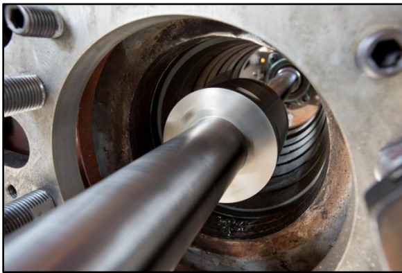
Figure 37 – Line Bore of Upper Pin
