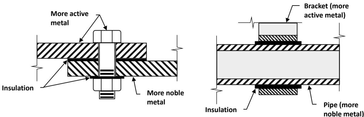
**Figure 2.5.4.5-1—Insulation methods to prevent galvanic corrosion.**
