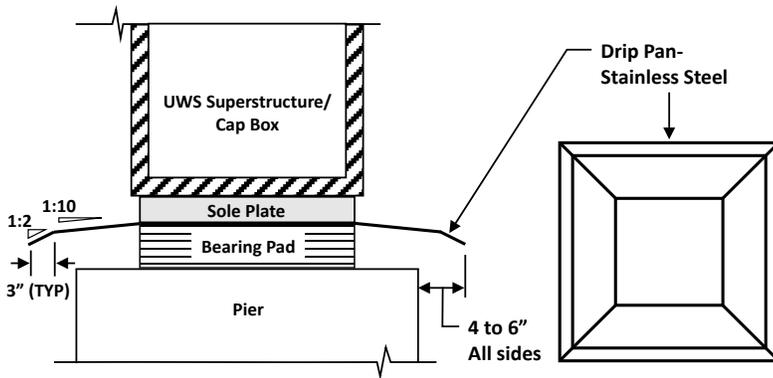
Figure 2.5.1-6—Example drip pan detail.
