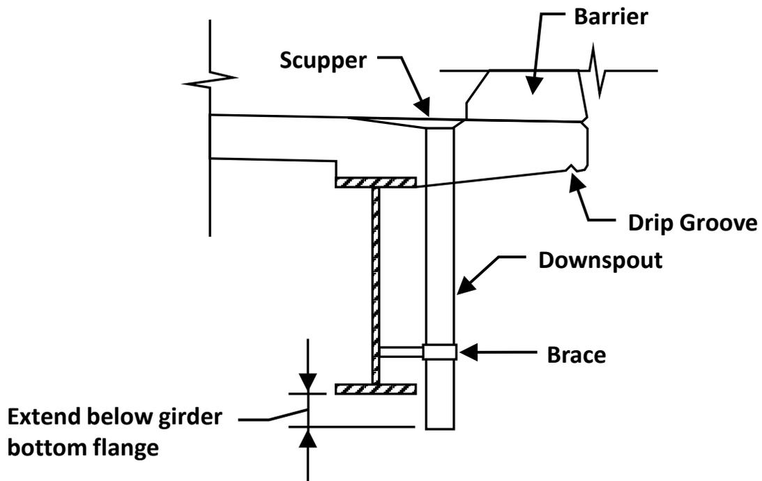
Figure 2.5.1-8—Example downspout detail.
