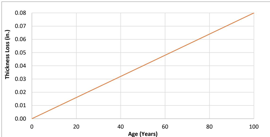
**Figure 2.4.3-1—Estimated upper-bound section loss for fully-exposed UWS plates (i.e., total section loss on top and bottom surfaces) in "high" corrosive environments.**
