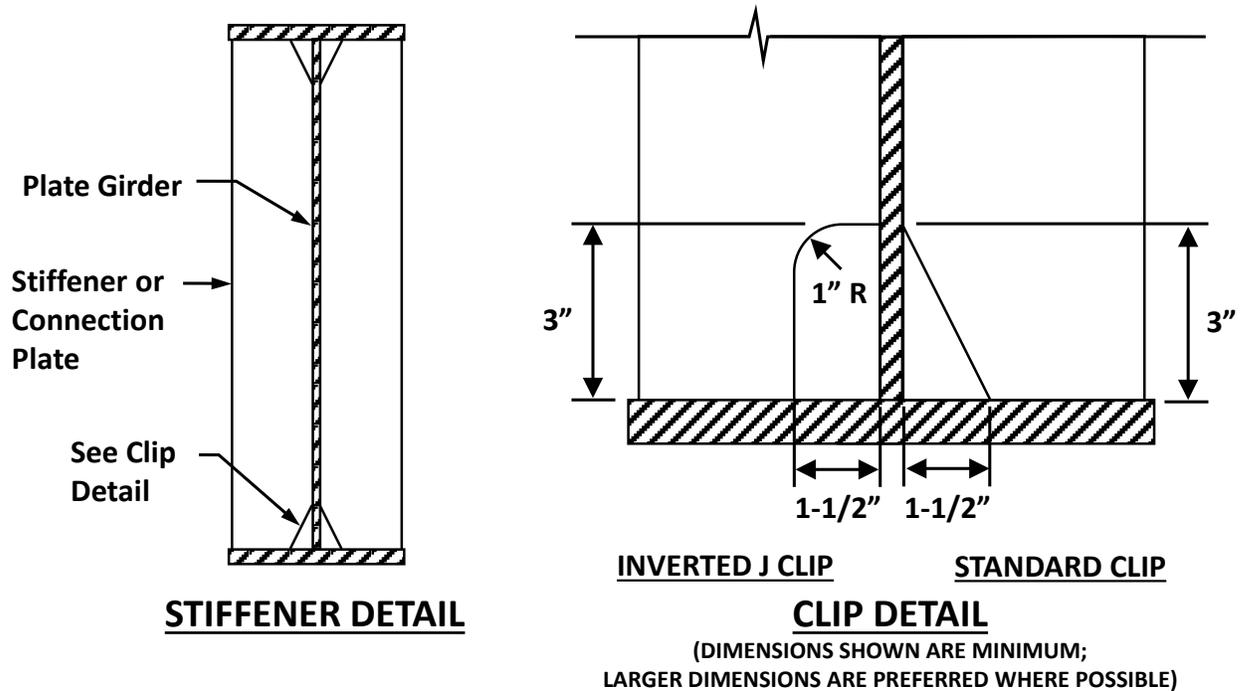
Figure 2.5.2-1—Size stiffener clips to avoid trapping debris.
