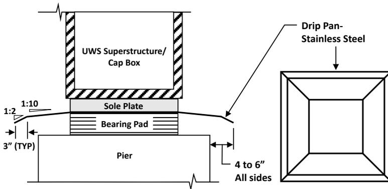
Figure 2.5.1-6—Example drip pan detail.
