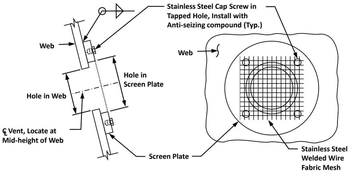
Figure 2.5.1-14—Example box girder screened vent hole detail.
