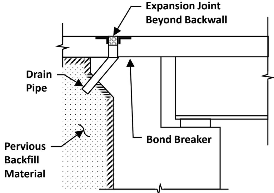
Figure 2.5.1-10—Example of locating the expansion joint at the back of the backwall.
