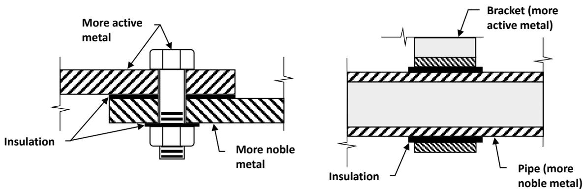
**Figure 2.5.4.5-1—Insulation methods to prevent galvanic corrosion.**
