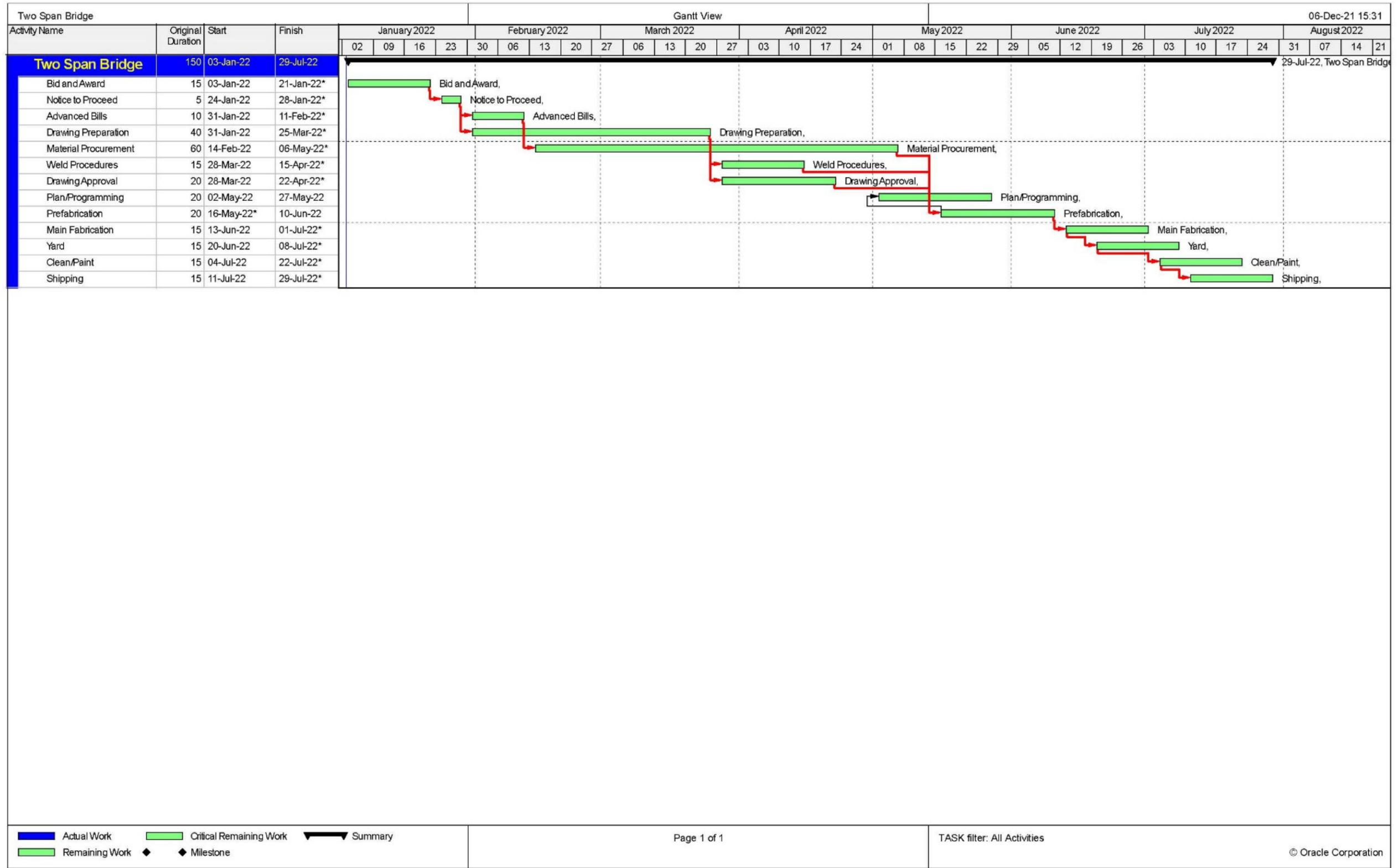
Figure 1: Typical Project Fabrication Schedule.
