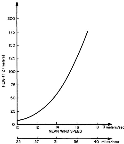
Fig. 1. Typical wind speed profile vs height (suburban terrain)
