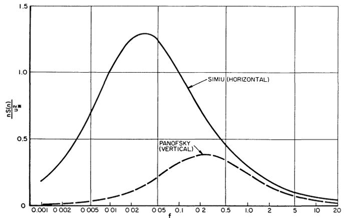
Fig. 3. Spectra of longitudinal and vertical wind components
