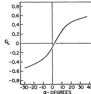
Fig. 6. Lift coefficient of new Tacoma Narrows Bridge
