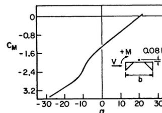
Fig. 7. Moment coefficient of new Tacoma Narrows Bridge
