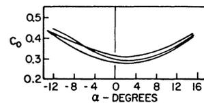
Fig. 5. Drag coefficient of new Tacoma Narrows Bridge
