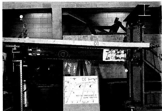
Fig. 20. Testing of composite beam-to-column connection
