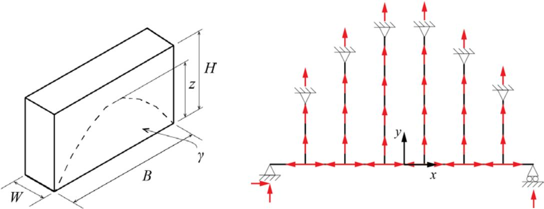
Figure 10 Schematic diagram of the building dimensions and tension members (tie and hangers) for Exchange House
