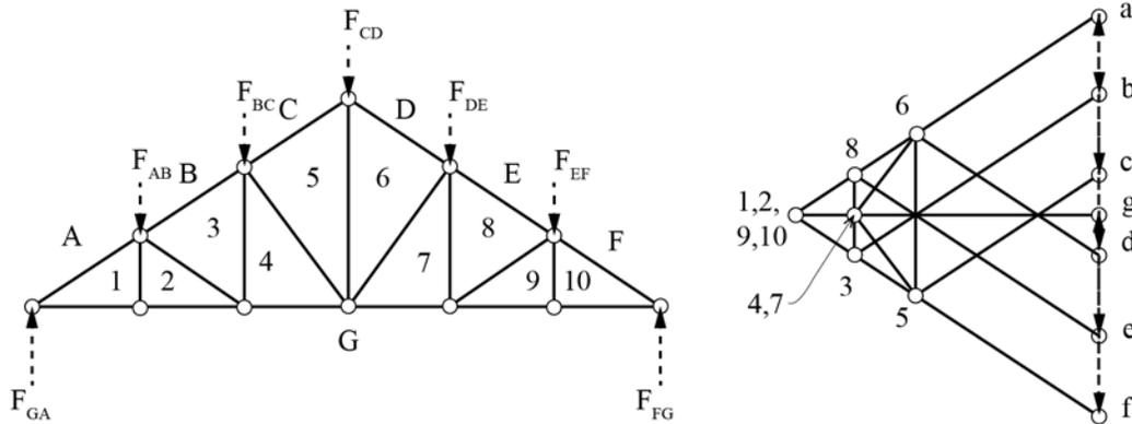
Figure 19 Form and force diagrams for gable truss
