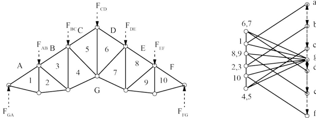
Figure 20 Constant force gable truss (force is constant in top chord)
