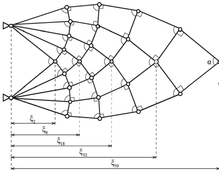
Figure 16 Optimal Discrete Michell Truss
