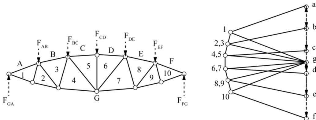
Figure 22 Truss designed for constant and equal force in top and bottom chord
