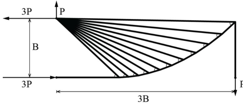
Figure 7 Cantilever with only compression chord.
