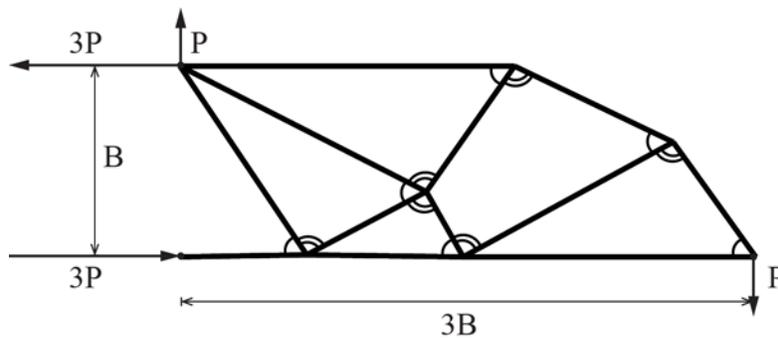
Figure 6 Bounded optimal truss with 12 members
