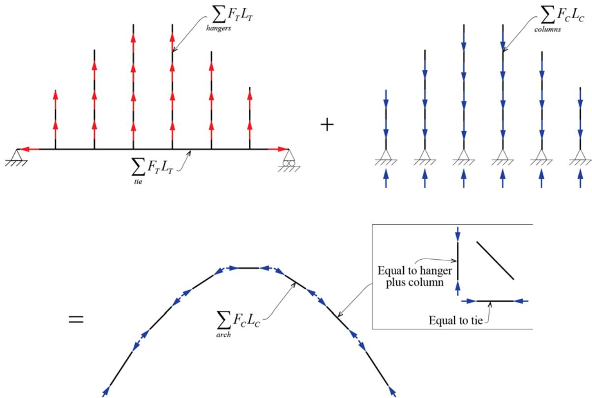
Figure 14 Calculation of load path of the arch for Exchange House
