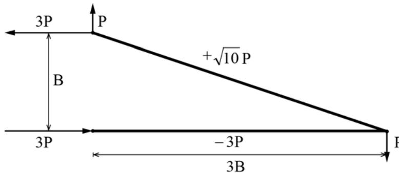
Figure 3 Truss geometry selected for shortest path, which coincides with the moment diagram
