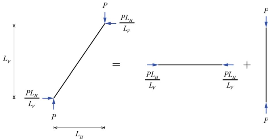
Figure 12 Segment of an arch decomposed into a horizontal and vertical component
