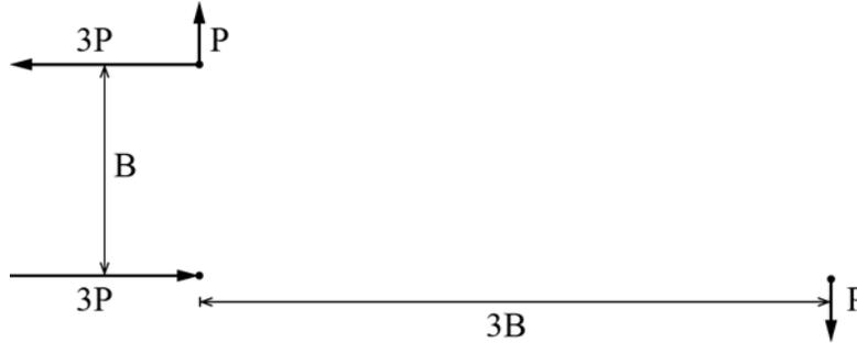
Figure 2 Illustration of Maxwell's Theorem using a 3:1 cantilever
