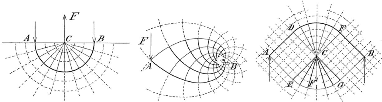
Figure 15 Minimal load path structures taken from Michell (1904): semi-infinite fan (left), orthogonal systems of equiangular spirals (center) and centrally loaded beam (right)
