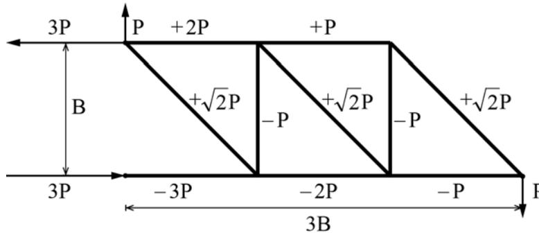
Figure 4 Geometry of a Pratt truss
