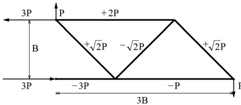
Figure 5 Geometry of a Warren truss
