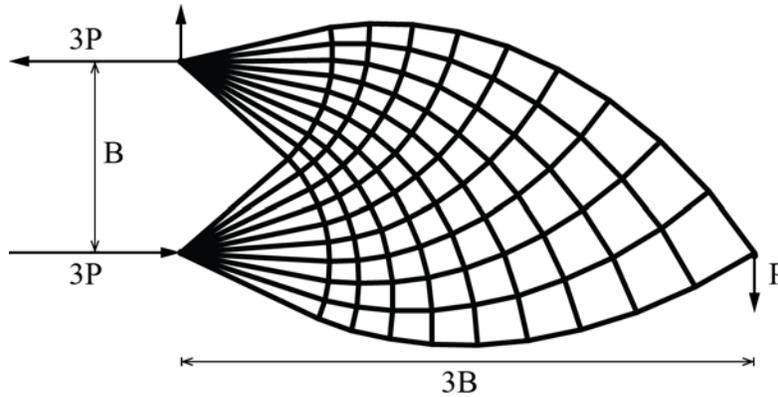
Figure 8 Optimal geometry for 3:1 cantilever based on the three-point load solution
