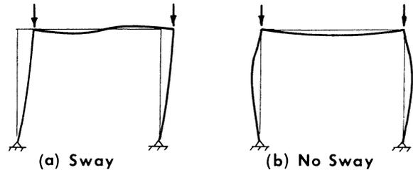
Fig. 1. Sway and no-sway buckling modes
