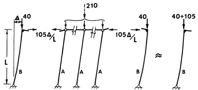
Fig. 9. Bracing force as equivalent column load
