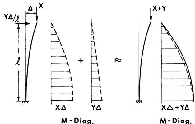
Fig. 7. Replacement of shear by equivalent axial load
