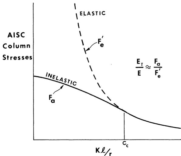
Fig. 3. AISC column stresses
