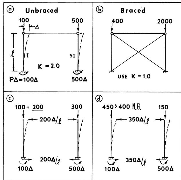
Fig. 6. Quantitative description of frame instability
