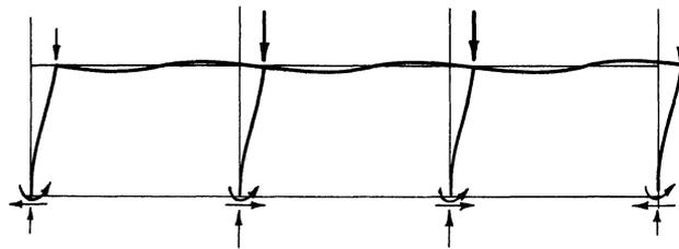
Fig. 5. Column bracing in unbraced frames
