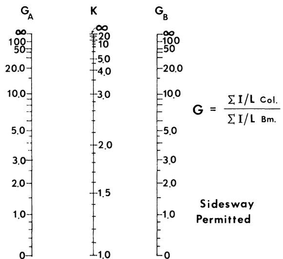
Fig. 2. Alignment chart for determining  $K$ -factors
