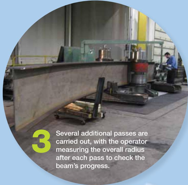
**3** Several additional passes are carried out, with the operator measuring the overall radius after each pass to check the beam's progress.
