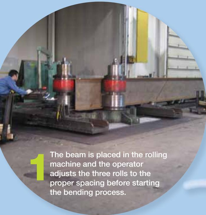
**1** The beam is placed in the rolling machine and the operator adjusts the three rolls to the proper spacing before starting the bending process.
