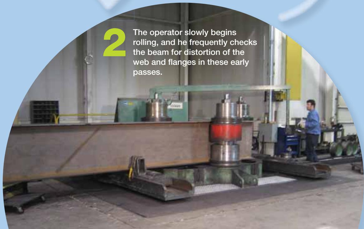
**2** The operator slowly begins rolling, and he frequently checks the beam for distortion of the web and flanges in these early passes.
