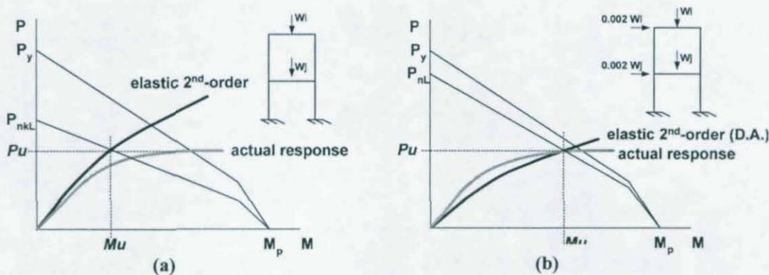
Fig. 1 – Comparison of beam-column interaction checks for (a) the effective length approach and (b) direct analysis approach
