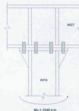
Figure 6: Example Connection Design (8-1" dia. bolts)
