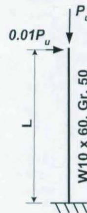
Fig. 2 – Cantilever Example
