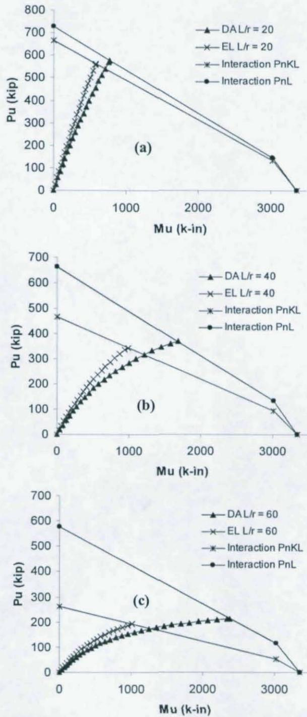
Fig. 3 – Comparison of P-M interaction curves for cantilever column example
