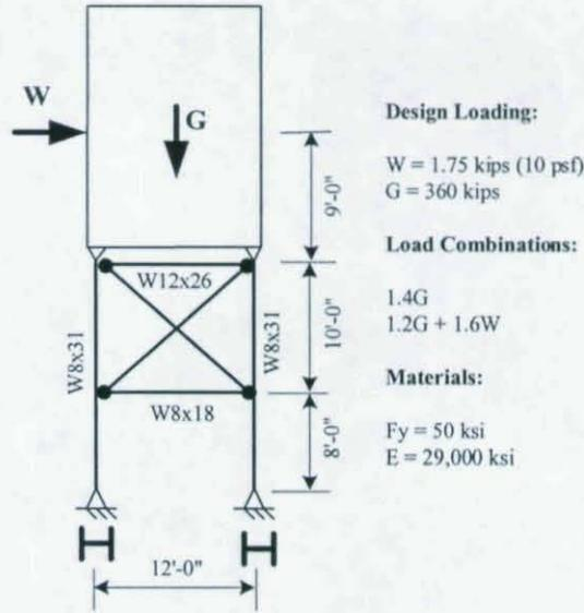
Figure 7 – Grain Bin Support Frame
