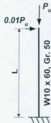
Fig. 2 – Cantilever Example
