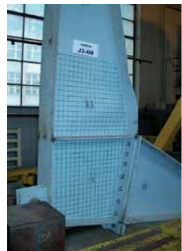
Figure 8c. Failure mode of the joint – experimental test
