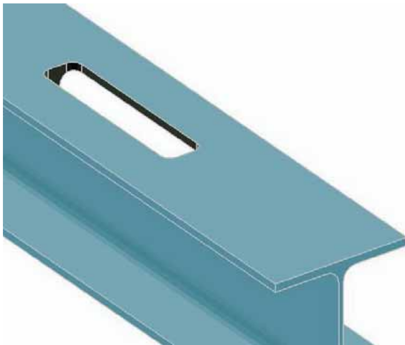
Figure 5 (b): Perspective View of Fuse From Above
