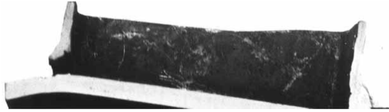
Figure 1. Fillet weld after failure
