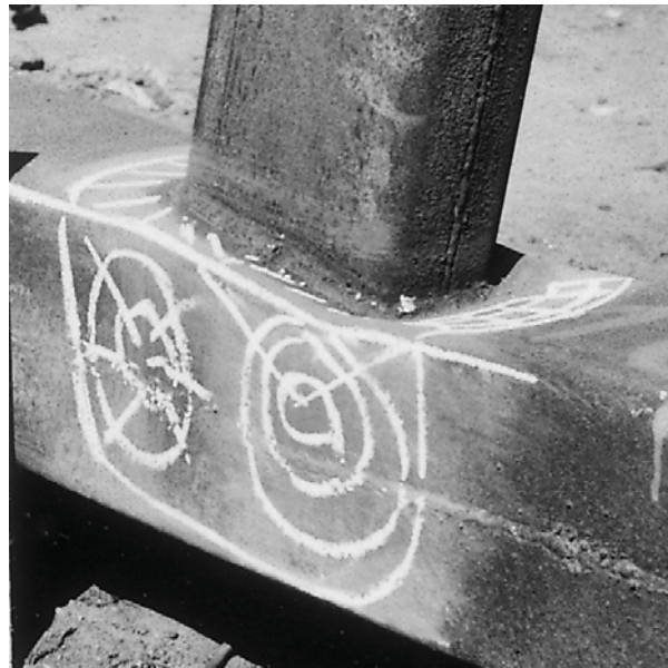
Figure 1. Fillet weld after failure
