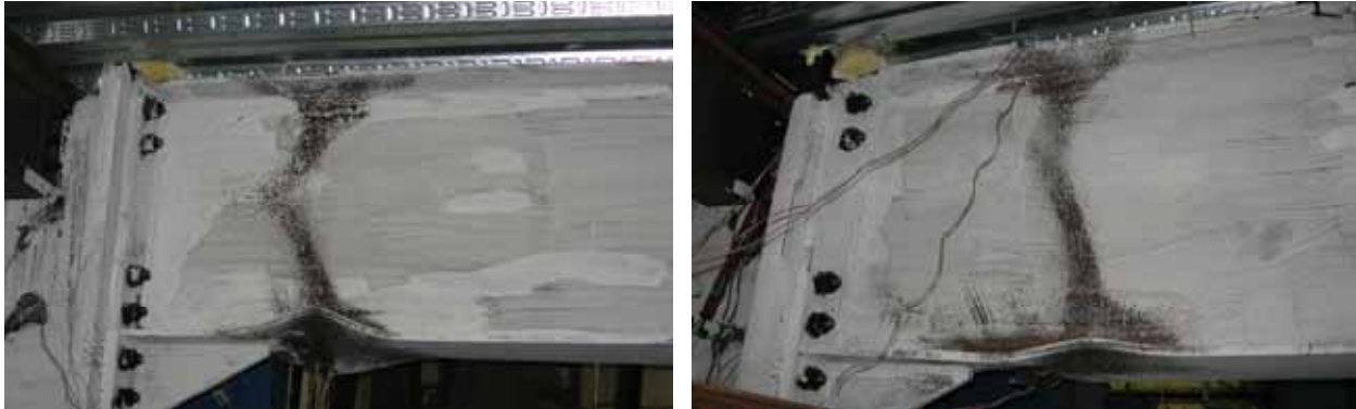
Figure 6. Yielding and Bottom Flange Buckle
