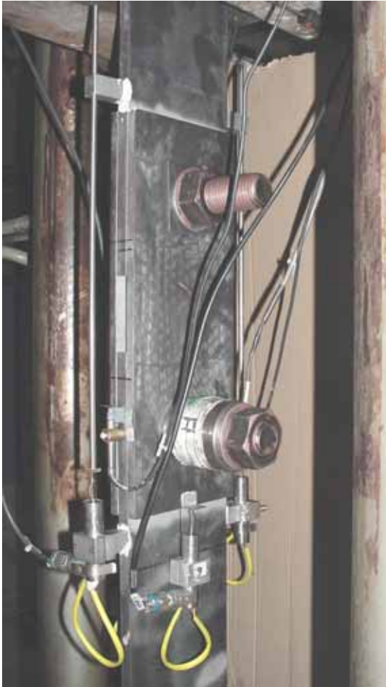
Figure 15. Test set up to measure load-deformation behaviour of preloaded connection.
