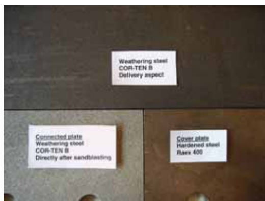
Fig. 4. visual aspect of rust free COR-TEN B
