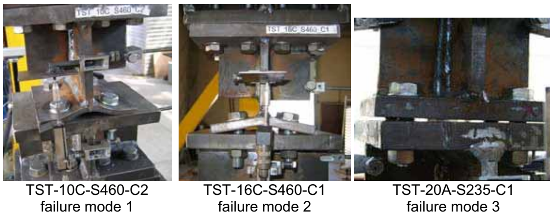
Figure 5. Examples of failure modes of T-stub specimens
