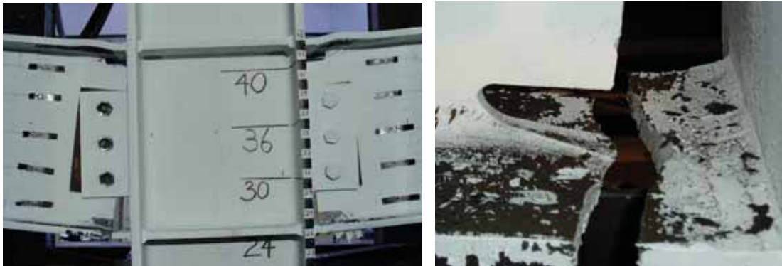
Figure 4: Failure mode of the WUF-B Test Specimen
