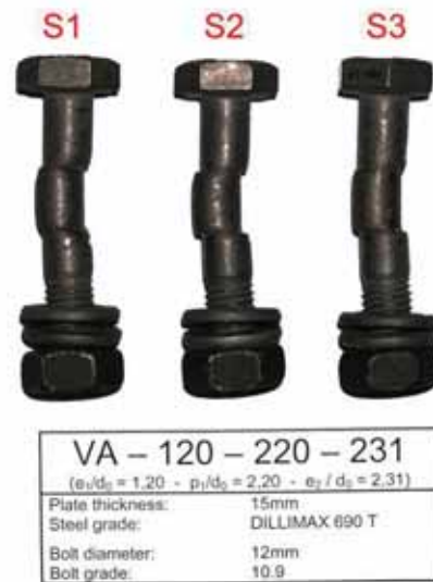
Figure 2.2: Load – displacement – curve for bolt class 10.9 and deformed bolts
