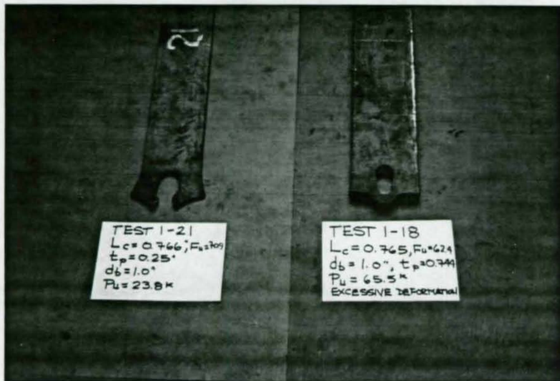
Figure 12. Specimens of Different Thickness with the Same End Distance. For the specimen on the left, t_p = 0.25 in. and F_y/F_u = 1.34 ; for the specimen on the right, t_p = 0.744 in. and F_y/F_u = 1.41 .
