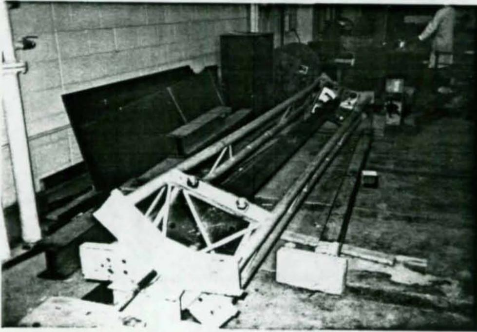
Figure 3.17 Assembly Jig for Bracing Specimens
