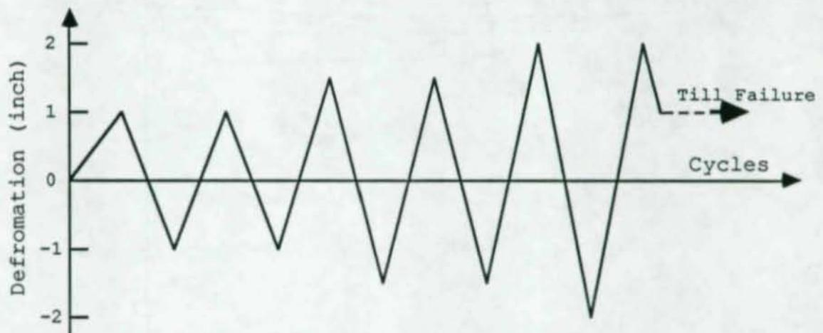
Figure 2.4 Loading History for Beam Testing
