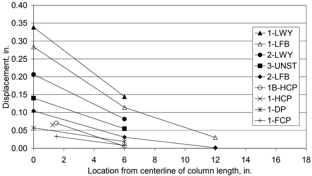
Figure 6 Column flange separation at 450 kips
