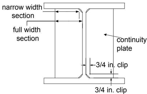
Figure 7 Narrow and full-width sections of continuity plates
