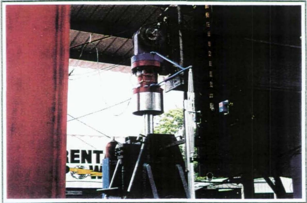
Figure 9 Photograph of Actuator and Beam End
