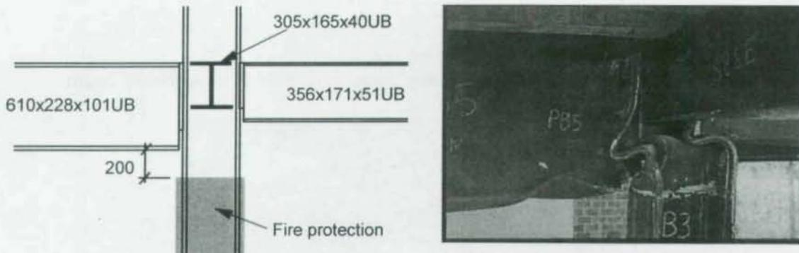
Figure 12 Extent of column fire protection and column deformation in Test 2
