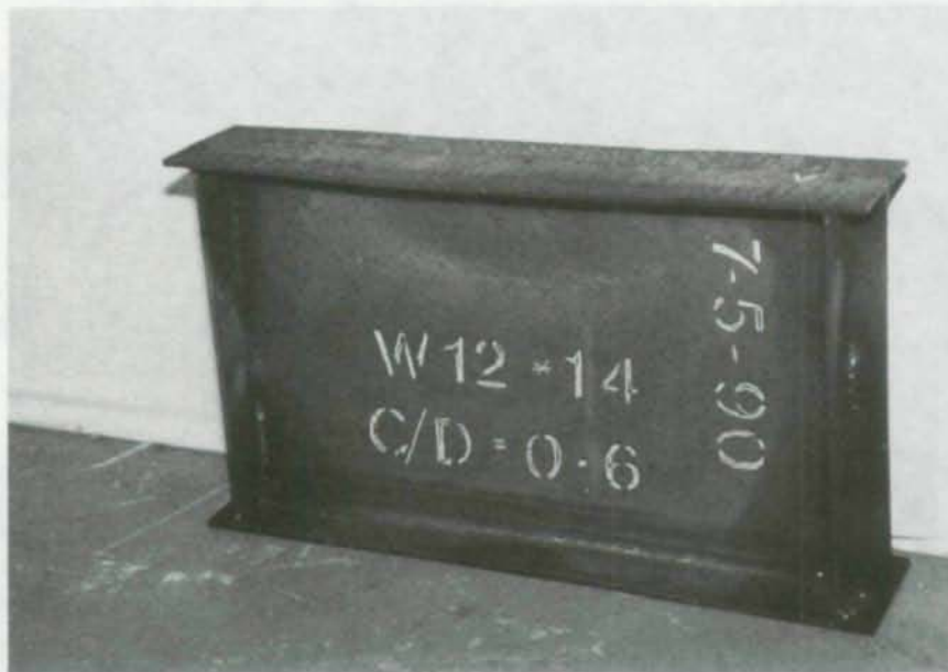
Crippling Between Supports
