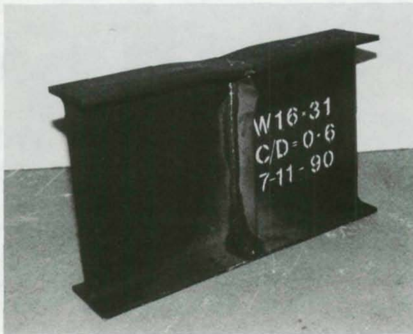
Figure (9) - Stiffener Crippling Under Load
