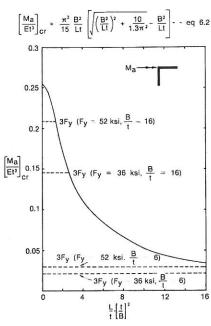
Fig.5 (a). Critical buckling curve for case I
