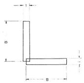
Fig.1 (b). Simplified angle section dimensions
