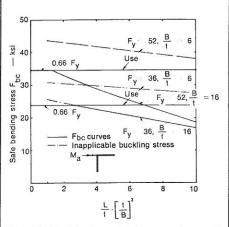
Fig.5 (b). Graph for determination of  $\boldsymbol{F}_{be}$  for case  $\boldsymbol{I}$
