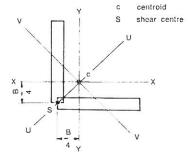
Fig.1 (a). Orientation of axes and locations of centroid and shear centre.
