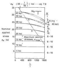
Fig.6. Graph for determination of actual max. section stress for case  $\boldsymbol{I}$
