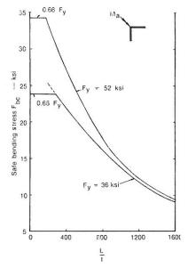
Fig.9. Critical buckling curve and curves for safe bending stress case II
