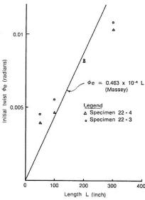
Fig.7. Initial twist  $\phi_{\rm e}$  test results for angle sections compared with Massey's relationship
