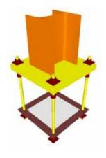
**100:** Conceptual. The Model Element may be graphically represented in the model with a symbol or other generic representation but does not satisfy the requirements for LOD 200. Information related to the Model Element (e.g., cost per square foot, tonnage of HVAC, etc.) can be derived from other Model Elements.
