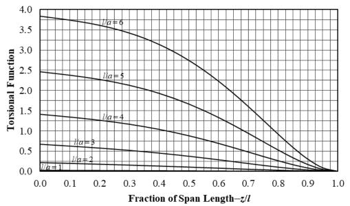
Replace the bottom graph for  $\theta' \times \left(\frac{GJ}{t} \times \frac{1}{a}\right)$  with:
