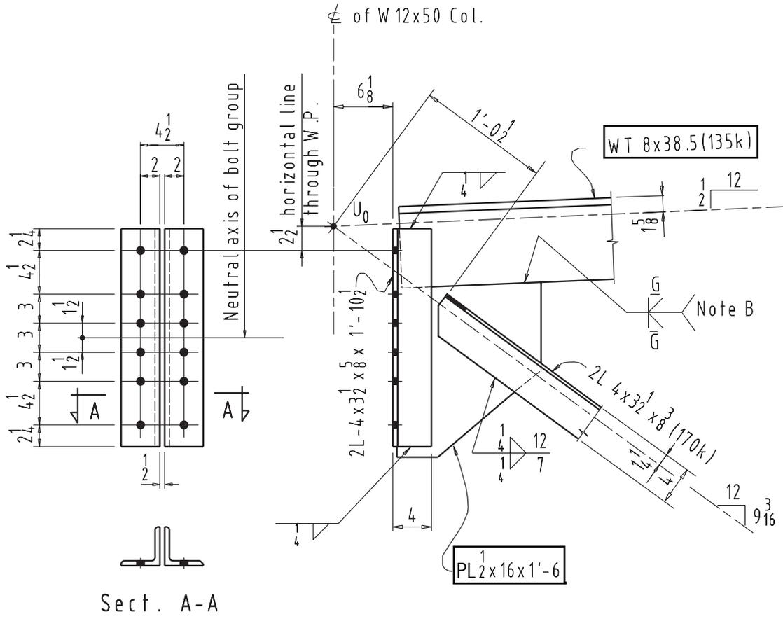
Figure 3-48. Top chord connection to column.
