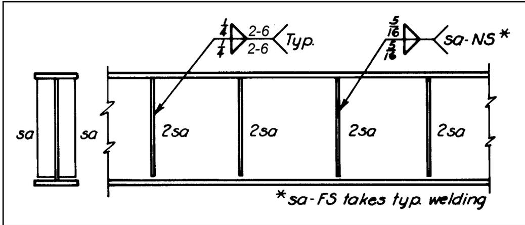
Figure 4-27. Typical welded joint.
