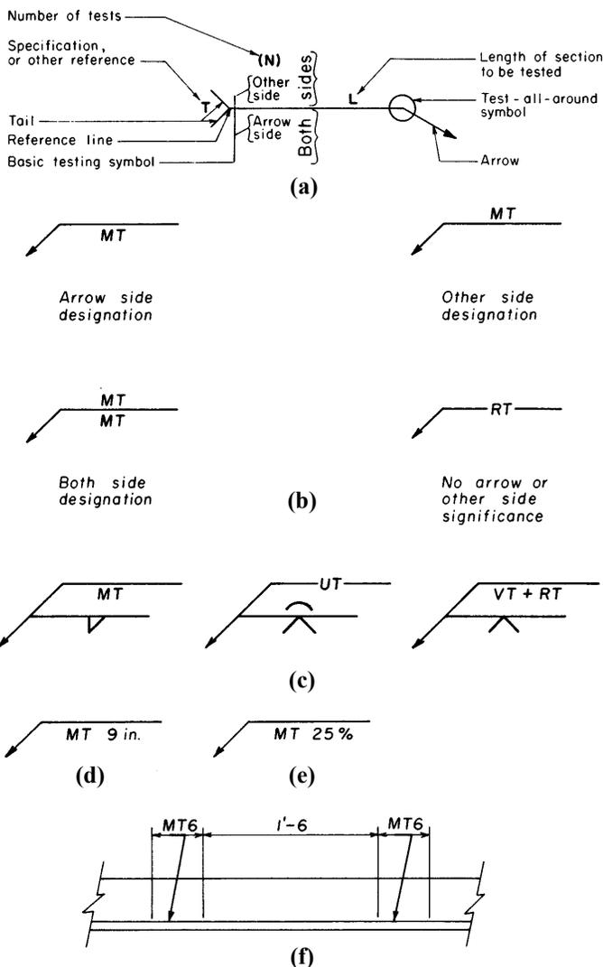
Figure 4-30. Non-destructive testing symbols combined with welding symbols.
