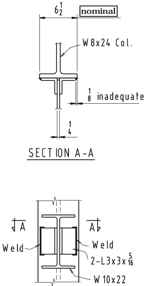
Figure 7-85. Improper connection detail.
