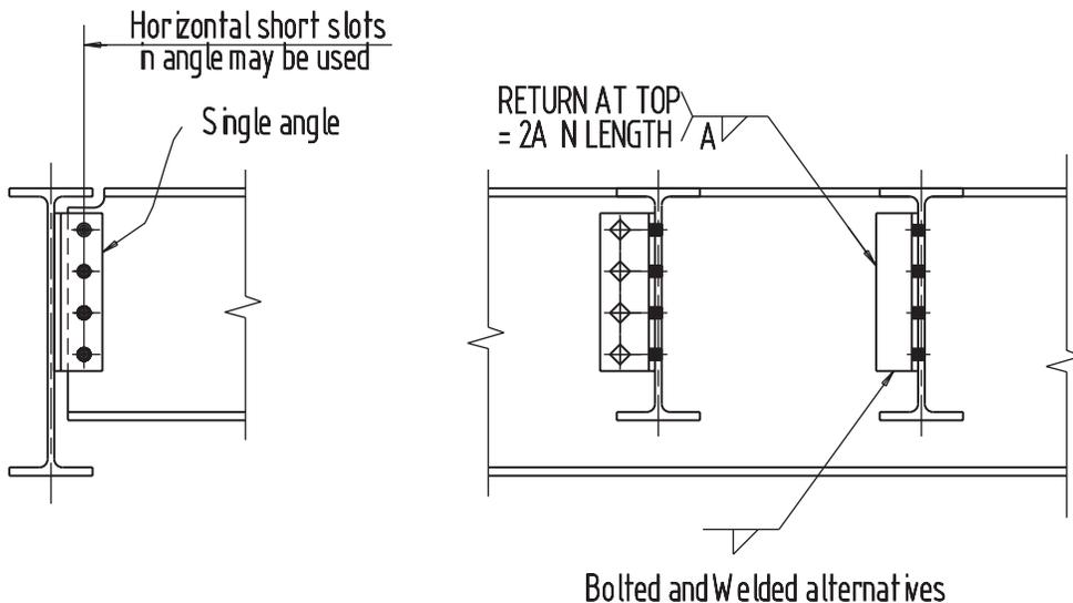
Figure 3-14. Single angle connection.
