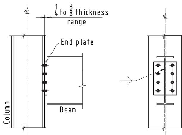
Figure 3-8. Typical end-plate connection to a column flange.
