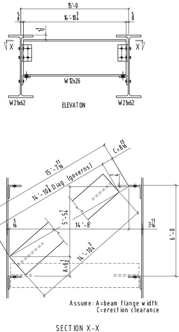
Figure 7-86. Clearance available for erecting seated filler beams where the side angle connections are to be shop-fastened to the supporting girder beams.
