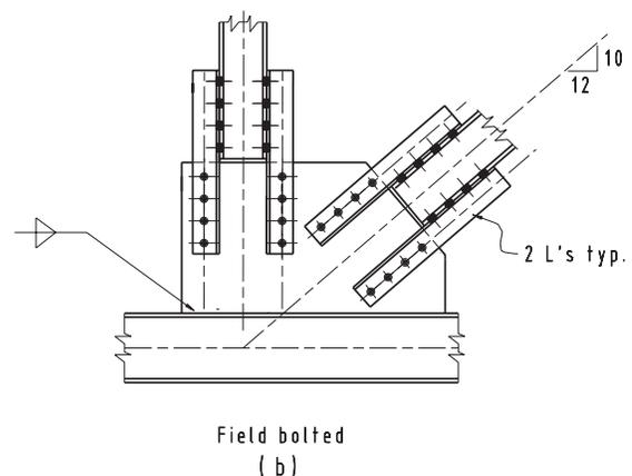
Figure 7-47. Construction of heavily loaded trusses consisting of W shapes for both chord and web members.
