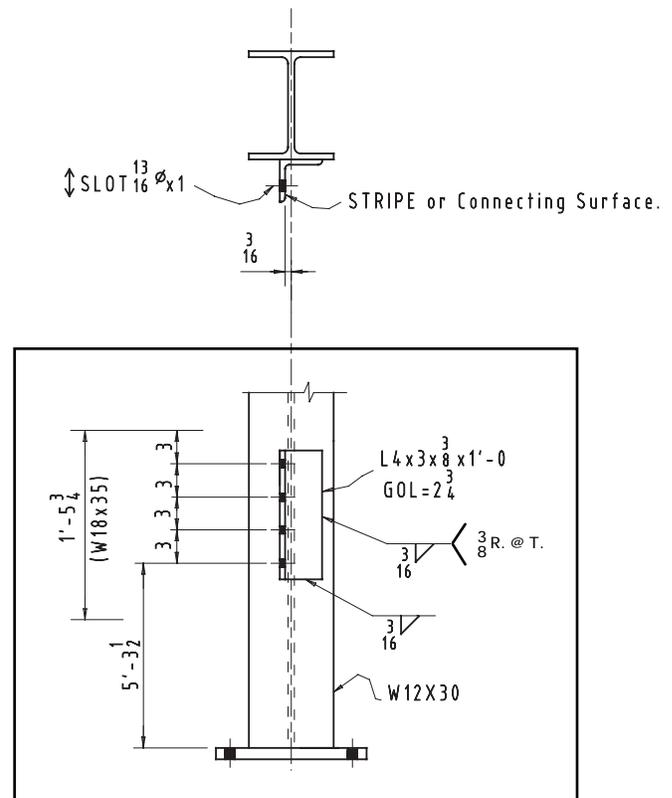
Figure 4-2. Wrap around connection use.
