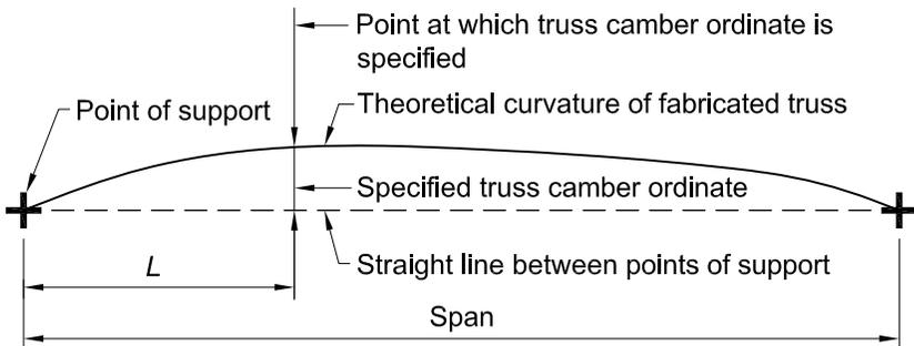
Taking  $L$  as the distance from the point at which truss camber is specified to the closer point of support, in. (mm), the tolerance on truss camber at that point is calculated as  $L/800$ .  $L$  must be equal to or less than one-half the span.
