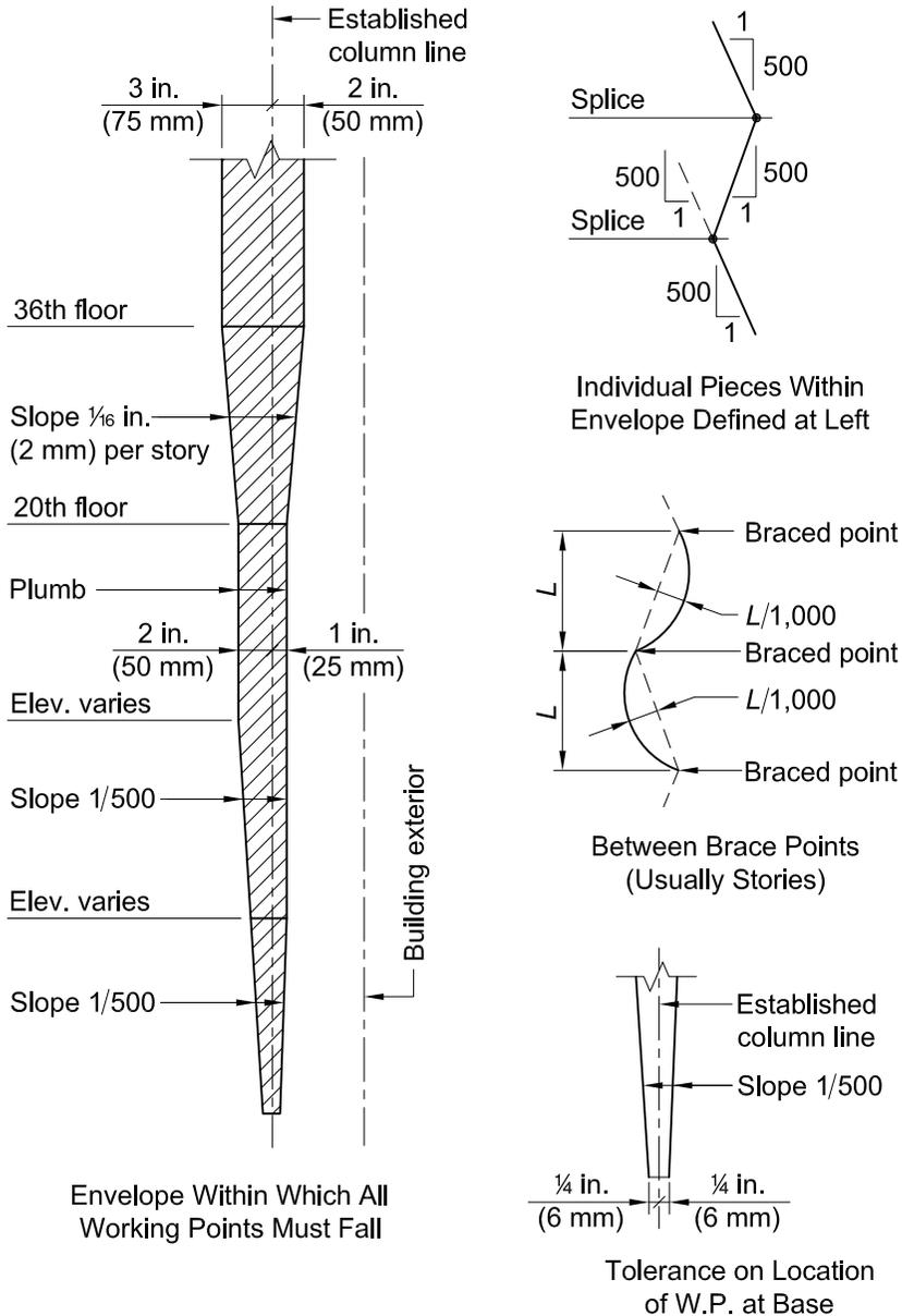
Note: The plumb line through the base working point for an individual column is not necessarily the precise plan location because Section 7.13.1.1 deals only with plumbness tolerances and does not include inaccuracies in location of the established column line, foundations, and anchor rods beyond the erector's model.
