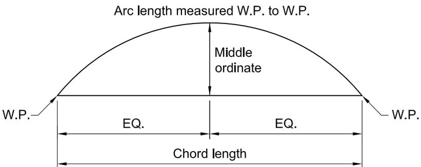
Fig. C-6.1. Illustration of the tolerance on curved structural steel member.
