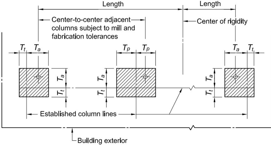
Fig. C-7.2. Tolerances in plan location of column.
