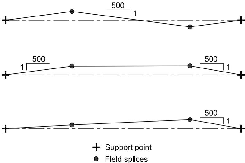
Fig. C-7.7. Alignment tolerances for members with field splices.
