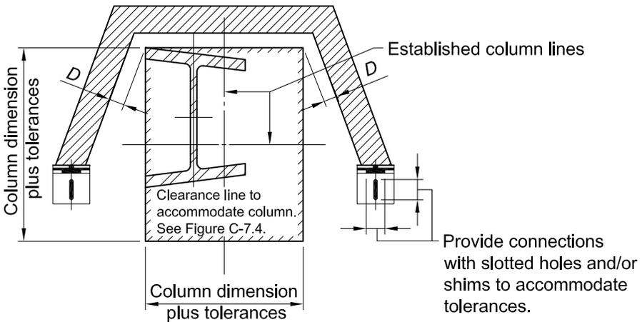
If fascia joints are set from nearest column finish line, allow  $\pm 5/8$  in. (16 mm) for vertical adjustment. The entity responsible for the fascia details must allow for progressive shortening of steel columns.
