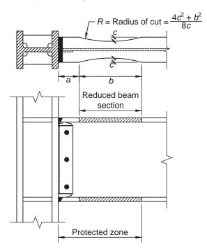
Fig. 5.1. Reduced beam section connection.
