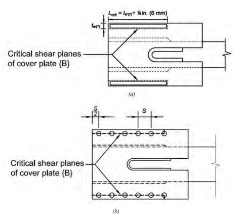
Fig. C-11.8. Critical shear plane of cover plate {B}, (a) field-welded connection; (b) field-bolted connection
