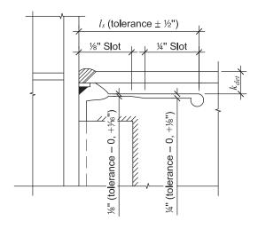
Fig. 14.3. Slot widths and tolerances.
