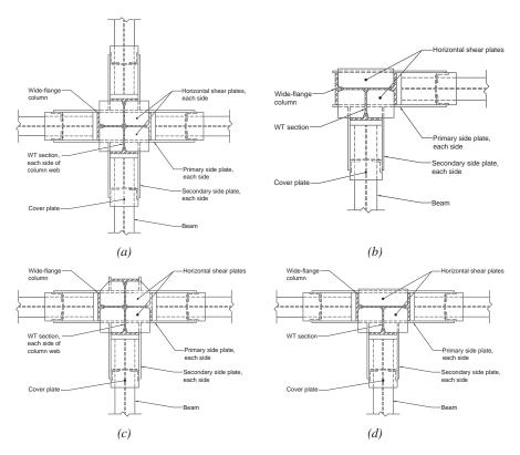
Fig. 11.5. SidePlate biaxial dual strong-axis configurations in plan view: (a) full four-sided wide-flange column configuration; (b) corner two-sided wide-flange column configuration with single WT; (c) tee three-sided wide-flange column configuration with double WT (primary); and (d) tee three-sided wide-flange column configuration with single WT.
