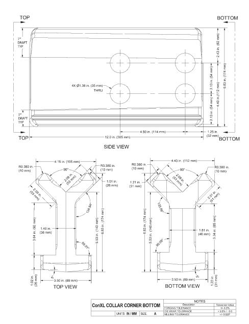
Fig. 10.14. Forged collar corner bottom (CCB).
