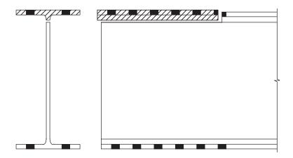
Fig. 13.7. Alternate block shear mechanism.
