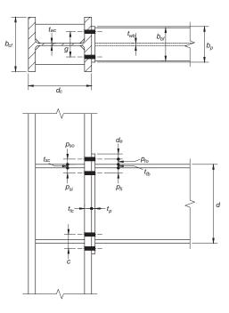
Fig. 6.2. Four-bolt unstiffened extended end-plate (4E) geometry.
