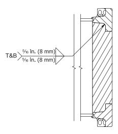
Fig. 10.8. Collar-web-extension-to-collar-flange welds, elevation.
