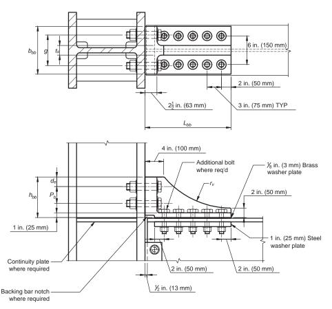
Fig. 9.5. B-series connection detailing.
