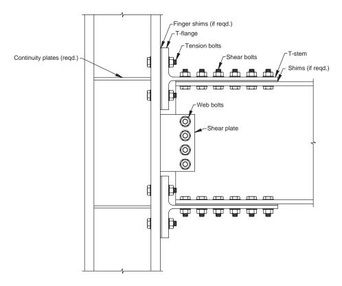
Fig. 13.1. Typical double-tee connection.
