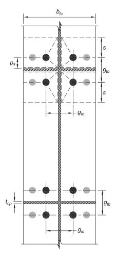
Fig. 13.8. Dimension for yield-line analysis of column flange.
