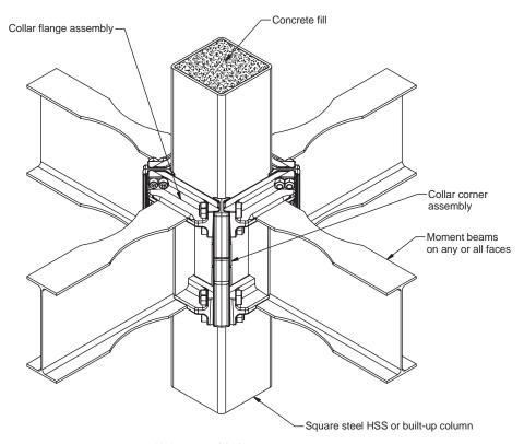
Fig. 10.1. Assembled ConXL moment connection.
