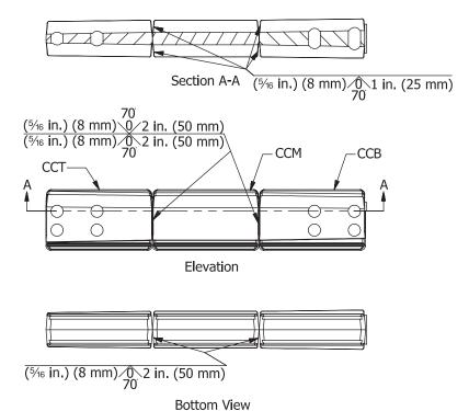
Fig. 10.6. Collar corner assembly welding.
