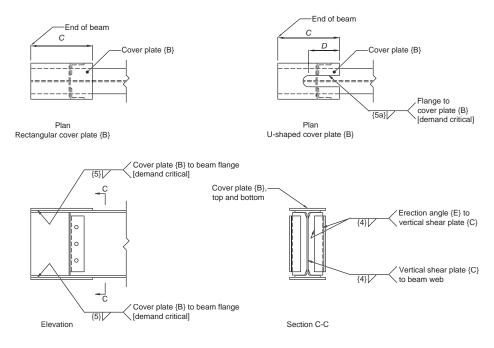
Fig. 11.14. Beam shop detail (field-welded).
