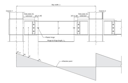
Fig. 11.6. Plastic hinge location and hinge-to-hinge length.
