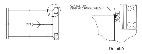
Fig. 10.9. Collar-flange-assembly-to-beam welds, elevation.
