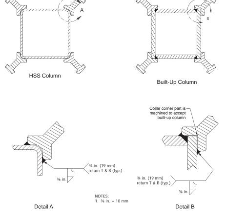
Fig. 10.7. Collar-corner-assembly-to-column weld, plan view.
