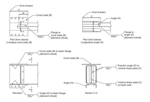
Fig. 11.15. Beam shop detail, field-bolted standard (configuration A).
