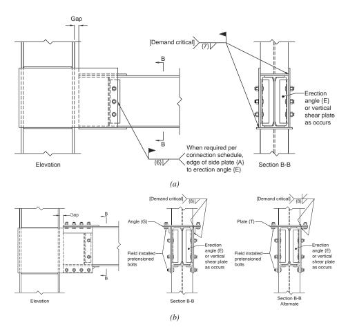
Fig. 11.16. Beam-to-side plate field erection detail: (a) elevation and section B-B, field-welded; (b) elevation and section B-B, field-bolted standard (configuration A).
