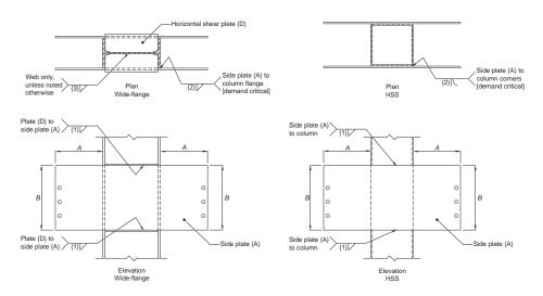
Fig. 11.12. Two-sided SidePlate moment connection (B-type), column shop detail.
