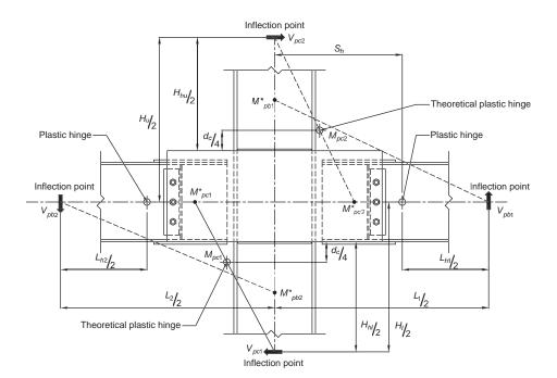
Fig. 11.10. Force and distance designations for computation of column-beam moment ratios.
