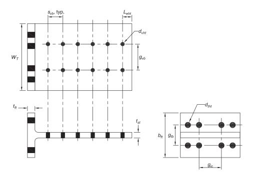
Fig. 13.5. T-stub dimensions for double-tee connections.
