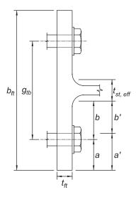
Fig. 13.6. T-stub flange dimensions for double-tee connections.
