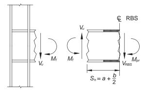
Fig. 5.2. Free-body diagram between center of RBS and face of column.
