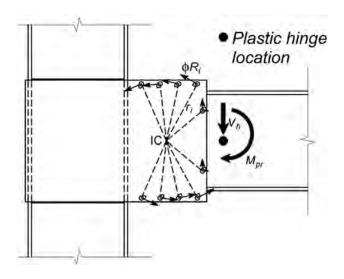
Fig. C-11.11. Instantaneous center of rotation of a sample bolt group.
