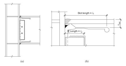
Fig. 14.1. SW Beam-to-column moment connection.
