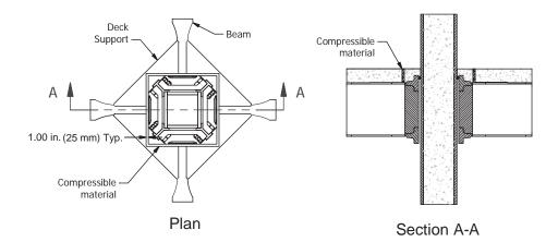
Fig. 10.4. Use of compressible material to isolate structural slab from connection.
