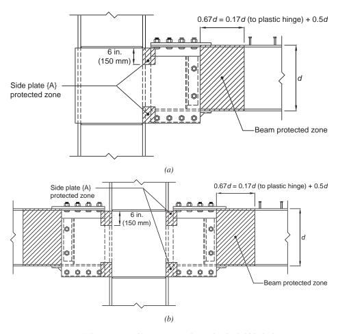
Fig. 11.8. Location of beam protected zone for the field-bolted connection: (a) one-sided connection; (b) two-sided connection.
