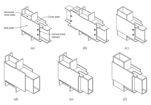
Fig. 11.1. Assembled SidePlate uniaxial field-welded configurations: (a) one-sided wide-flange beam and column construction; (b) two-sided wide-flange beam and column construction; (c) wide-flange beam to either HSS or built-up box column; (d) HSS beam without cover plates to wide-flange column; (e) HSS beam with cover plates to wide-flange column; and (f) HSS beam with cover plates to either HSS or built-up box column.
