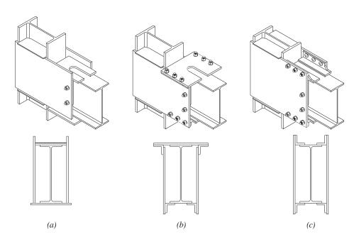
Fig. 11.3. SidePlate field-welded and field-bolted connection comparison: (a) typical field-welded connection; (b) typical field-bolted standard connection (configuration A); and (c) typical field-bolted narrow connection (configuration B).
