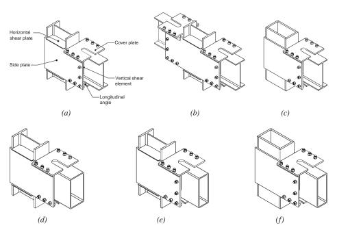
Fig. 11.2. Assembled SidePlate uniaxial field-bolted standard configurations (configuration A): (a) one-sided wide-flange beam and column construction; (b) two-sided wide-flange beam and column construction; (c) wide-flange beam to either HSS or built-up box column; (d) HSS beam to wide-flange column; (e) HSS beam with cover plate to wide-flange column; and (f) HSS beam with cover plates to either HSS or built-up box column.
