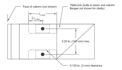
(b) Buckling restraint spacer plate placement
