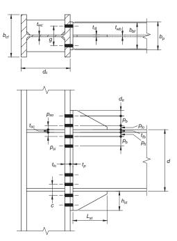
Fig. 6.4. Eight-bolt stiffened extended end-plate (8ES) geometry.
