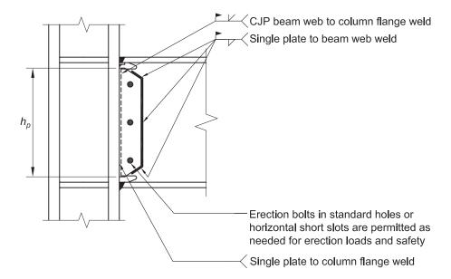
Fig. 8.2. General details of beam web-to-column flange connection.
