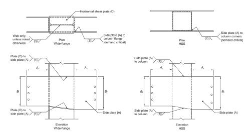
Fig. 11.13. Two-sided SidePlate moment connection (C-type), column shop detail.
