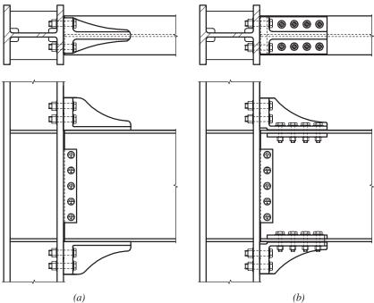
Fig. 9.1. Kaiser bolted bracket connection.
