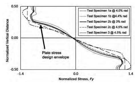
Fig. C-11.5. Stress profile along depth of side plate {A} at the column face at maximum load cycle.
