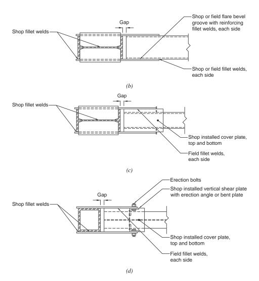
Fig. 11.4(b-d). SidePlate uniaxial configuration geometry and major components: (b) HSS beam without cover plates to wide-flange column, plan view; (c) HSS beam with cover plates to wide-flange column, plan view; and (d) wide-flange beam to built-up box column, plan view.
