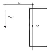
Fig. 14.4. Eccentrically loaded weld group.
