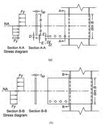
Fig. C-11.7. (a) Side plate {A} elevation view and stress diagram at the net section; (b) side plate {A} elevation view and stress diagram at the column face configuration A (standard).
