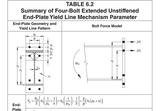
**Step 9.** Check shear rupture of the extended portion of the end-plate in the four-bolt extended unstiffened end-plate (4E):
