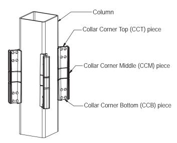
Fig. 10.2. Column with attached collar corner assemblies.
