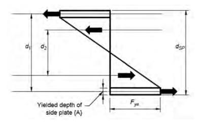
Fig. C-11.6. Idealized plastic stress distribution for computation of the effective plastic modulus, Z<sub>eff</sub>, of the side plate.
