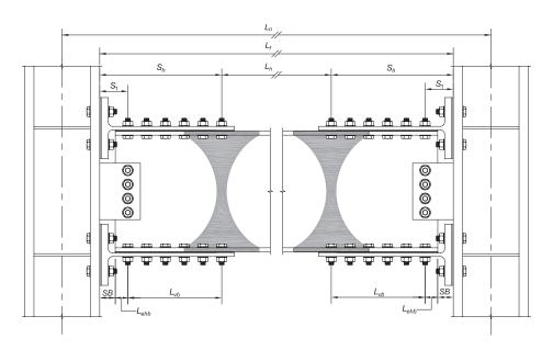
Fig. 13.2. Beam dimensions for double-tee connections.
