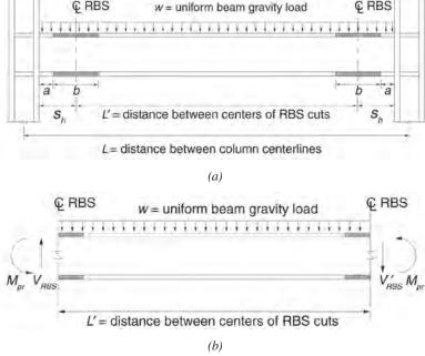
Fig. C-5.1. Example calculation of shear at center of RBS cuts: (a) beam with RBS cuts and uniform gravity load; (b) free-body diagram of beam between RBS cuts and calculation of shear at RBS.
