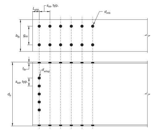
Fig. 13.4. Additional beam dimensions for double-tee connections.
