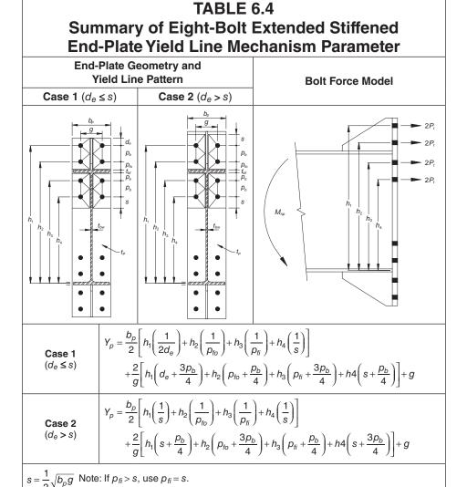
The stiffener-to-beam-flange and stiffener-to-end-plate welds shall be designed to develop the stiffener plate in shear at the beam flange and in tension at the end-plate. Either fillet or CJP groove welds are suitable for the weld of the stiffener plate to the beam flange. CJP groove welds shall be used for the stiffener-to-end-plate weld. If the end-plate is  $\frac{3}{2}$  in. (10 mm) thick or less, double-sided fillet welds are permitted.
