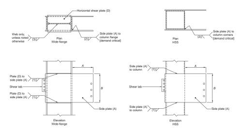
Fig. 11.11. One-sided SidePlate moment connection (A-type), column shop detail.
