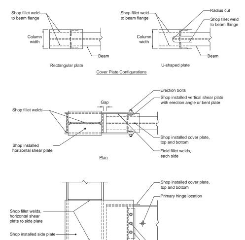
Fig. 11.4(a). SidePlate uniaxial configuration geometry and major components: typical wide-flange beam to wide-flange column, detail, plan and elevation views.
