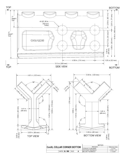
Fig. 10.18. Cast collar corner bottom (CCB).
