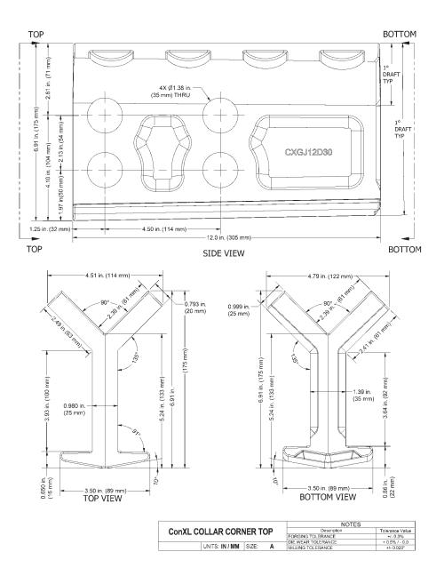
Fig. 10.16. Cast collar corner top (CCT).
