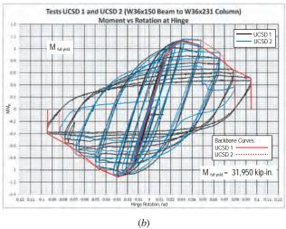
Fig. C-11.2(a–b). SidePlate moment frame tests—backbone curves for (a) W40×294 (W1000×438) beam (field-welded); (b) W36×150 (W920×223) beam (field-welded) (measured at the beam hinge location).
