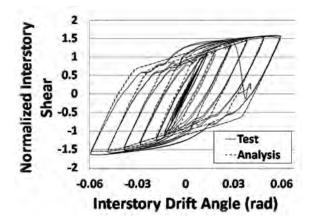
Fig. C-12.1 Testing vs. FEA analysis for frame modeled with all material nonlinearity in the Yield-Link elements.
