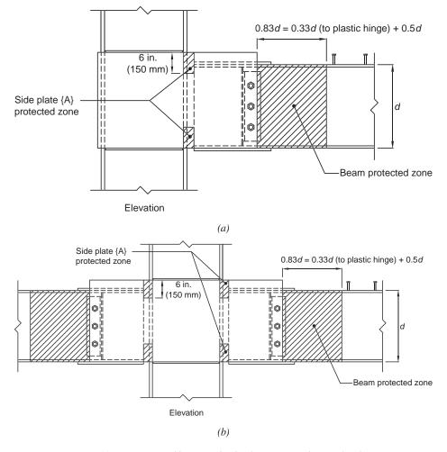
Fig. 11.7. Location of beam and side plate protected zones for the field-welded connection: (a) one-sided connection; (b) two-sided connection.
