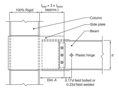
Fig. 11.17. Modeling of component stiffness for linear-elastic analysis.
