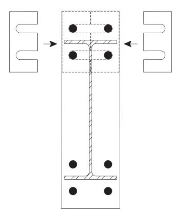
Fig. 6.6. Typical use of finger shims.
