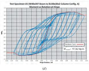
Fig. C-11.2(c-d). SidePlate moment frame tests—backbone curves for (c) W40×211 (W1000×314) beam (field-bolted); (d) W40×397 (W1000×591) beam (field-bolted) (measured at the beam hinge location).
