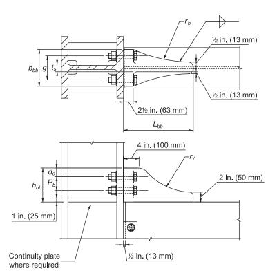
Fig. 9.4. W-series connection detailing.
