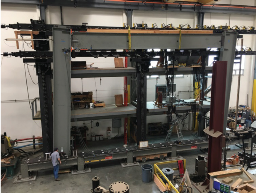
Fig. C-12.1. Testing new largest Link size with 6-in. 2 (3900 mm 2 ) yield area.
