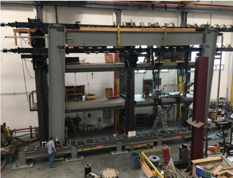
*Fig. C-12.1. Testing new largest Link size with 6 in.<sup>2</sup> yield area.*
