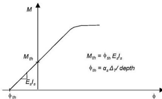
Fig. C-A-N9.2.8. Relationship between moment and thermal gradient.
