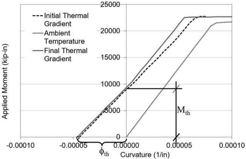
Fig. C-A-N9.2.7. Comparison of fiber model moment curvature to transformed cracked and fully cracked moment of inertia (Varma et al., 2009).
