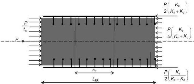
Fig C-A-N9.1.13. Load applied to concrete only, resisted by composite section.
