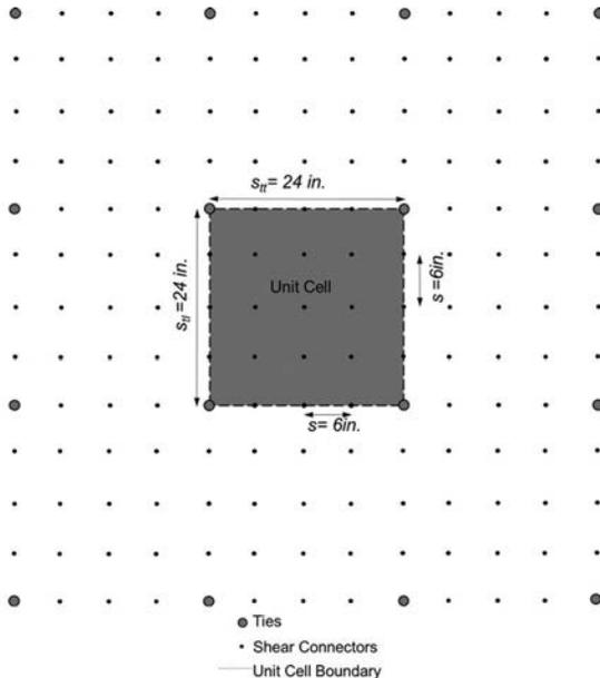
Fig. C-A-N9.3.7. Unit cell for calculating  $Q_{cv}^{avg}$ .
