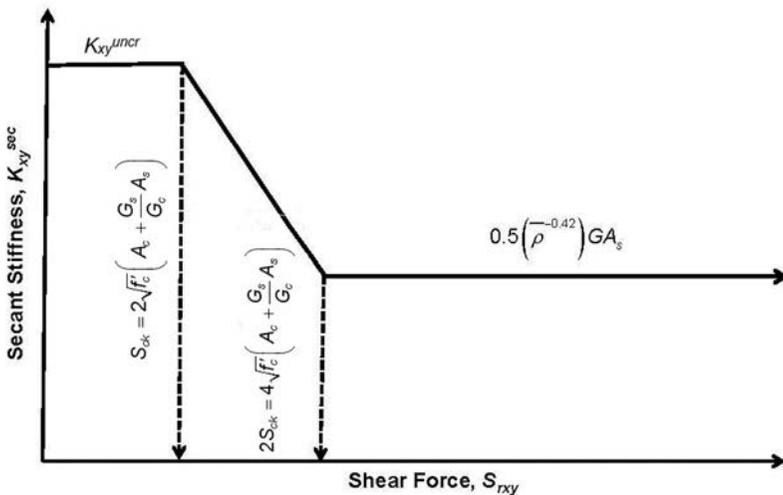
Fig. C-A-N9.2.5. A simple model for secant stiffness with no accident thermal loading (Varma et al., 2011a).
