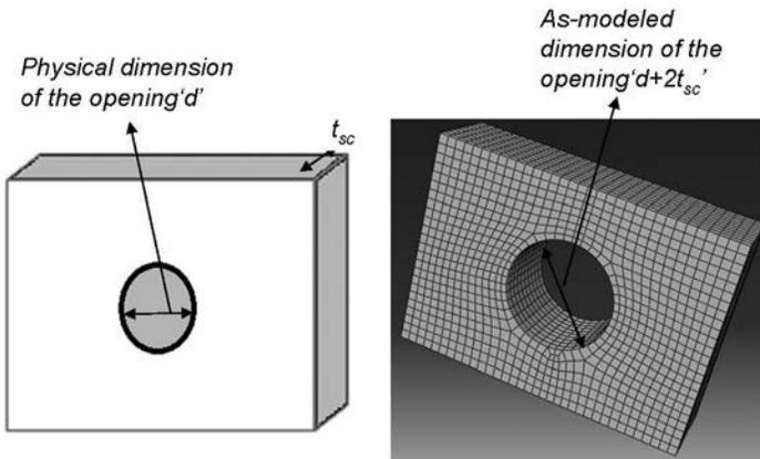
Fig. C-A-N9.1.23. Modeling of large openings with free edge at opening perimeter.
