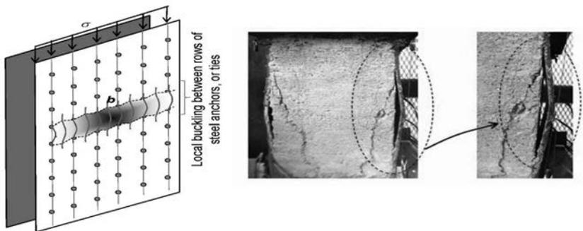
Fig. C-A-N9.1.5. The buckling mode of the faceplate (Zhang et al., 2014).
