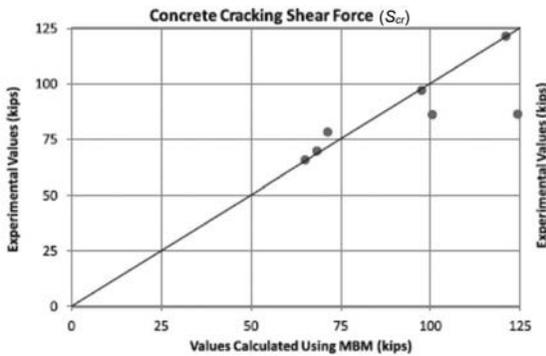
Fig. C-A-N9.2.3. Experimental versus calculated values of cracking strength (Varma et al., 2014).
