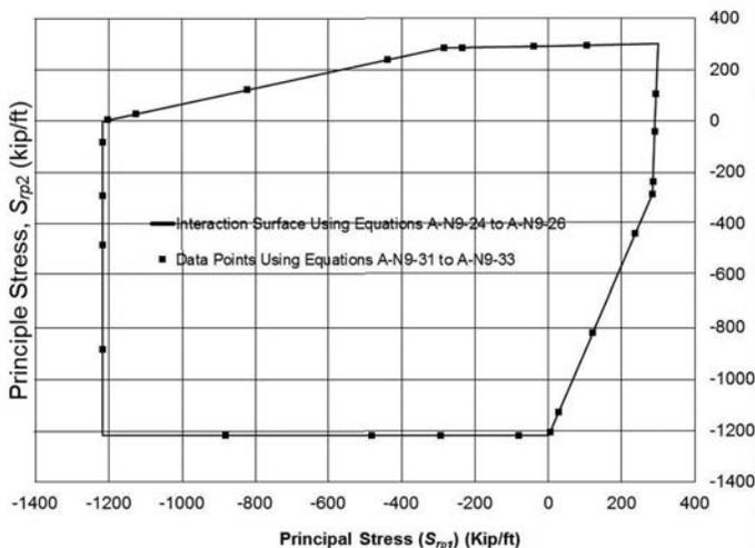
Fig. C-A-N9.3.12. Interaction surface and data points using alternate forms of interaction equations.
