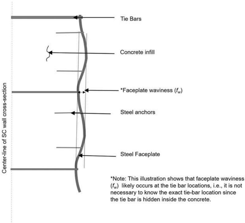
*Fig. C-NM2.1. Faceplate waviness. (The faceplate waviness and the variation in tie-bar dimensions has been exaggerated for illustration purposes.)*
