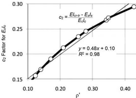
Fig. C-A-N9.2.2. Calibration of  $c_2$  versus  $\rho'$  (Varma et al., 2011a).
