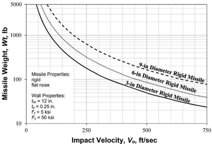
Fig. C-A-N9.1.18. Nondeformable (rigid) missile resistance of minimum SC wall.
