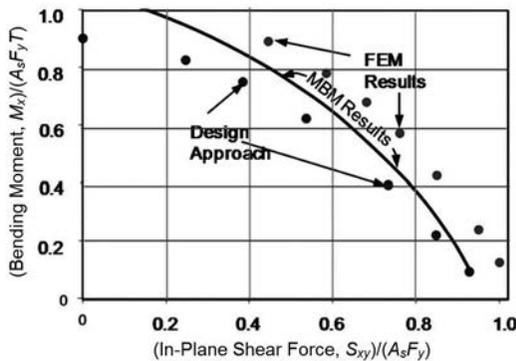
Fig. C-A-N9.3.11. Moment-shear interaction for SC wall (Varma et al., 2014).
