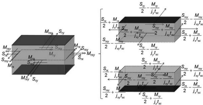
Fig. C-A-N9.3.8. Combined forces acting on panel section and notional halves (Varma et al., 2014).
