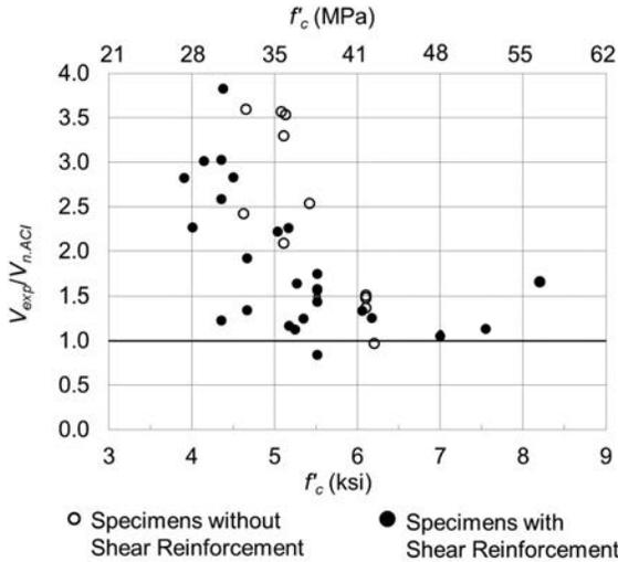
Fig. C-A-N9.1.2. Range of concrete compressive strength from experimental database.
