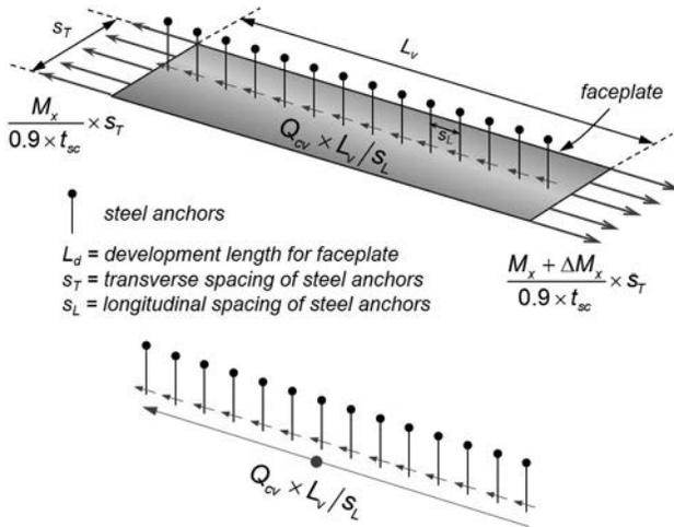
(b) Free body diagram of the bottom faceplate in tension
