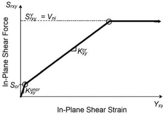
Fig. C-A-N9.3.3. In-plane shear strain curve (Varma et al., 2011b).
