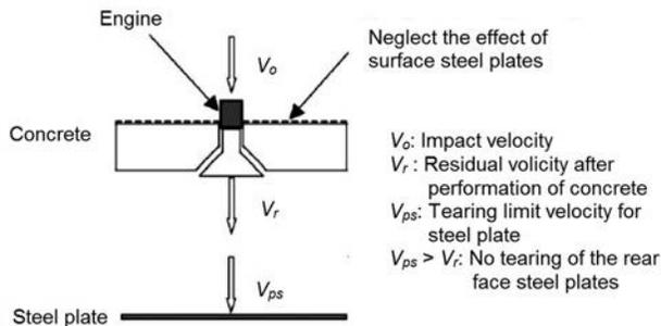
Fig. C-A-N9.1.16. Evaluation procedure for tearing of SC panels against impact (Mizuno et al., 2005).
