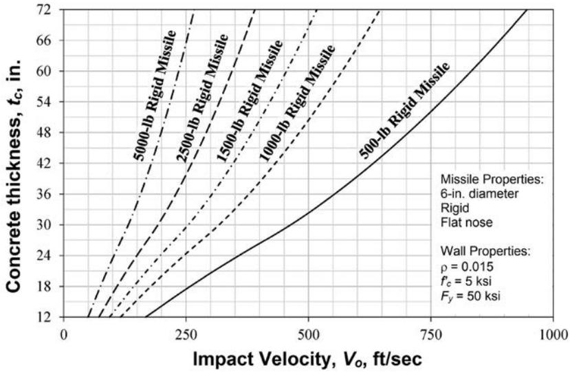
(a) 6-in.-diameter, flat-nose, rigid missile, 0.015 reinforcement ratio
