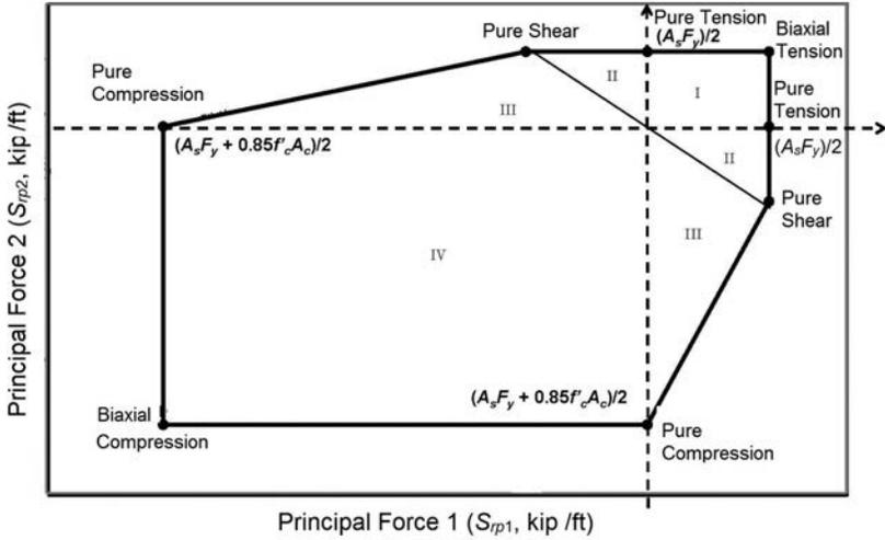
Fig. C-A-N9.3.9. Interaction surface for in-plane forces in principal force space (Varma et al., 2014).
