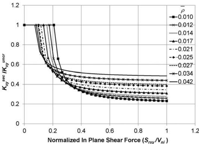
Fig. C-A-N9.2.4. Variation of secant stiffness of SC walls (Varma et al., 2011a).
