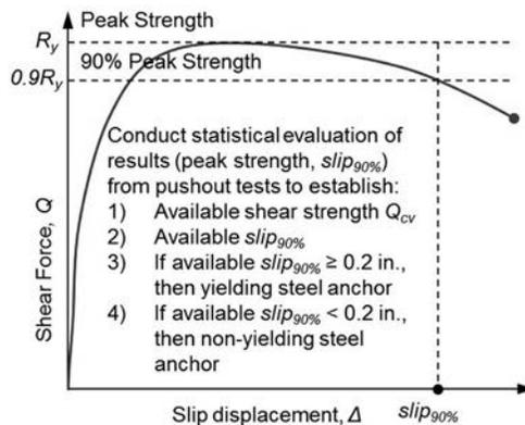
Fig. C-A-N9.1.7. Typical steel anchor force-slip behavior from pushout tests.
