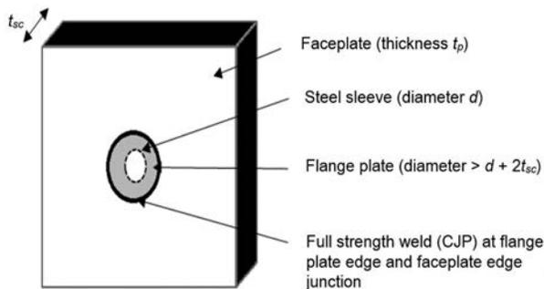
Fig. C-A-N9.1.22. Small circular opening—detailing illustration for fully developed edge with flange plate thickness  $\geq 1.25t_p$ .
