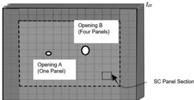
\*Depending on the degree of mesh refinement, the SC panel section may/may not be the same as the element in the FE mesh
