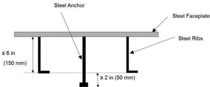
Fig. C-A-N9.1.3. Embedment depth of steel ribs.
