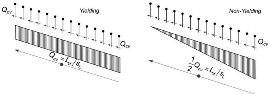
Fig. C-A-N9.1.10. Interfacial shear resistance of yielding and nonyielding steel anchors (LRFD).
