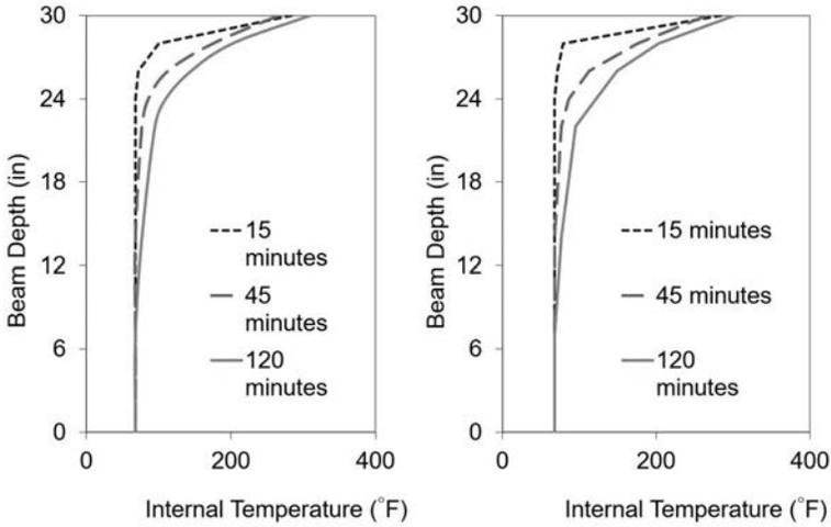
(a) Analytically determined thermal gradient      (b) Experimentally determined thermal gradient (fiber model)
