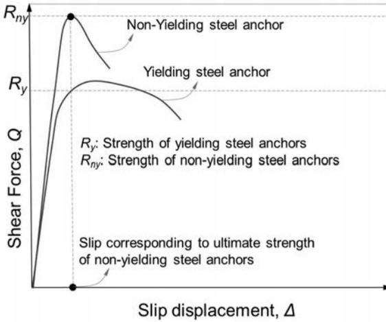
Fig. C-A-N9.1.8. Strength of yielding steel anchors that form a part of nonyielding steel anchor systems.
