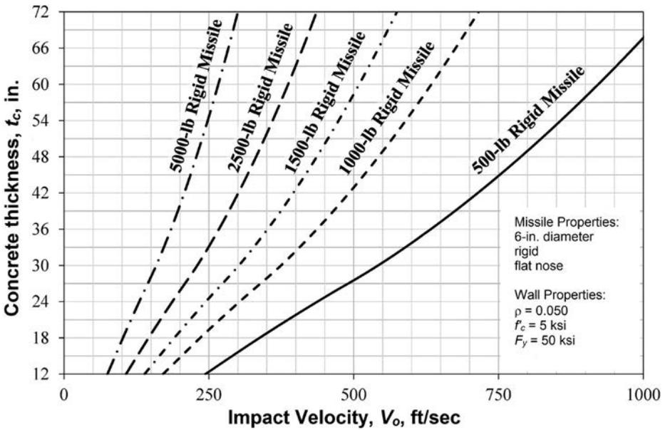
(b) 6-in.-diameter, flat-nose, rigid missile, 0.050 reinforcement ratio
