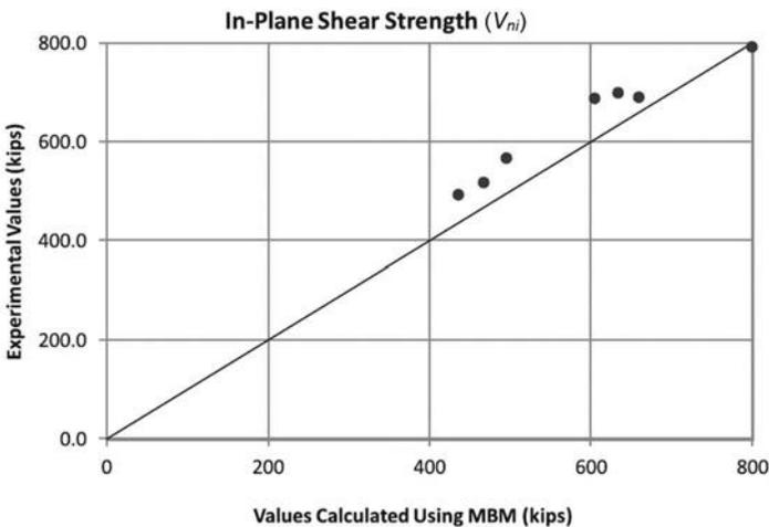
Fig. C-A-N9.3.5. Experimental versus calculated values of in-plane shear strength (Varma et al., 2014).
