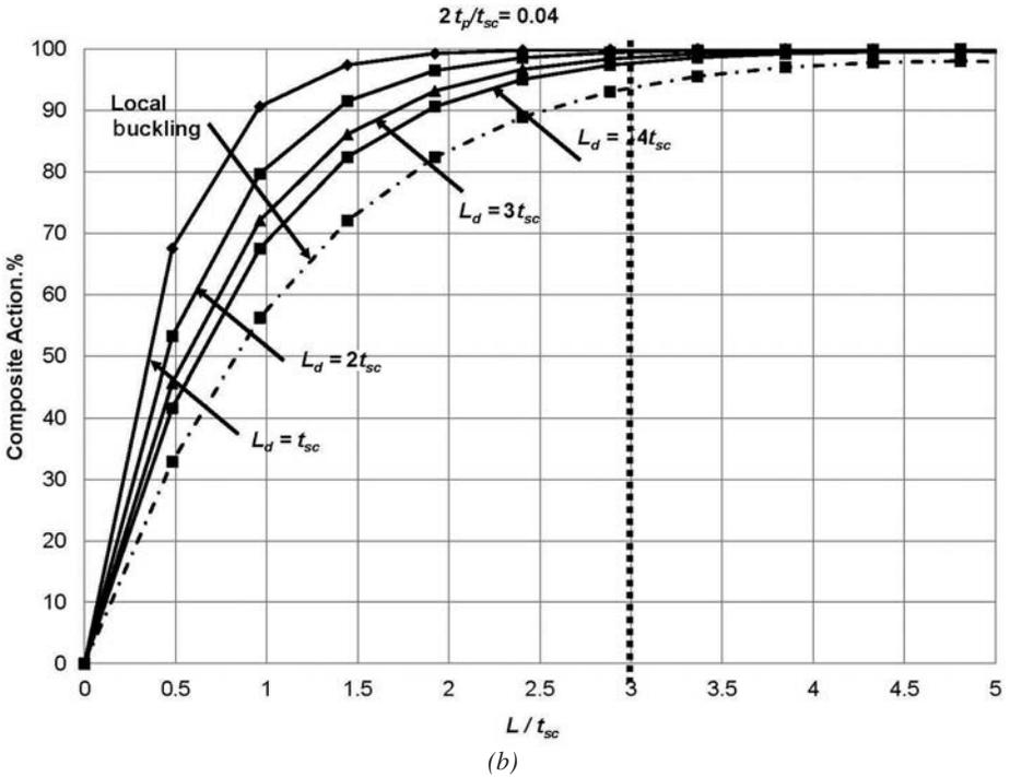
Fig. C-A-N9.1.12. Development of strain compatibility with distance from member end (Zhang et al., 2014).
