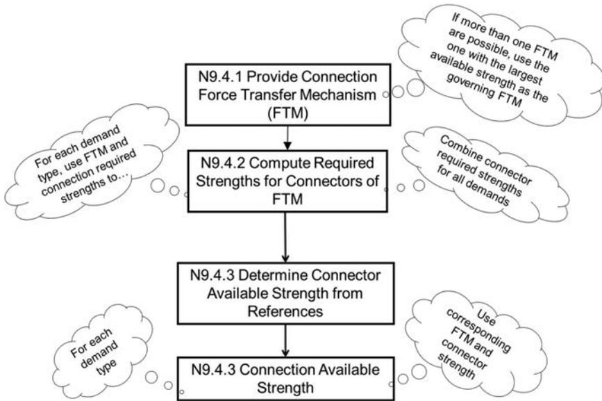
Fig. C-A-N9.4.2. Calculation of connection available strength.
