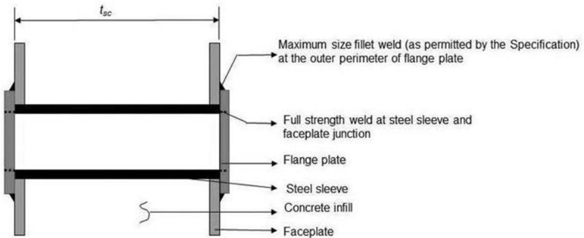
Fig. C-A-N9.1.21. Small circular opening—detailing illustration for fully developed edge with flange plate thickness  $\leq 1.25t_p$ .
