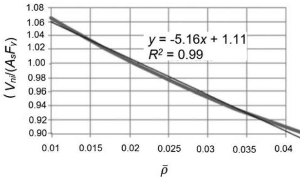
Fig. C-A-N9.3.4. Calibration of  $\bar{\rho}$  versus  $(V_{ni}/A_s F_y)$
