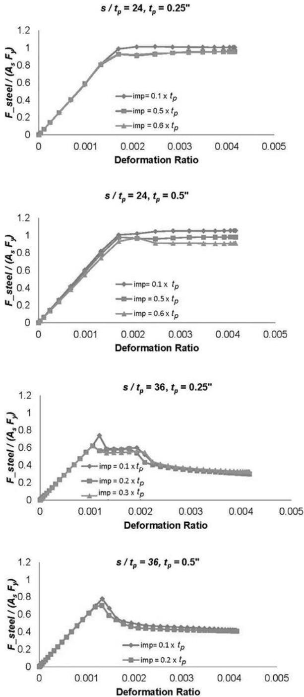
Fig. C-NM2.2. Normalized force carried by faceplates versus average strain.
