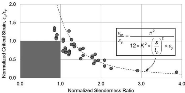
Fig. C-A-N9.1.6. The relationship between buckling strain of plate and normalized slenderness ratio (Zhang et al., 2014).
