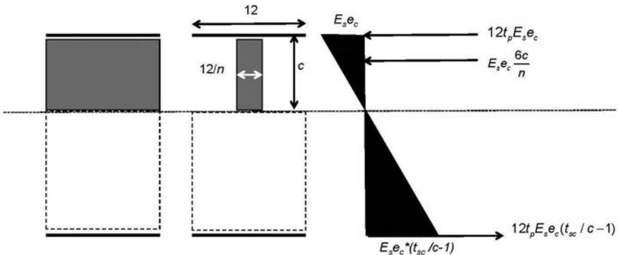
Fig. C-A-N9.2.1. Flexural stiffness of cracked-transformed section of SC walls.
