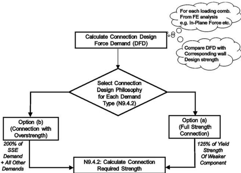
Fig. C-A-N9.4.1. Calculation of connection required strength.
