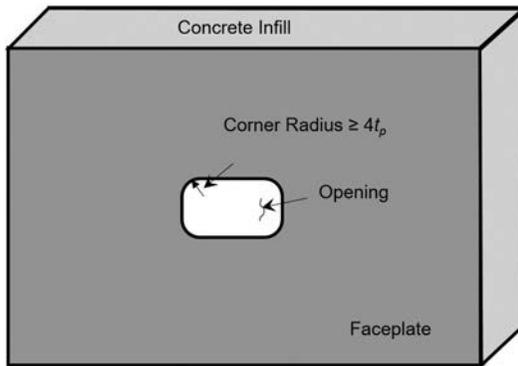
Fig. C-A-N9.1.20. Radius of reentrant corners (elevation view of the SC panel section).
