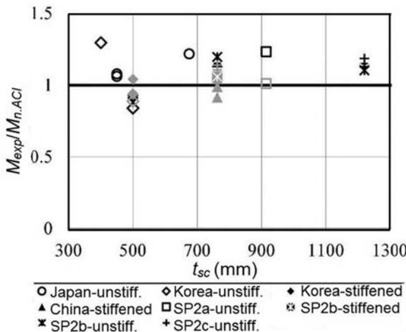
Fig. C-A-N9.3.2. Comparison of experimental flexural strength data with strength using modified Equation C-A-N9-11 (Sener et al., 2015).
