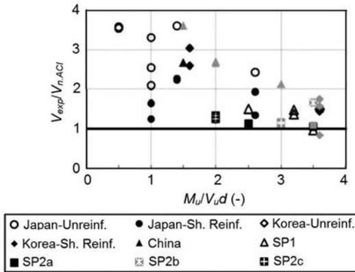
(a) Variation with shear span-to-depth ratio
