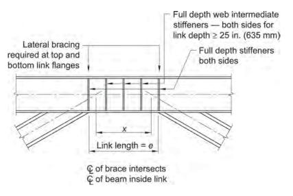
*Fig.C-F3.5. EBF* with W-shape bracing (x < e).
