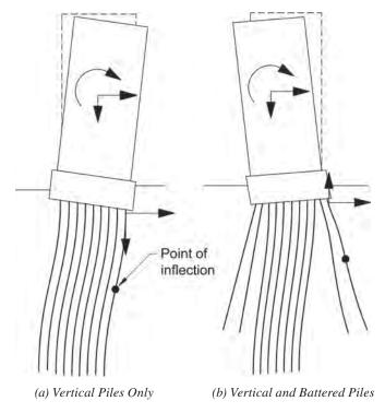
Fig. C-D4.1. Deformations of piles and forces acting on an individual pile.
