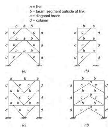
Fig. C-F3.1. Examples of eccentrically braced frames.
