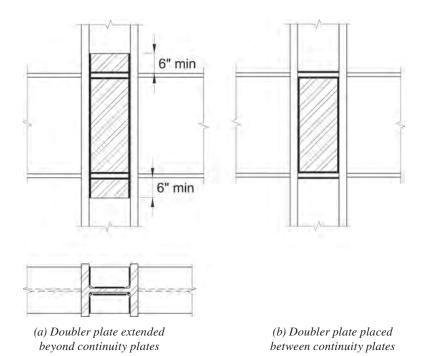
Fig. C-E3.8. Doubler plate used with continuity plates.
