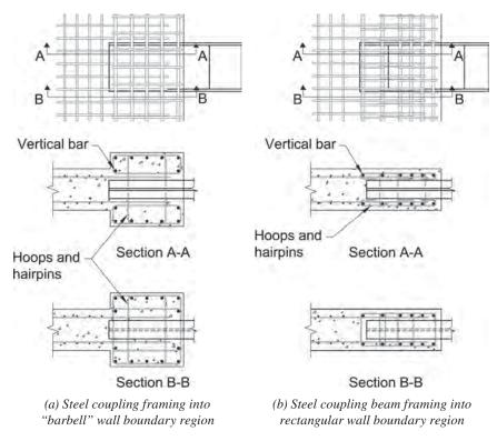
Fig. C-H5.1. Example details of a steel coupling beam embedded in reinforced concrete wall.
