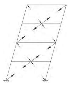
Fig. C-F2.3. Anticipated braced-frame mechanism.
