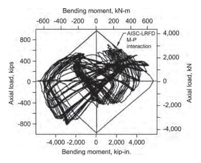
Fig. C-D4.2. Axial load-moment interaction for H-pile test.
