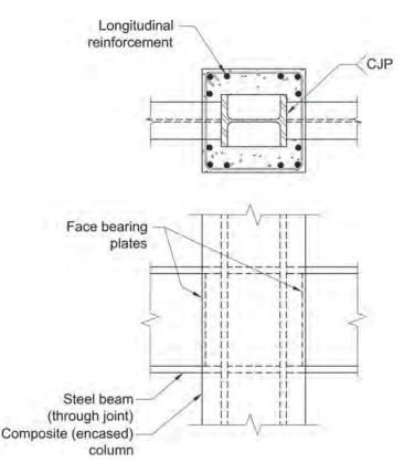
*Fig. C-G3.1. Encased composite column-to-steel beam moment connection.*
