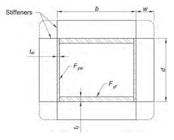
Fig. C-F3.8. Built-up box link cross section with intermediate stiffener.
