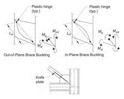
Fig. C-F2.7. Forces induced by buckling of the braces.
