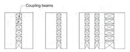
Fig. C-H4.2. Examples of coupled wall geometry.
