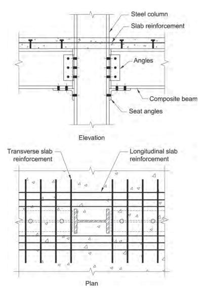
Fig. C-D2.12. Composite partially restrained connection.
