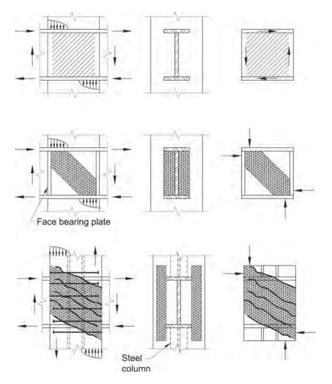
Fig. C-D2.11. Panel shear mechanisms in steel beam-to-reinforced concrete column connections (Deierlein et al., 1989).
