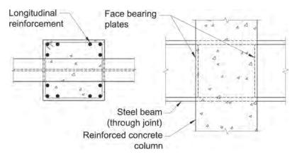
Fig. C-D2.10. Reinforced concrete column-to-steel beam moment connection.
