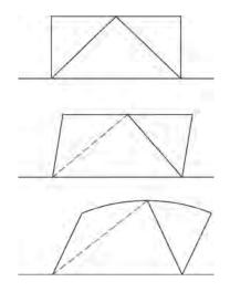
Fig. C-F4.4. Post-yield change in deformation mode for V- and inverted-V BRBF.
