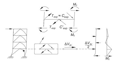
Fig. C-F2.9. Unbalanced brace story shear strengths in MT-SCBF.
