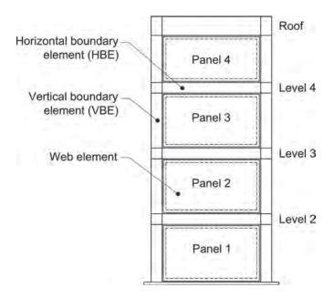
Fig. C-F5.1. Schematic of special plate shear wall.
