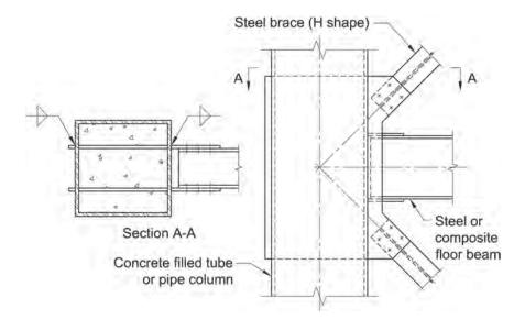
Fig. C-H1.3. Filled HSS or pipe column-to-steel concentric base.
