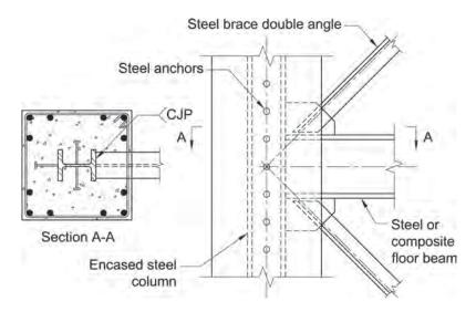
Fig. C-H1.1. Reinforced concrete (or composite) column-to-steel concentric brace.
