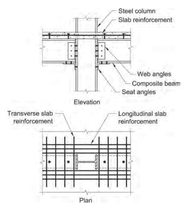
Fig. C-G4.1. Composite partially restrained connection.
