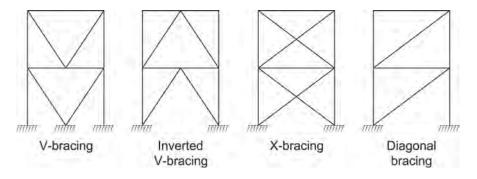
Fig. C-F2.1. Examples of concentric bracing configurations.
