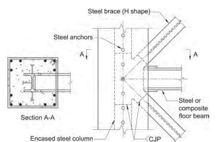
Fig. C-H1.2. Reinforced concrete (or composite) column-to-steel concentric brace.
