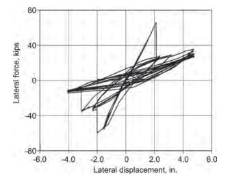
Fig. C-E4.1. Strength degradation in undetailed truss girder.
