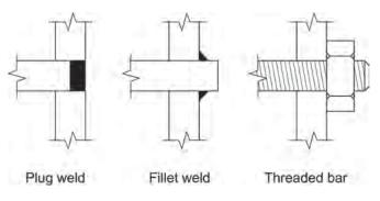
Fig. C-H7.5. Examples of tie-to-plate connection detail.
