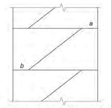
$<sup>\</sup>phi V_n$  of link a (active link) <  $\phi V_n$  of link b (inactive link)
