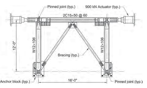
Fig. C-K3.1. Example of test subassemblage.
