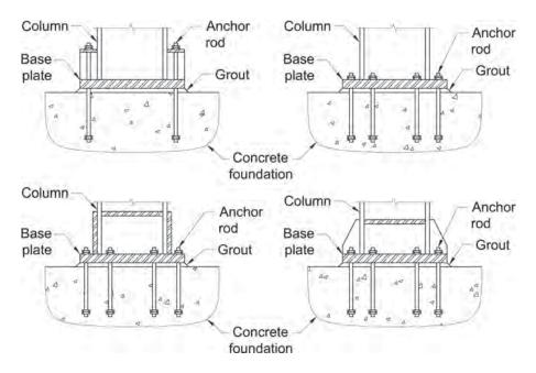
Fig. C-D2.7. Example of "rigid base" plate assembly for moment frames.
