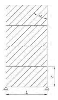
Fig. C-F5.5. Strip model of an SPSW.
