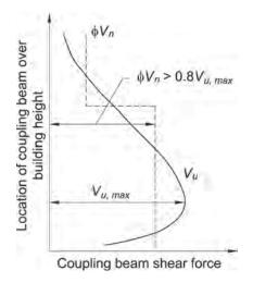
Fig. C-H4.4. Vertical distribution of coupling beam shear.
