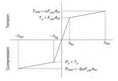
Fig. C-F4.3. Diagram of brace force-displacement.
