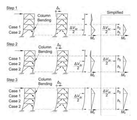
Fig. C-F2.11. Column in-plane flexural demand for a uniform MT-SCBF.
