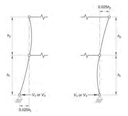
Fig. C-D2.4. Model to determine column drifts.
