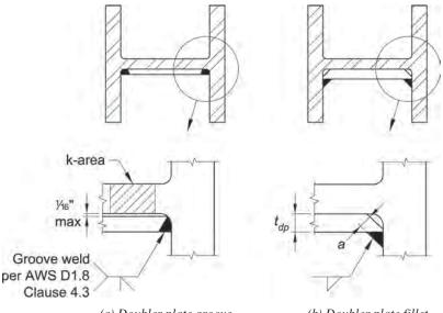
(a) Doubler plate groove welded to column flanges
