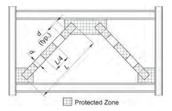
Fig. C-F2.14. Protected zone of inverted V-braced frame.
