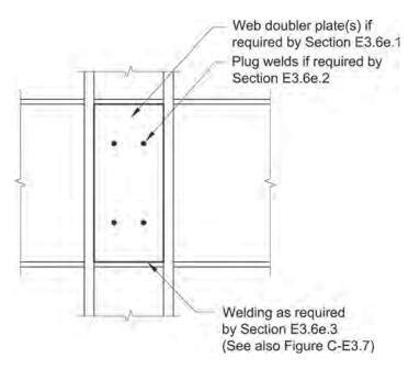
Fig. C-E3.4. Connecting web doubler plates with plug welds.
