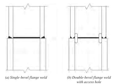
Fig. C-E3.10. Splice details with partial-penetration-groove welds.
