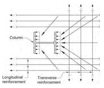
Fig. C-G4.2. Concrete slab bearing force transfer.
