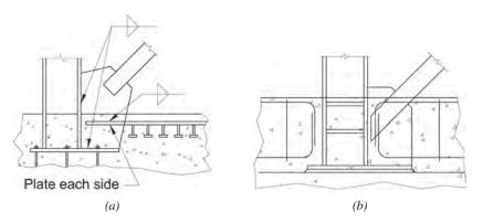
Fig. C-D2.6. Examples of shear transfer to a concrete grade beam.
