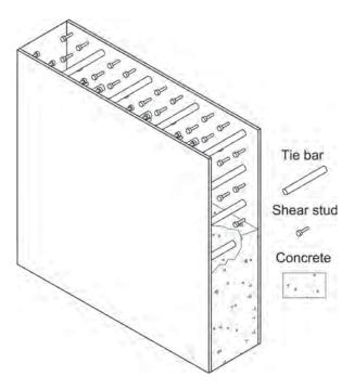
Fig. C-H7.3. C-PSW/CF without boundary elements.
