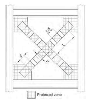
Fig. C-F2.15. Protected zone of X-braced frame.
