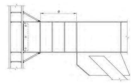
Fig. C-F3.10. Example of a reinforced link-to-column connection.
