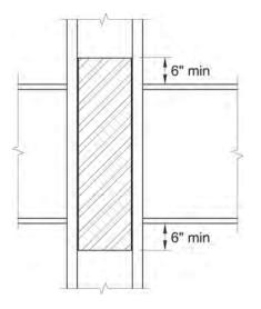
Fig. C-E3.7. Doubler plates used without continuity plates.
