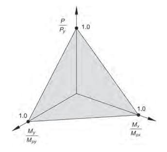
Fig. C-E3.1. Linear yield surface for bi-axial bending.
