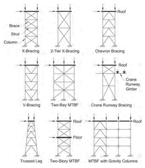
Fig. C-F2.5. Typical MTBF configurations.
