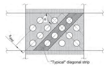
Fig. C-F5.7. Schematic detail of special perforated steel plate wall and typical diagonal strip.
