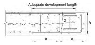
Fig. C-H5.2. Reinforcement to prevent splitting failures.
