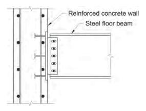
Fig. C-D2.9. Steel beam-to-reinforced concrete wall gravity load shear connection.
