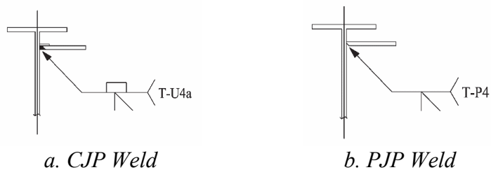
Fig. 4. Alternative welds for joints with clearance on one side only.
