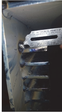
Fig. 15. Measurement of weld leg size.
