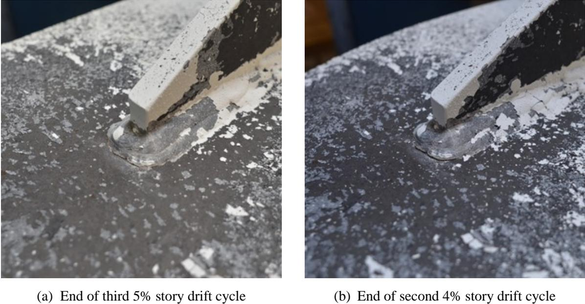
**Figure 3.15.** Top flange fracture initiation and propagation 8ES-1.375-1.5-36wrap
