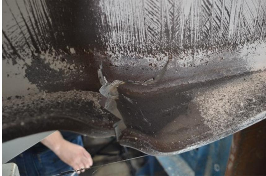
**Figure 3.9.** Partial fracture of the beam web 4ES-1.375-1.25-24Wrap
