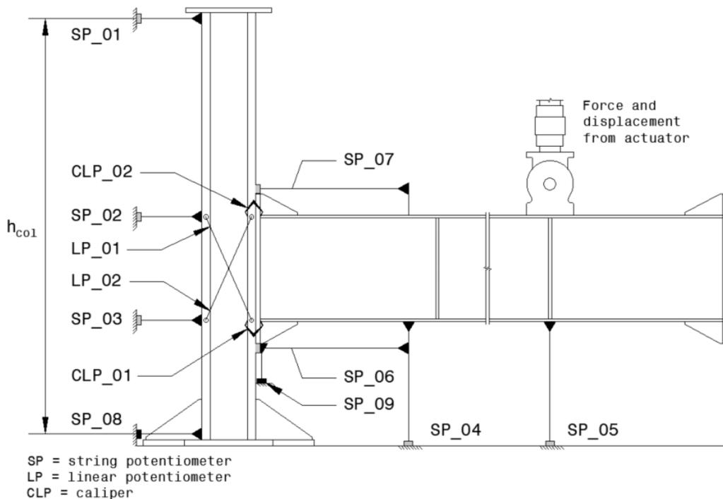
**Figure 2.7.** Instrumentation plan for all tests
