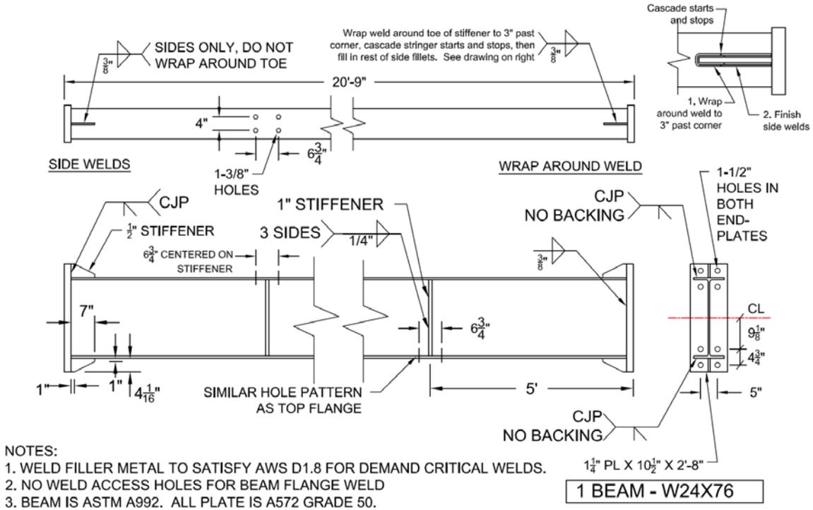
**Figure 2.3.** Details of the W24×76 specimens (Each end represents one specimen)
