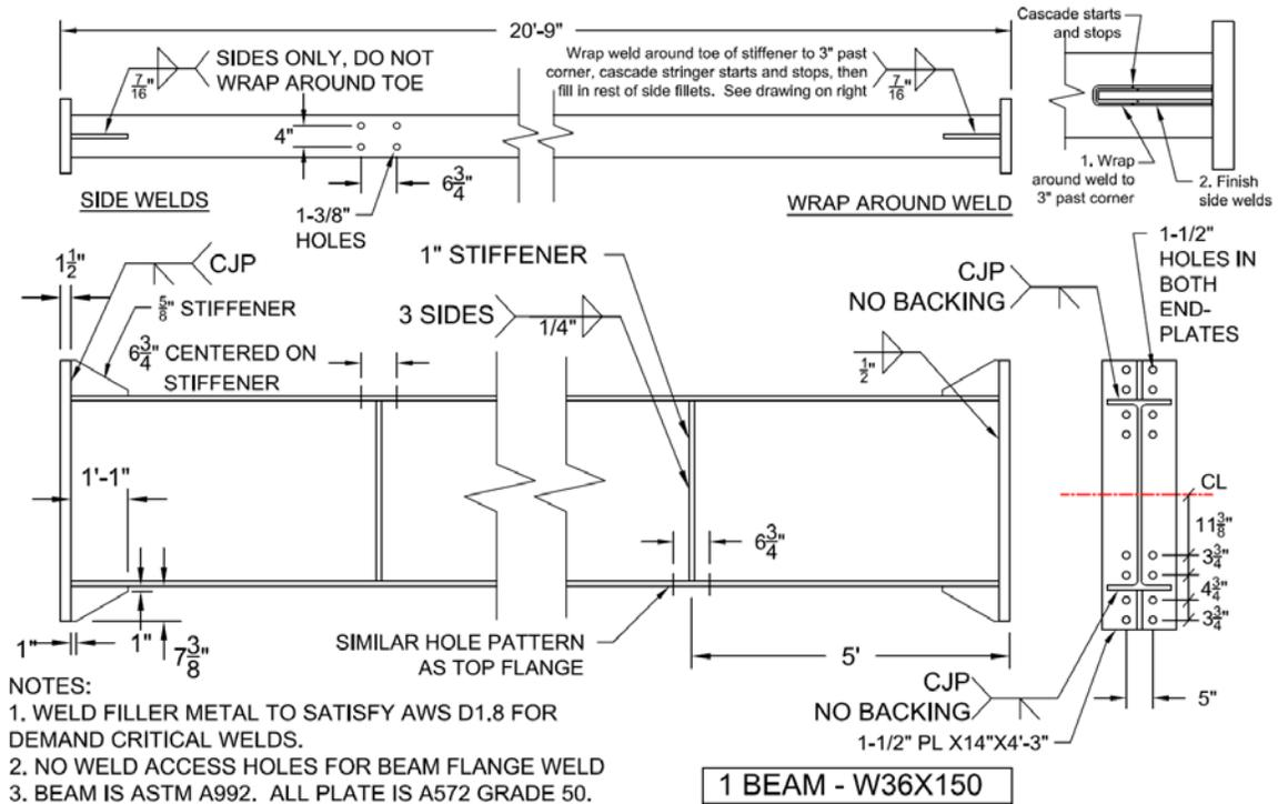
**Figure 2.4.** Details of the W36×150 specimens (Each end represents one specimen)
