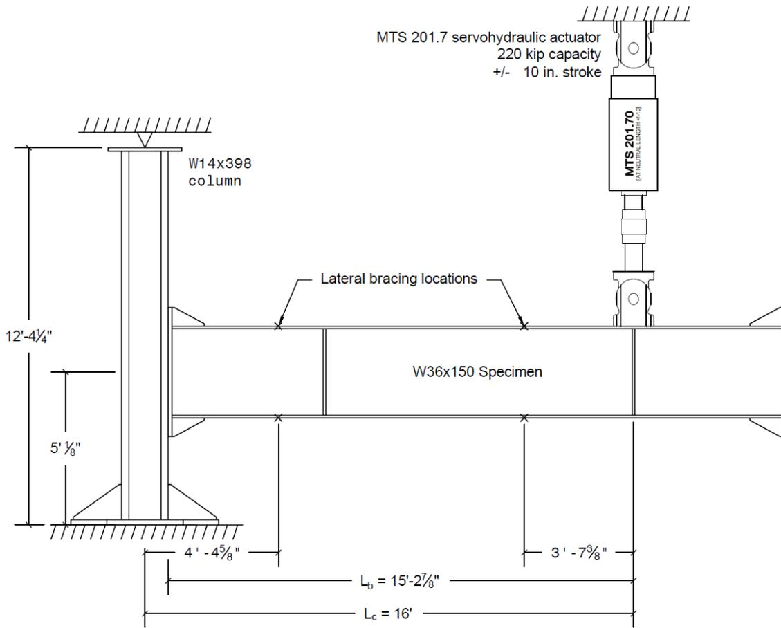
**Figure 2.5.** Schematic drawing of beam-to-column moment connection test setup
