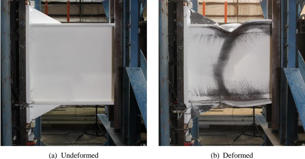
**Figure 3.14.** Undeformed and deformed conditions of 8ES-1.375-1.5-36wrap
