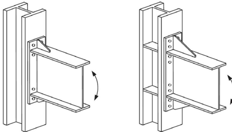
(a) Four-bolt extended stiffened (4ES) (b) Eight-bolt extended stiffened (8ES)
