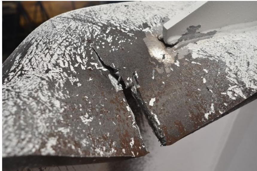
**Figure 3.5.** Top flange fracture of 4ES-1.375-1.25-24sides
