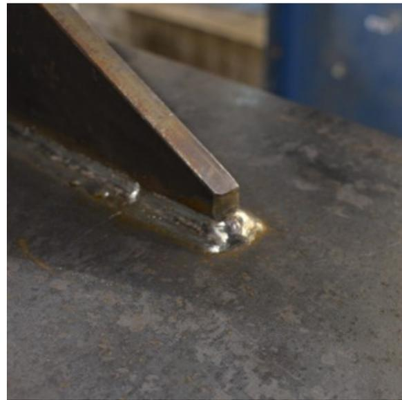
(b) Weld wrapped around stiffener toe
