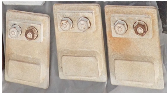
Figure 4-3. Galvanized Plates with Bolted and Welded Features After 80 Cycles of Accelerated Corrosion Testing
