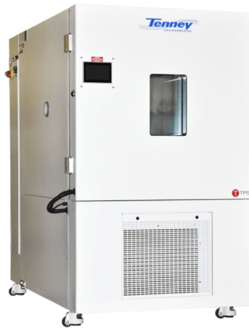
Figure 3-15. Tenney Environmental Chamber
