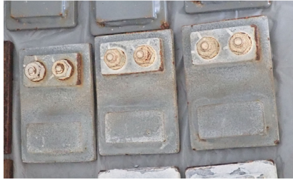
Figure 4-11. 1-Coat IOZ Plates with Bolted and Welded Features After 80 Cycles of Accelerated Corrosion Testing
