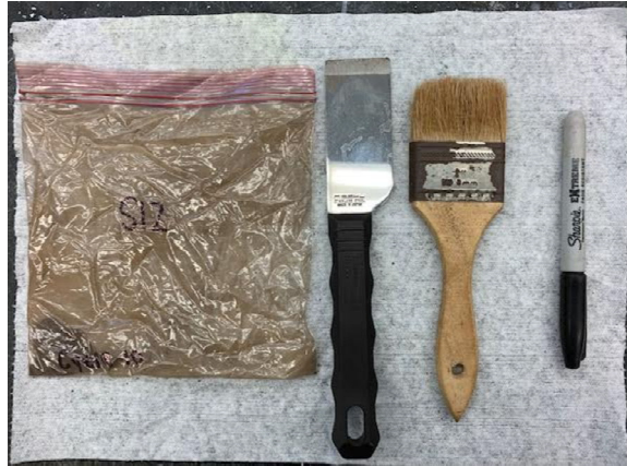
Figure 3-25. Ziplock Bag, Putty Knife, Paintbrush, and Marker Used for Collecting and Labeling Corrosion Products Scraped from Specimens
