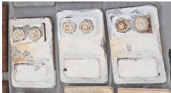
Figure 4-7. Metallized Plates with Bolted and Welded Features After 80 Cycles of Accelerated Corrosion Testing
