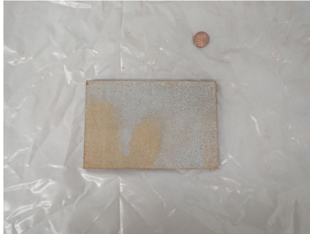
Figure 4-9. 1-Coat IOZ Specimen Discoloration After 80 Cycles of Accelerated Corrosion Testing
