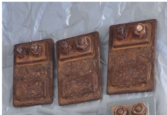
Figure 4-16. UWS Plates with Bolted and Welded Features After 80 Cycles of Accelerated Corrosion Testing
