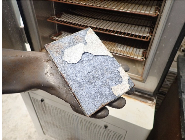
Figure 4-6. Metallized Coating Deterioration on 4” x 6” Face of Specimen After 55 Cycles of Accelerated Corrosion Testing
