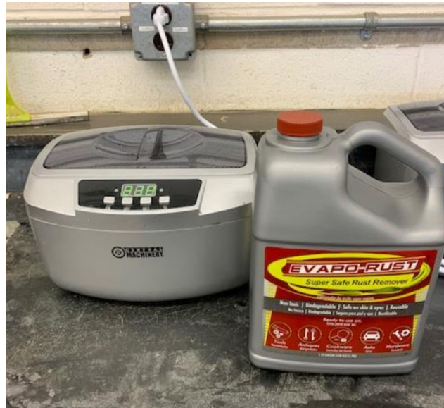
Figure 3-28. Ultrasonic Cleaner and Evapo-Rust Solution
