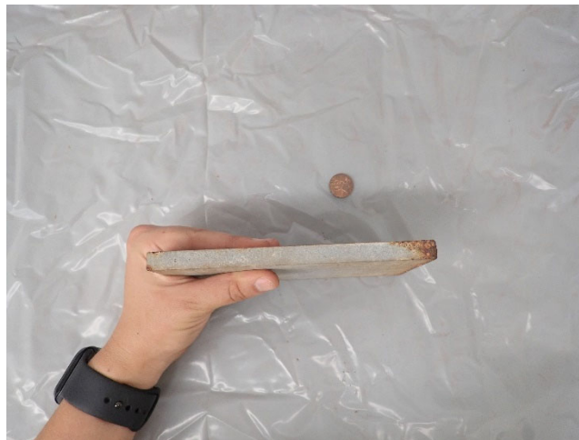
Figure 4-10. 1-Coat IOZ Specimen with Corrosion at the Corner After 80 Cycles of Accelerated Corrosion Testing
