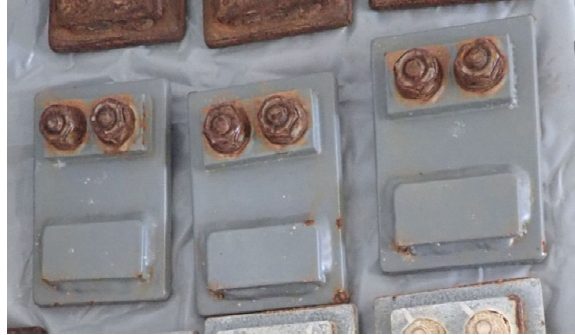
Figure 4-14. 3-Coat OZ Plates with Bolted and Welded Features After 80 Cycles of Accelerated Corrosion Testing
