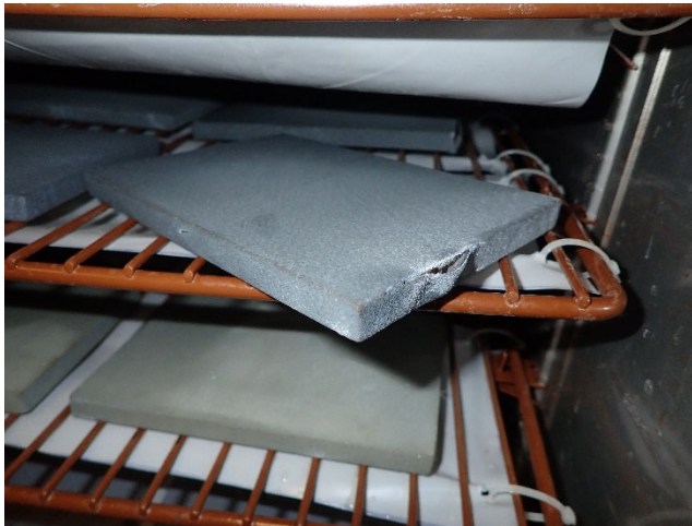
Figure 4-5. Metallized Coating Pulling Away on the Edge After 7 Cycles of Accelerated Corrosion Testing
