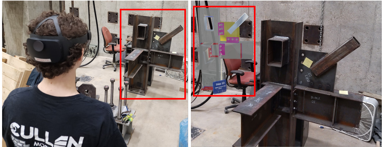
Figure 8.2: User 1 viewing the final beam-column connection (shown in in red rectangle) through the headset and a corresponding view in the program (hologram shown in red rectangle)
