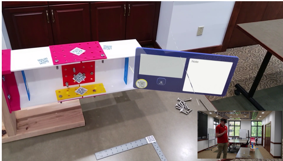
Figure 9.1: User interacting with the note dialogue box by adding a note via speech-to-text to a user-specified location on a completed steel bridge connection assembly
