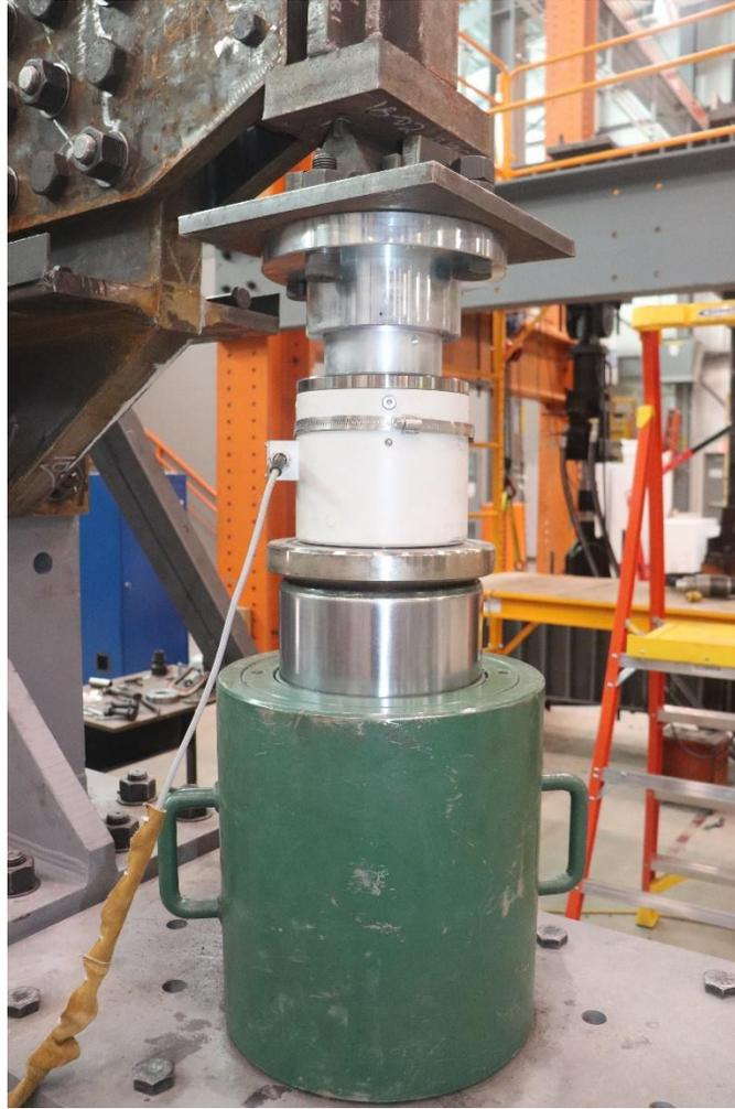
Figure 5.5: Load column: actuator, load cell, and load application wedge
