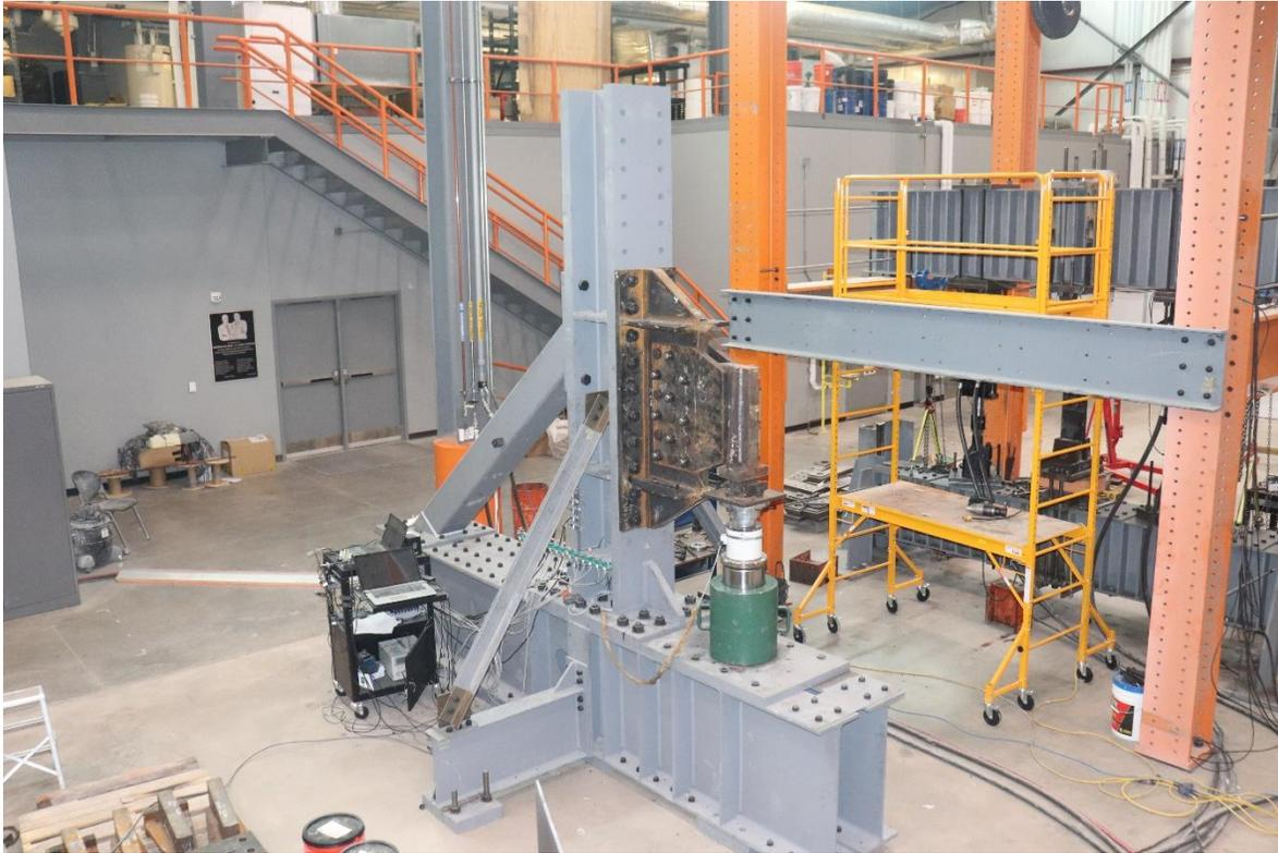
Figure 5.4: Eccentric Frame with 1×6 Test Specimen
