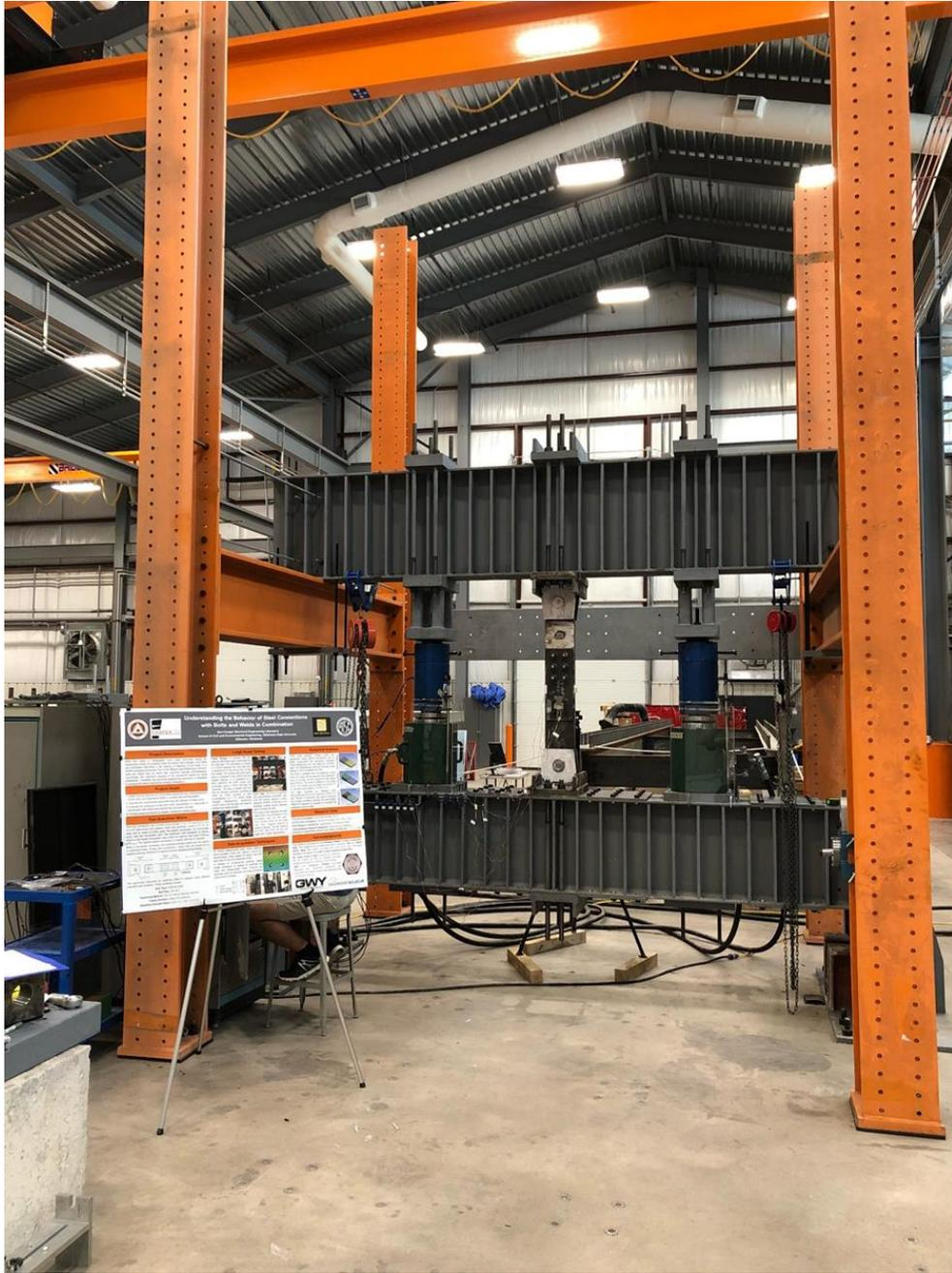
Figure 2.5: Constructed 500-kip test frame
