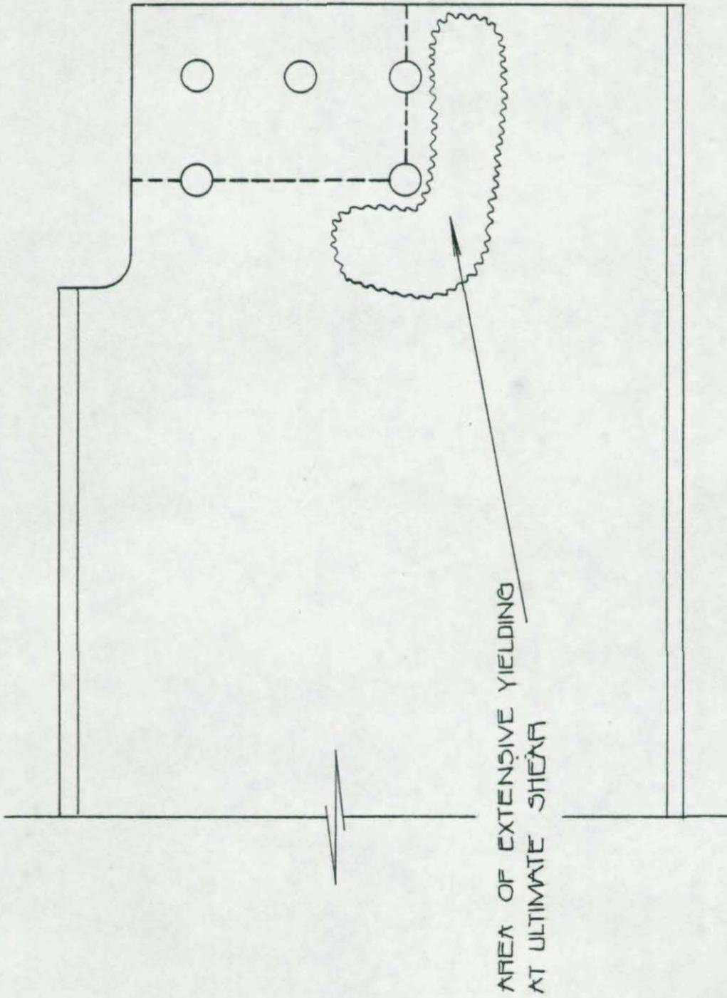
FIGURE 2 BEAM WITH COPEd TOP FLANGE AT CONNECTION
