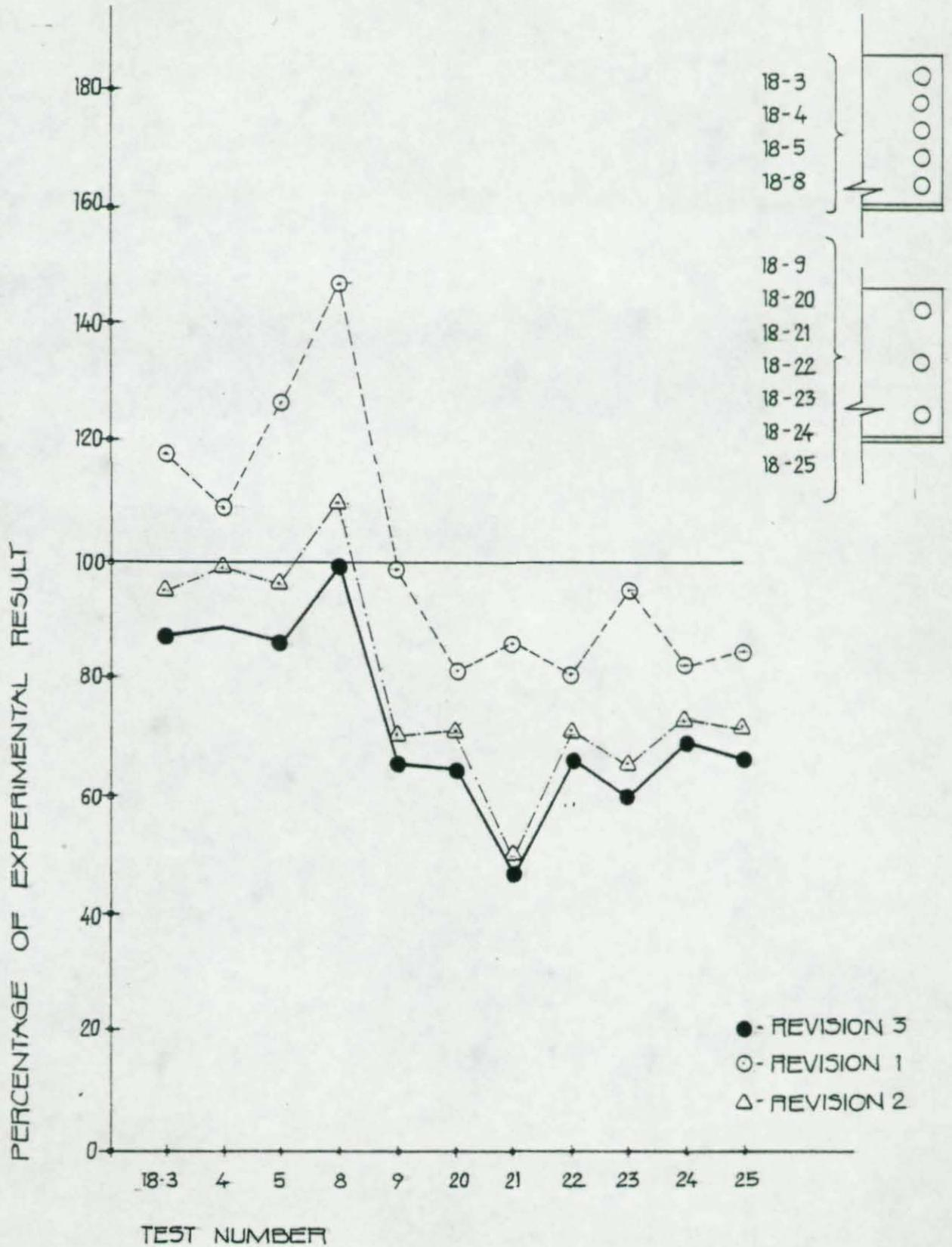
FIGURE 20 COMPARISON OF REVISIONS FOR CISC COMPUTER PROGRAM, TWO LINES OF BOLTS CONNECTIONS
