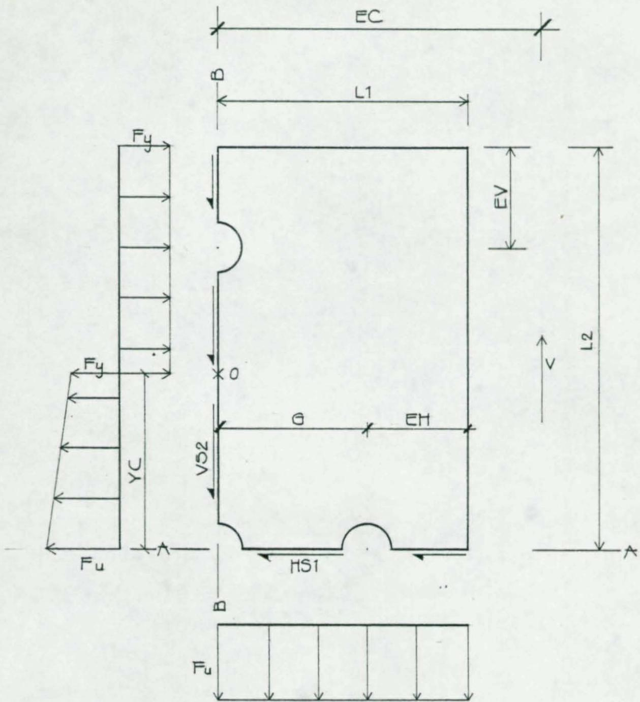
FIGURE 9 MOMENT MODEL, COPED FLANGE
