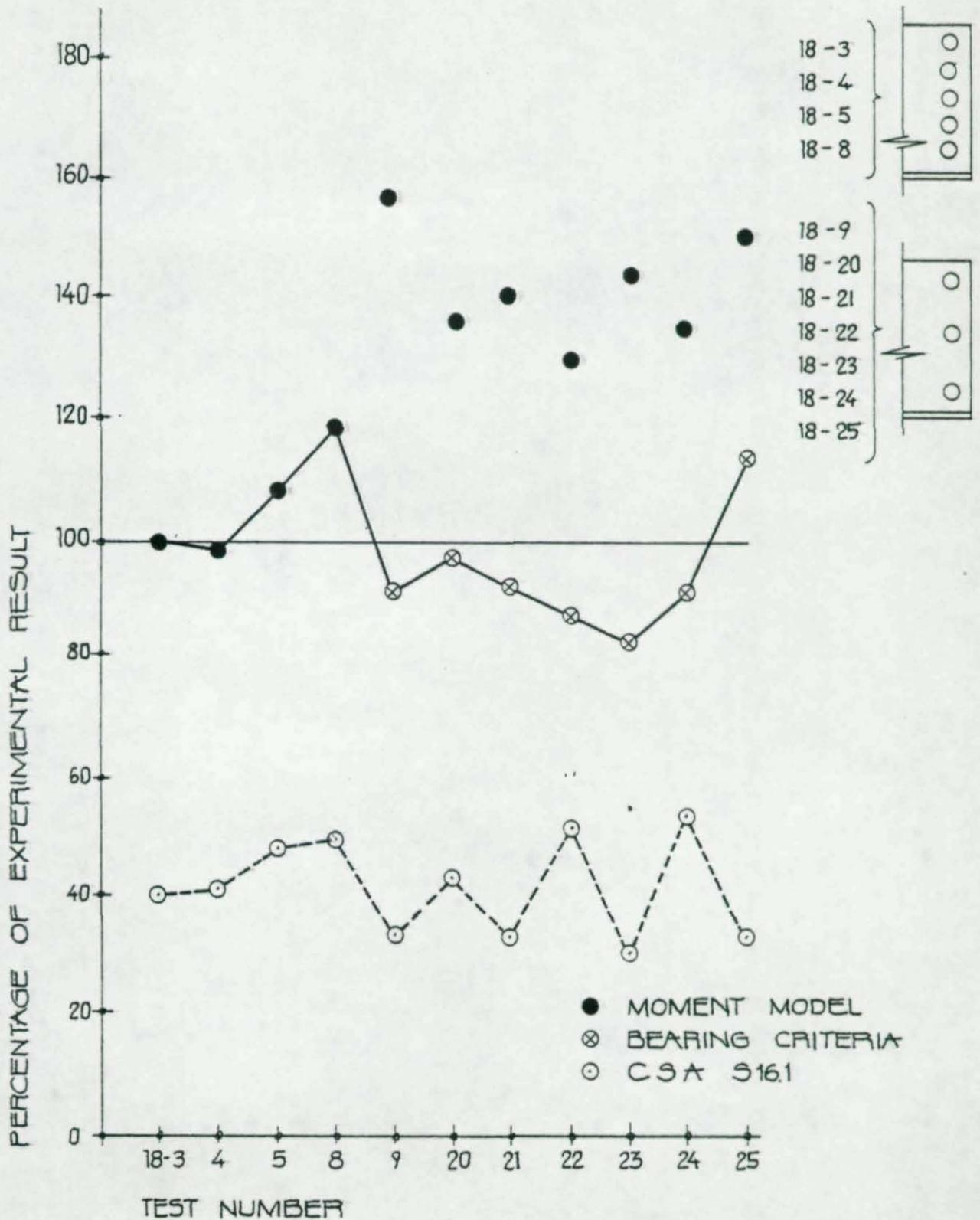
FIGURE 18 COMPARISON OF CSA SPECIFICATION TO "MOMENT" MODEL FOR COPEDED BEAMS WITH TWO LINES OF BOLTS CONNECTIONS,
