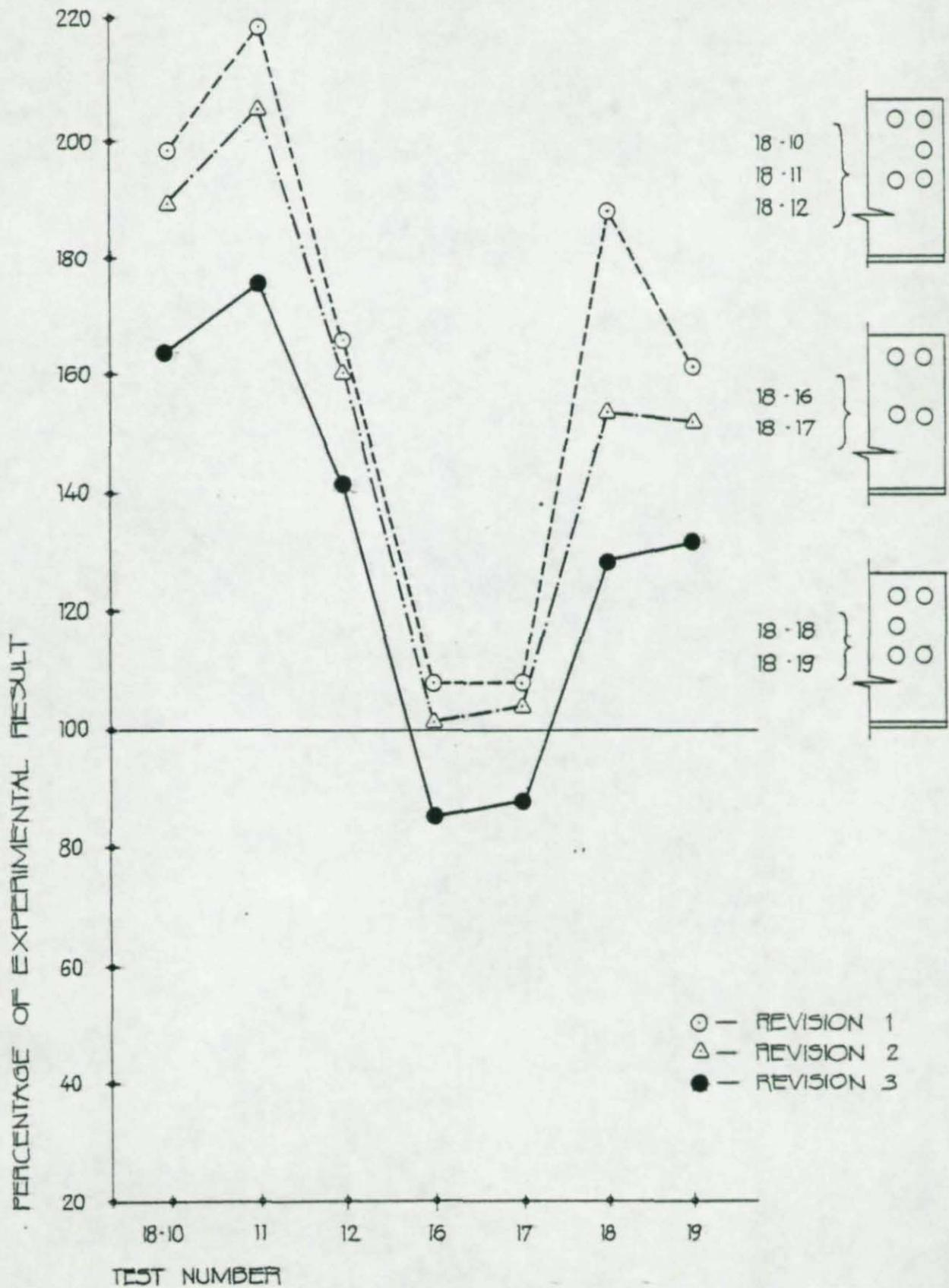
FIGURE 21 COMPARISON OF RESULTS OBTAINED BY REDUCING ECCENTRICITY AND REMOVING END TEAR-OUT LIMIT.
