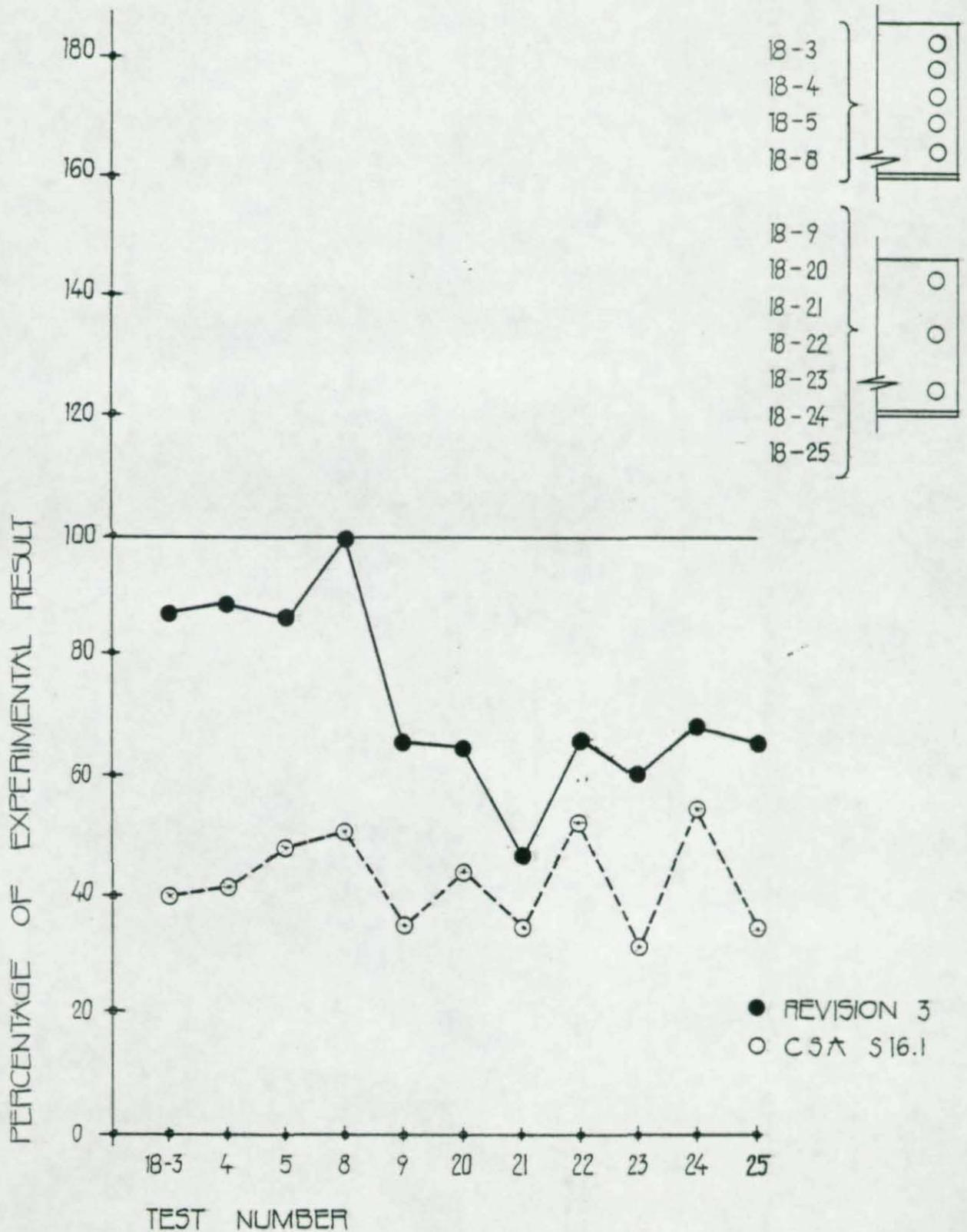
FIGURE 23 : COMPARISON OF REVISION 3 TO CURRENT CSA SPECIFICATION ; DOUBLE LINE OF BOLTS CONNECTIONS
