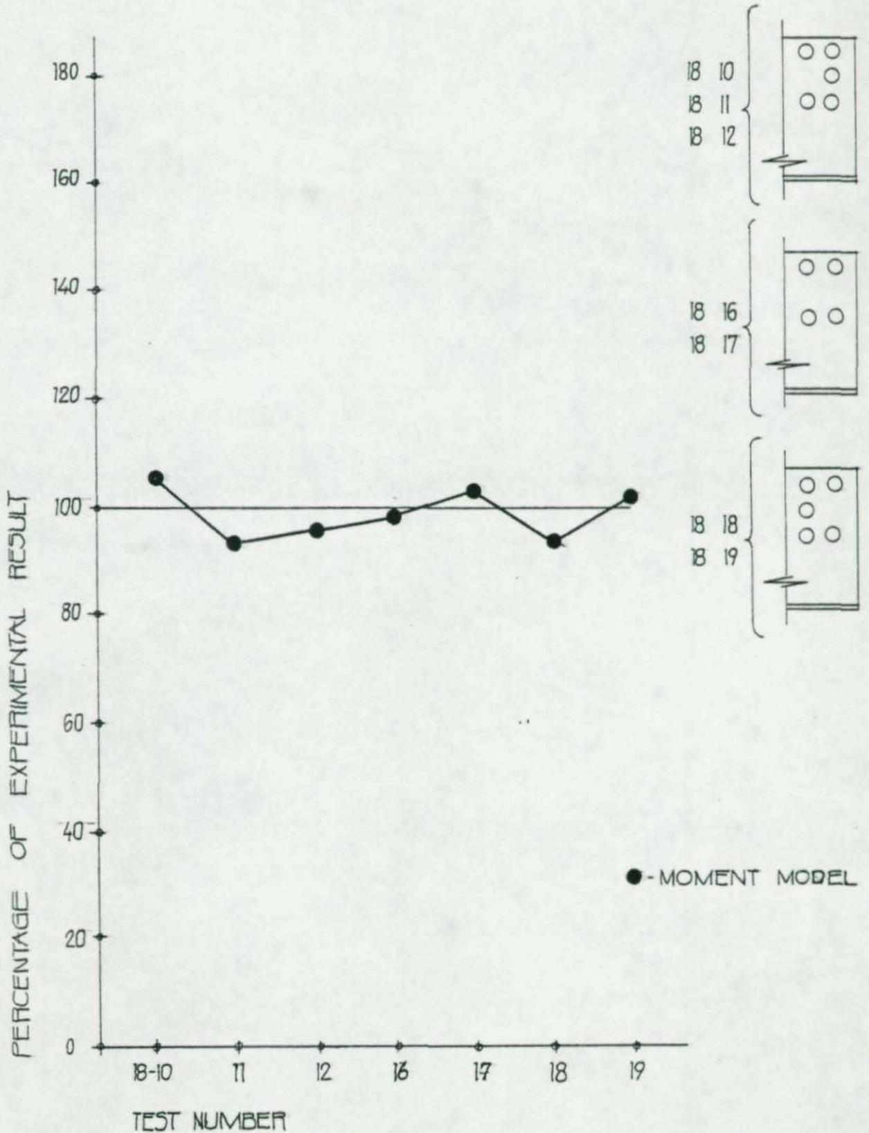
FIGURE 14 PERCENTAGE OF EXPERIMENTAL RESULT VERSUS TESTS OF UNCOPED BEAMS, UNIV. OF TEXAS - AIS C PROJECT,
