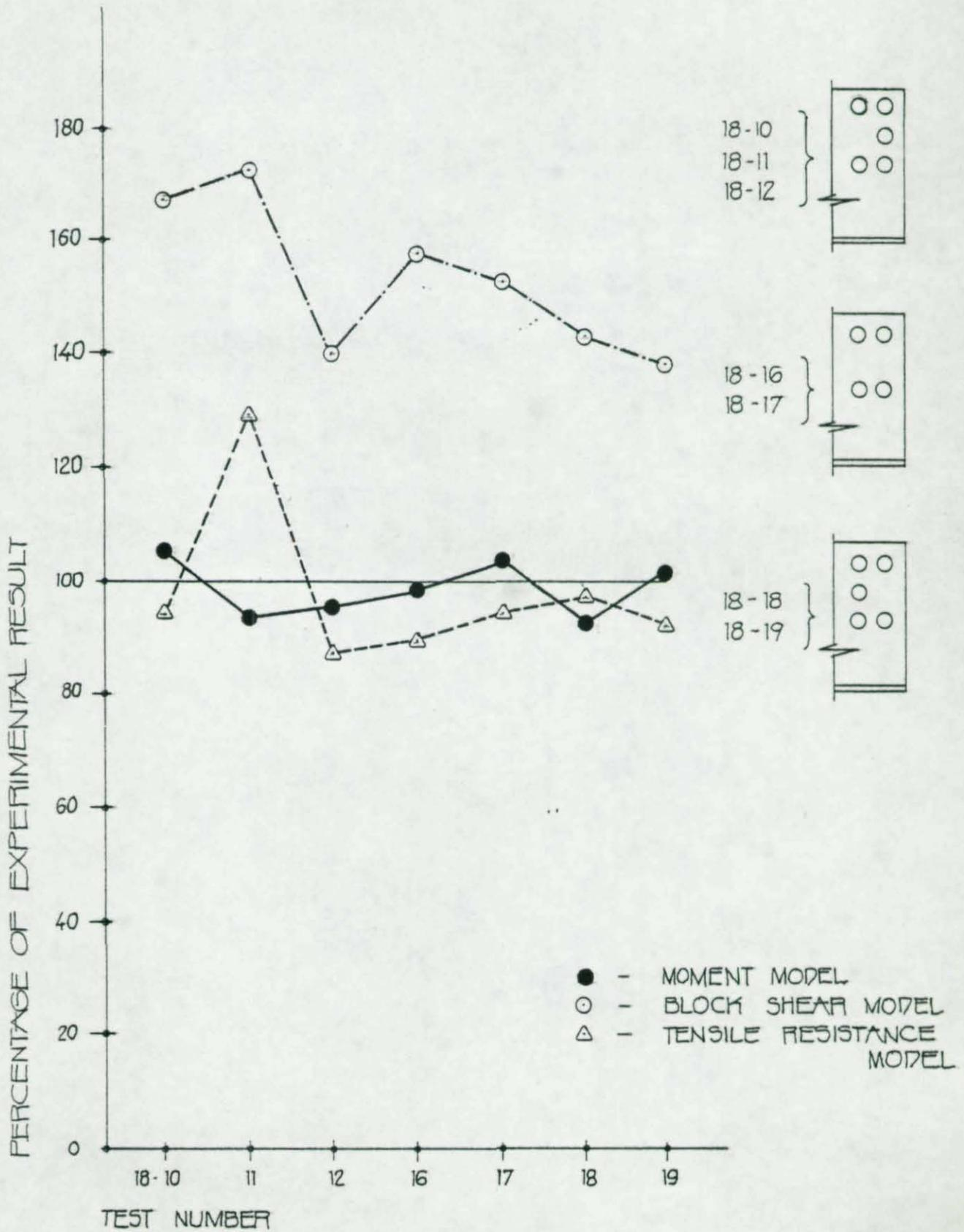
FIGURE 17 COMPARISON OF CSA SPECIFICATION TO "MOMENT" MODEL FOR COPED BEAMS WITH SINGLE LINE OF BOLTS CONNECTIONS
