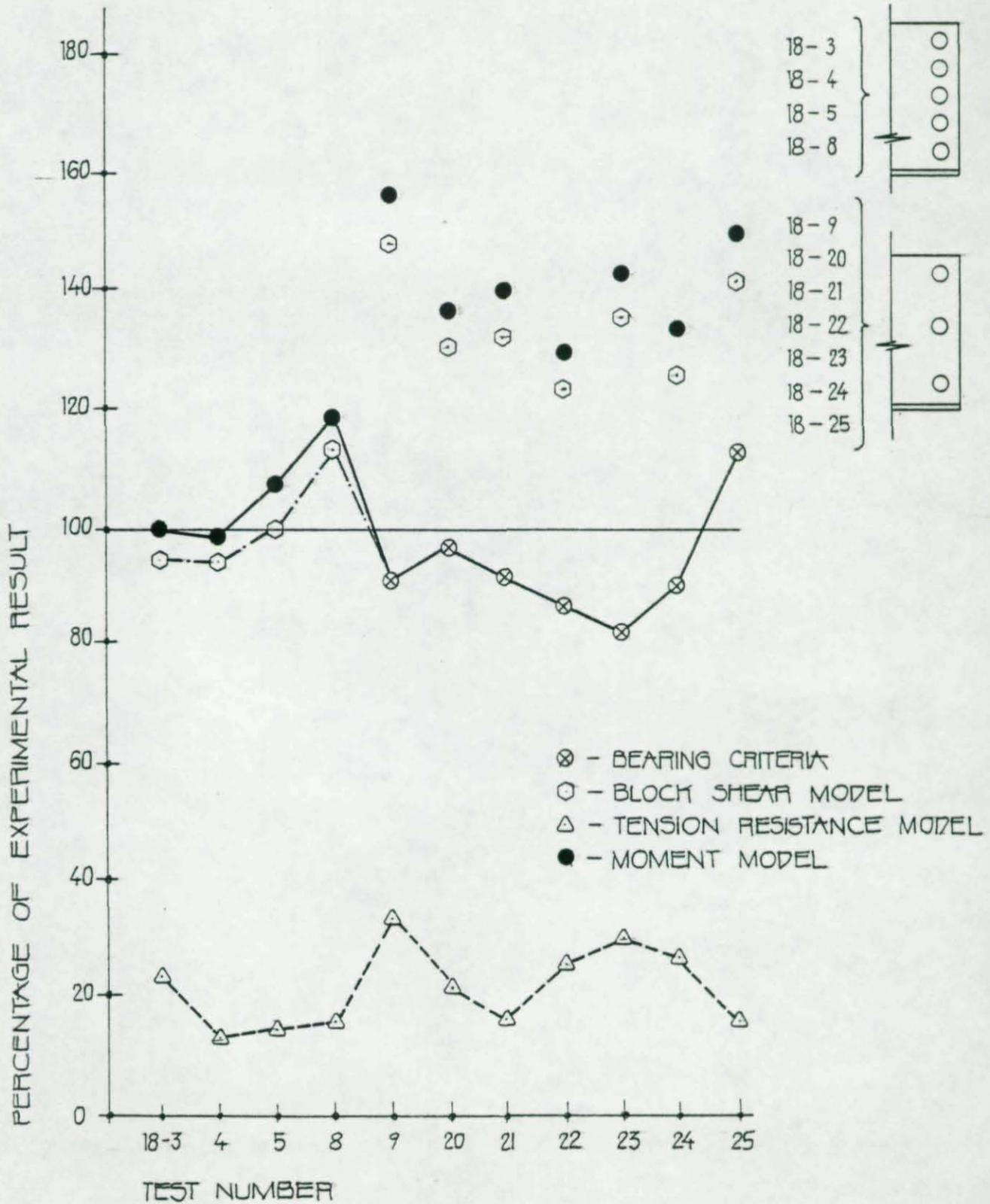
FIGURE 16 COMPARISON OF MODELS FOR COPEL BEAMS WITH TWO LINES OF BOLTS CONNECTIONS.
