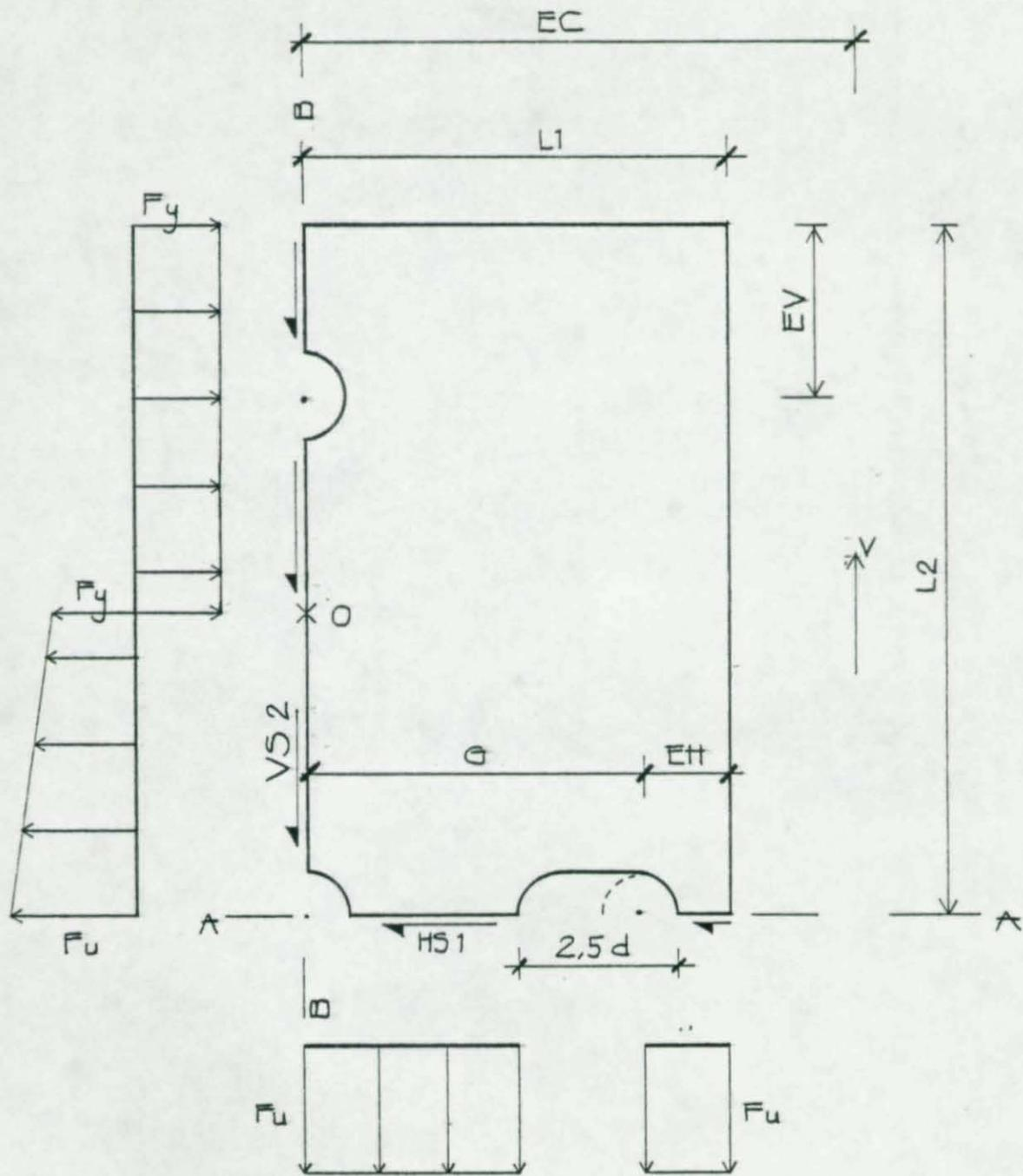
FIGURE 10 MOMENT MODEL , COPED FLANGE , SLOTTED HOLES
