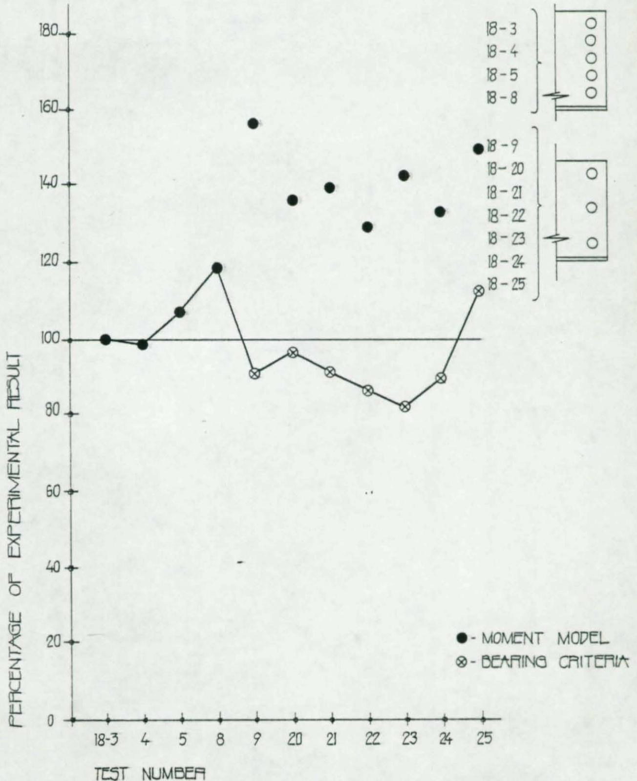
FIGURE 13 PERCENTAGE OF EXPERIMENTAL RESULT VERSUS TESTS OF COPEL BEAMS WITH TWO LINES OF BOLTS CONNECTIONS, UNIV. OF TEXAS, AISC PROJECT
