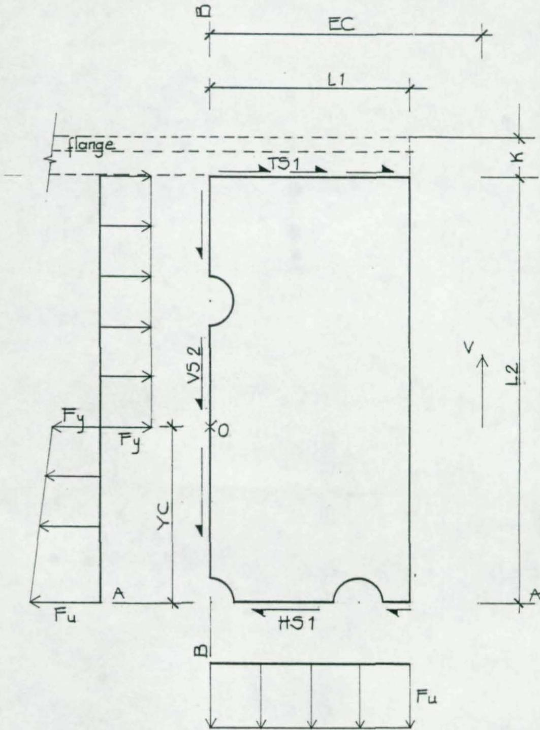
FIGURE 11 - MOMENT MODEL - UNCOPED FLANGE
