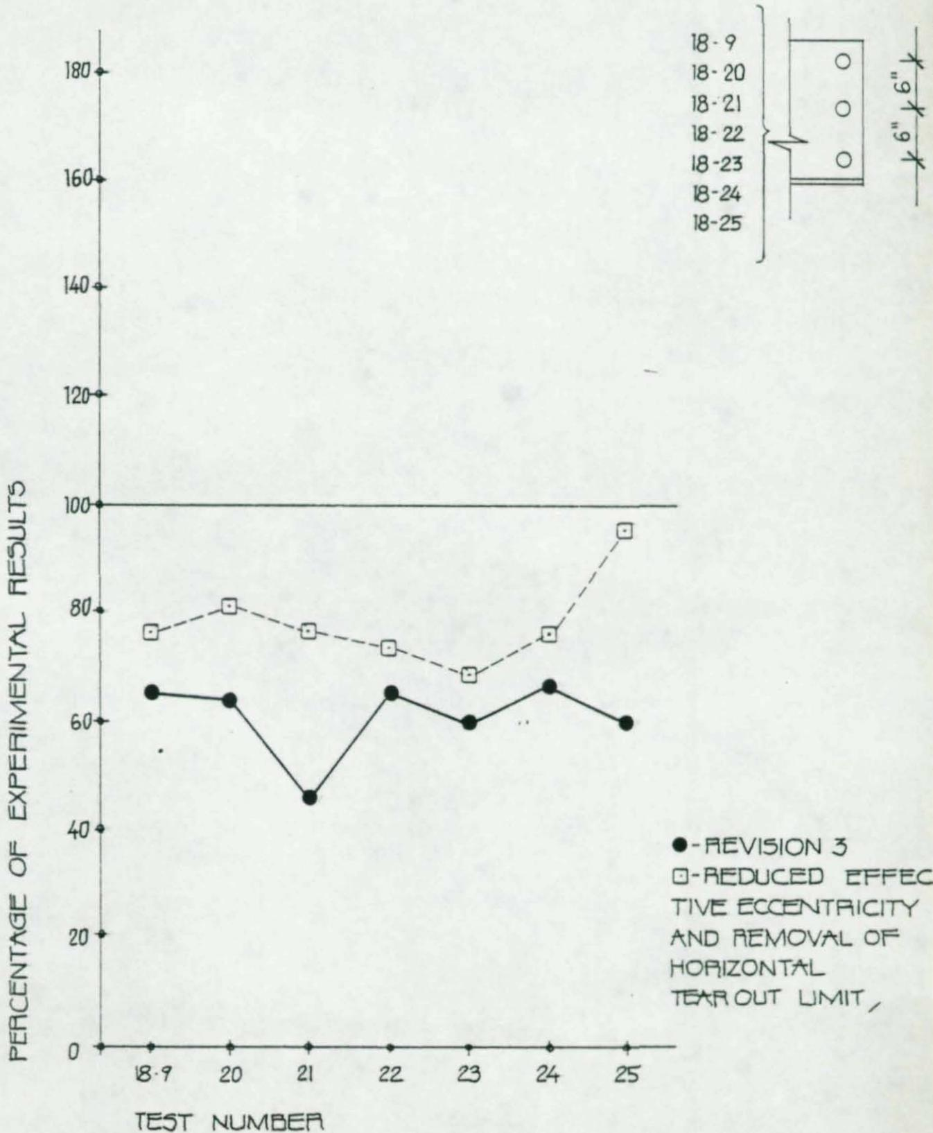
FIGURE 22 COMPARISON OF REVISION 3 TO CURRENT CSA SPECIFICATION ; SINGLE LINE OF BOLTS CONNECTIONS,
