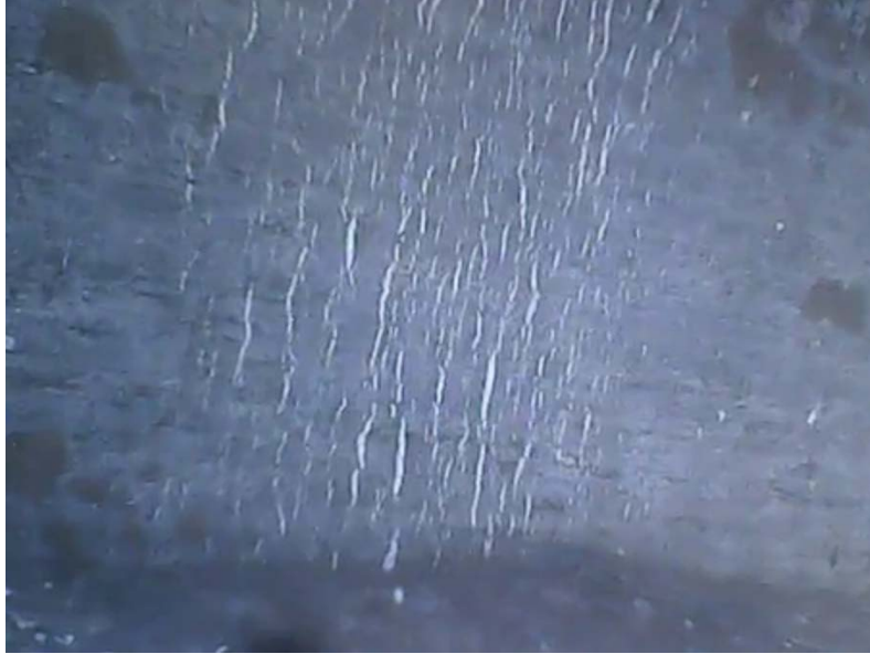
Figure A.8 – Fracture initiation on bottom side of specimen during cycle 2 when bottom side was in tension.
