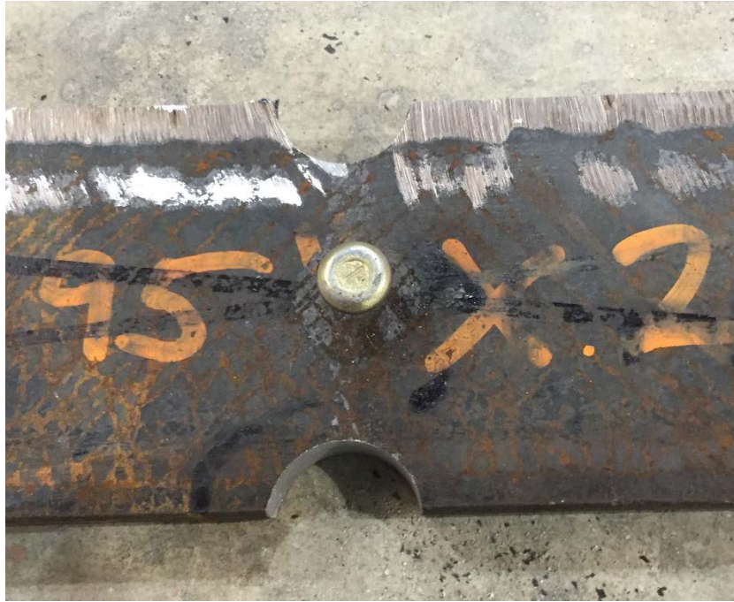
Figure 2.6 – Completed fastener specimen.
