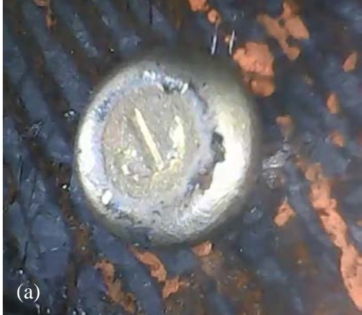
Figure A.9 – (a) Fracture initiation on Specimen W24-PnAF075-T59-R000 at the top of the fastener head during cycle 4 on the top side of the specimen when the top side was in tension and (b) full fracture through the bottom side of the specimen in cycle 9 when the bottom side was in tension.
