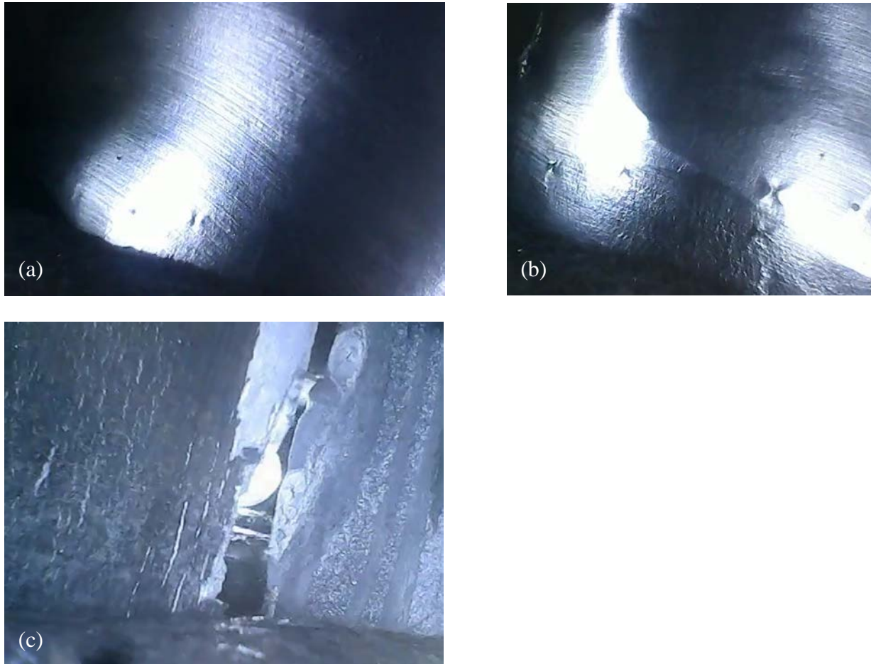
Figure A.21 – (a) First visible defects can be seen on weld surface on specimen W36-BSW-T94-R000 during cycle 1, (b) a very clear folded steel defect can be seen in the bottom right of the picture during cycle 2, and (c) full fracture through the bottom side of the specimen in cycle 4 when the bottom side was in tension
