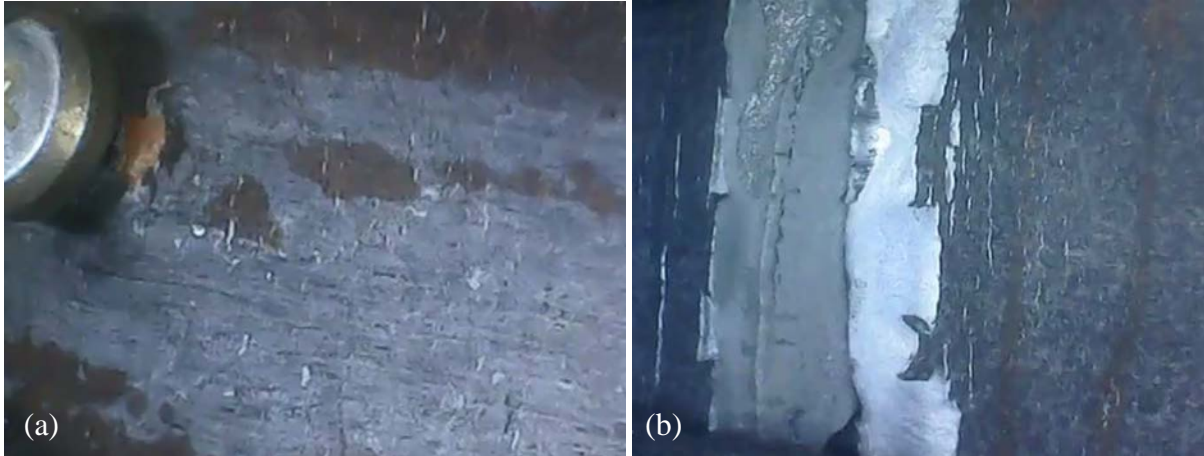
Figure A.2 – (a) Minor fracture initiation on Specimen W36-PnAF062.5-T94-R000 on the top of the specimen near the head of the fastener and (b) complete fracture occurred at cycle 5 through the bottom side of the specimen.
