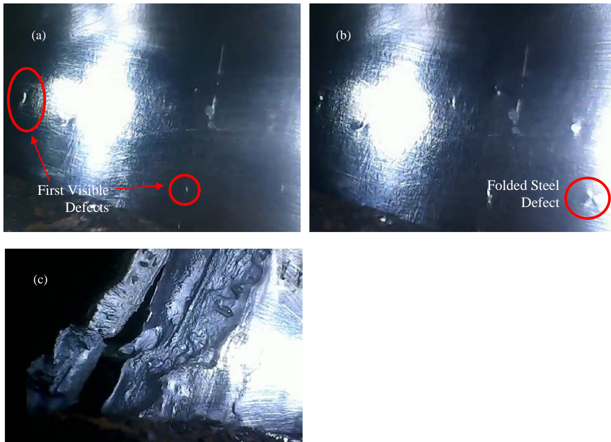
Figure 3.11 – a) First visible defects on specimen W24-BSW-T59-R000 during first cycle on top side of specimen in tension, b) Folded steel defect on specimen during cycle 2 on top side of specimen in tension, and c) final fracture through top side of specimen in tension during cycle 13.
