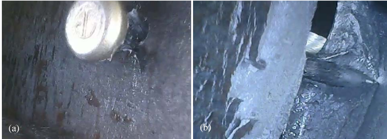
Figure A.7 – (a) Fracture initiation and propagation during cycle 2 for specimen W36-PnAF075-T94-R100 on the top side of the specimen around the fastener shaft when the top side was in tension and (b) full fracture through the bottom side of the specimen during cycle 2 when the bottom side was in tension.
