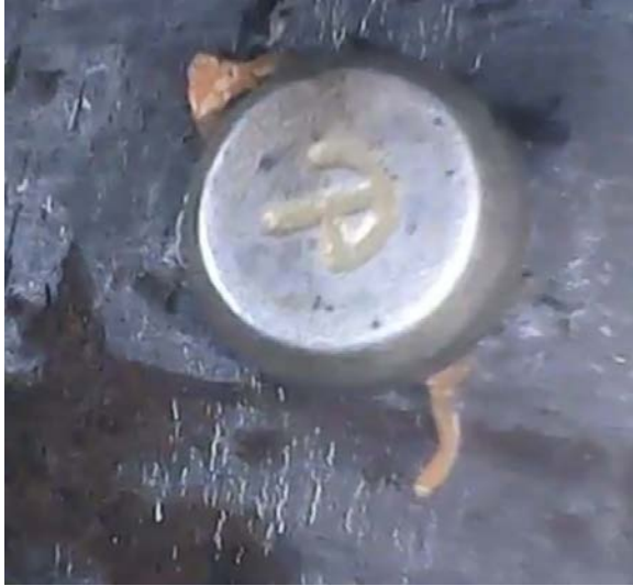
Figure A.4 – a) Multiple fracture initiation on Specimen W36-PnAF062.5-T94-R025 around the fastener head during cycle 2 when the top side of the specimen was in tension and b) full fracture through the bottom side of the specimen when the bottom side was in tension during cycle 2.
