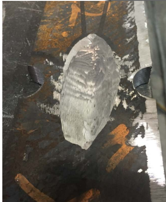
Figure 2.7 – (a) Dimensions of the boat shaped notch, and (b) finished ground notch before welding.
