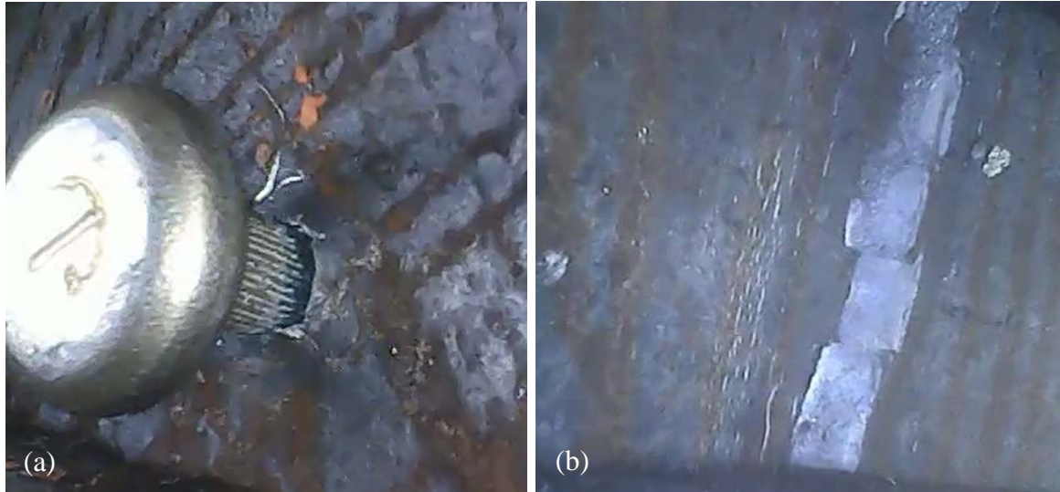
Figure A.62 – (a) Fracture initiation on the top side of the fastener shaft during cycle 2 on the top side of the specimen when the top side was in tension and (b) full fracture through the bottom side of the specimen during cycle 4 when the bottom side was in tension.
