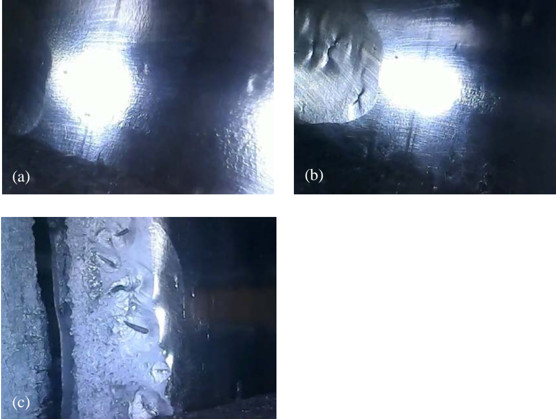
Figure A.24 – (a) Small visible defects on surface of weld on specimen W36-BSW-T94-R100 during cycle 1, (b) multiple folded steel defects forming in cycle 2 in the area where a void was ground out, and (c) final fracture through top of specimen during cycle 2 when top side was in tension.
