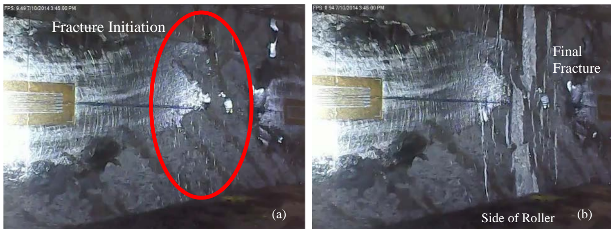
Figure 3.4– Fracture initiation at multiple locations at the bottom of Specimen W24-B2-T59-R025 on cycle 3, complete fracture at the bottom side of the specimen at cycle 5.
