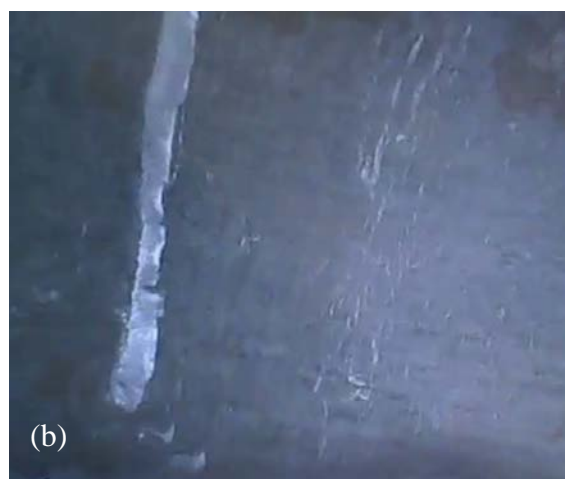
Figure A.5 – (a) Fracture initiation and propagation directly under the fastener head in specimen W36-PnAF062.5-T94-R100 during cycle 2 on the top side of the specimen while the top side was in tension and (b) complete fracture through the bottom of the plate during cycle 3 when the bottom was in tension.
