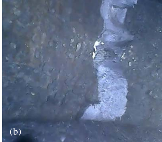
Figure A.9 – (a) Fracture initiation on Specimen W24-PnAF075-T59-R000 at the top of the fastener head during cycle 4 on the top side of the specimen when the top side was in tension and (b) full fracture through the bottom side of the specimen in cycle 9 when the bottom side was in tension.
