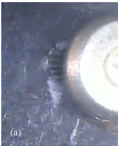
Figure A.5 – (a) Fracture initiation and propagation directly under the fastener head in specimen W36-PnAF062.5-T94-R100 during cycle 2 on the top side of the specimen while the top side was in tension and (b) complete fracture through the bottom of the plate during cycle 3 when the bottom was in tension.
