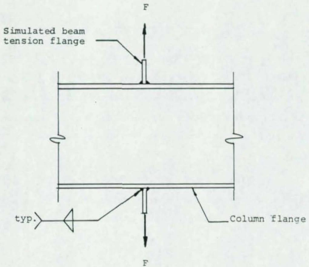
Figure 24. Test Set-up Used in Reference 2
