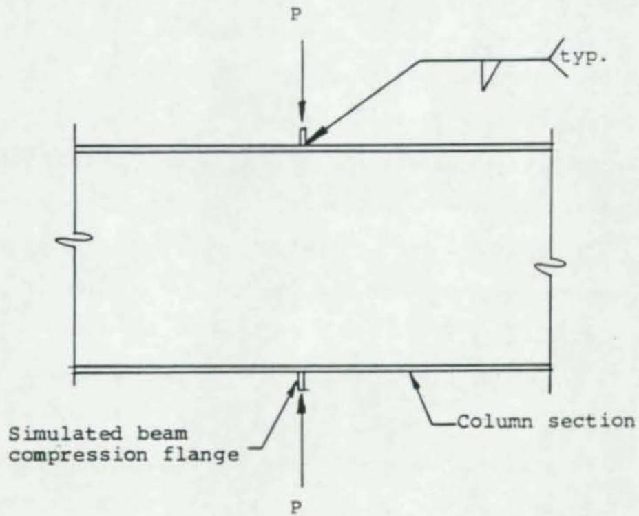
Figure 5. Test Set-up Used in Reference 2
