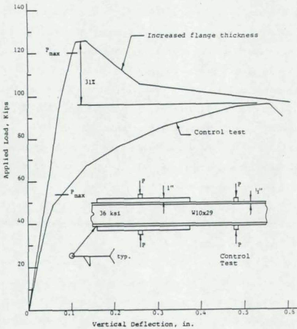
Figure 6. Effect of Cover Plate on Web Capacity
