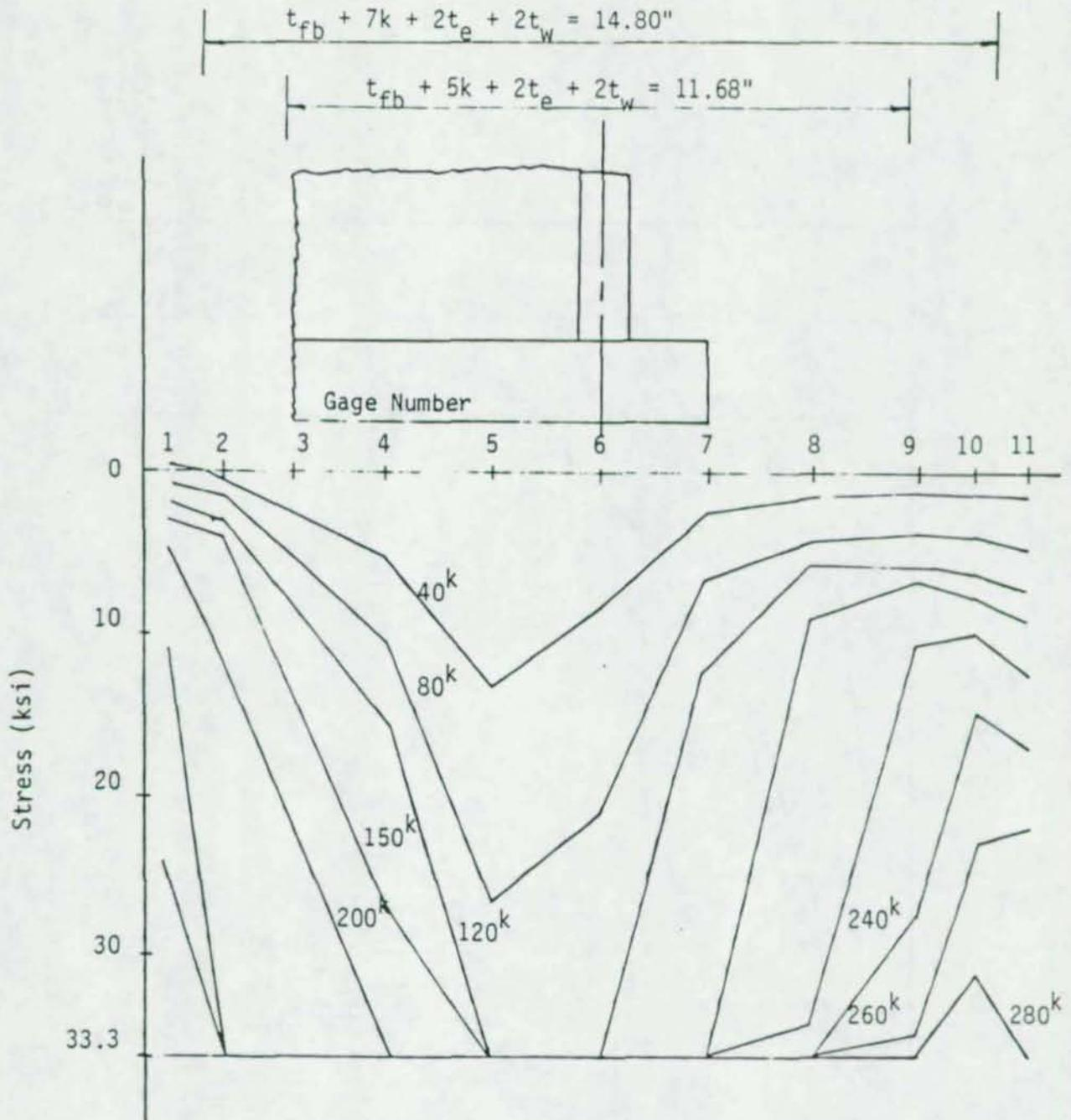
Figure 17. Stress Distribution - Test 3
