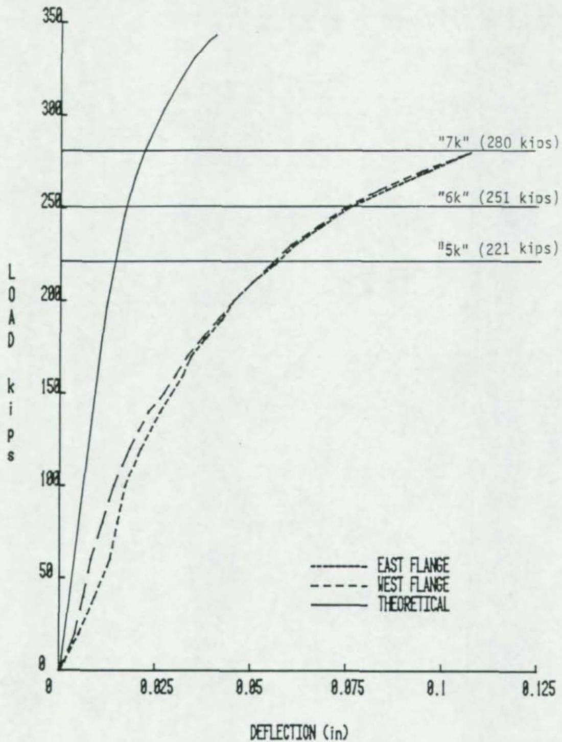
Figure 16. Load vs. Deflection - Test 3
