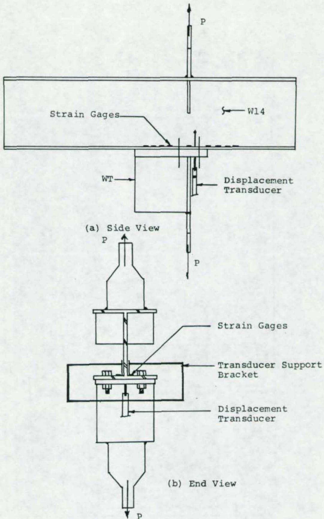
Figure 35. Column Flange Strength Test Set-up
