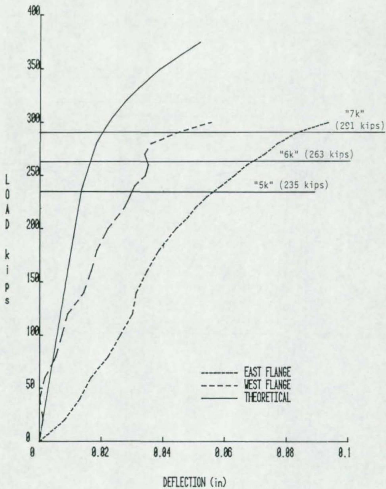
Figure 22. Load vs. Deflection - Test 6
