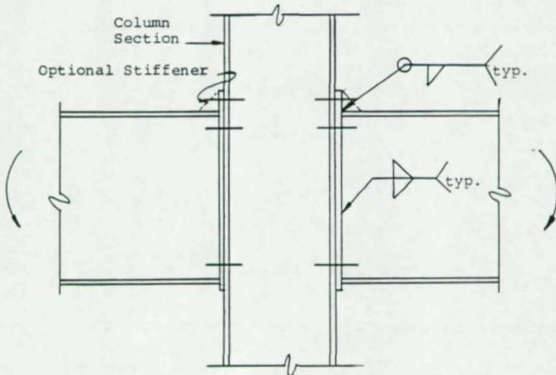
Figure 2. Typical End-Plate Moment Connection
