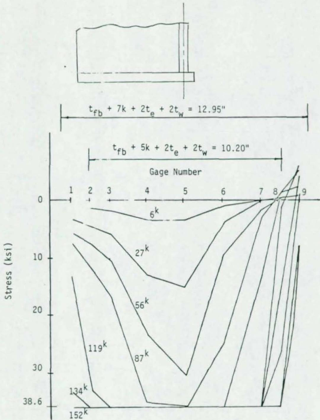
Figure 13. Stress Distribution - Test 1
