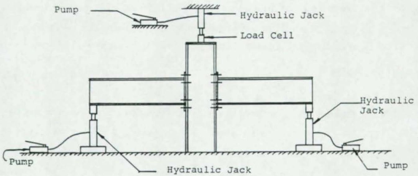
Figure 33. Test Set-up used in Reference 24
