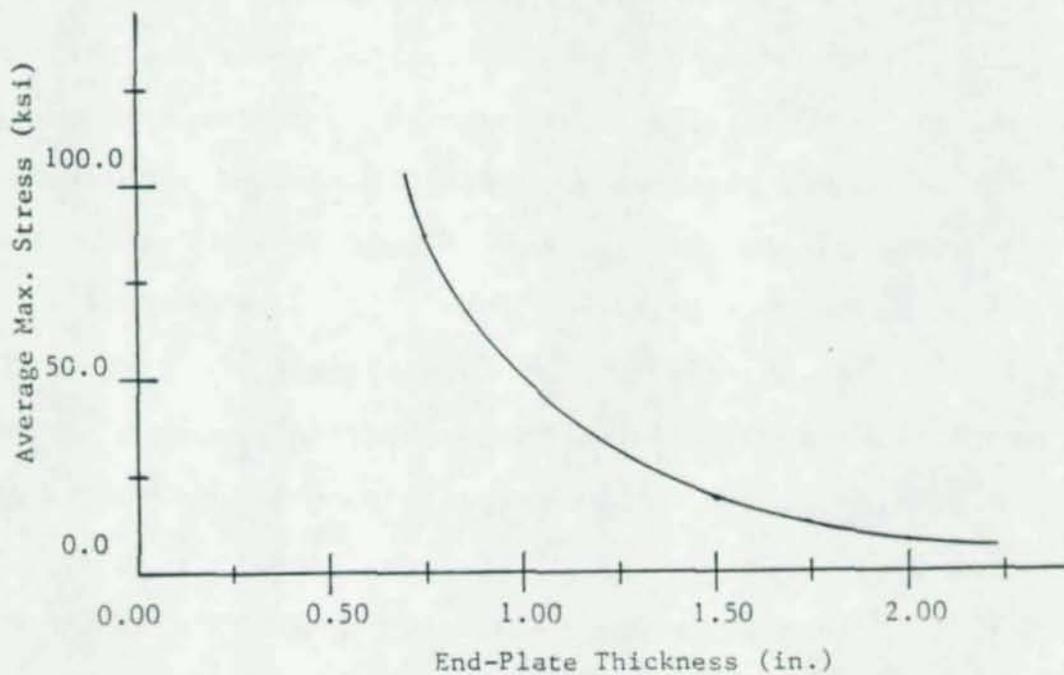
(b) Maximum Bending Stress Versus End-Plate Thickness
