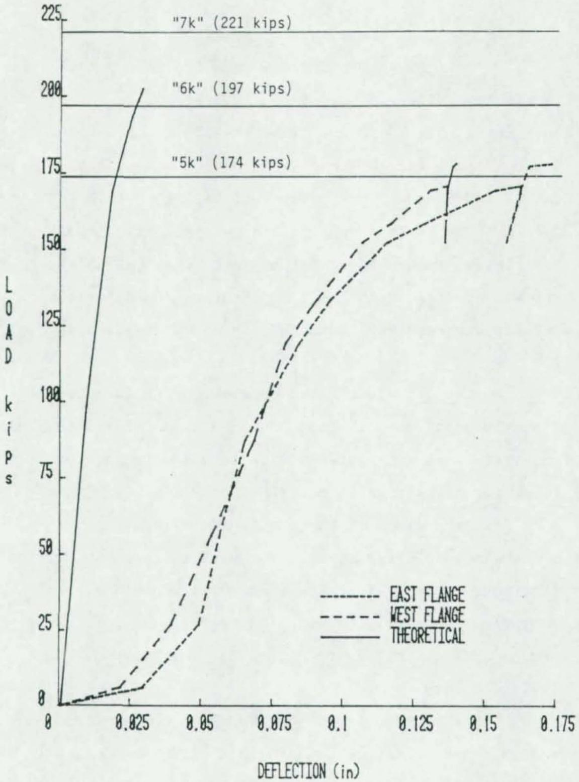
Figure 12. Load vs. Deflection - Test 1
