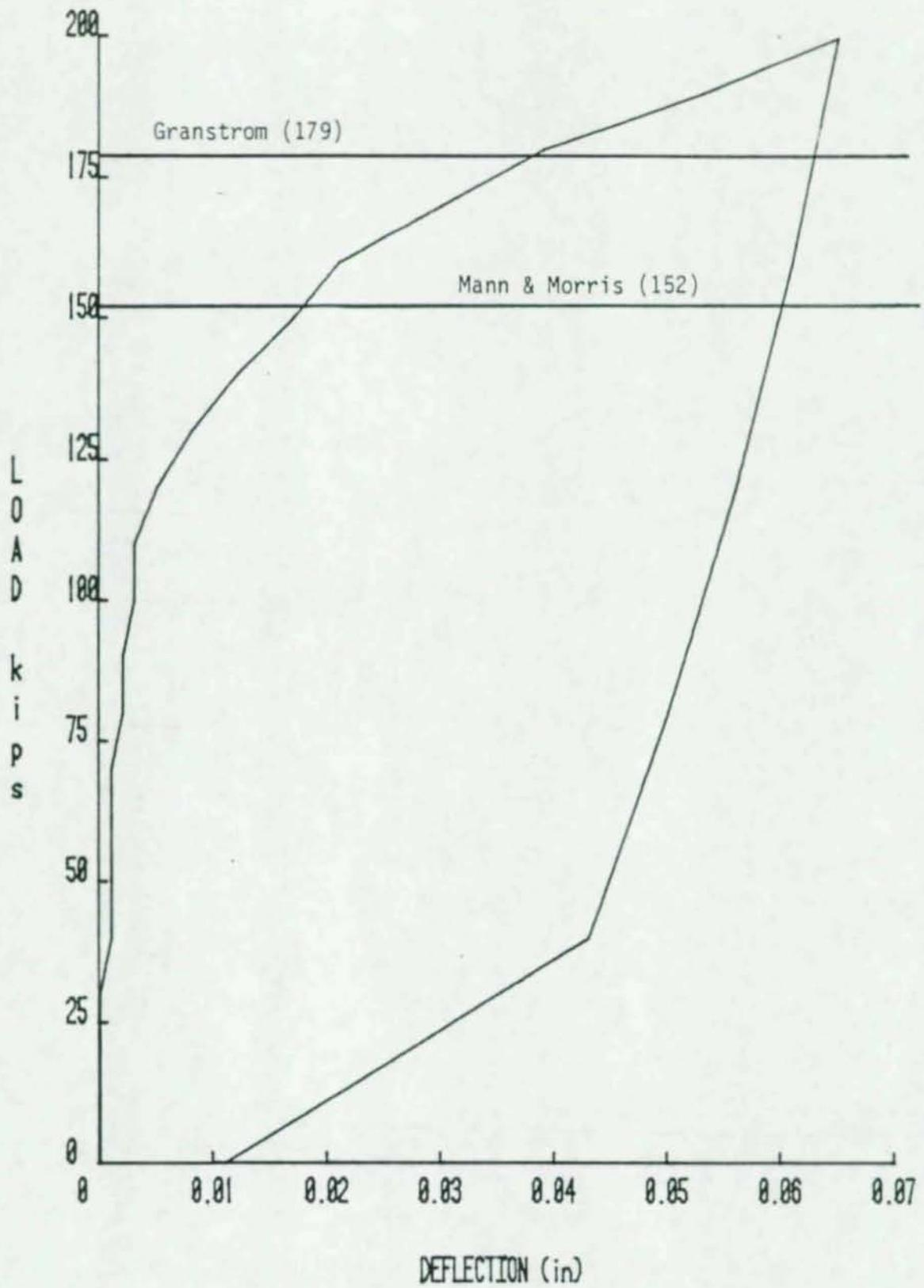
Figure 37. Load vs. Plate Separation - Test 1
