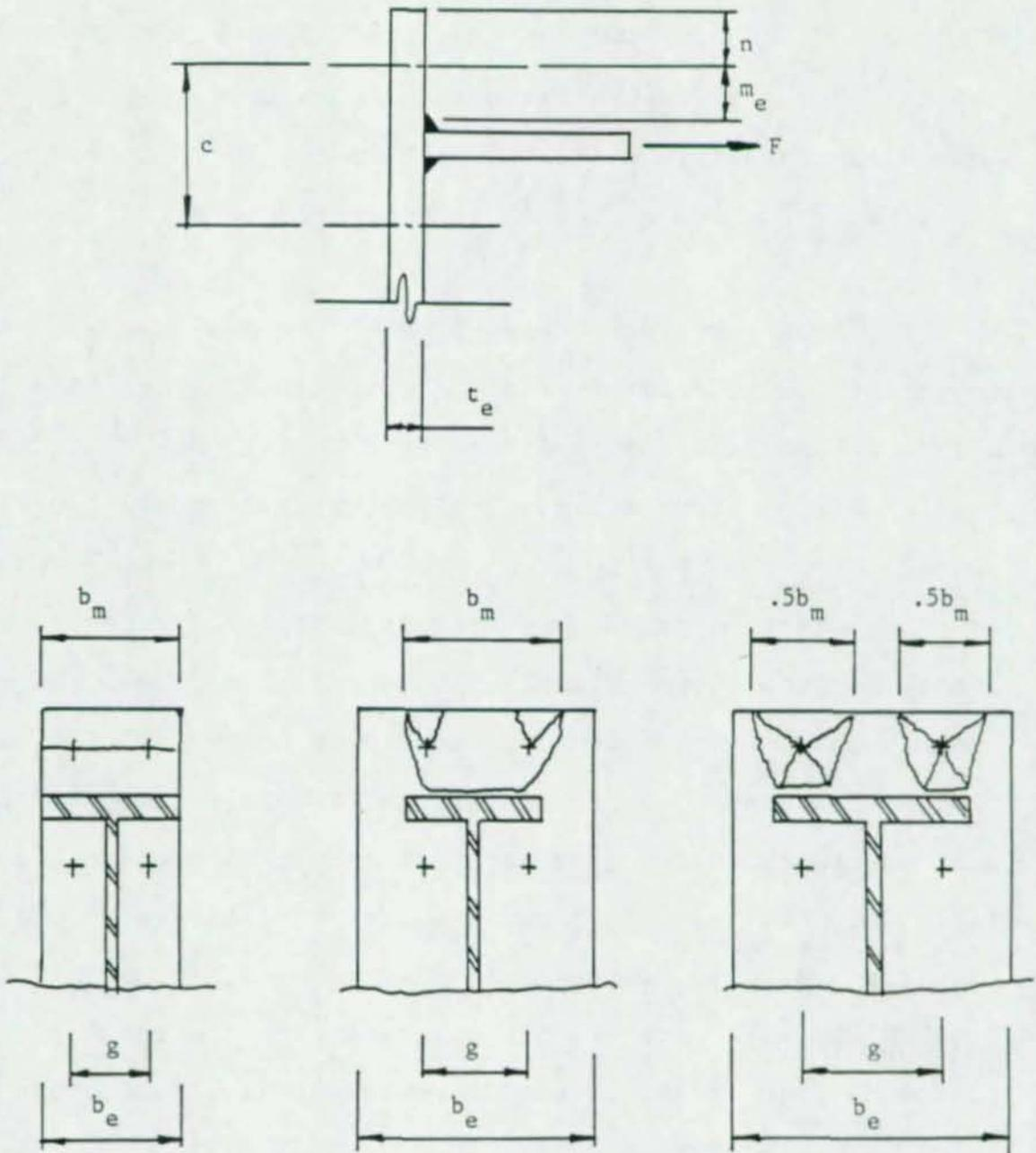
Figure 28. Effective Width of End-Plate
