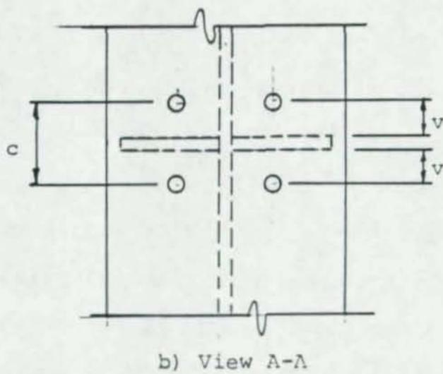
Figure 29. Stiffened Column Web and Flange used in Reference 6.
