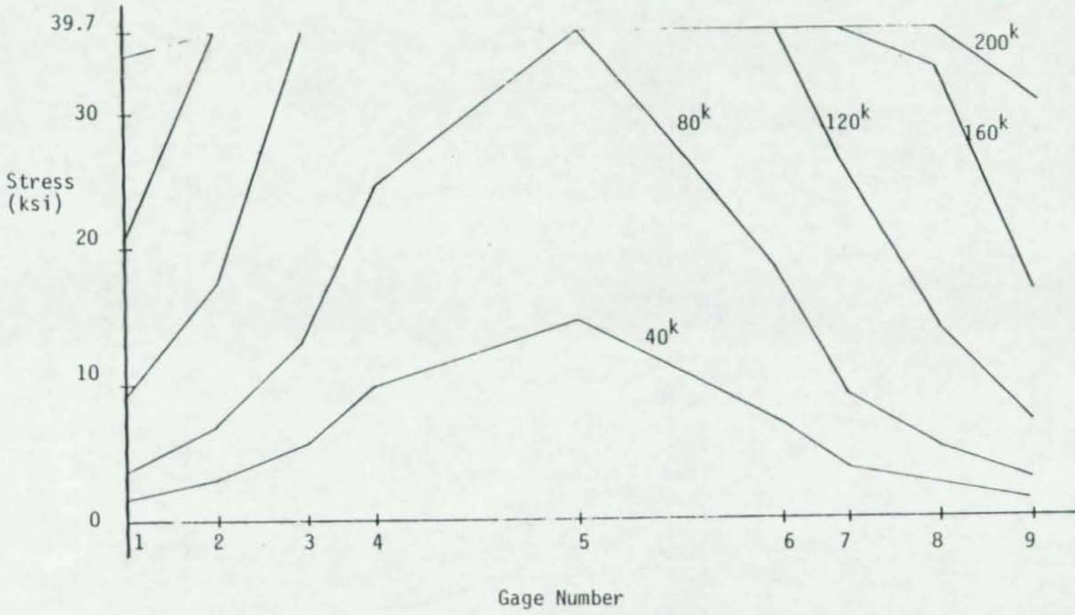
Figure 42. Flange Stress Distribution - Test 3
