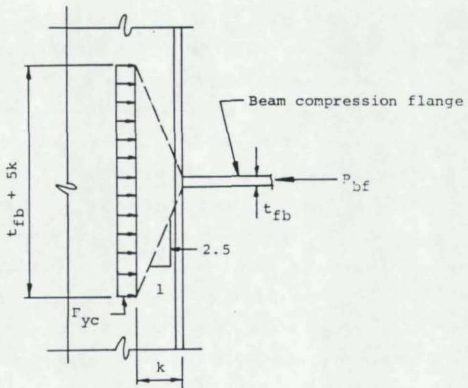
Figure 4. Distribution of Stresses at Beam Compression Flange
