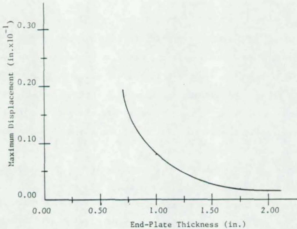
(a) Maximum Displacement Versus End-Plate Thickness
