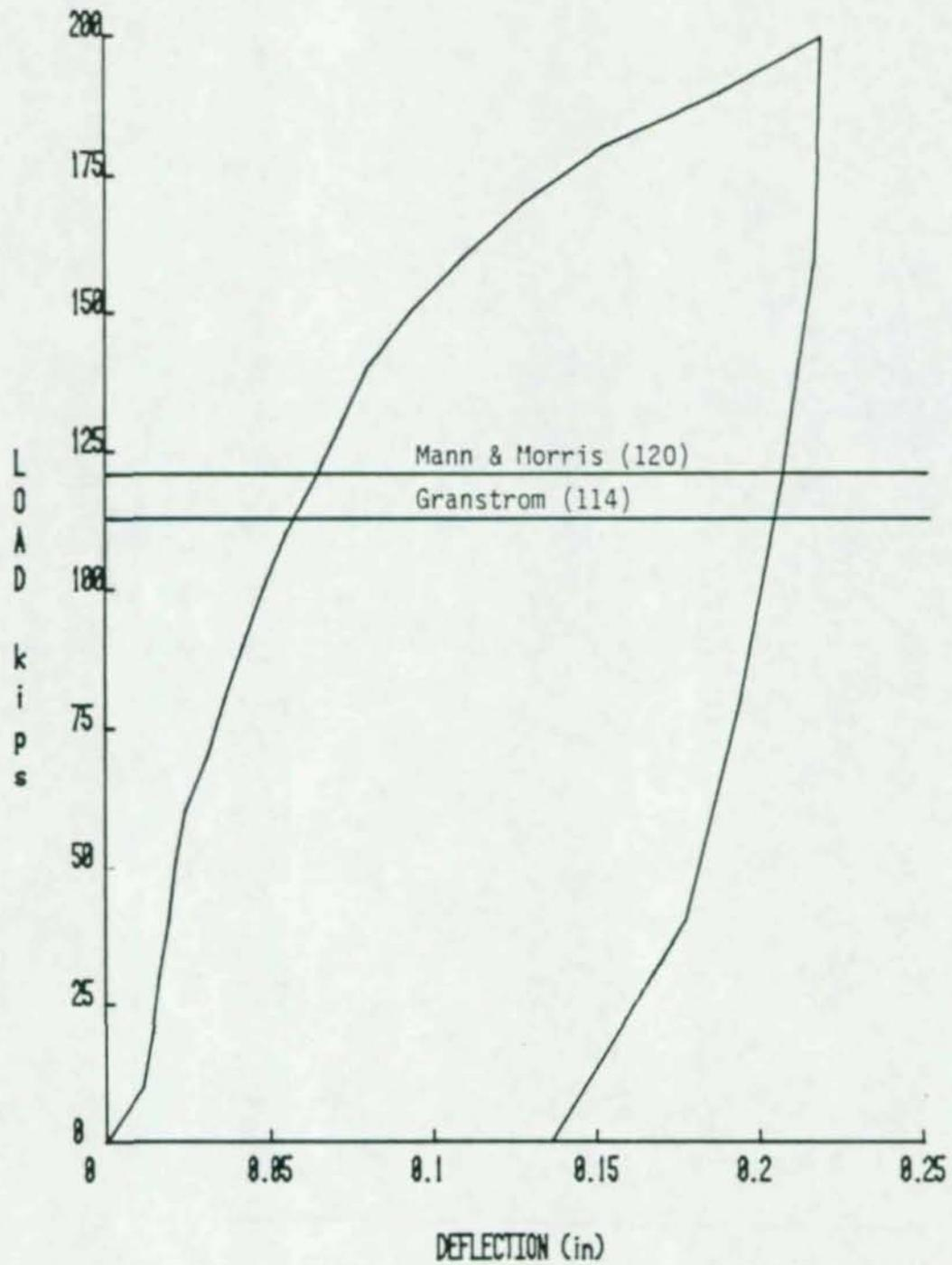
Figure 41. Load vs. Plate Separation - Test 3
