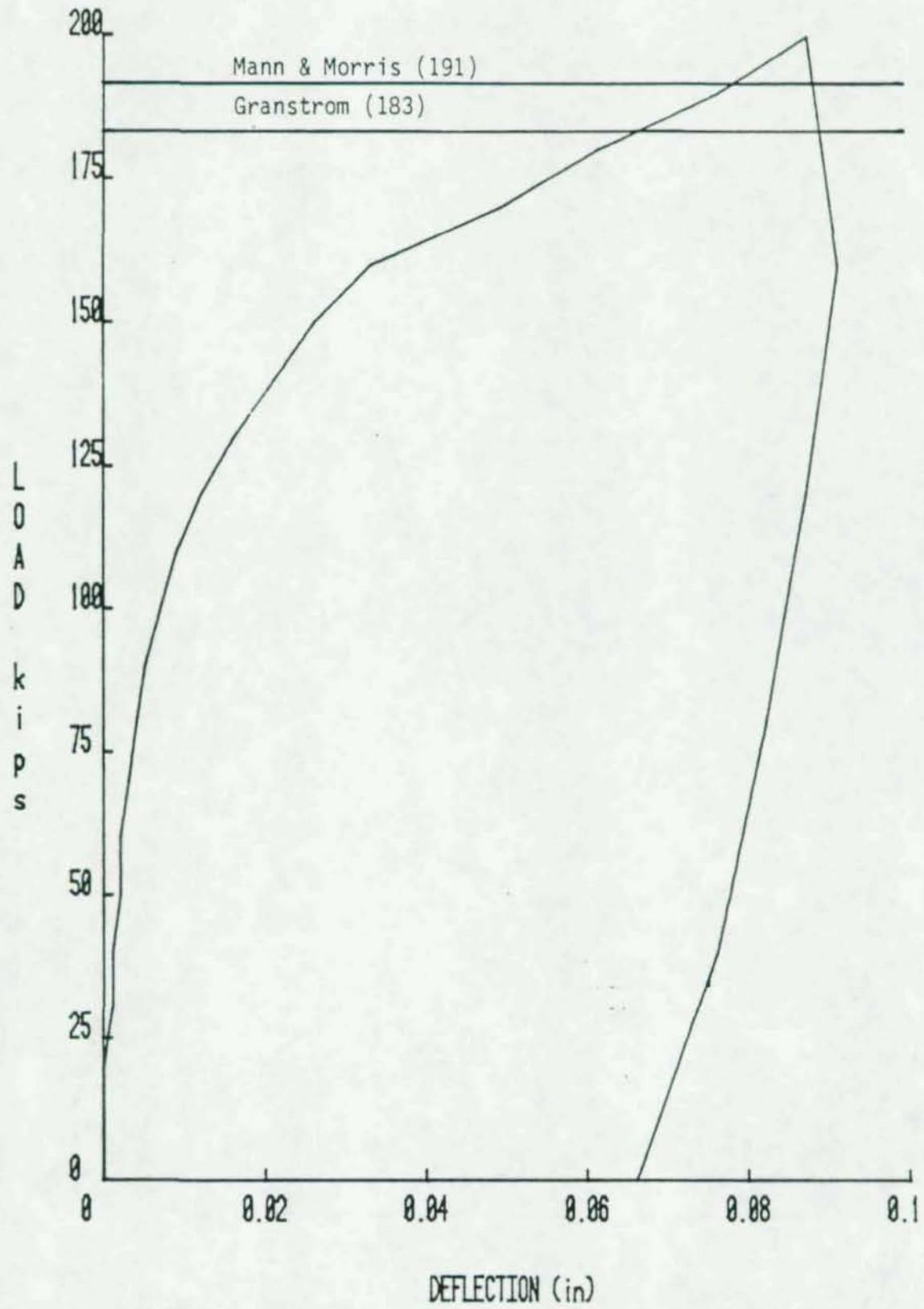
Figure 39. Load vs. Plate Separation - Test 2
