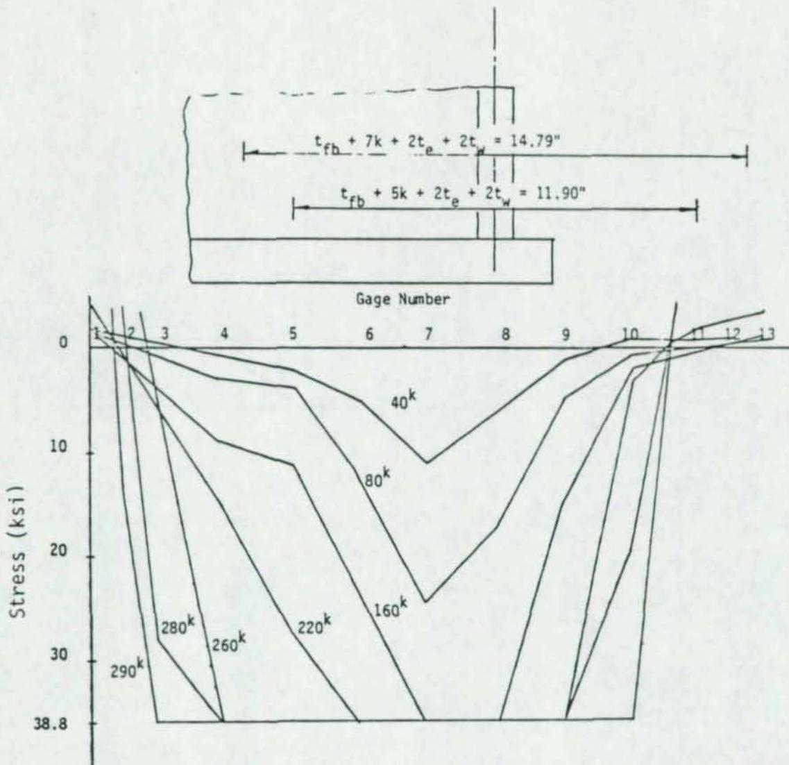
Figure 21. Stress Distribution - Test 5
