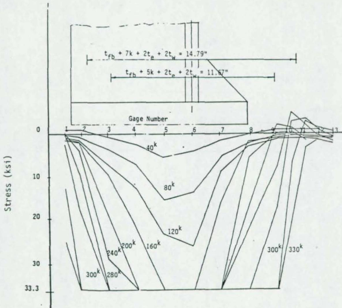
Figure 19. Stress Distribution - Test 4
