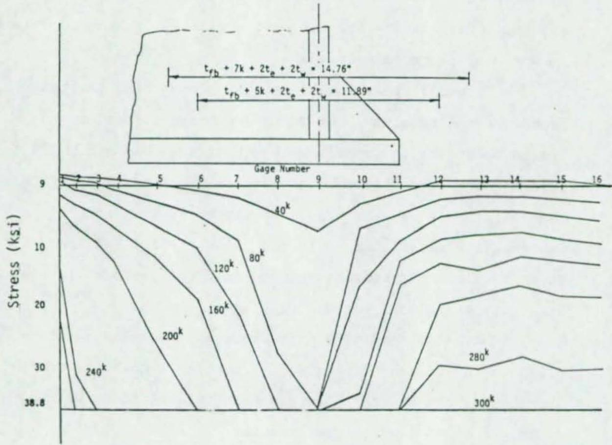
Figure 23. Stress Distribution - Test 6
