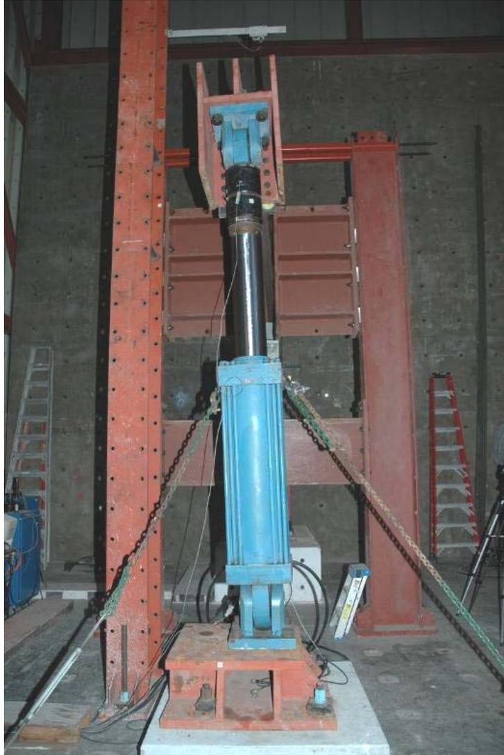
Figure 3.5 Specimen BFP-1: Actuator Skewed to East Side at +6% Drift (2nd Cycle)
