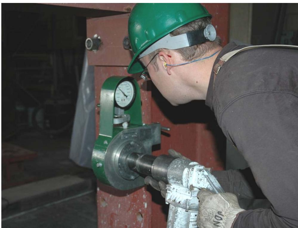
Figure 2.12 Tension Control Bolt Pretension Verification
