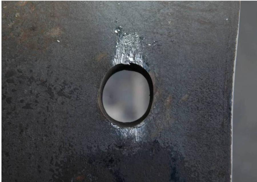
Figure 3.25 Specimen BFP-2: Beam Flange Bolt Hole Ovalization and Necking at Outermost Bolt Row (after Testing)
