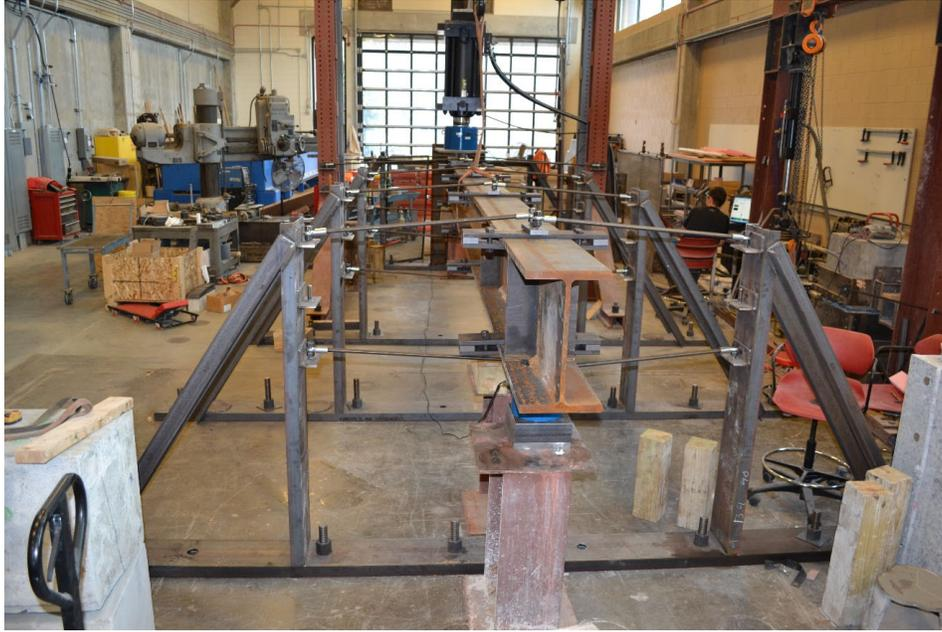
Figure 26: View from tail end of beam showing lateral bracing (Specimen 5A)
