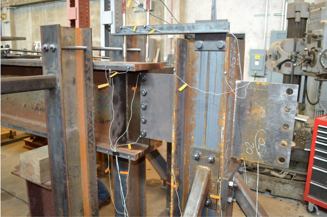
Figure 27: Instrumentation at the connection (Specimen 5D)
