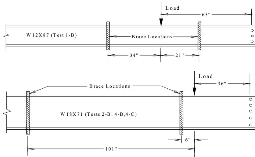
Figure 4.7a: Bracing locations for Phase I and II tests
