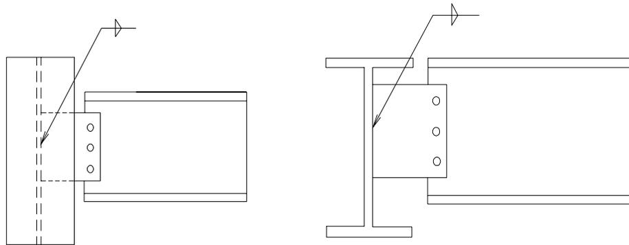
Figure 2.1: Unstiffened extended shear tabs
