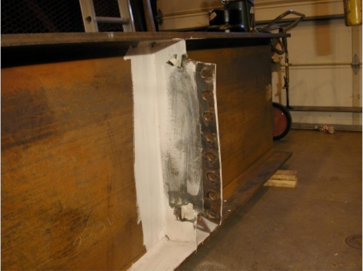
Figure I.10: Girder showing various failure modes after testing (Test 7-C)
