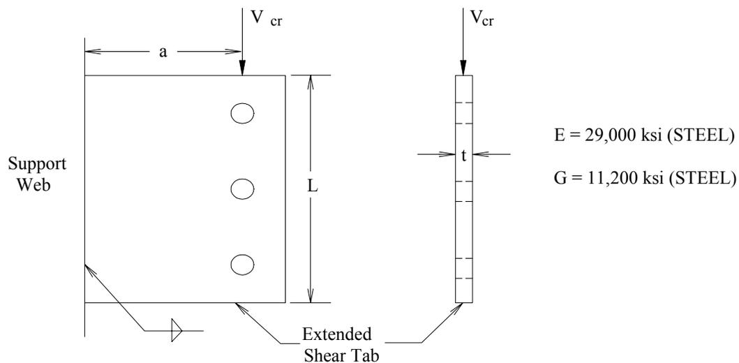
Figure 4.6: Schematic for tab thickness determination for the unstiffened tests
