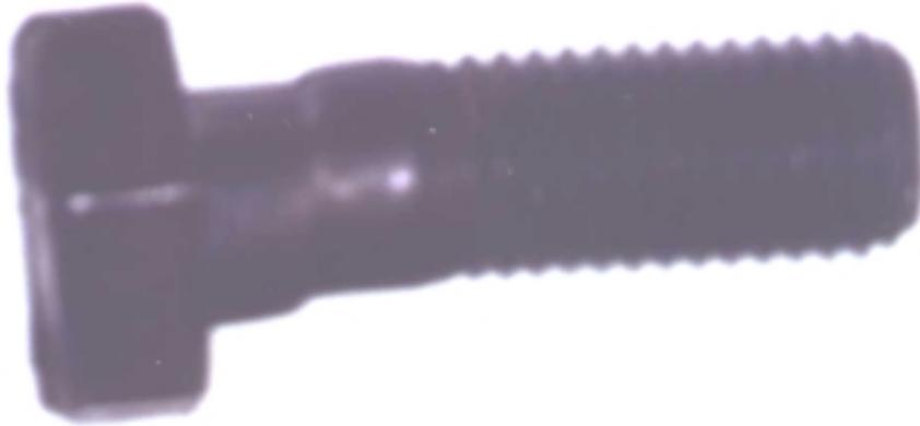
Figure I.1: Bolt Shear (Test 1-U)
