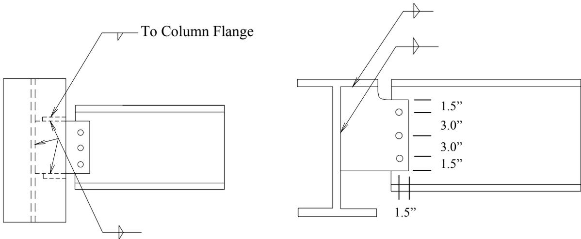
Figure 2.2: Stiffened extended shear tabs
