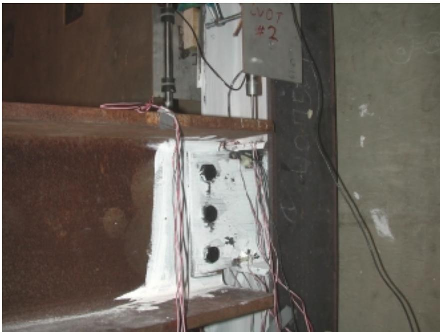
Figure B.12: Stiffened extended shear tab with strain gages and wiring (Test 3-G)
