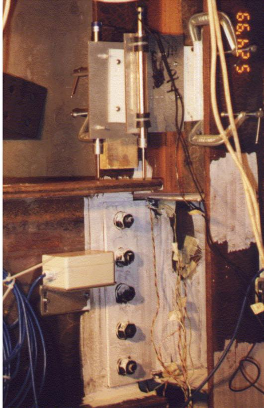
Figure B.11: LVDT setup for column tests (Test 4-C)
