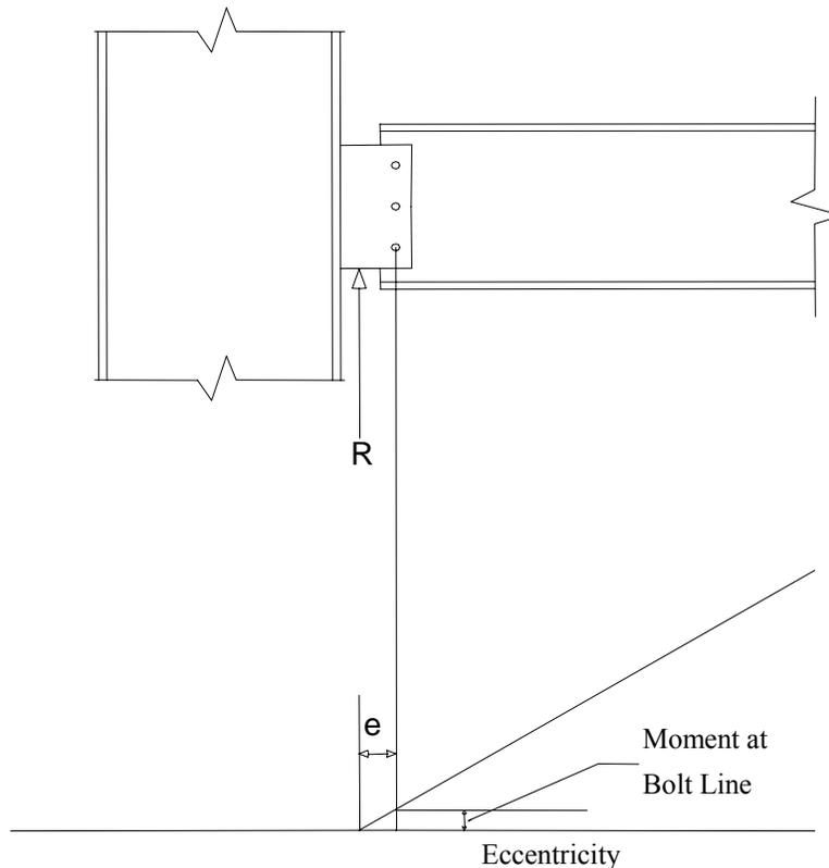
Figure 3.1: Determination of connection moment
