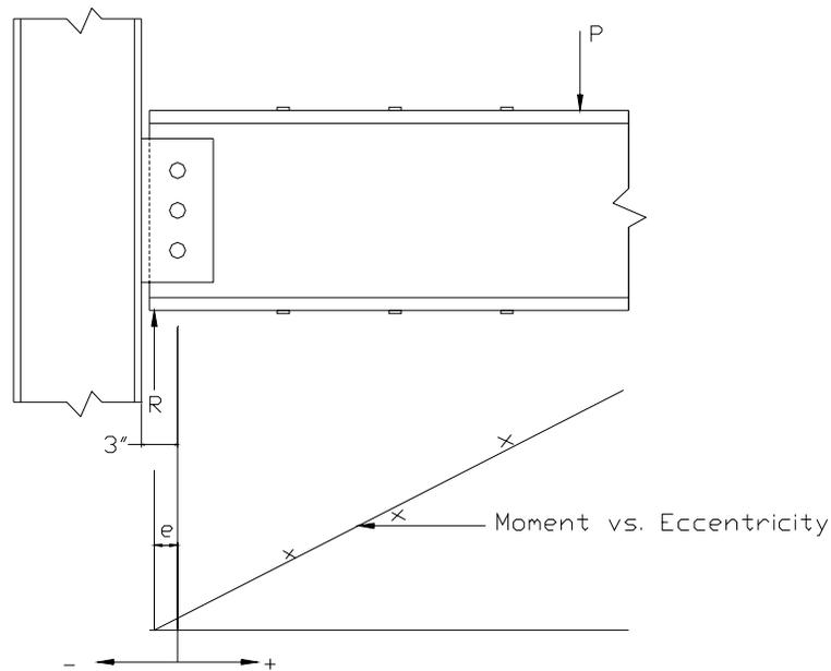
Figure 5.4: Sign convention for shear force eccentricity
