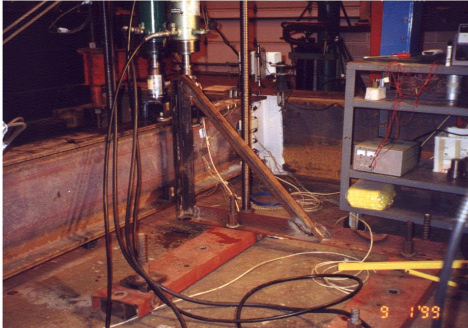
Figure B.7: Bracing near the point of loading (Test 2-B)
