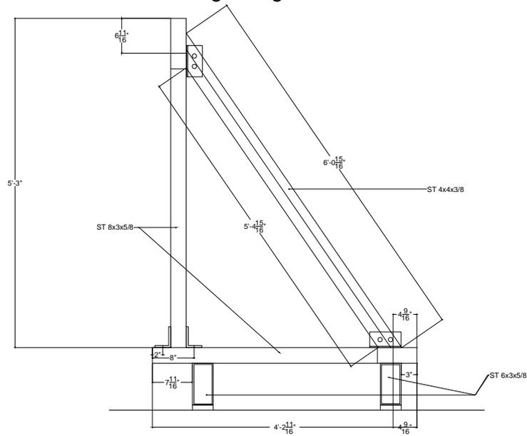
Figure M.2: Side view of the triangular brace serving as the vertical rolling surface
