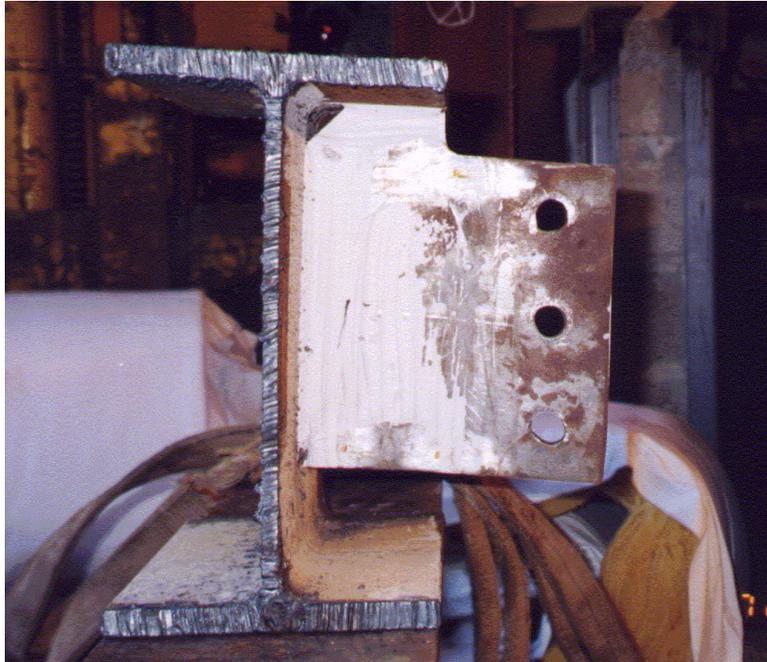
Figure I.3: Shear Yield (Test 1-A)
