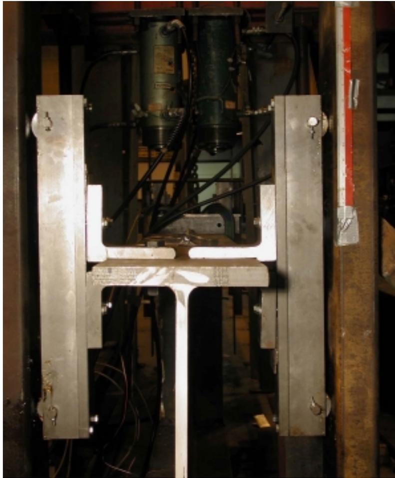
Figure B.15: View of rotational-lateral bracing roller system
