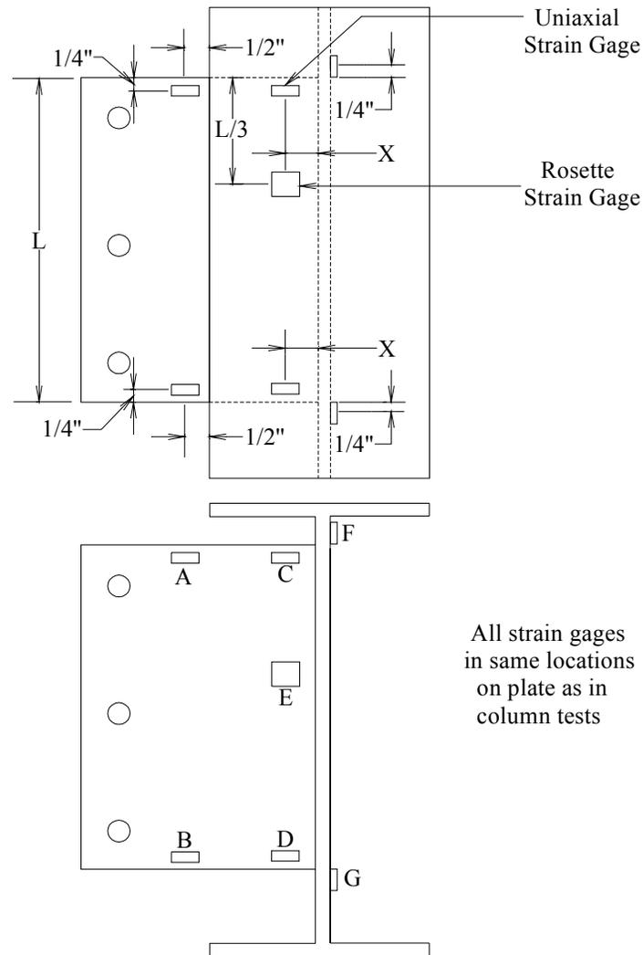
Figure 4.10a: Strain gage locations on shear tabs
