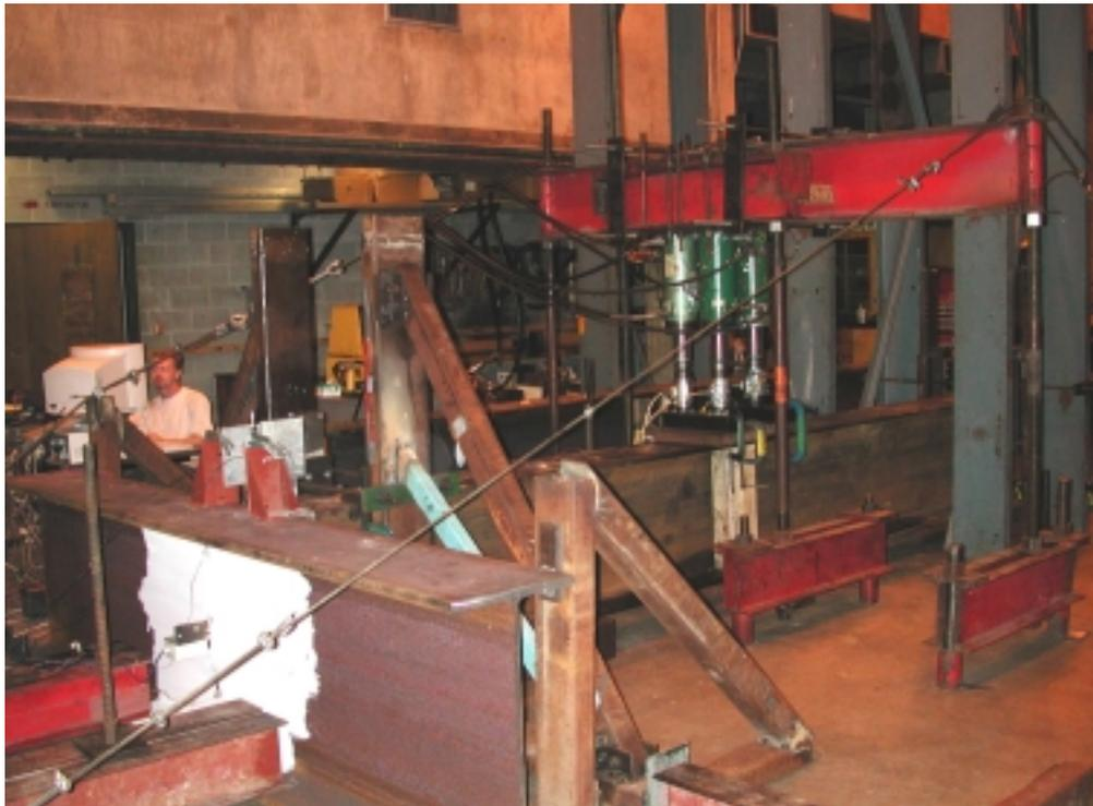
Figure B.4: Typical test setup for Phase III girder test (Test 5-A)
