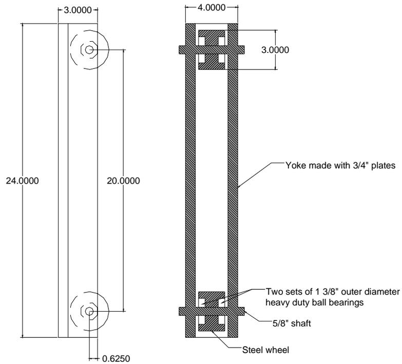
**Figure M.4: Detail of the roller yoke**
