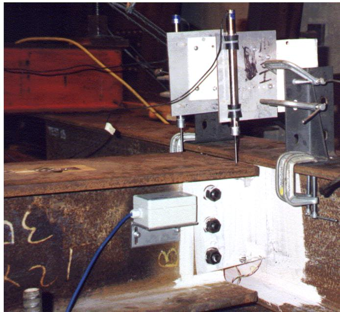
Figure B.10: LVDT setup for girder tests (Test 1-B)
