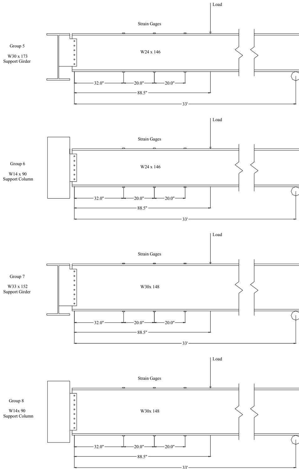
Figure 4.2b: Setups for beam and support member combinations in Phase III
