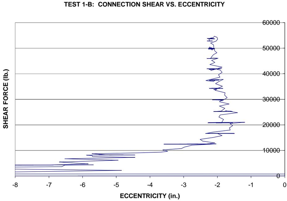
Figure 5.5: Shear force vs. eccentricity (All Data)
