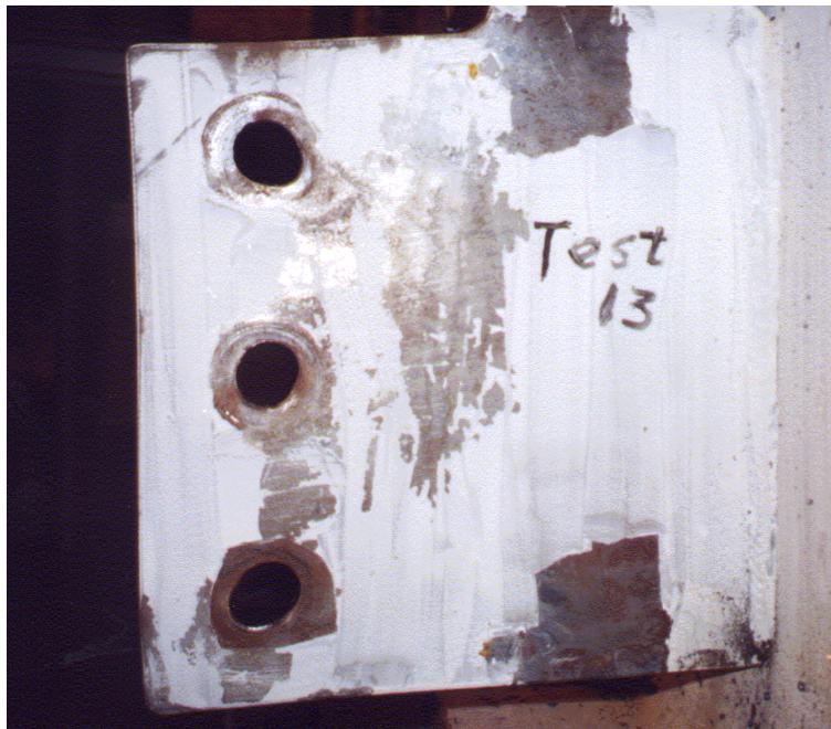
Figure I.2: Bolt Bearing (Test 1-A)
