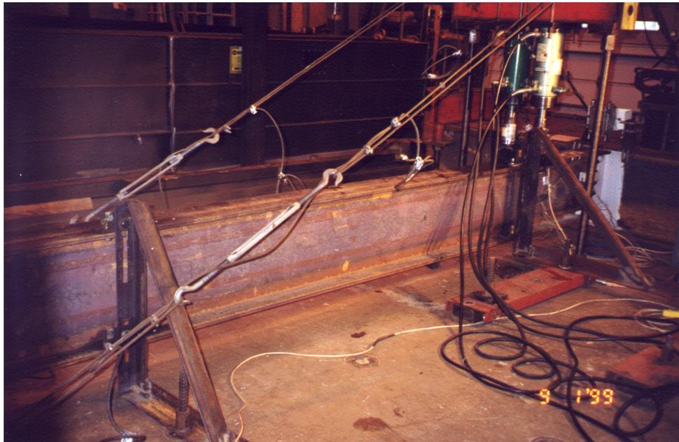
Figure B.8: Bracing locations for girder test (Test 2-B)
