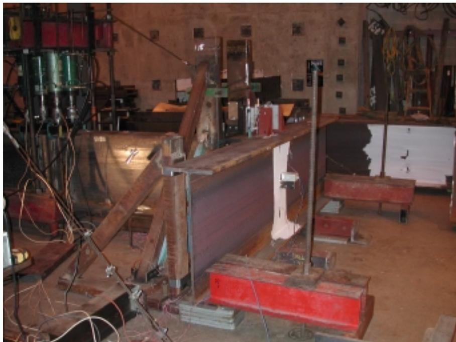
Figure B.14: Girder bracing for Phase III girder tests (Test 5-B)
