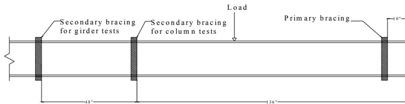
Figure 4.7b: Bracing locations for Phase III tests
