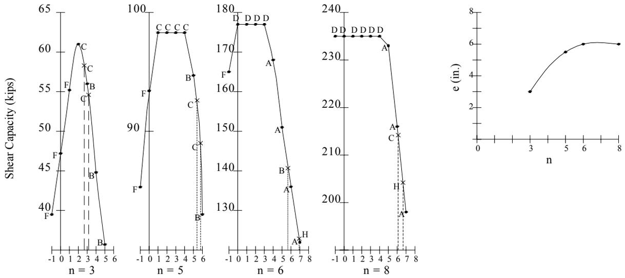
Figure B - Eccentricities for Column Connections
