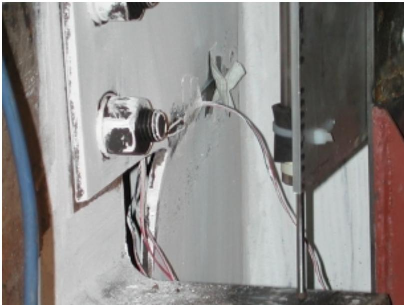
Figure I.9: Plate extension buckling (Test 7-C)
