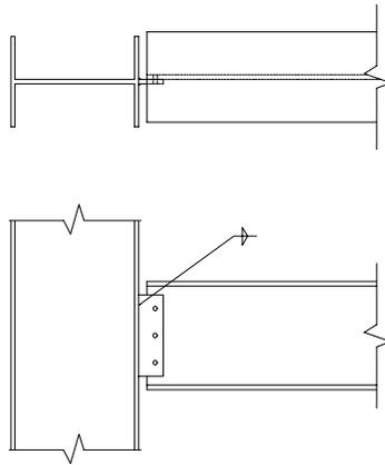
Figure 1.1: Typical shear tab connection to column flange
