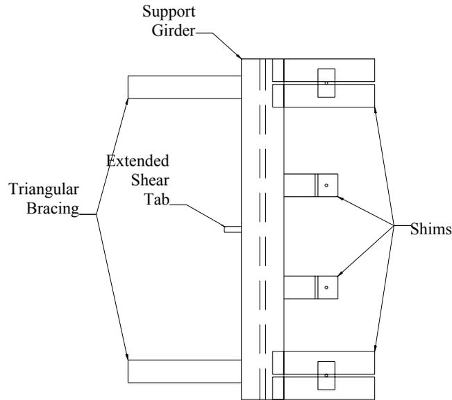
Figure 4.5b: Test girder supports for Phase III
