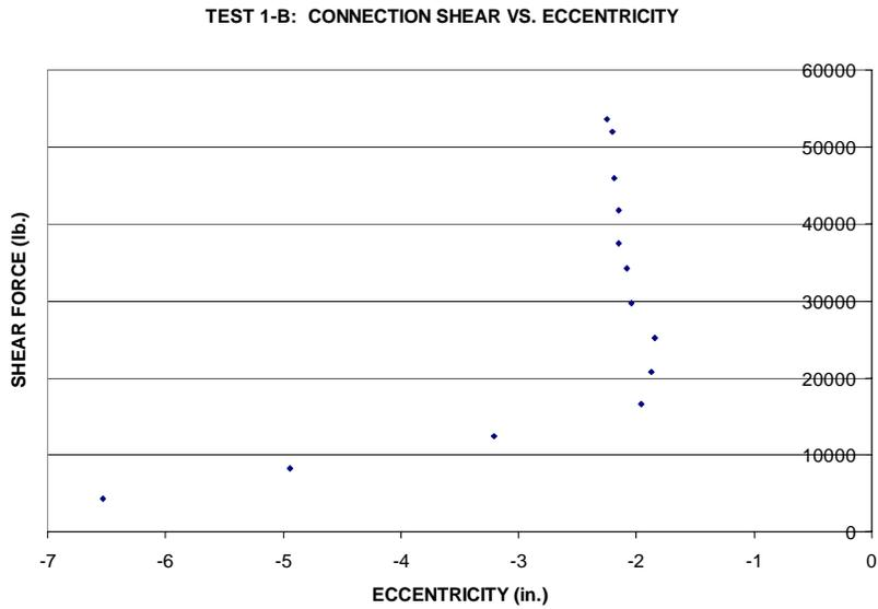
Figure 5.6: Shear force vs. eccentricity (5000 lb. load increments)
