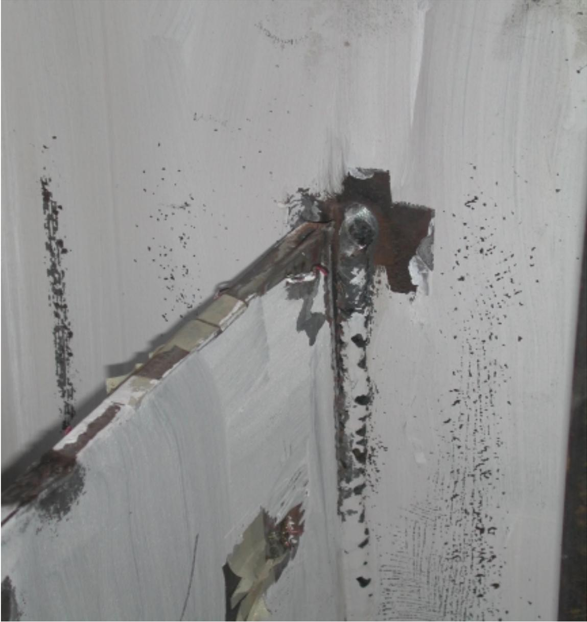
Figure I.7: Tearing of weld near top of shear tab (Test 6-U)
