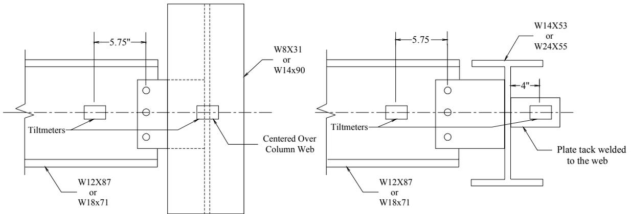
Figure 4.9: Location of tiltmeters
