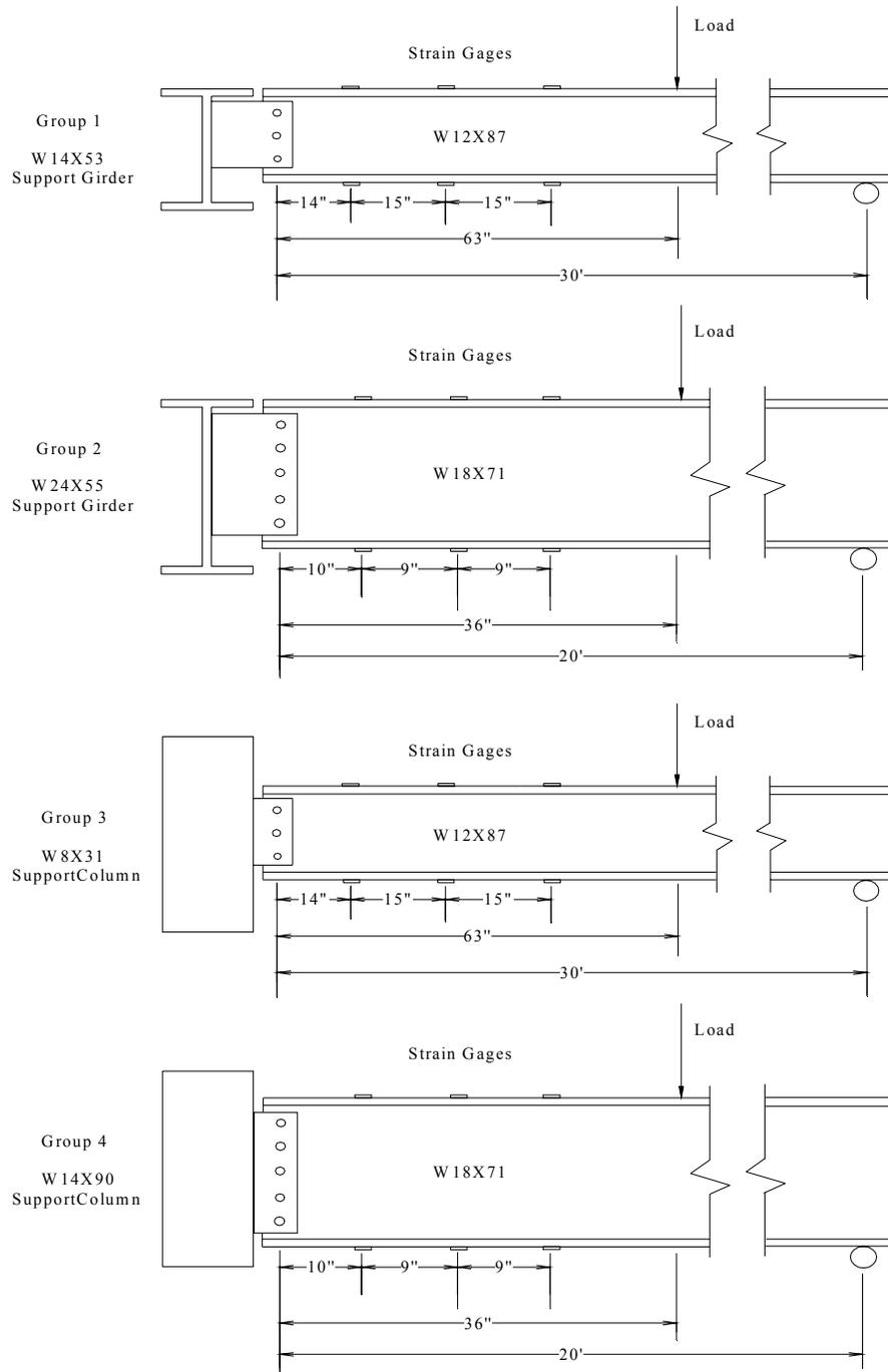
Figure 4.2a: Setups for beam and support member combinations in Phases I and II
