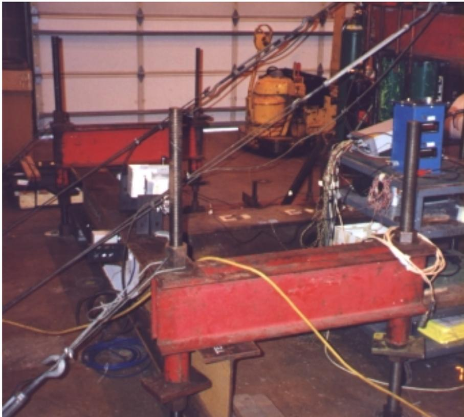
Figure B.6: Typical Phase I girder tie-downs (Test 1-B)
