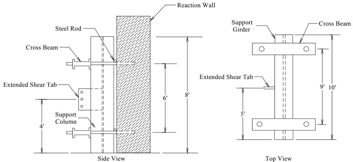
Figure 4.5a: Test column and girder supports
