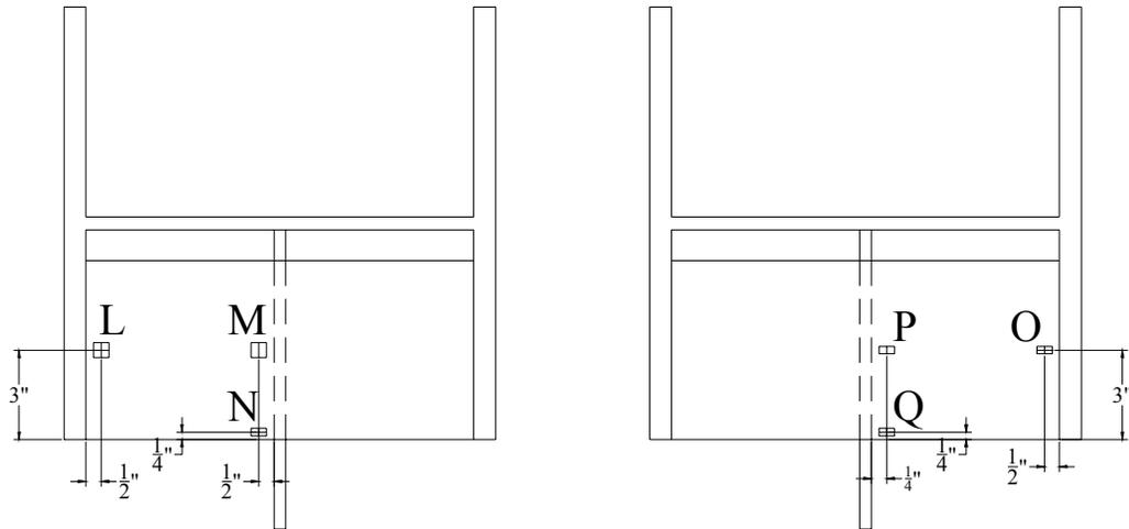
Figure 4.10b: Strain gage locations on stiffeners
