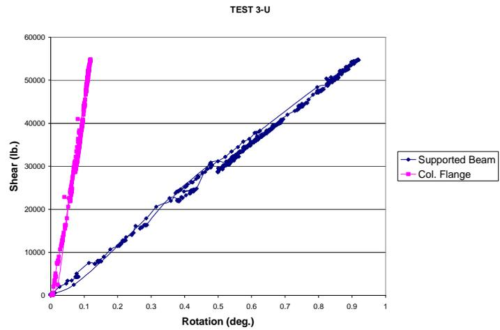
\*NOTE: Tiltmeter mounted to column flange gives unrealistic web rotation for this test.
