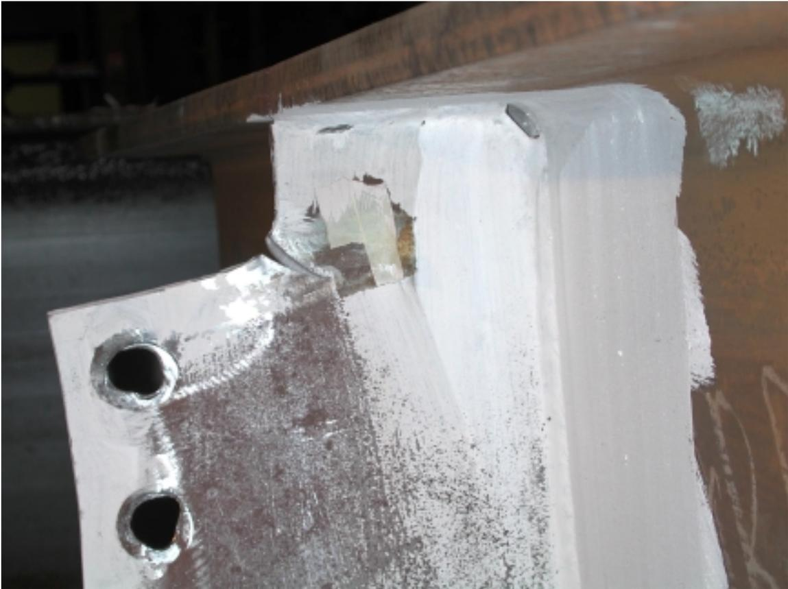
Figure I.8: Tearing of the shear tab (Test 7-C)
