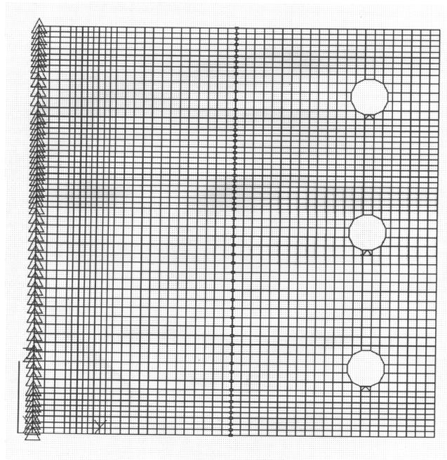
Figure J.2: F.E.A. mesh size and load location
