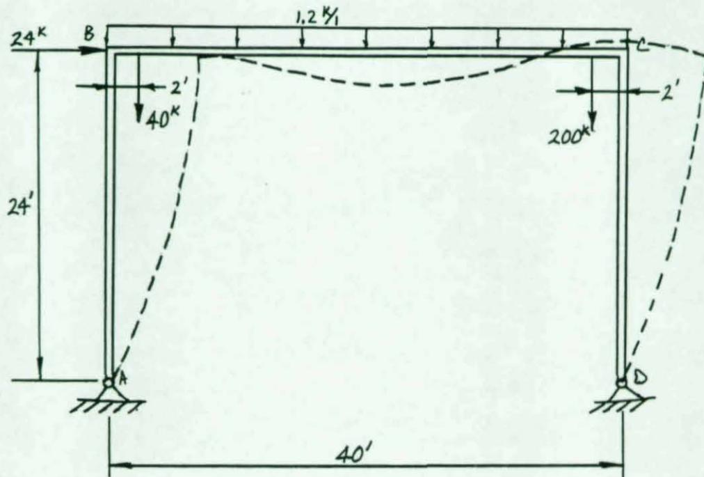
PRELIMINARY ANALYSIS - ASSUME POINTS OF CONTRAFLEXURE OCCUR AT POINTS 4ft FROM POINT B AND 8ft FROM C.
