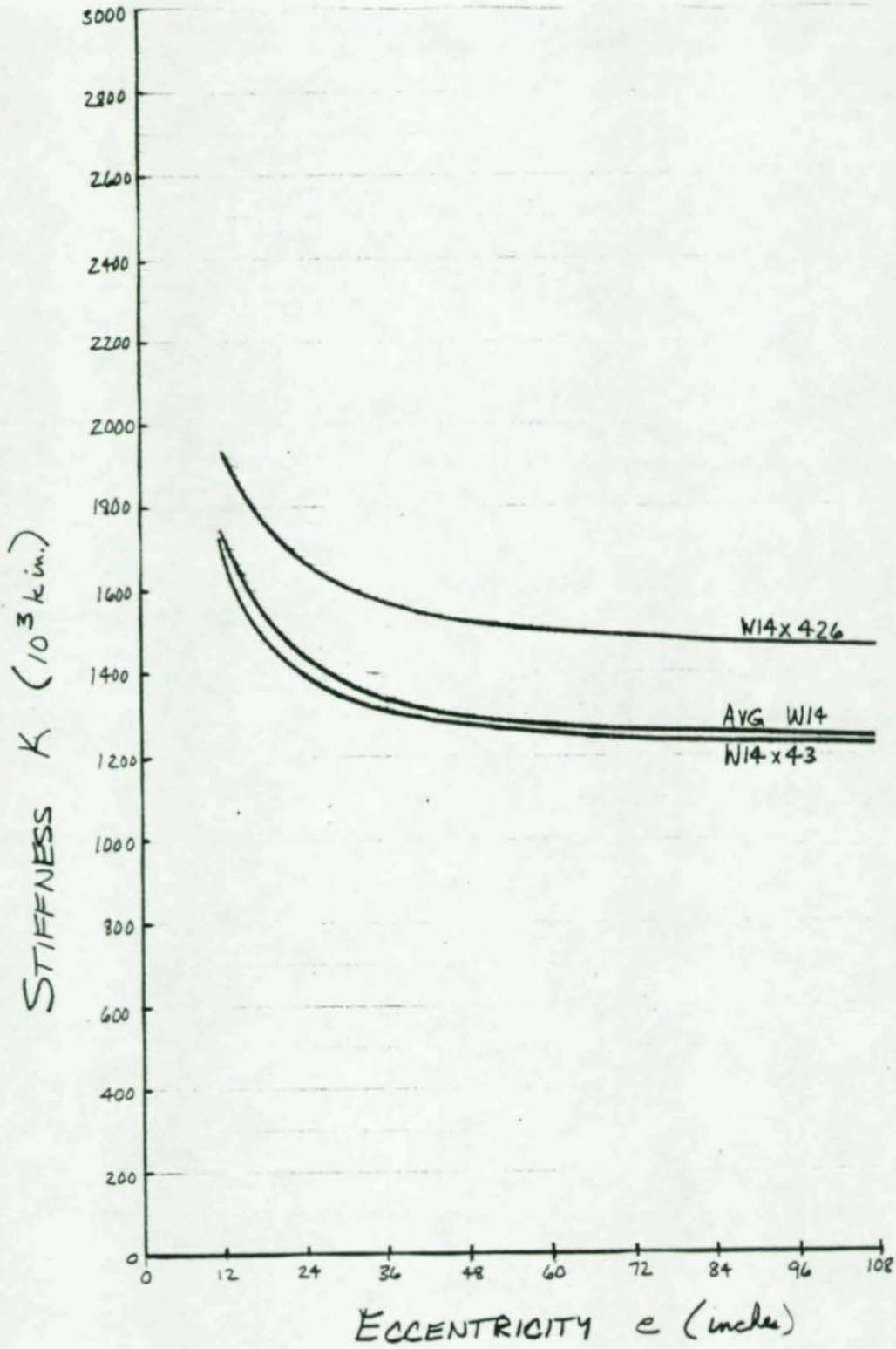
FIGURE 9 - COMPARISON OF STIFFNESS FOR W14 COLUMNS.
