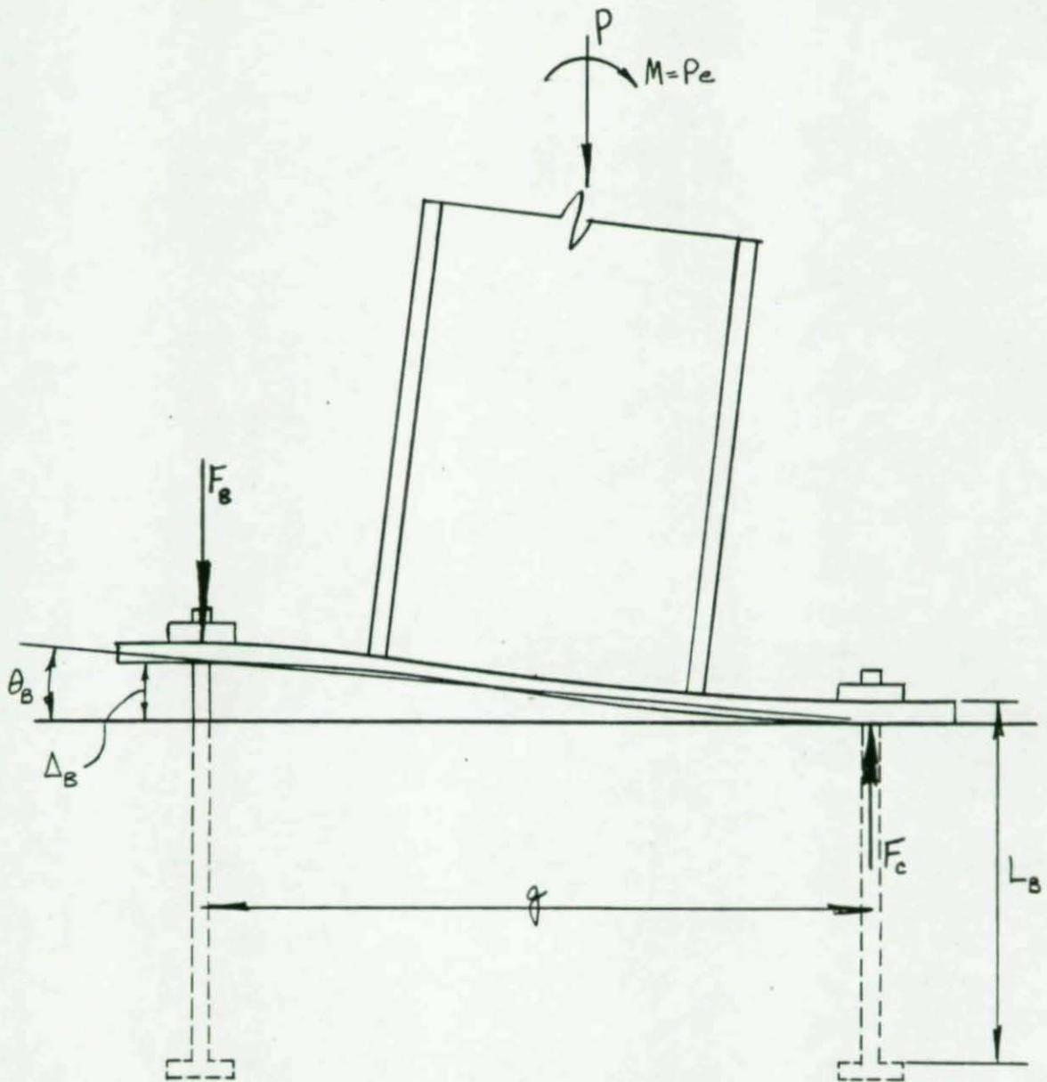
$A_B = \text{TOTAL AREA OF TENSION ANCHOR BOLTS.}$
