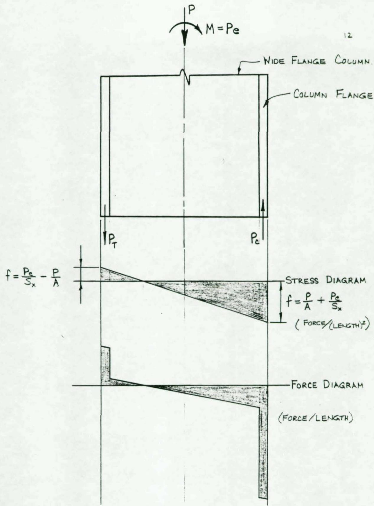
FIGURE 4 - STRESS AND FORCE DISTRIBUTIONS ON COLUMN.
