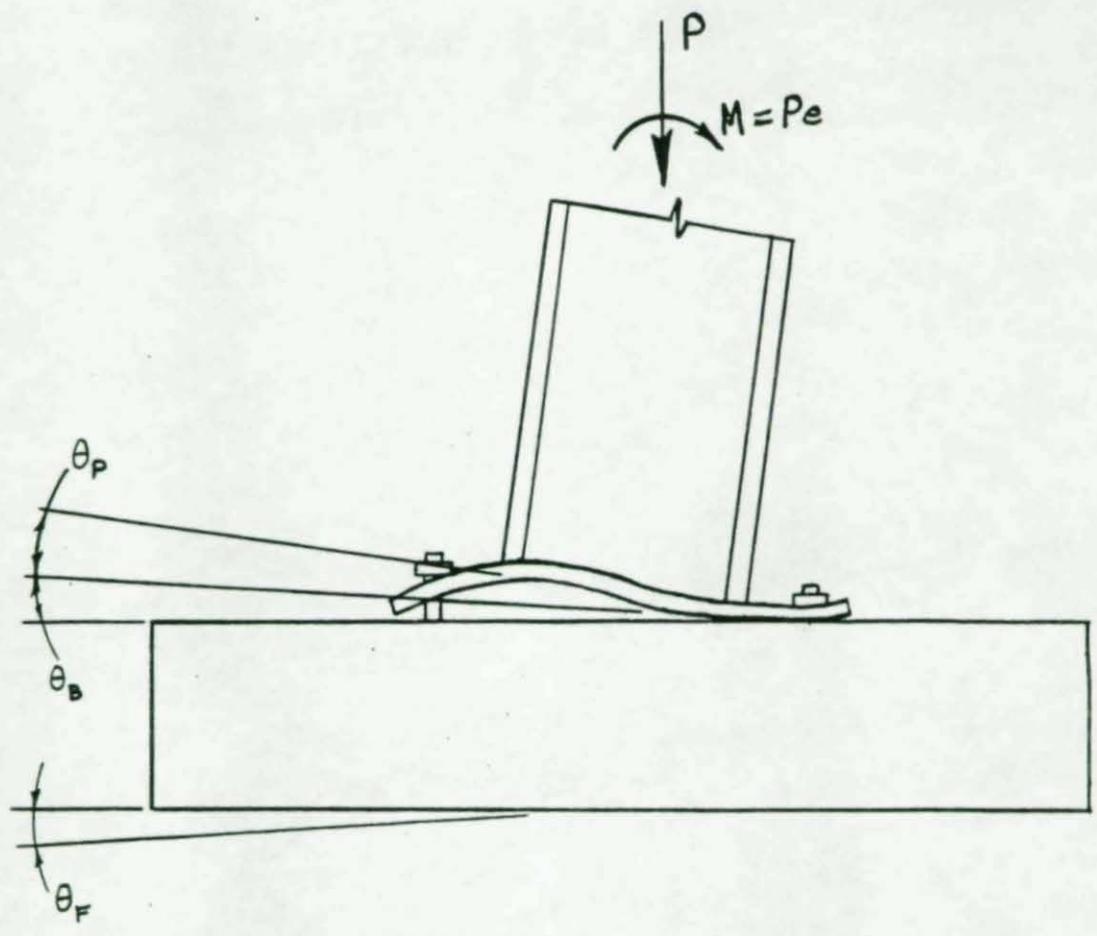
FIGURE 2 - THREE COMPONENTS OF ROTATION.
