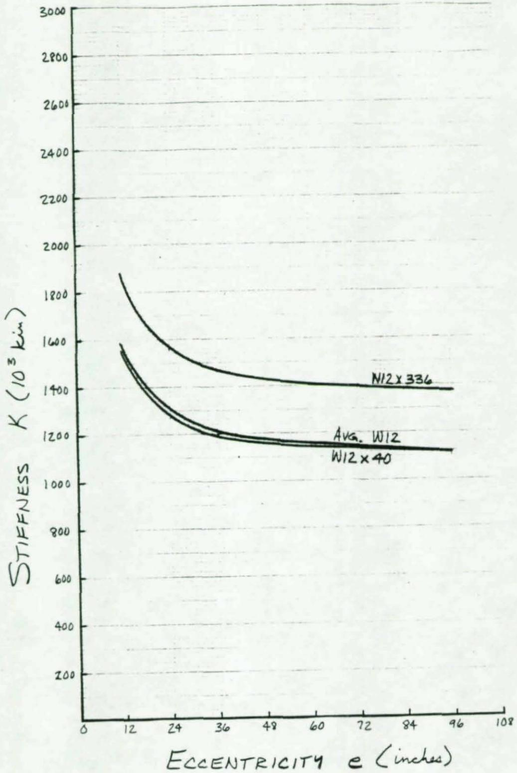
FIGURE 10 - COMPARISON OF STIFFNESS FOR W12 COLUMNS.
