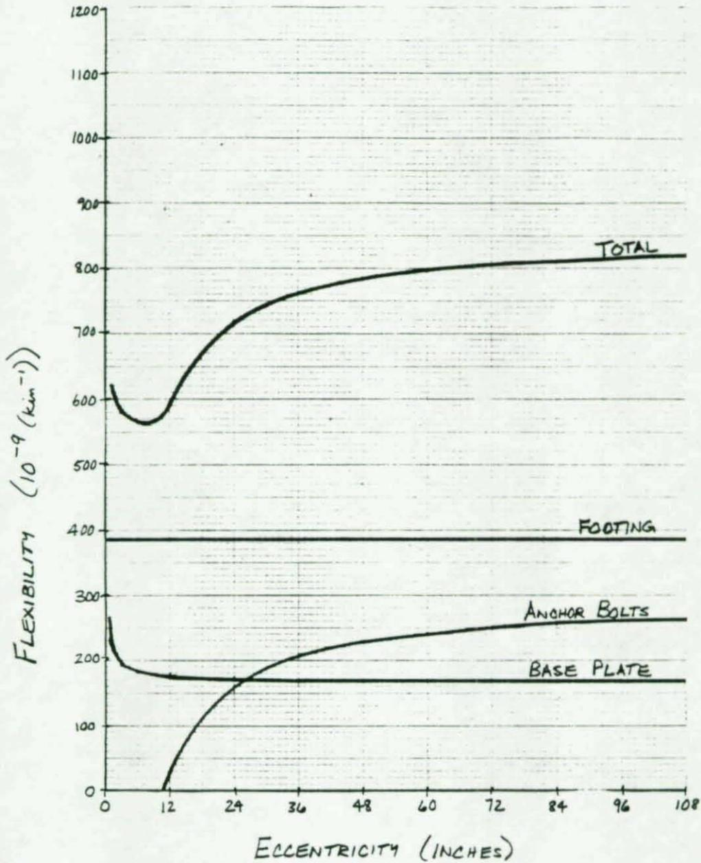
FIGURE 8 - COMPARISON OF THREE COMPONENTS OF THE BASE FLEXIBILITY.
