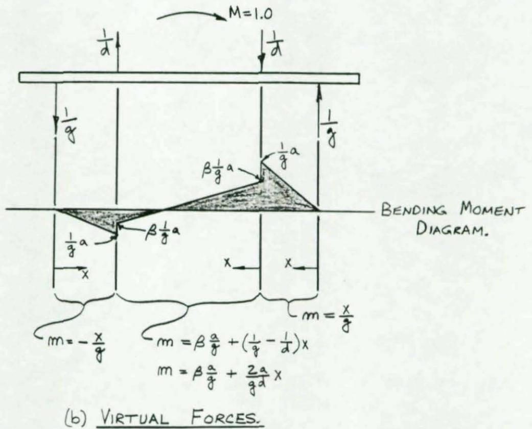
FIGURE 6 - FORCES ON BASE PLATE AND RESULTING BENDING MOMENT DIAGRAMS.
