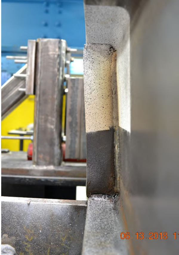
Figure A-107: Side view of W10X19-SC-E0 after testing showing the stiffener conditions
