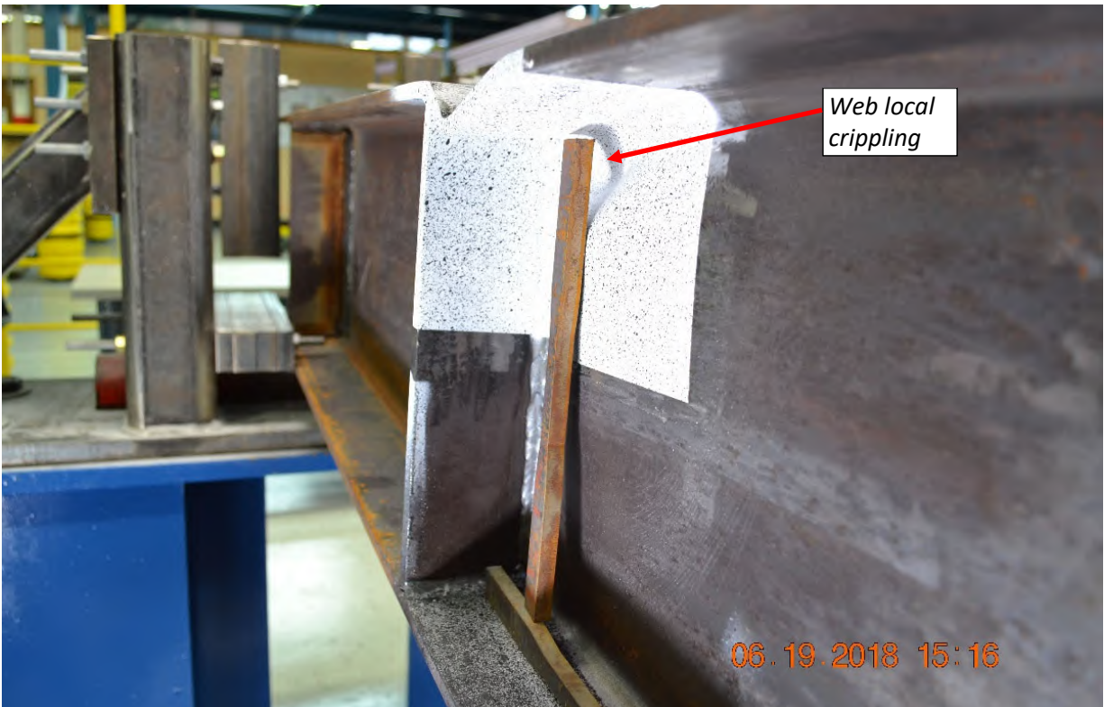
Figure A-65: W12X26-SC-E2 after testing emphasizing web crippling
