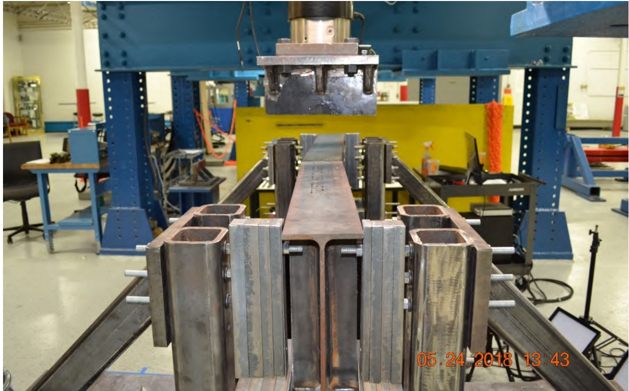
Figure A-16: Side view of W16X31-SC-E0 after testing showing lateral-torsional buckling
