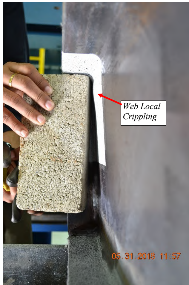
Figure A-101: W10X19-DC-E2 after testing emphasizing web crippling
