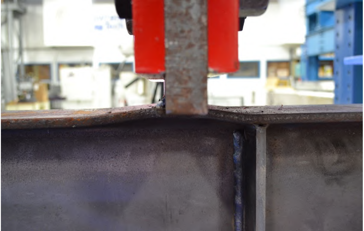
Figure A-135: Close-up view of W16X31-ST-E3 after testing
