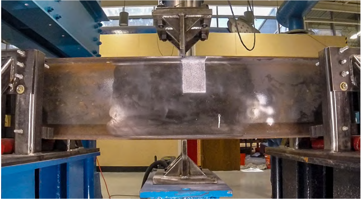
Figure A-71: Elevation of W16X31-DC-NA prior to testing
