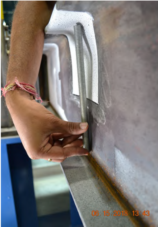
Figure A-19: W10X19-SC-NA after testing emphasizing web crippling
