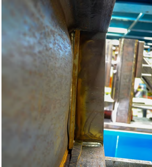
Figure 3.7-23: W12X26-DC-E2 after testing emphasizing web crippling
