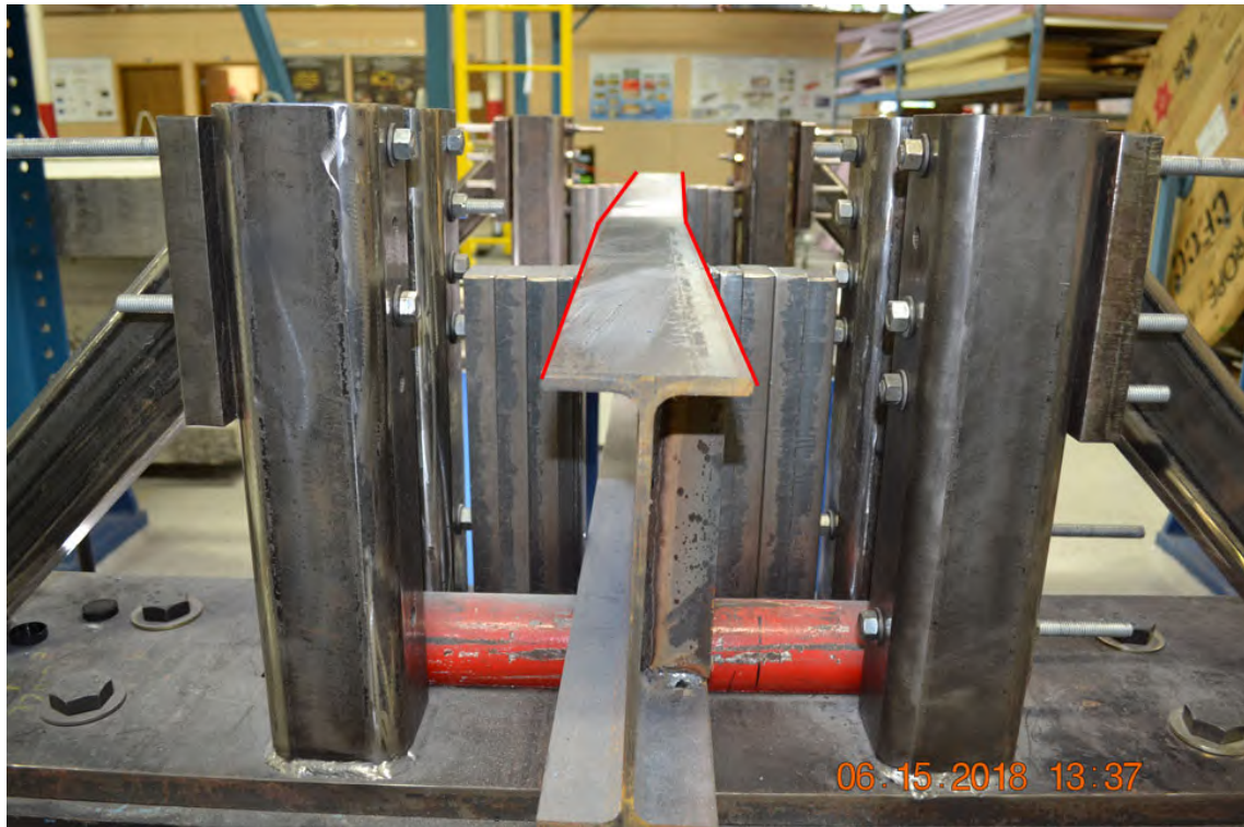
Figure A-21: Side view of W10X19-SC-NA after testing showing lateral torsional buckling
