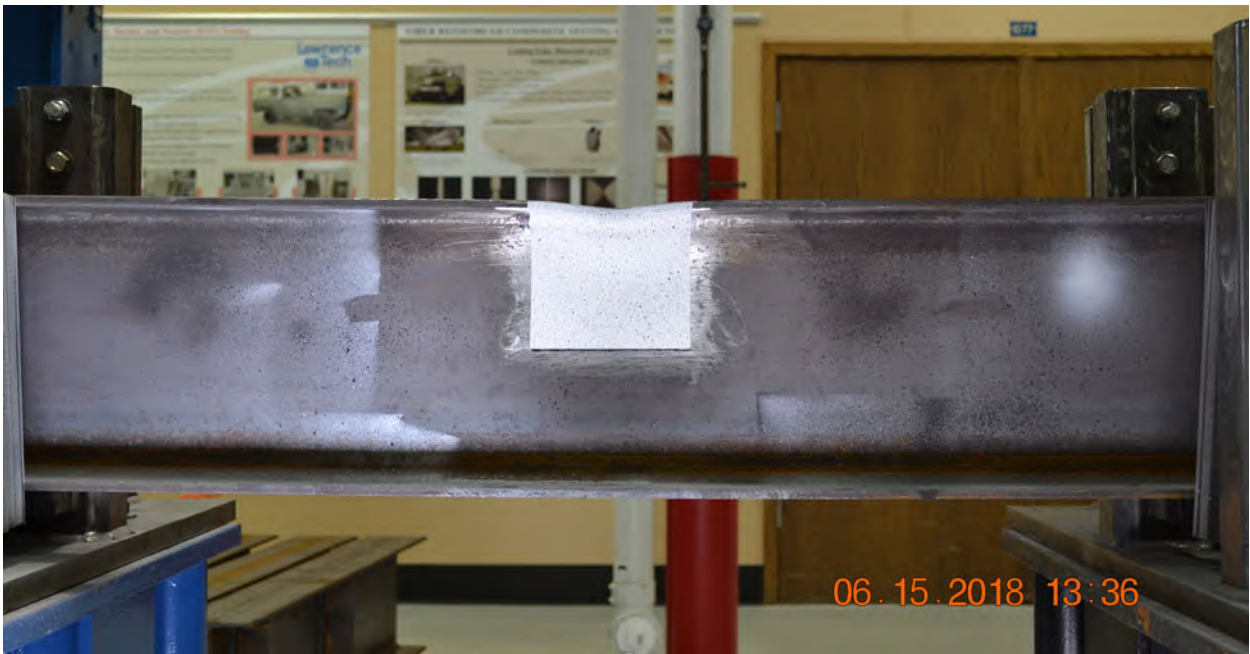
Figure A-18: Elevation of W10X19-SC-NA after testing
