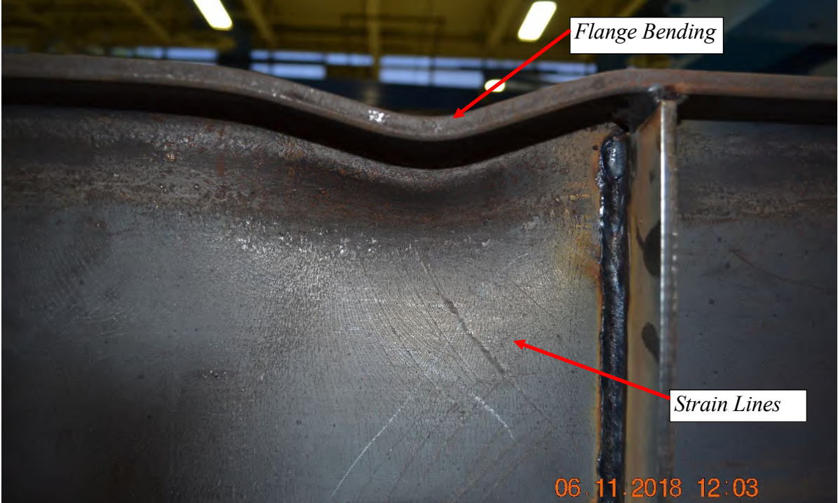
Figure 3.7-18: Close-up view of W10X19-DC-E4 after testing
