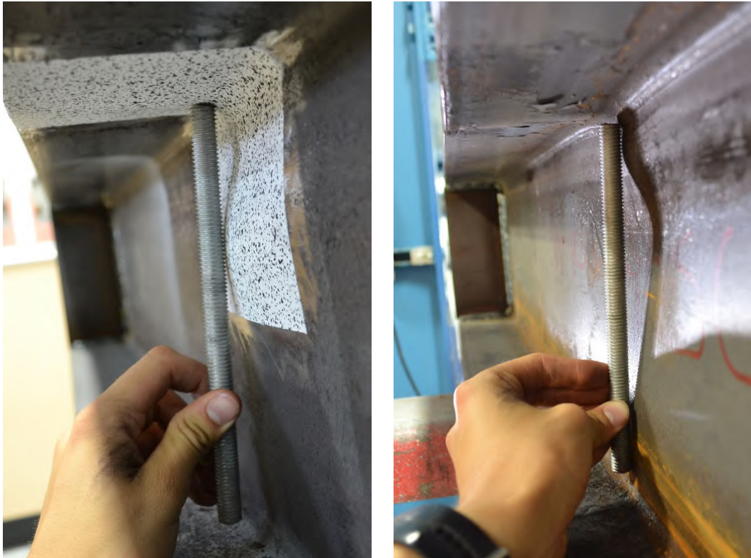
Figure 3.7-12: W10X39-SC-NA after testing emphasizing web crippling
