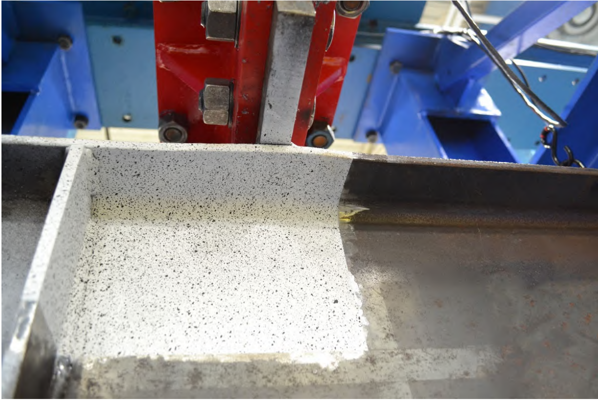
Figure A-129: Close-up view of W16X31-ST-E6 after testing from front side
