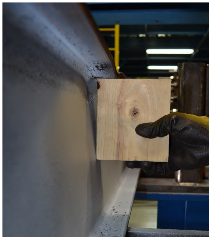
Figure A-91: W10X19-DC-NA after testing emphasizing web crippling
