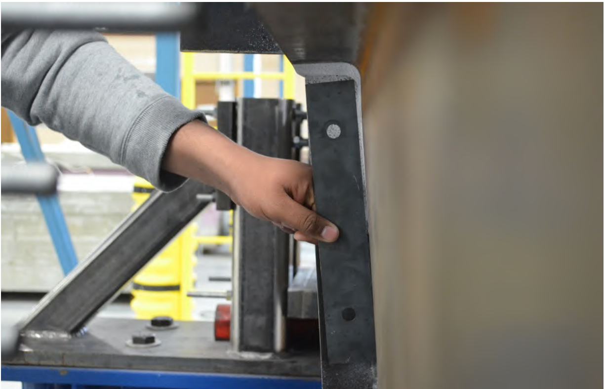
Figure A-83: W16X31-DC-E3 after testing emphasizing web crippling
