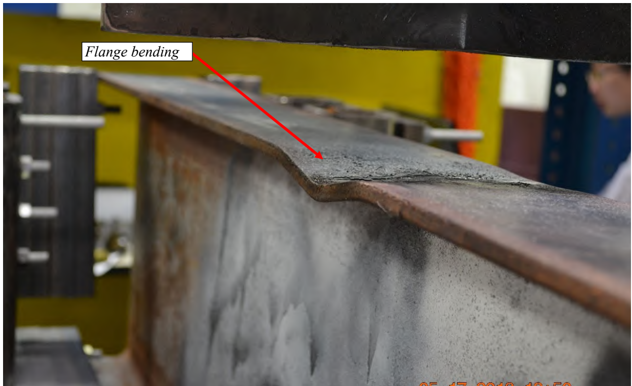
Figure A-87: Close-up of W16X31-DC-E0 emphasizing flange bending
