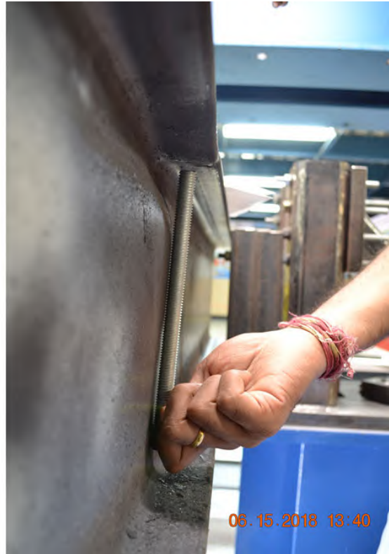
Figure A-19: W10X19-SC-NA after testing emphasizing web crippling
