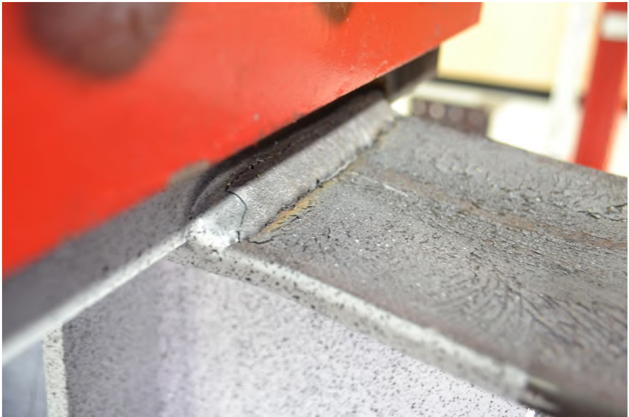
Figure A-171: Top weld condition of W12X26-ST-E2 after testing
