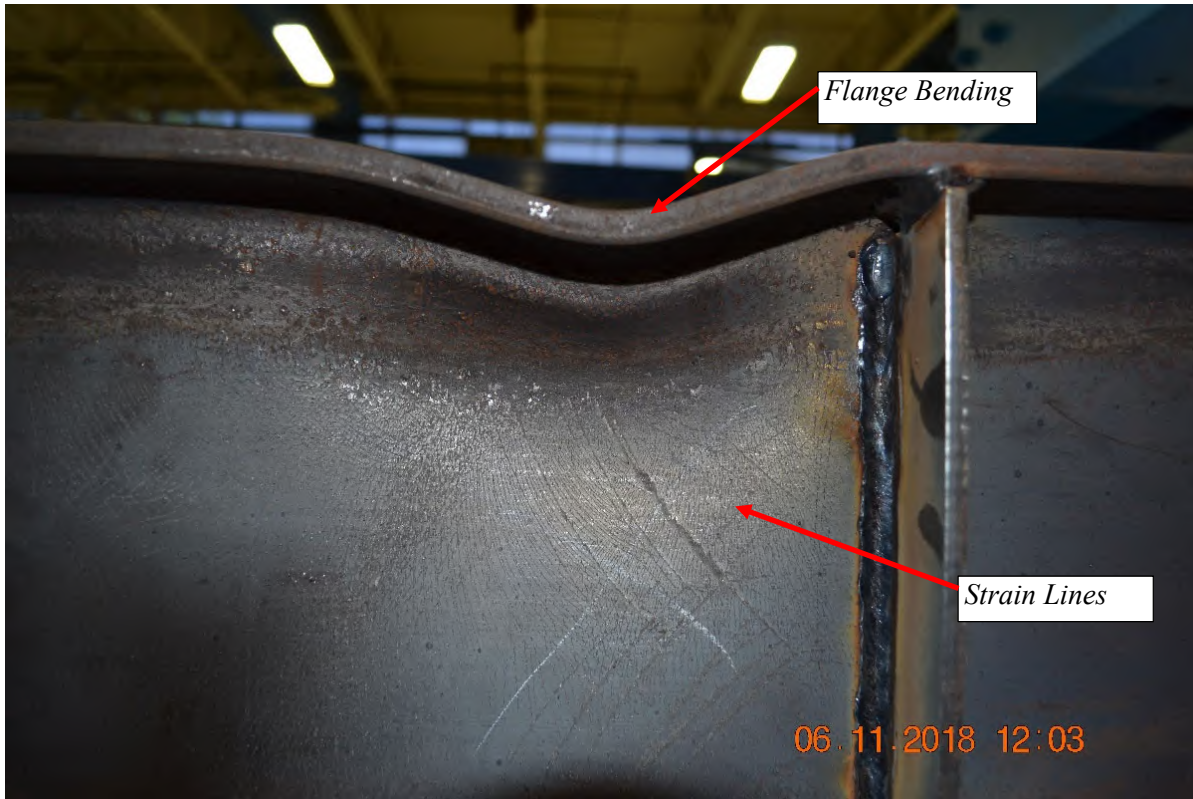
Figure A-95: Close-up view of W10X19-DC-E4 after testing
