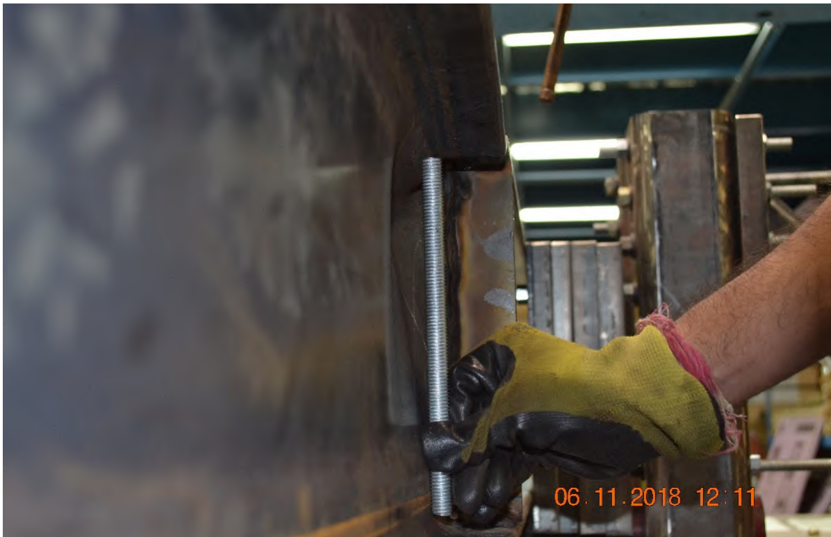
Figure A-96: W10X19-DC-E4 after testing emphasizing web crippling
