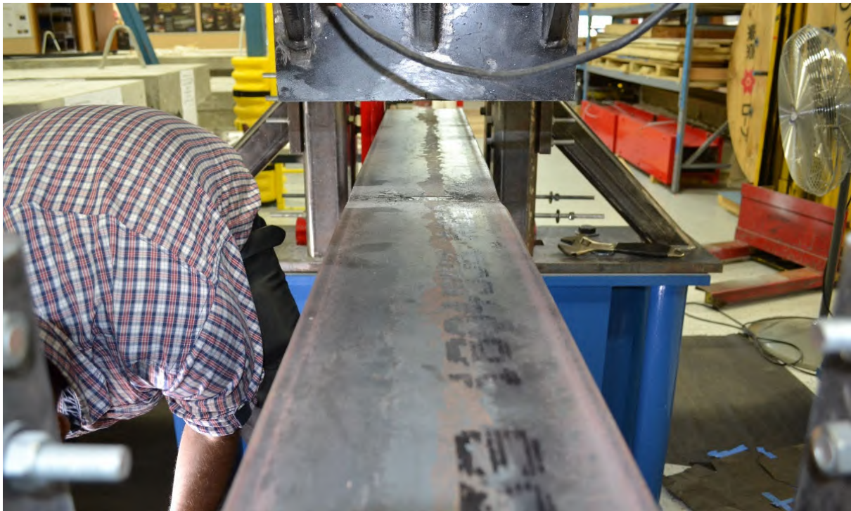
Figure A-40: Side view of W10X39-SC-NA after testing
