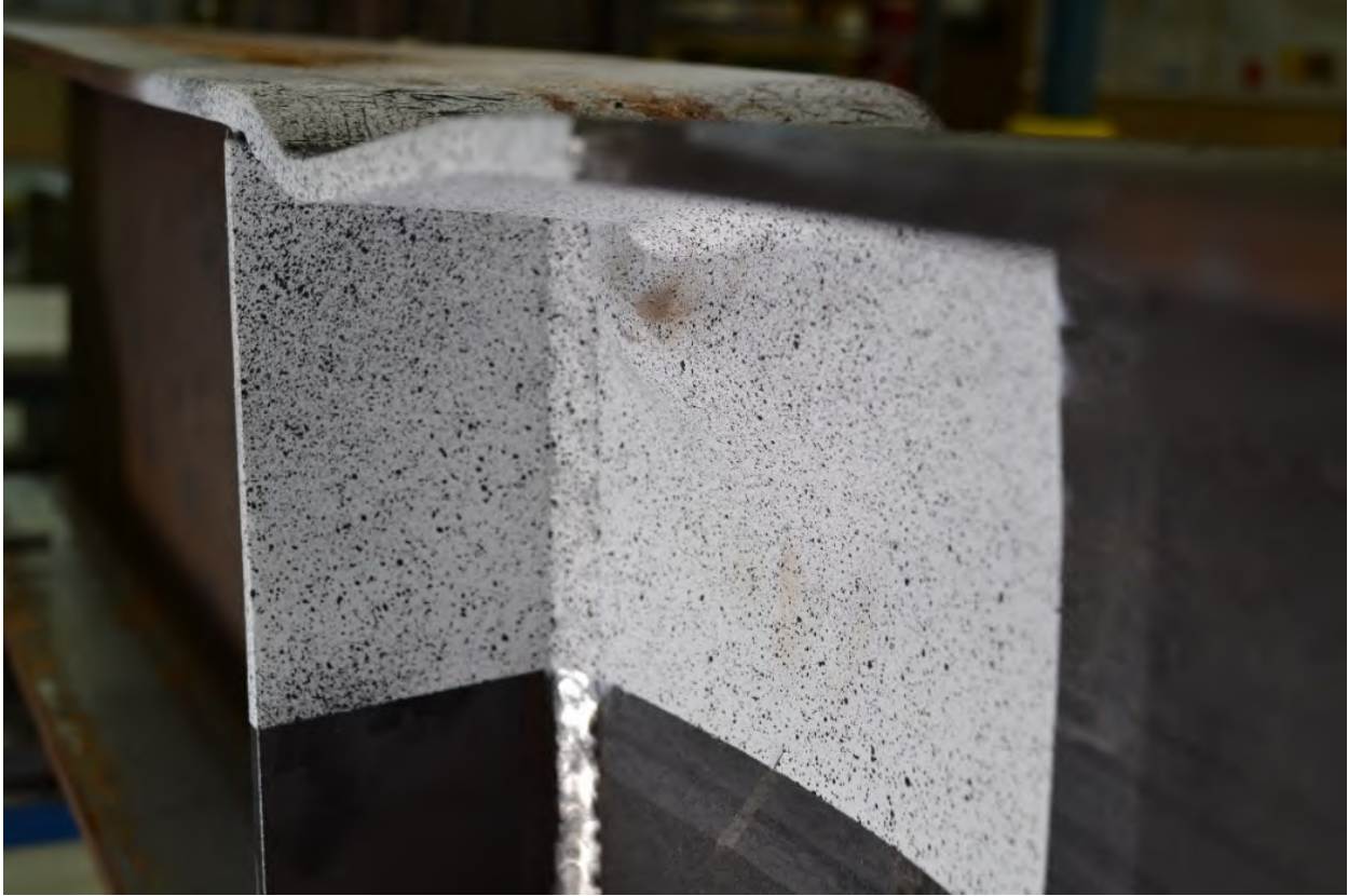
Figure A-119: W12X26-DC-E2 after testing further showing deformations near top flange
