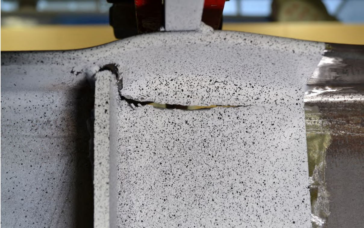
Figure A-170: W12X26-ST-E2 after testing emphasizing web fracture
