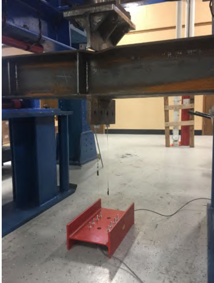
Figure 4.6-1: String pots attached to column specimen for measuring elastic displacement
