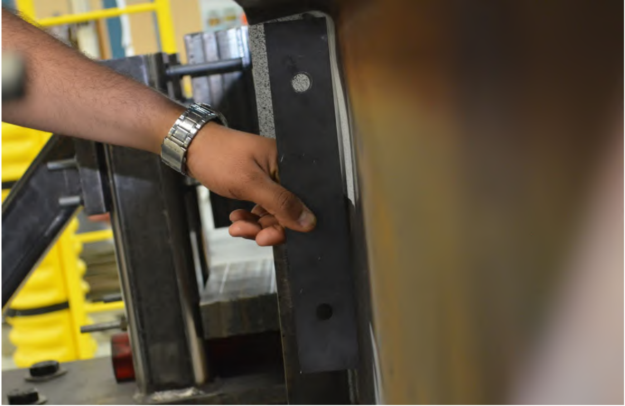
Figure A-7: W16X31-SC-E6 after testing emphasizing web local crippling
