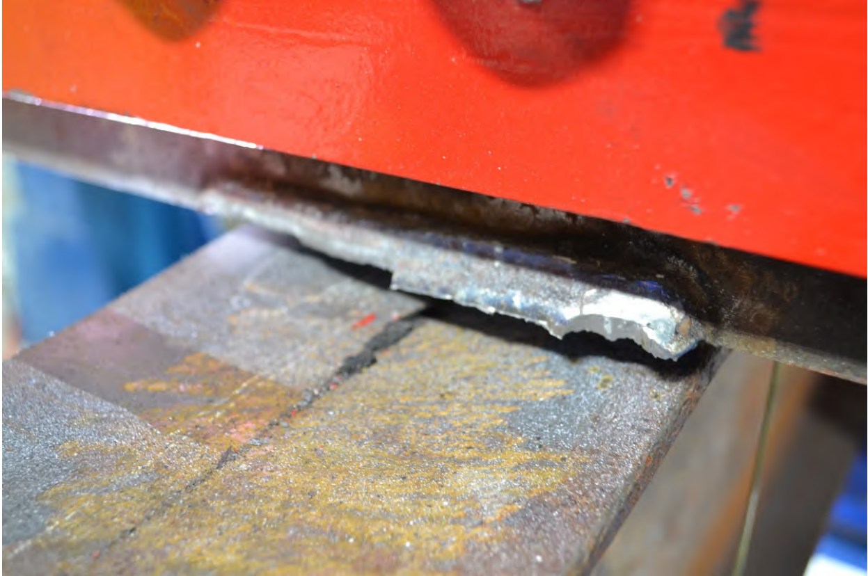
Figure A-127: Weld fracture of W16X31-ST-NA after testing (Side 2)
