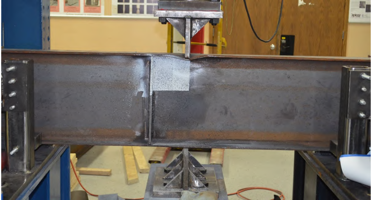
Figure A-76: Elevation of W16X31-DC-E6 after testing
