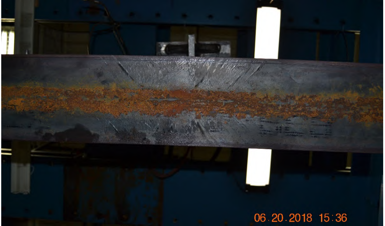
Figure A-70: Bottom view of W12X26-SC-E0 after testing emphasizing yielding
