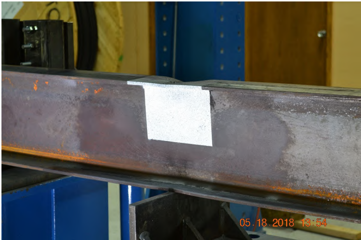
Figure A-89: Elevation of W10X19-DC-NA after testing
