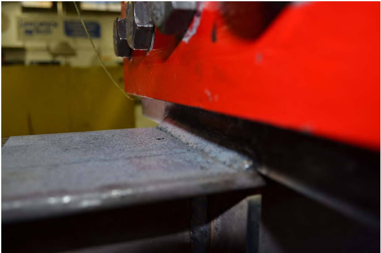
Figure A-175: Weld condition of W12X26-ST-E0 after testing (Side 2)
