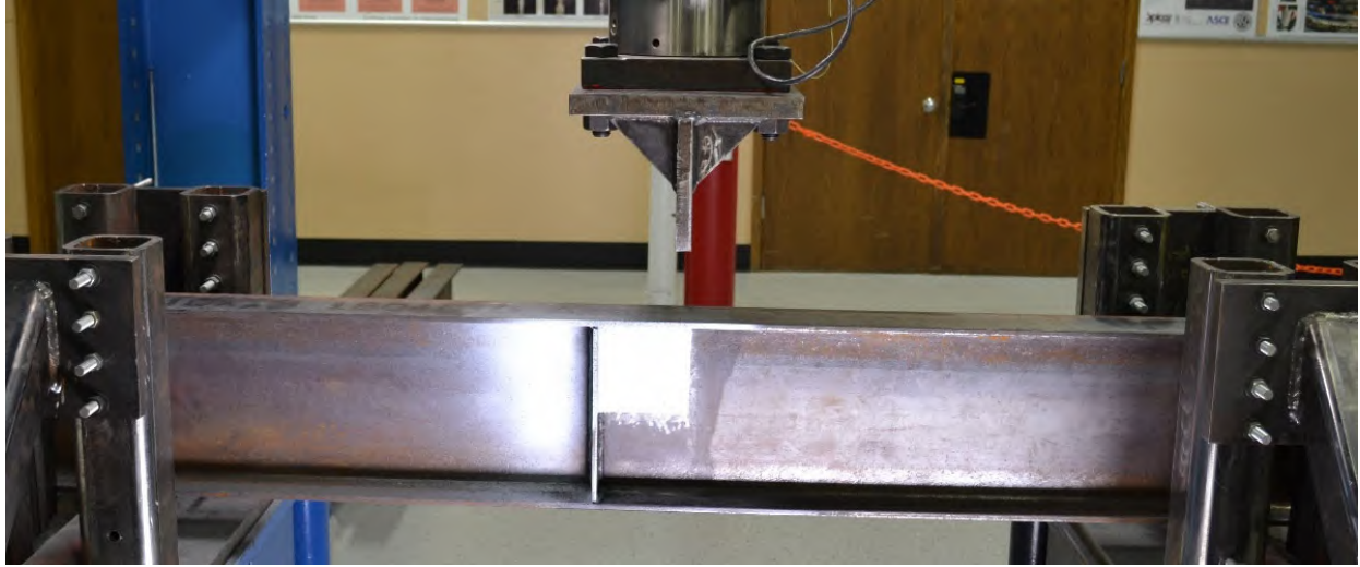
Figure A-22: Elevation of W10X19-SC-E4 prior to testing
