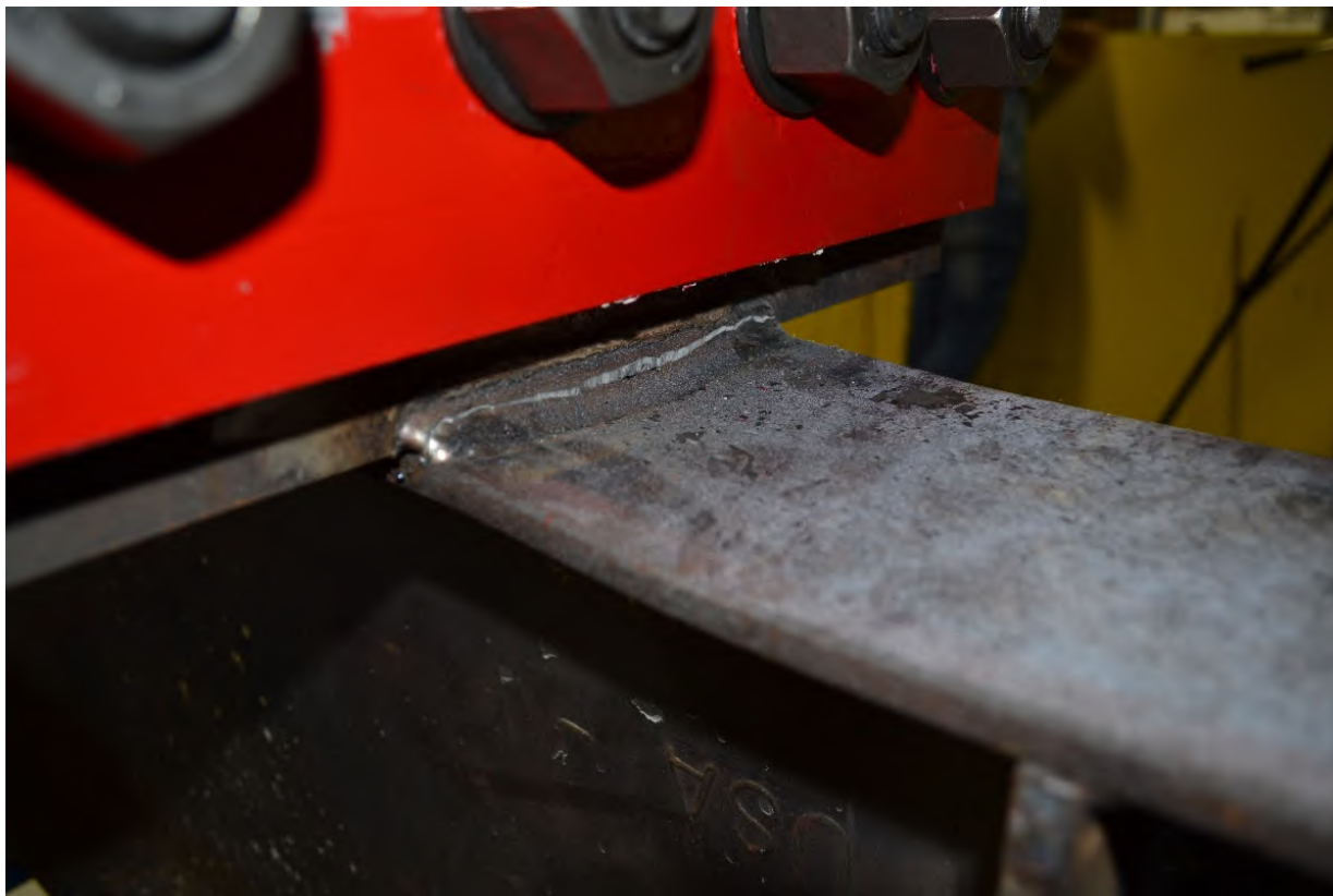
Figure A-132: Weld fracture of W16X31-ST-E6 after testing (Side 2)
