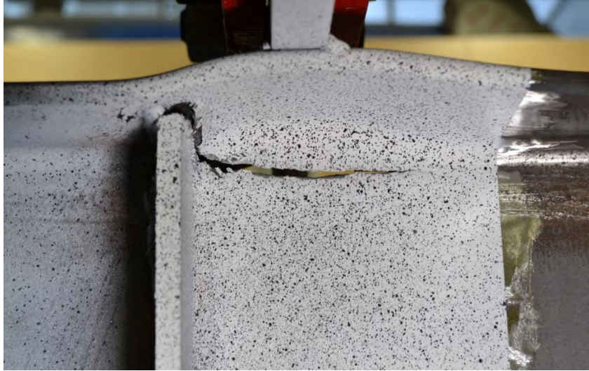
Figure 3.7-29: W12X26-ST-E2 after testing emphasizing web fracture
