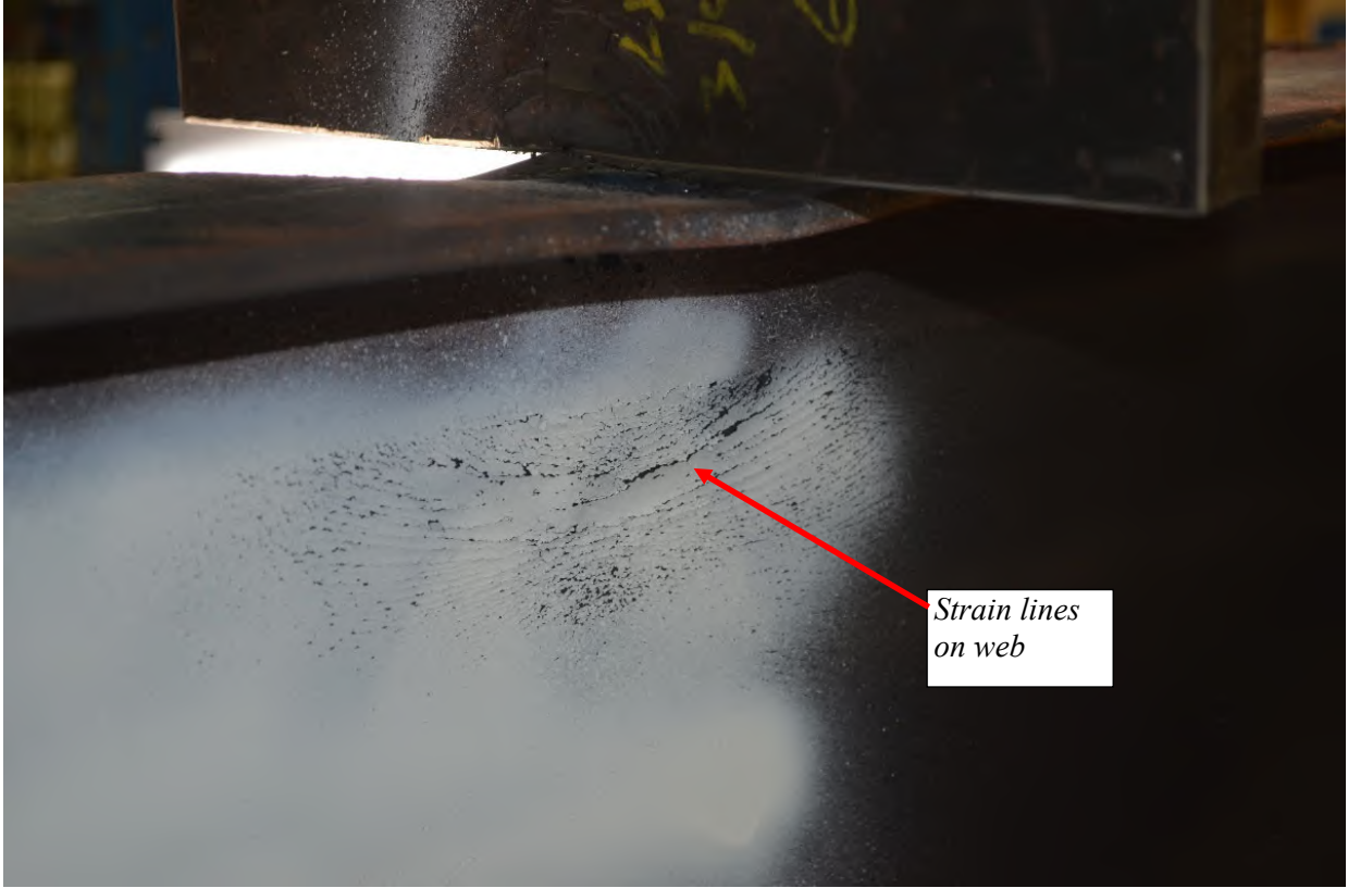
Figure A-75: W16X31-DC-NA after testing emphasizing web local yielding
