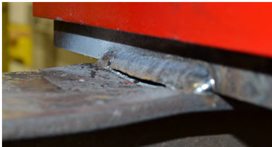
Figure 3.7-27: Weld fracture of W16X31-ST-E6 after testing
