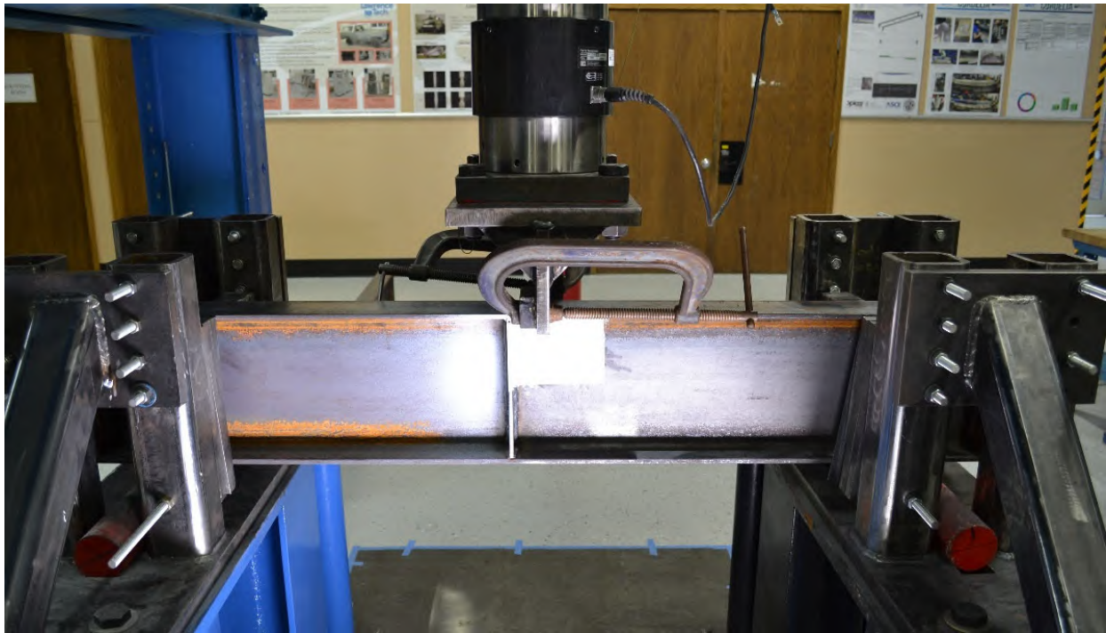
Figure A-27: Elevation of W10X19-SC-E2 prior to testing
