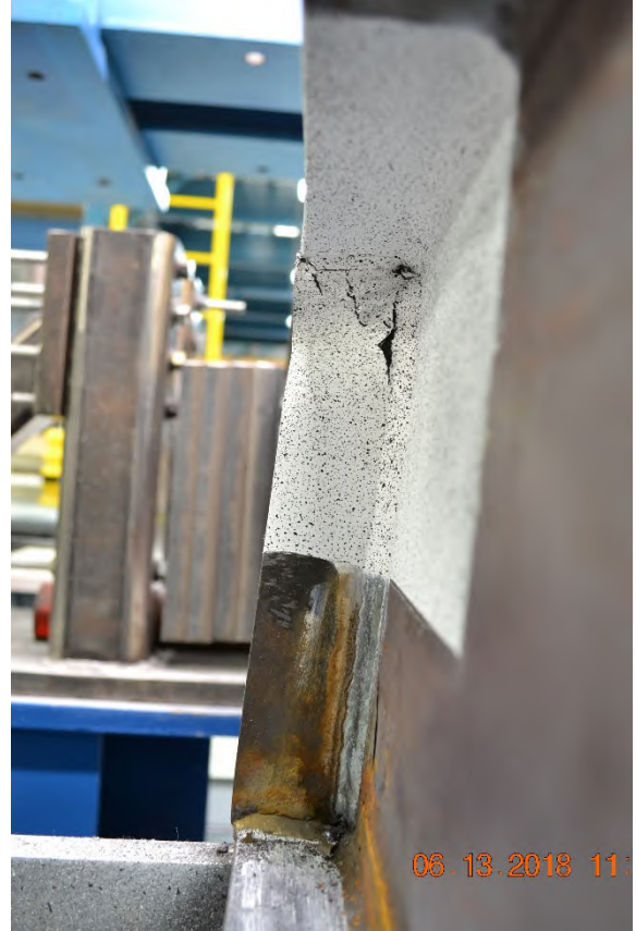
Figure A-107: Side view of W10X19-SC-E0 after testing showing the stiffener conditions
