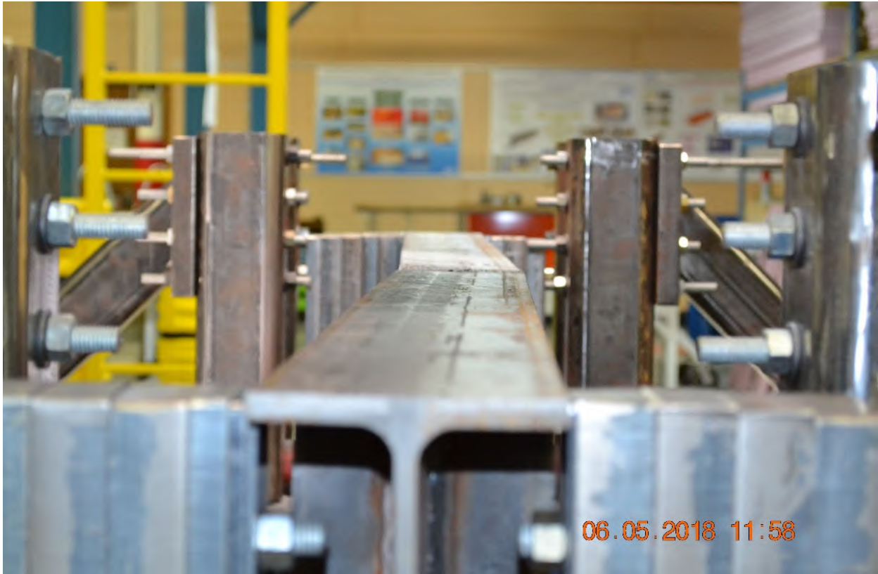
Figure A-26: Side view of W10X19-SC-E4 after testing showing lateral-torsional buckling
