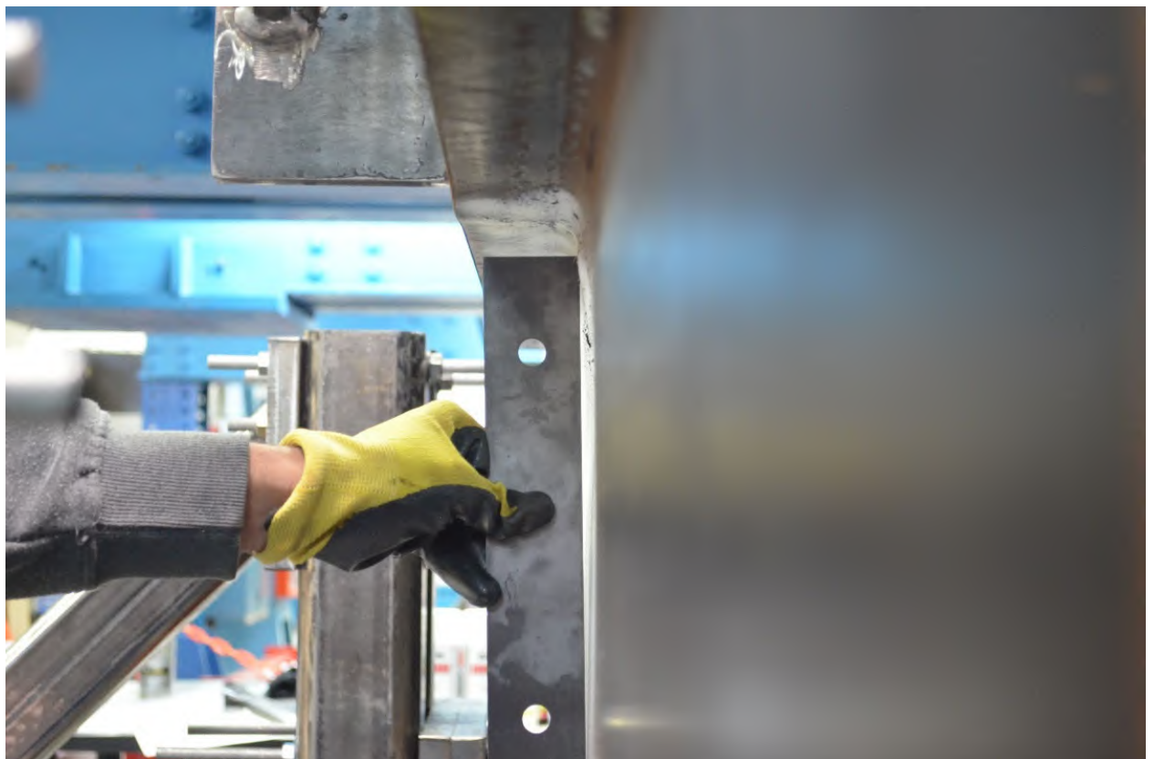
Figure A-74: W16X31-DC-NA after testing emphasizing web crippling
