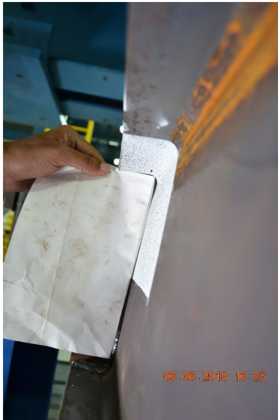
Figure A-30: W10X19-SC-E2 after testing emphasizing web crippling
