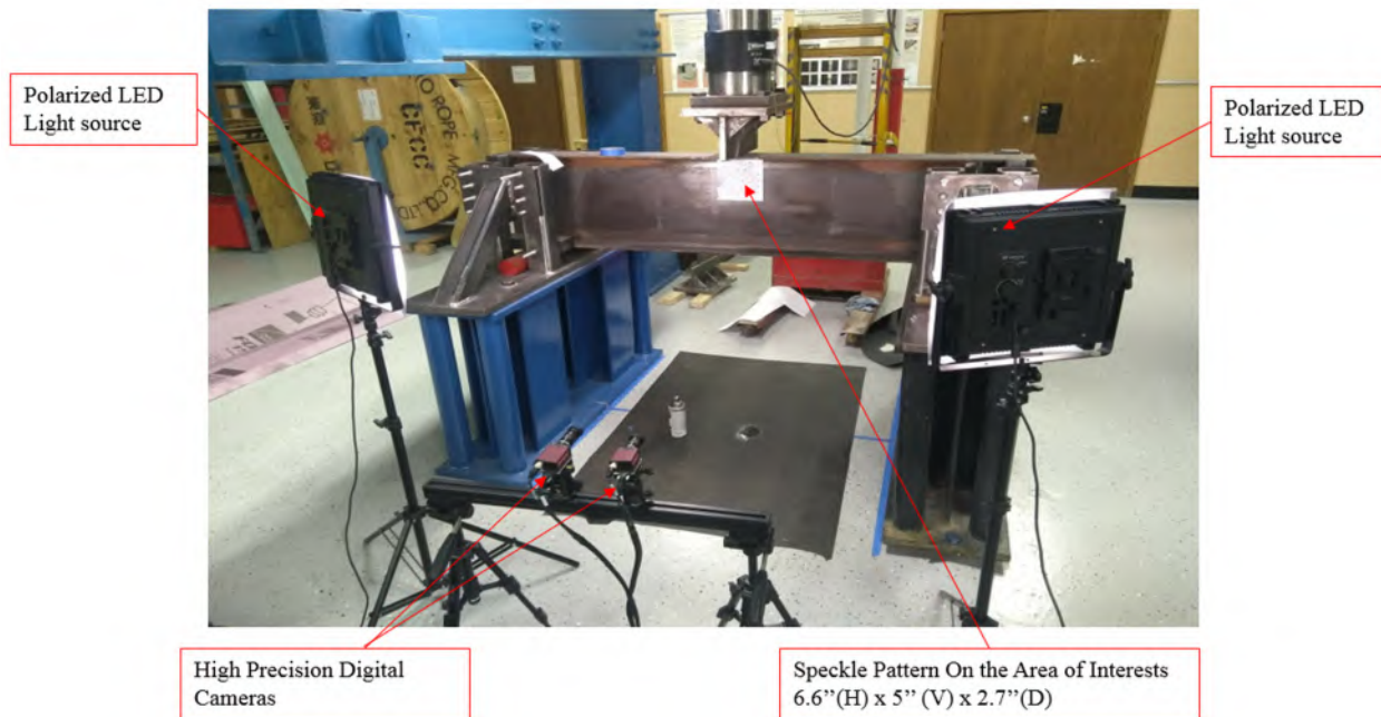
Figure 3.5-16: Test setup for DIC Instrumentation
