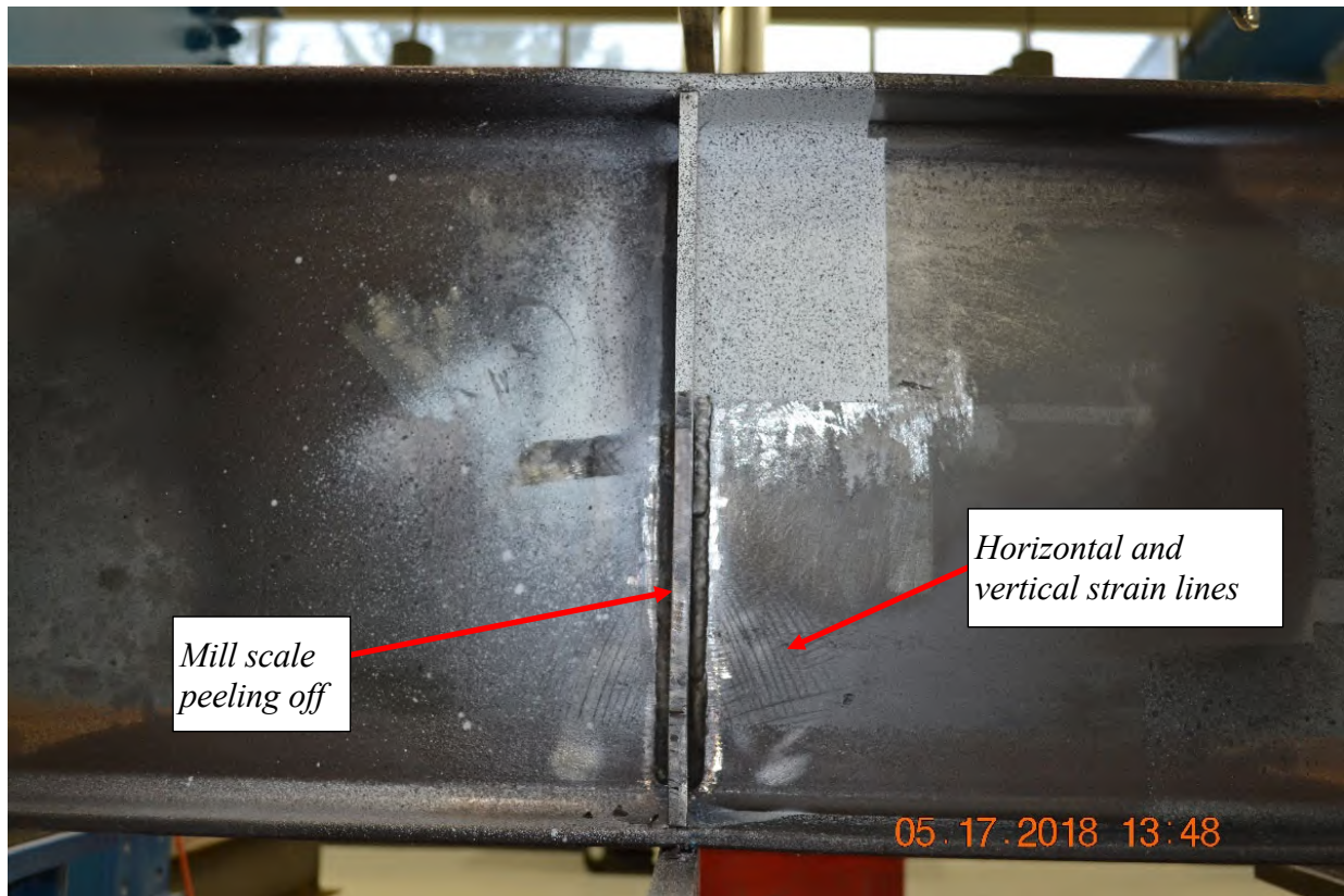
Figure 3.7-16: Elevation of W16X31-DC-E0 after testing
