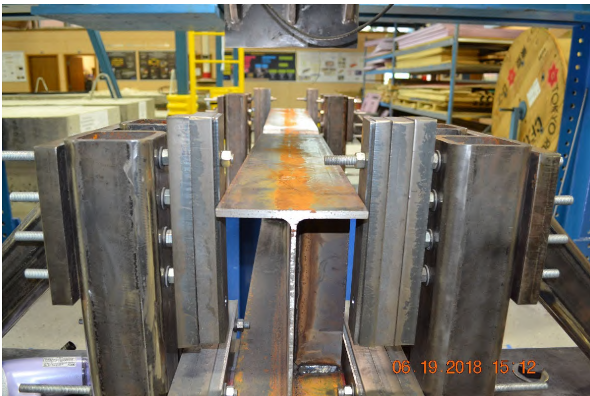
Figure A-57: Side view of W12X26-SC-NA after testing
