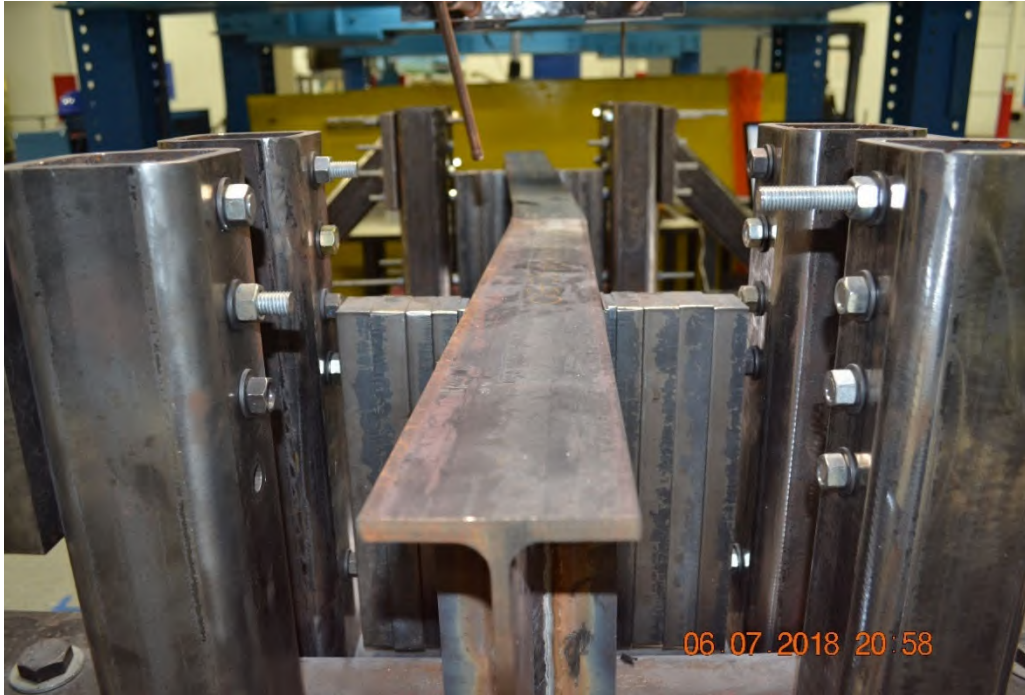
Figure 3.7-7: Side view of W10X19-SC-E0 after testing showing lateral-torsional buckling
