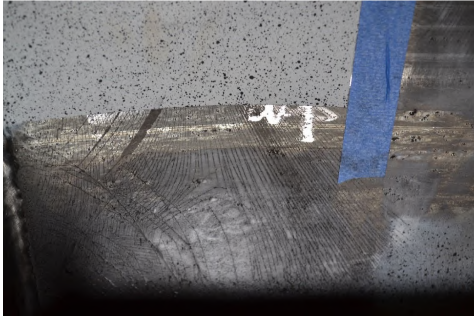
Figure A-117: Close-up view of W12X26-DC-E2 emphasizing the strain lines
