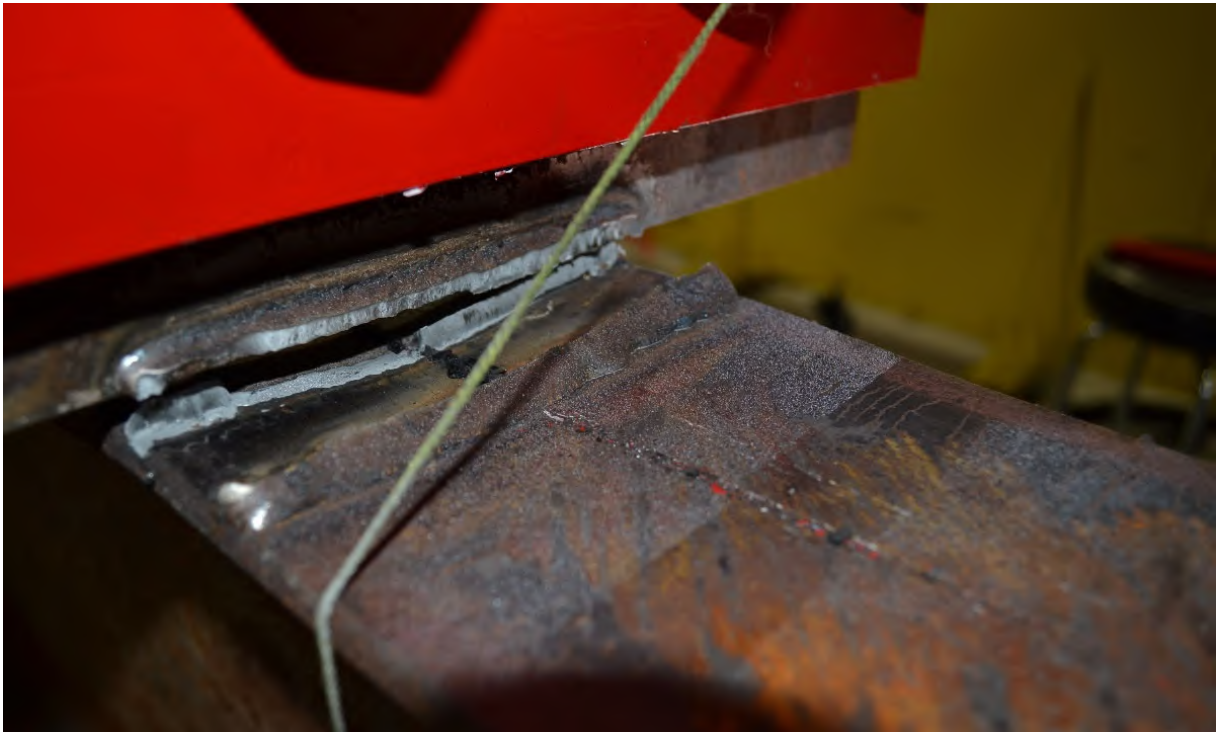
Figure A-126: Weld fracture of W16X31-ST-NA after testing (Side 1)
