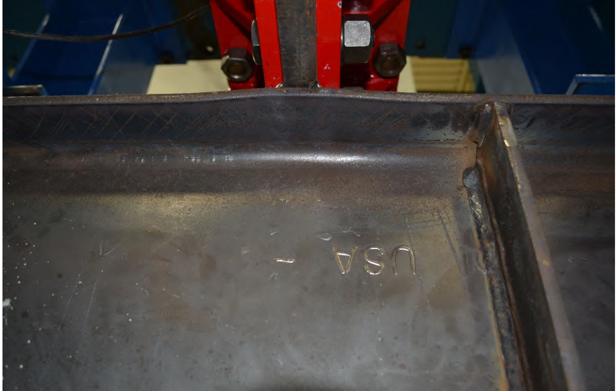
Figure A-130: Close-up view of W16X31-ST-E6 after testing from back side
