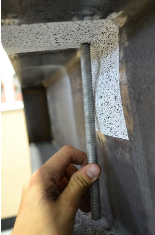
Figure A-39: W10X39-SC-NA after testing emphasizing web crippling
