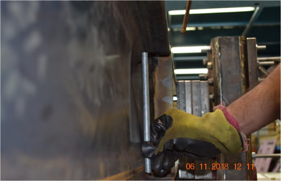
Figure 3.7-19: W10X19-DC-E4 after testing emphasizing web crippling
