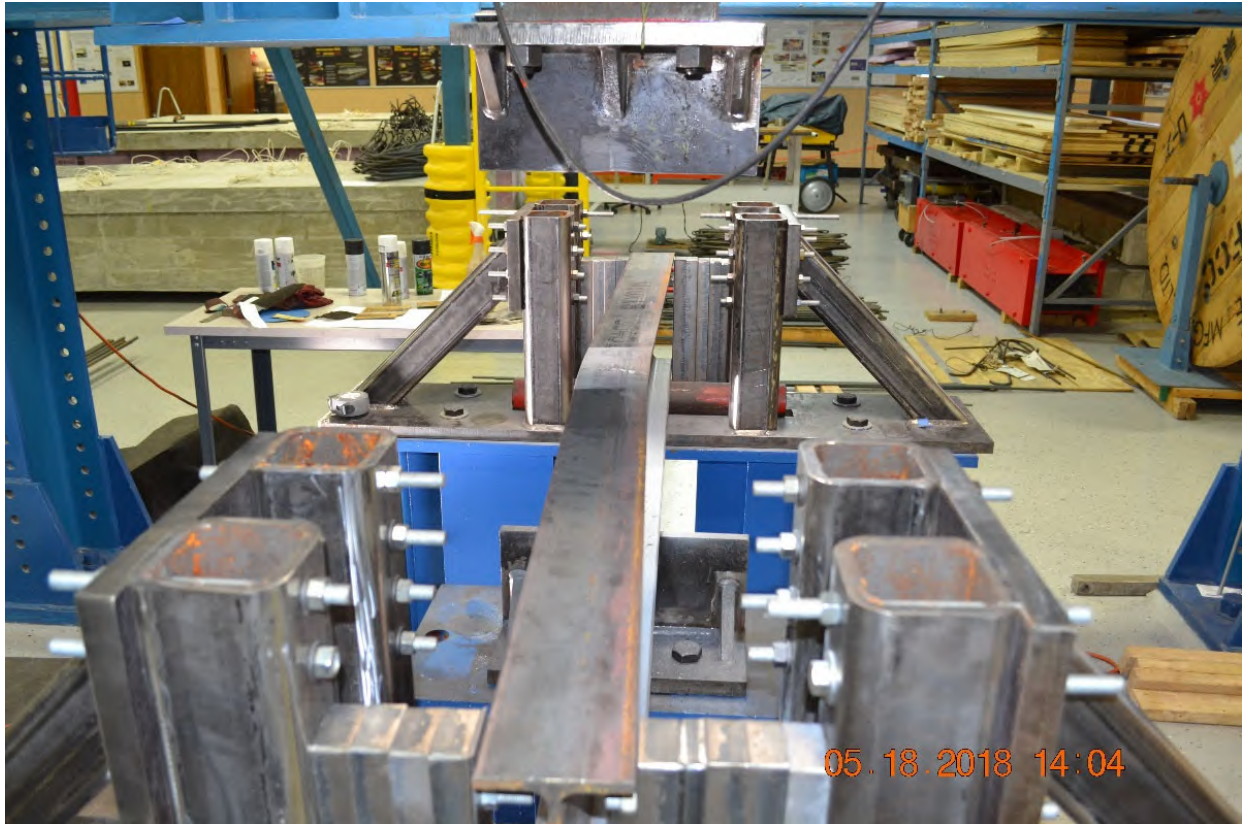
Figure A-92: Side view of W10X19-DC-NA after testing showing lateral translation
