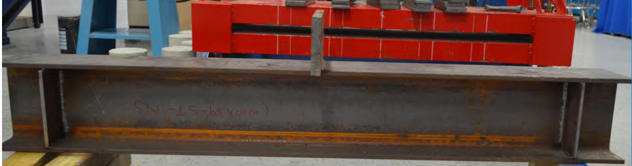
Figure 3.3-1: Photograph of W10X39-ST-NA (no stiffeners at midspan) prior to testing
