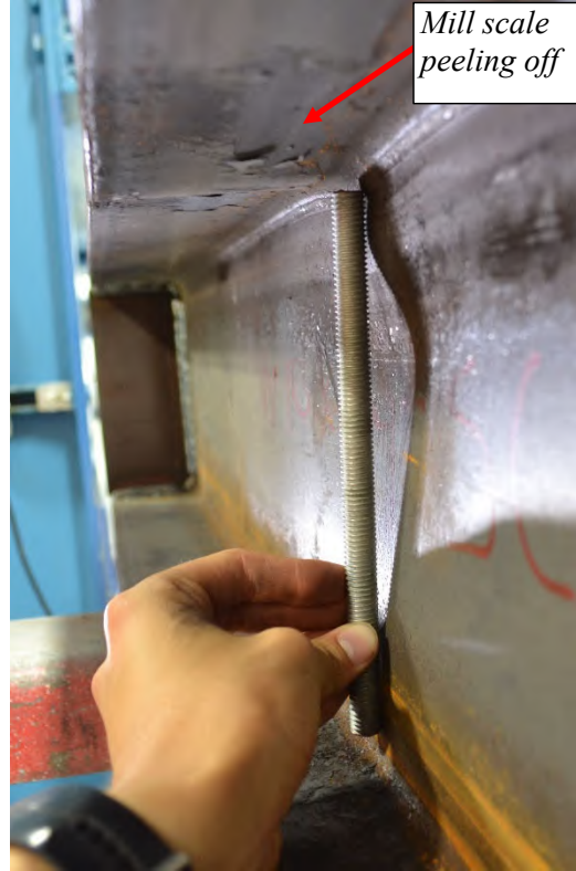
Figure A-39: W10X39-SC-NA after testing emphasizing web crippling
