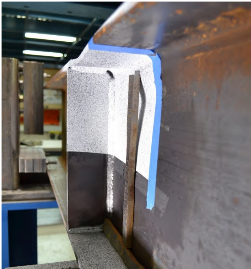
Figure A-114: Side view of W12X26-DC-E4 after testing emphasizing web local crippling
