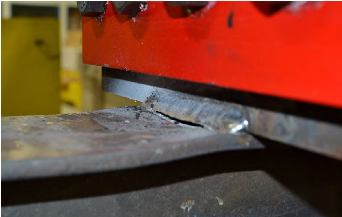
Figure A-131: Weld fracture of W16X31-ST-E6 after testing (Side 1)
