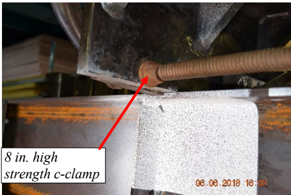
Figure 3.7-8: Method used to brace W10x19 specimens against lateral-torsional buckling
