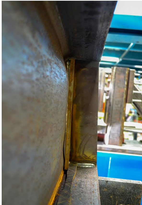
Figure A-118: W12X26-DC-E2 after testing emphasizing web crippling
