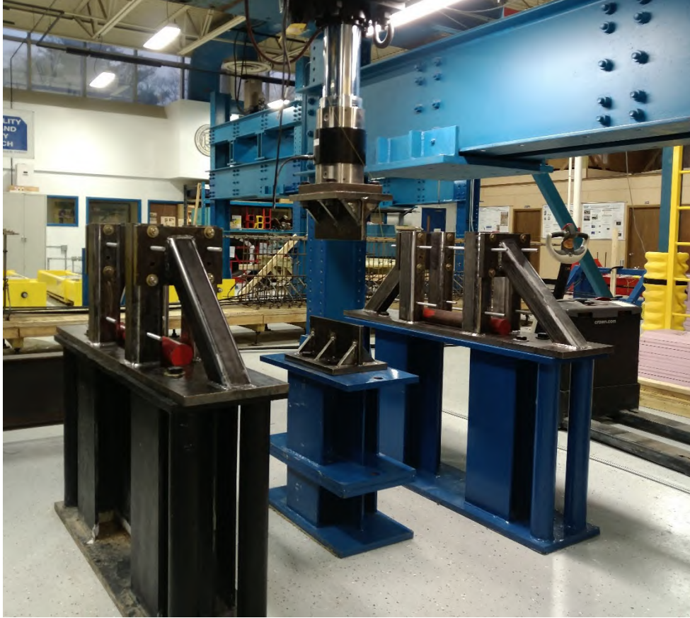
Figure 3.5-1: Photograph of test frame and 220 kip actuator in the STC
