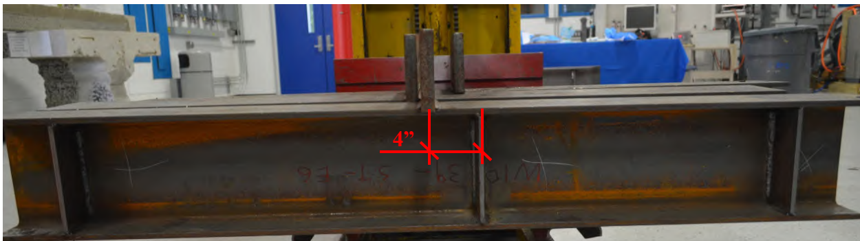
Figure 3.3-4: Photograph of W10X39-ST-E4 (eccentricity = 4 in.) prior to testing
