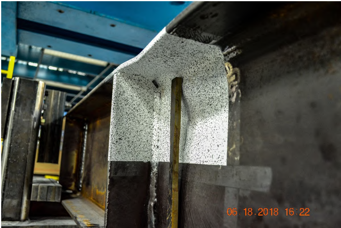
Figure A-61: W12X26-SC-E4 after testing emphasizing web local crippling
