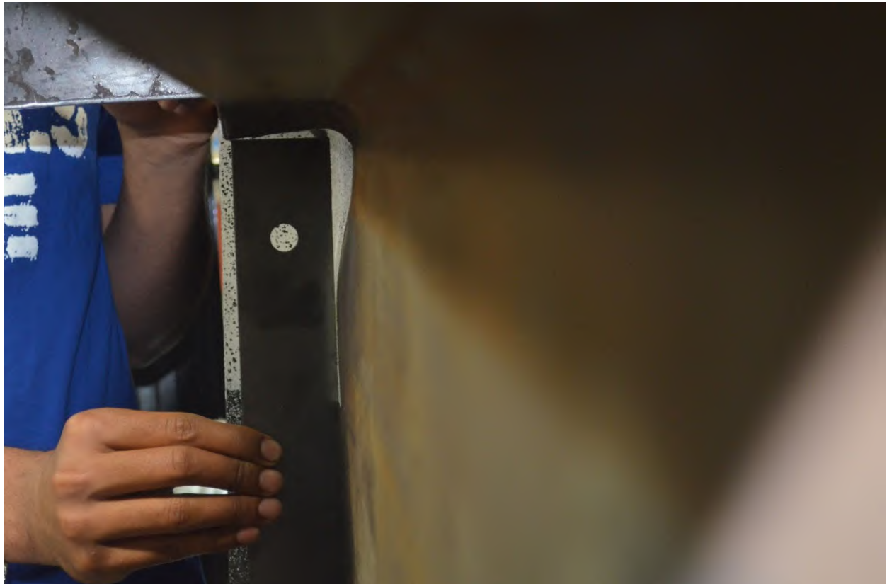
Figure A-79: W16X31-DC-E6 after testing emphasizing web local crippling
