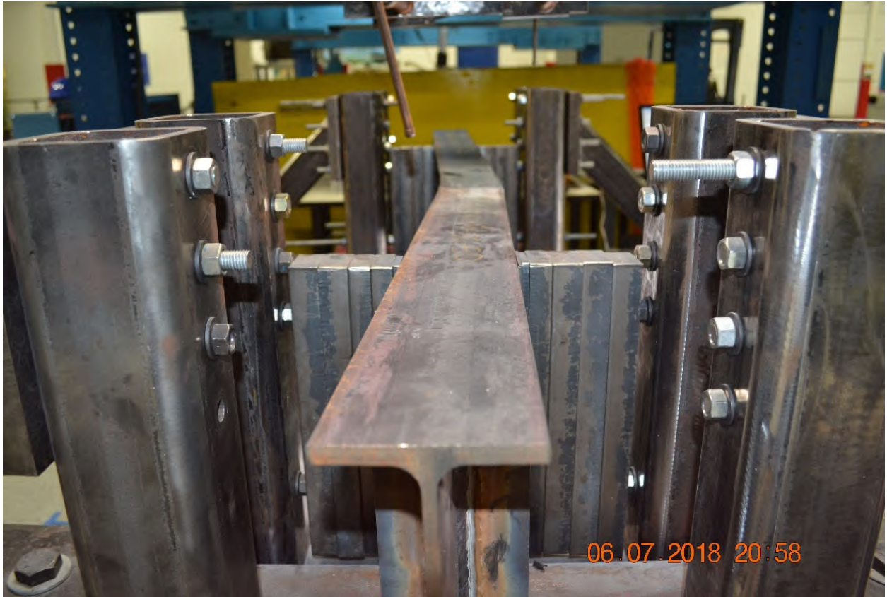
Figure A-36: Side view of W10X19-SC-E0 after testing showing lateral-torsional buckling
