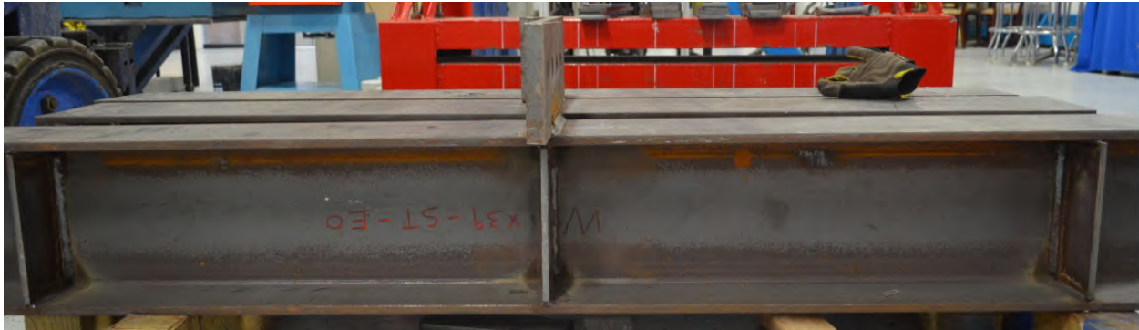
Figure 3.3-2: Photograph of W10X39-ST-E0 (no eccentricity) prior to testing
