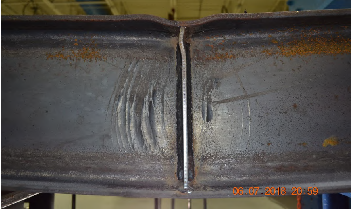
Figure A-34: Close-up view of backside W10X19-SC-E0 after testing
