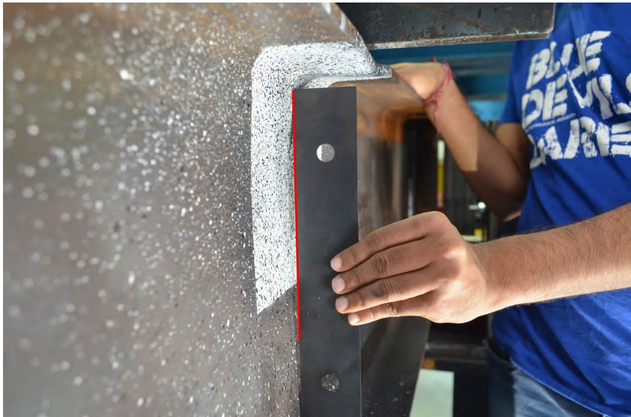
Figure A-4: W16X31-SC-NA after testing emphasizing web crippling
