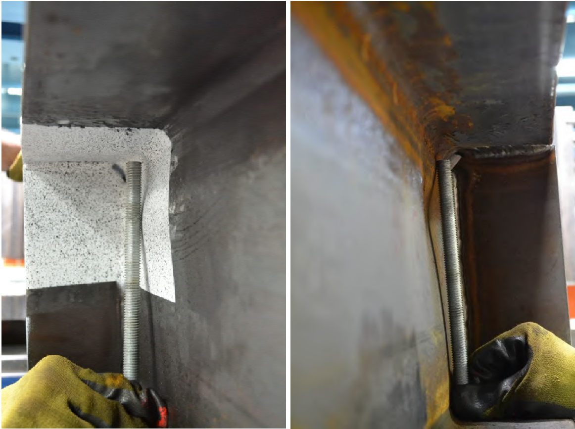
Figure A-44: W10X39-SC-E4 after testing emphasizing web crippling
