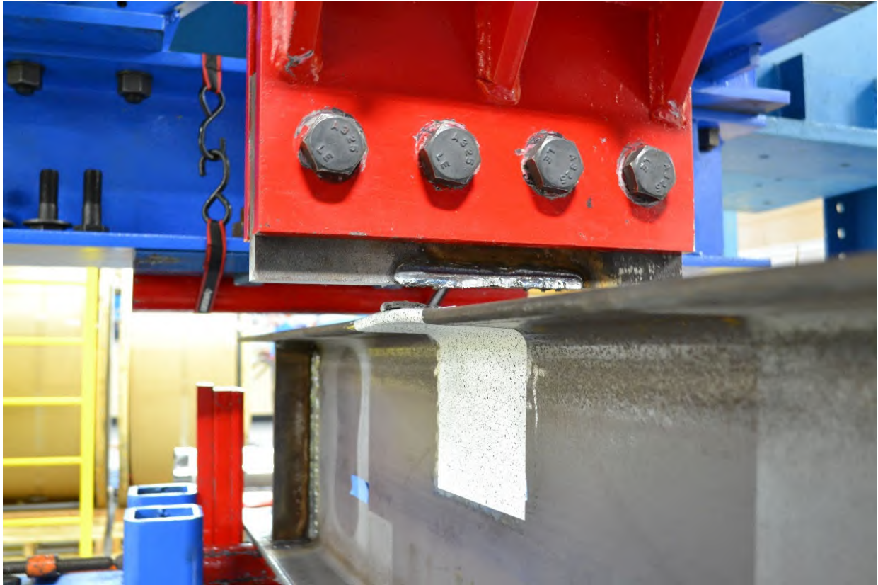
Figure A-161: Side view of W12X26-ST-NA after testing emphasizing flange bending
