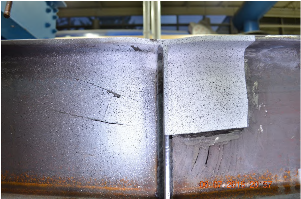
Figure A-33: Close-up elevation of W10X19-SC-E0 after testing
