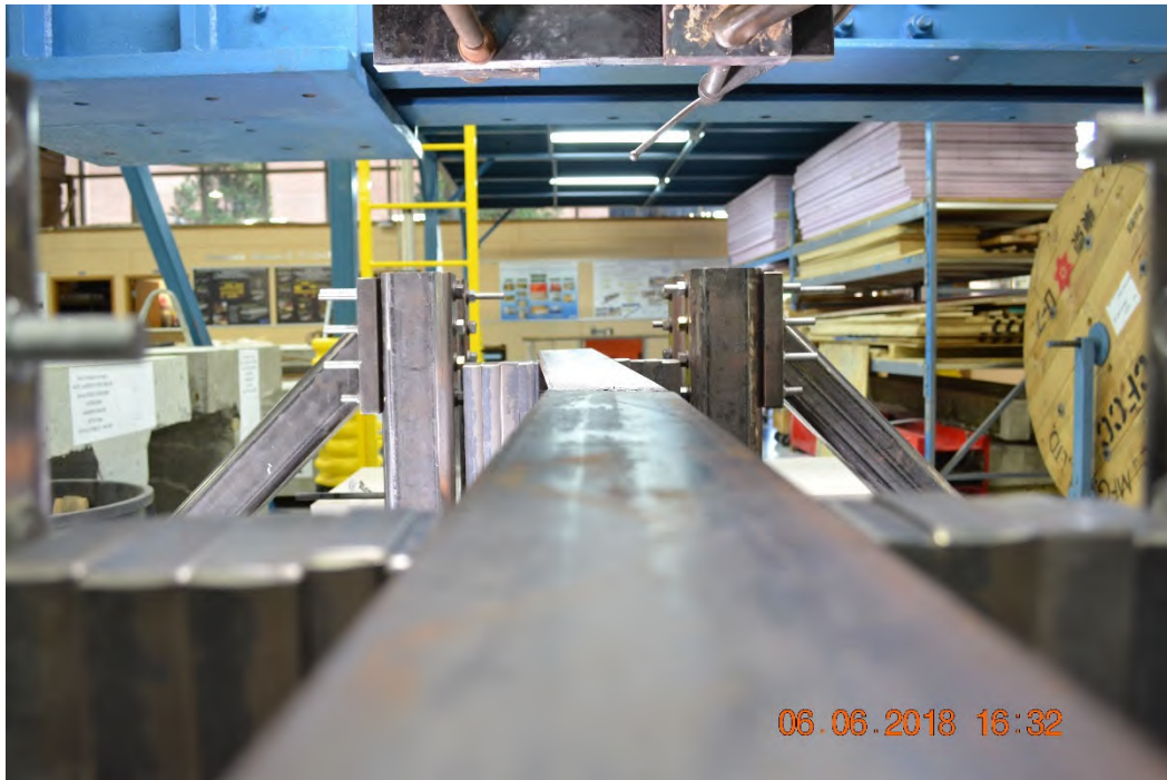
Figure A-31: Side view of W10X19-SC-E2 after testing showing lateral-torsional buckling
