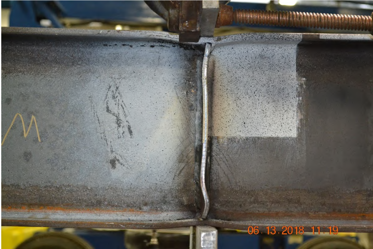
Figure A-105: Back view of W10X19-SC-E0 after testing
