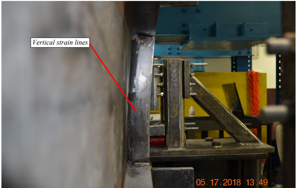
Figure A-86: Side view of W16X31-DC-E0 after testing
