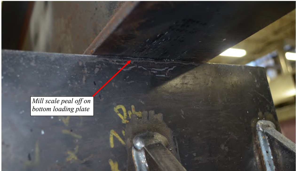
Figure A-78: Condition of bottom loading plate after testing
