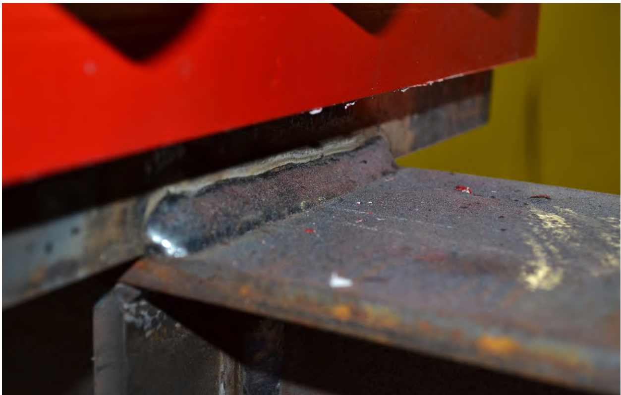
Figure A-141: Weld condition of W16X31-ST-E0 after testing (Side 2)
