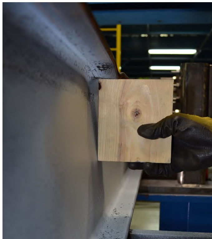
Figure 5.2-4: W10X19-DC-NA after testing emphasizing web crippling
