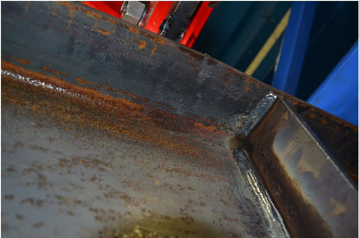
Figure A-166: W12X26-ST-E4 after testing emphasizing flange yielding
