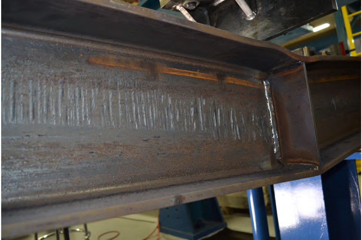
Figure A-53: Side view of W10X39-SC-E0 after testing showing web strain lines
