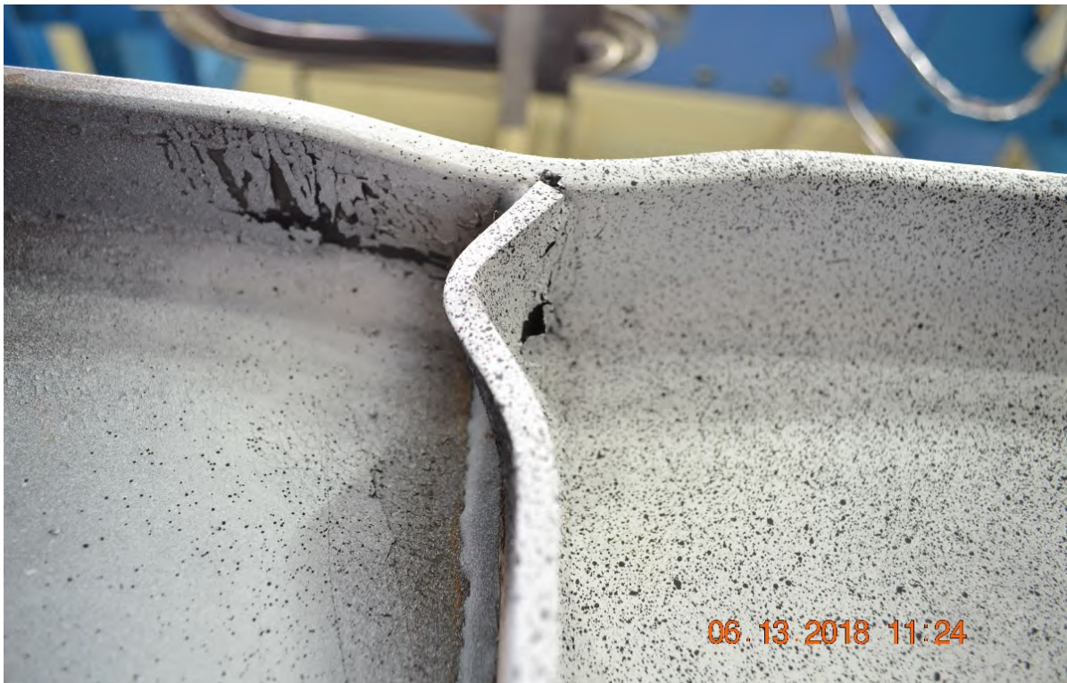
Figure A-106: W10X19-SC-E0 after testing emphasizing stiffener buckling
