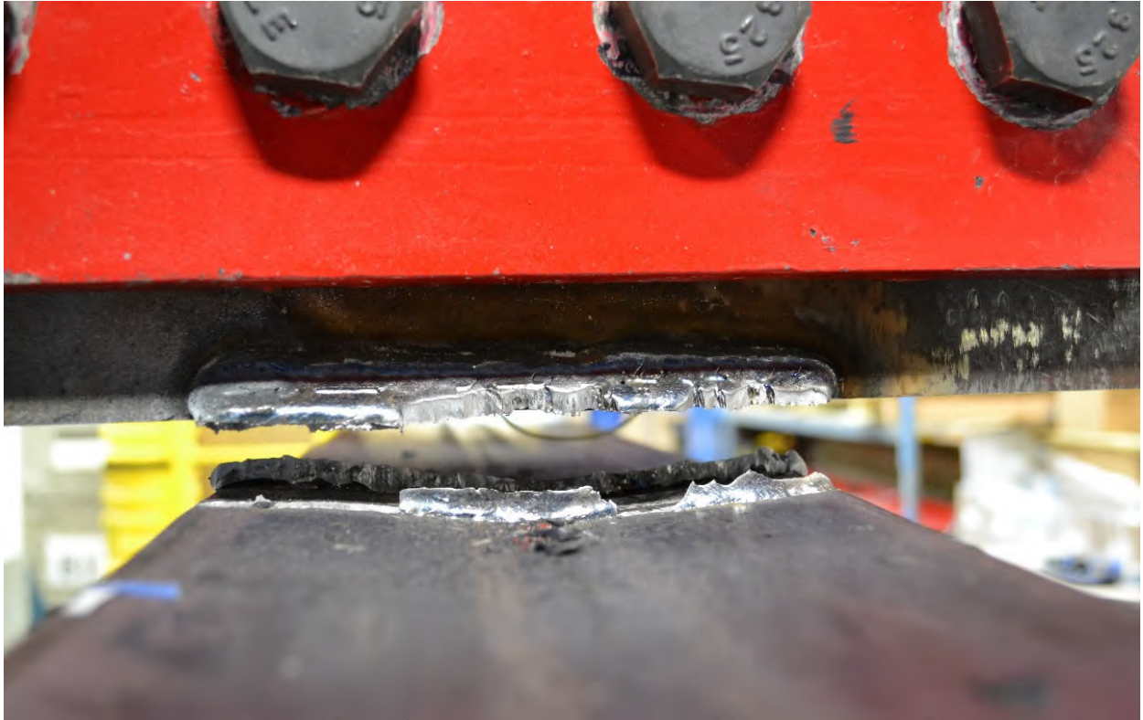
Figure A-162: Weld fracture of W12X26-ST-NA
