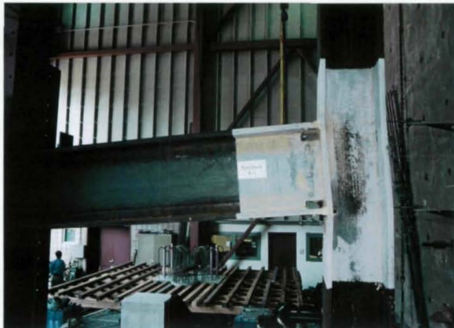
Figure 3.3 Specimen K1: Deformed Configuration at 10 in. Beam Deflection
