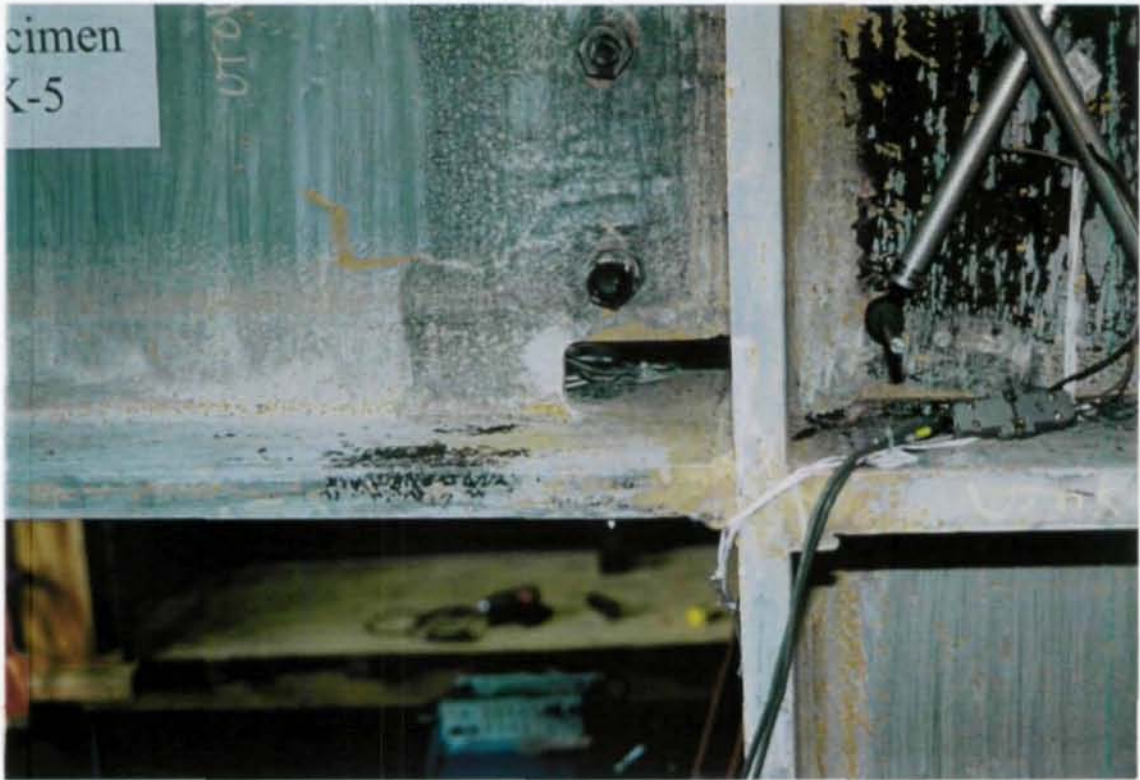
Figure 4.10 Specimen K5: Yielding in Panel Zone and Beam Flange at 3% Drift
