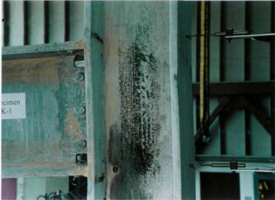
(a) Panel Zone Yielding and Column Kinking
