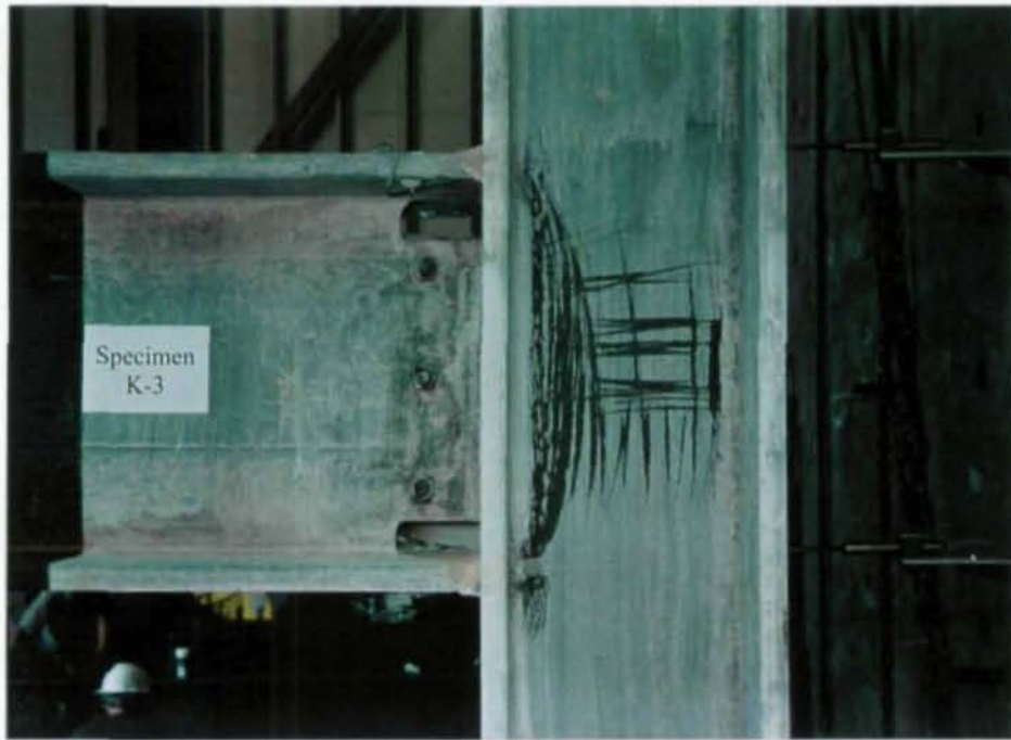
Figure 3.24 Specimen K3: Panel Zone Yielding Pattern at 1% Drift
