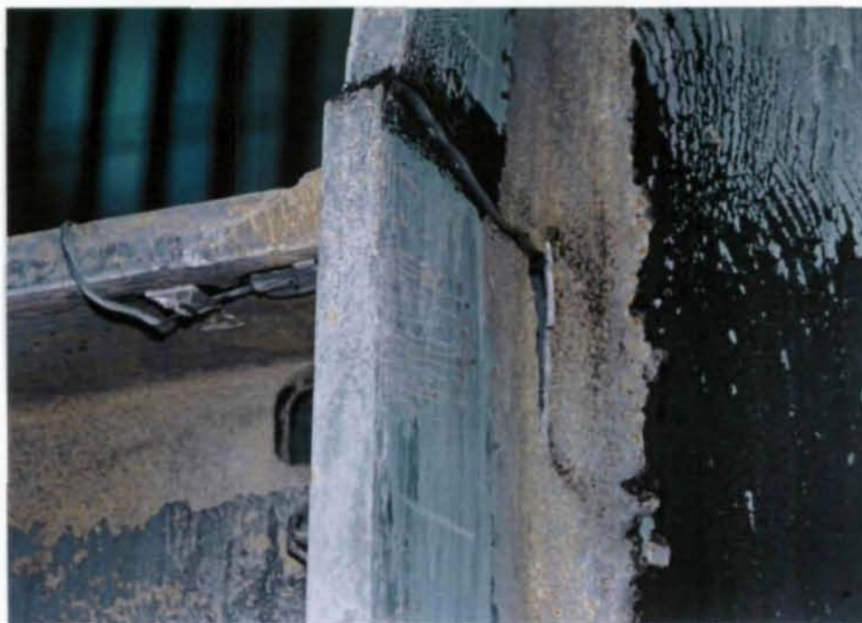
(b) Propagation of Fracture into Column Web near k Area
