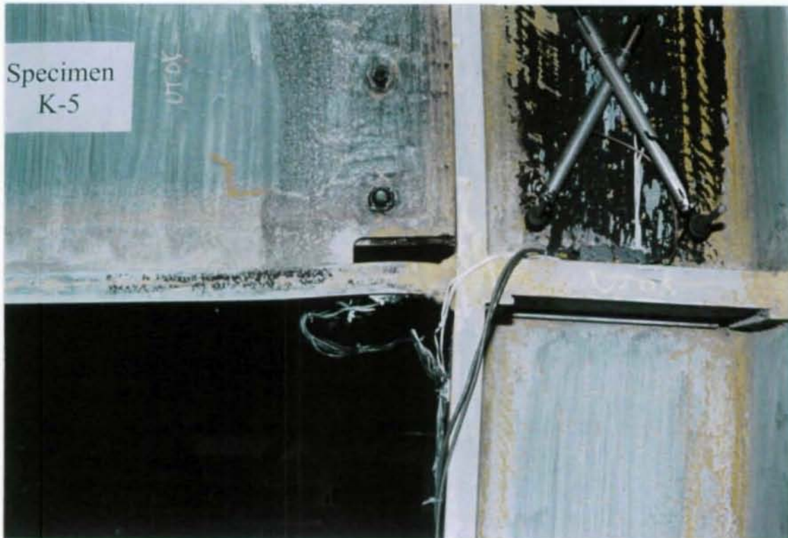
Figure 4.14 Specimen K5: Curvature of Beam Bottom Flange near Weld Access Hole at 5% Drift
