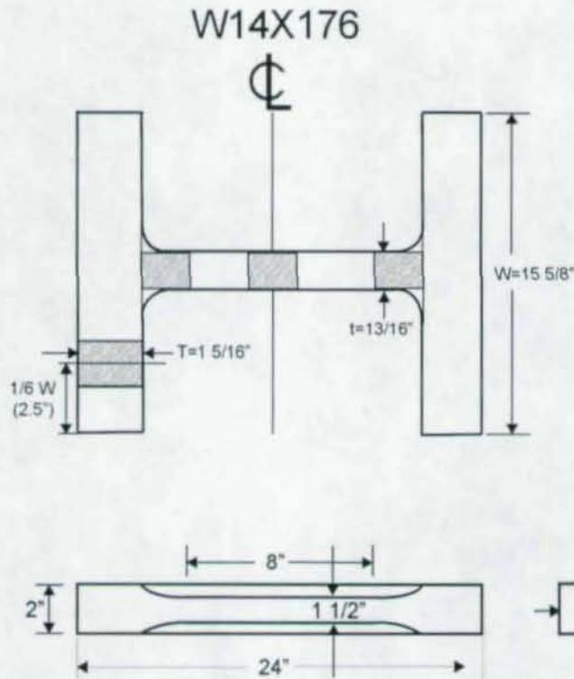
Figure 1 Column Section Tensile Coupon Locations.
