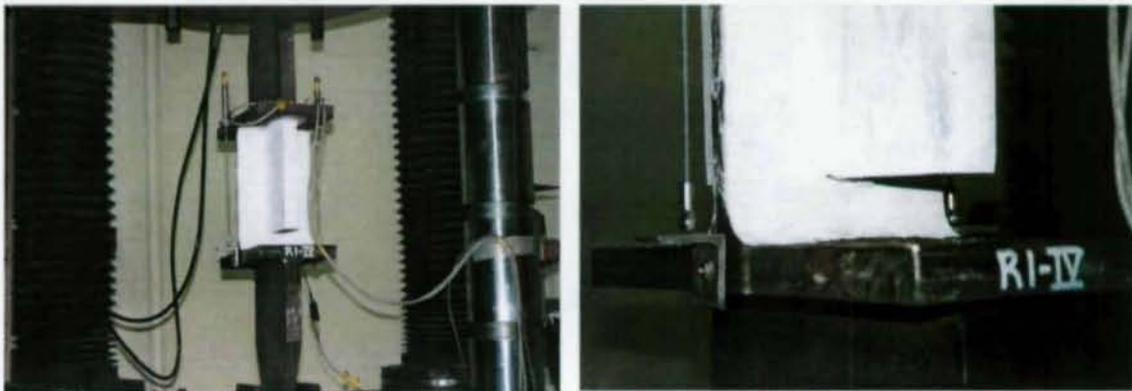
**Figure 17** Type IV Specimen Configuration Showing Stiffener Weld Terminating Beyond the K-area (Approx. 1-3/4 in. From Flange Inside Face).
