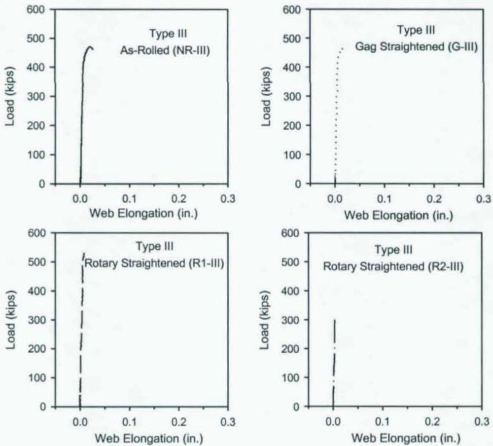
**Figure 13** Load vs. Web Elongation Behavior For Type III Specimens.
