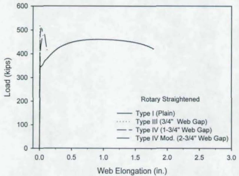
Figure 24 Effect of Stiffener Web Gap on Rotary Straightened Section Behavior.
