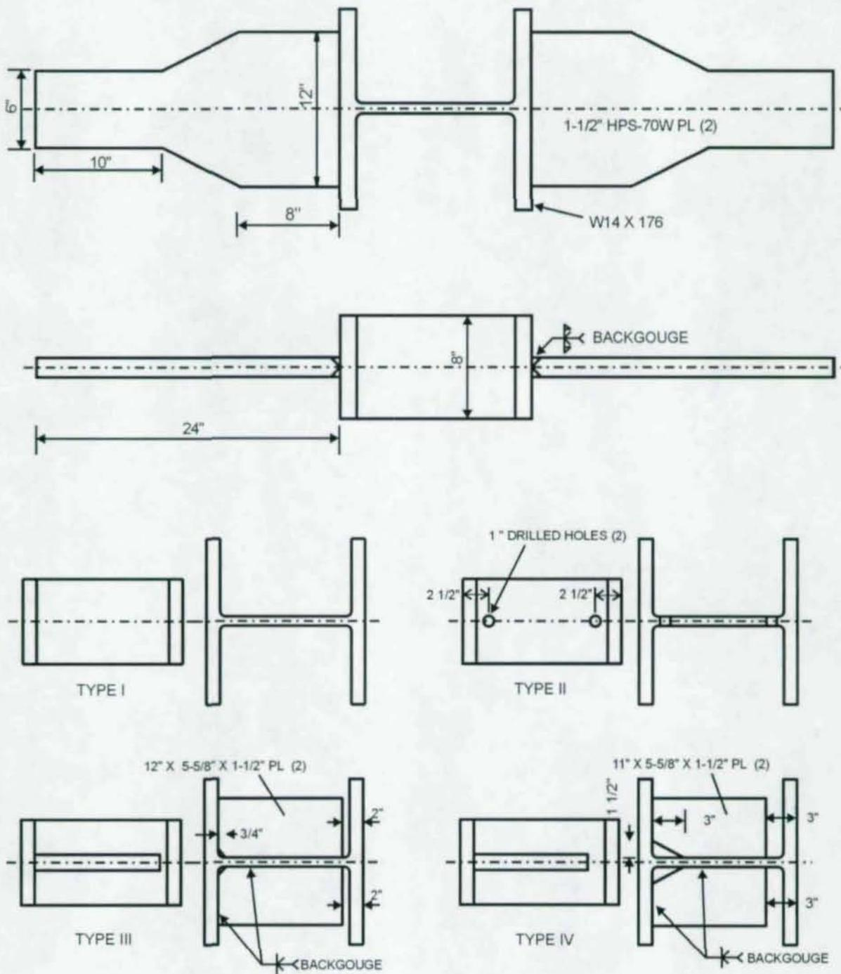
Figure 4 K-area Tension Test Specimen Design and Test Configurations.
