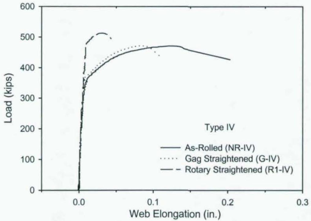
Figure 18 Load vs. Web Elongation Behavior For Type IV Specimens.
