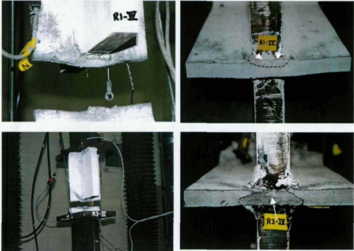
Figure 20 Ductile/Brittle Fracture of Rotary Straightened Type IV Specimens. Arrows Show Ductile Tearing Region.
