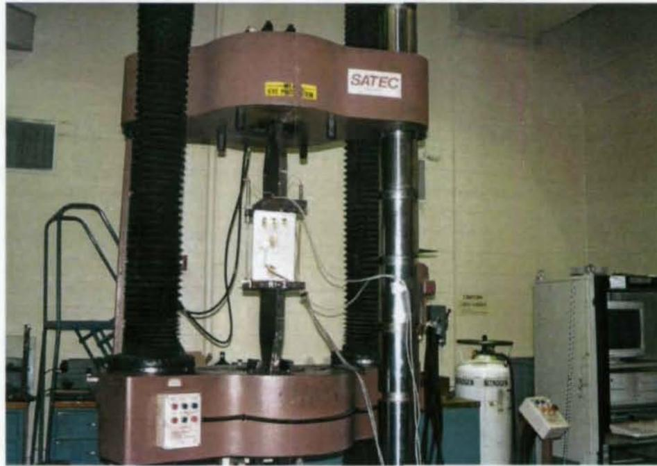
**Figure 6** Tension Load Test Specimen Installed in the 600 kip Capacity Test Machine.
