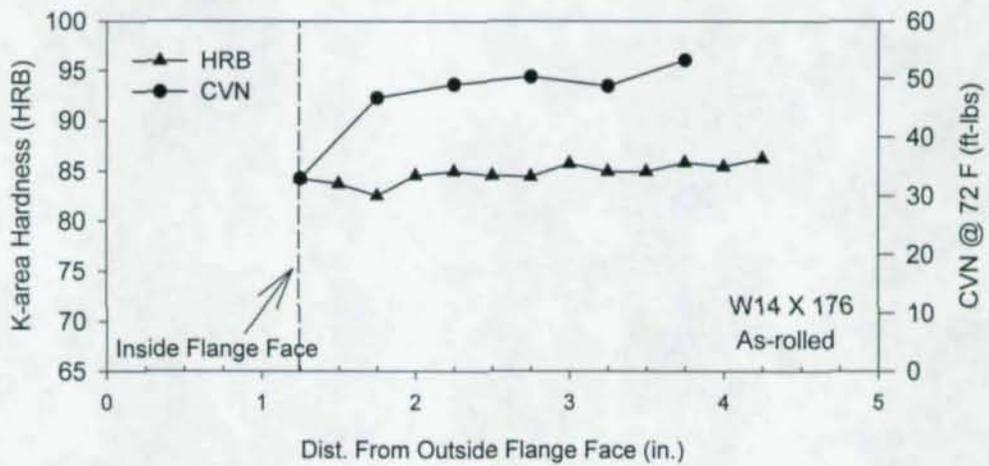
Figure 3 K-area Hardness and CVN for the Three Differently Processed Sections.
