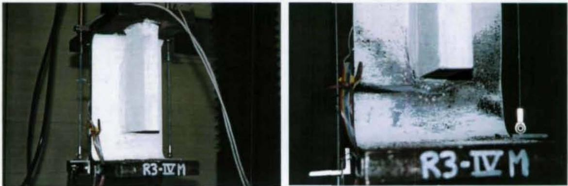
Figure 21 Modified Rotary Straightened Type IV Specimen Showing Fully Ductile Fracture Behavior (Stiffener Weld Terminates Approx. 2-3/4 in. From Flange Inside Face).
