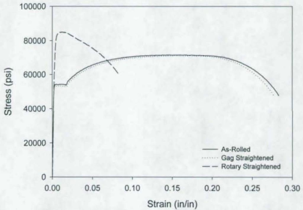
Figure 2 K-area Stress-Strain Behavior for the Three Differently Processed Sections.
