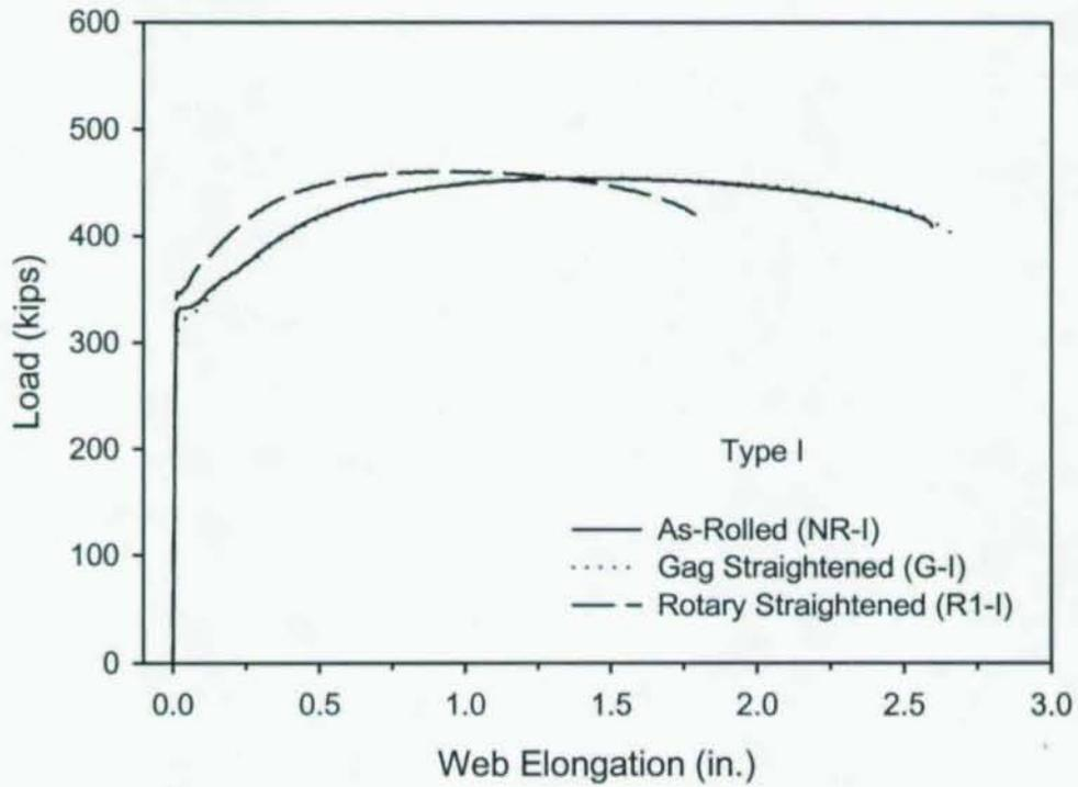
**Figure 8** Load vs. Web Elongation Behavior For Type I Specimens.
