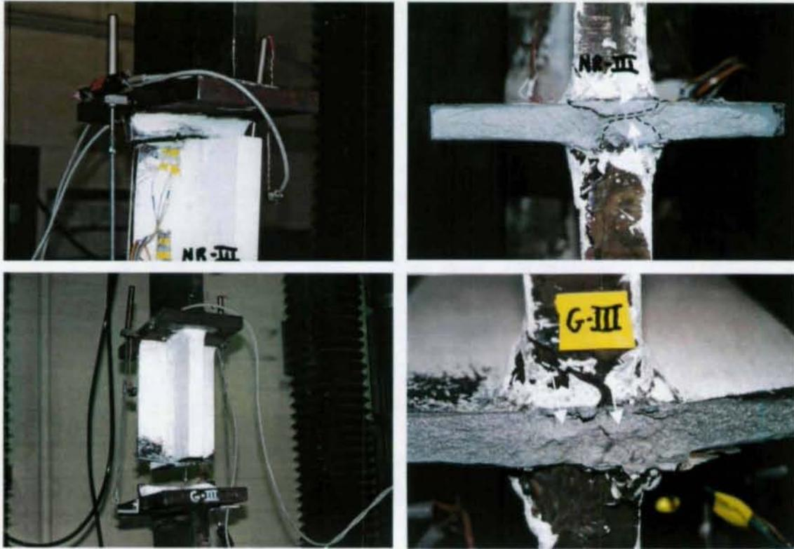
**Figure 16** Ductile/Brittle Fracture of As-Rolled (NR-III) and Gag Straightened (G-III) Type III Specimens. Arrows Show Initial Ductile Tearing.
