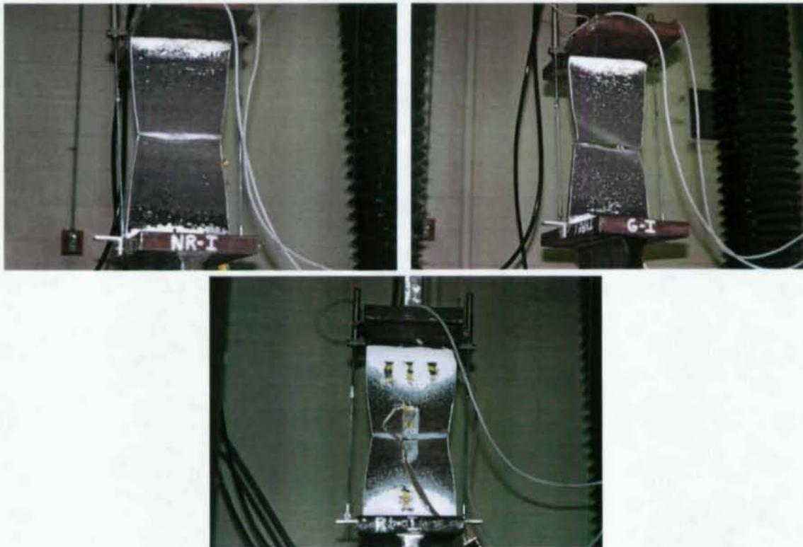
**Figure 9** Ductile Web Fracture of As-Rolled (NR-I), Gag Straightened (G-I) and Rotary Straightened (R1-I) Type I Test Specimens.
