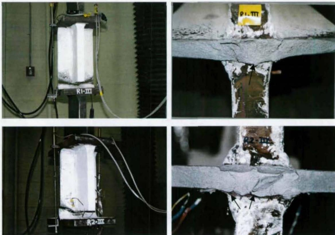
**Figure 15** Brittle Fracture of Rotary Straightened Type III Specimens. Arrow Denotes Weld Toe Cleavage Fracture Origin(s).
