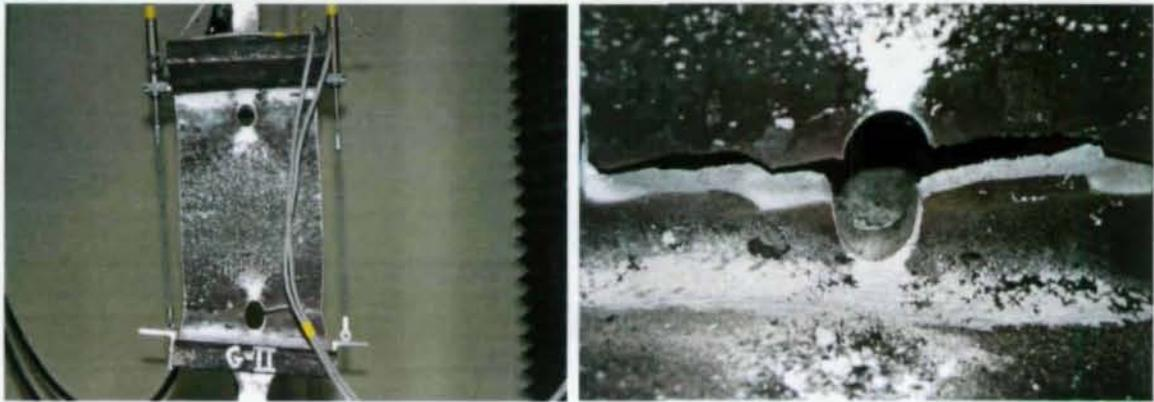
**Figure 12** Ductile Fracture of Type II Gag Straightened Specimen at Drilled Hole Due to Bending From Pull-Plate Weld Distortion.
