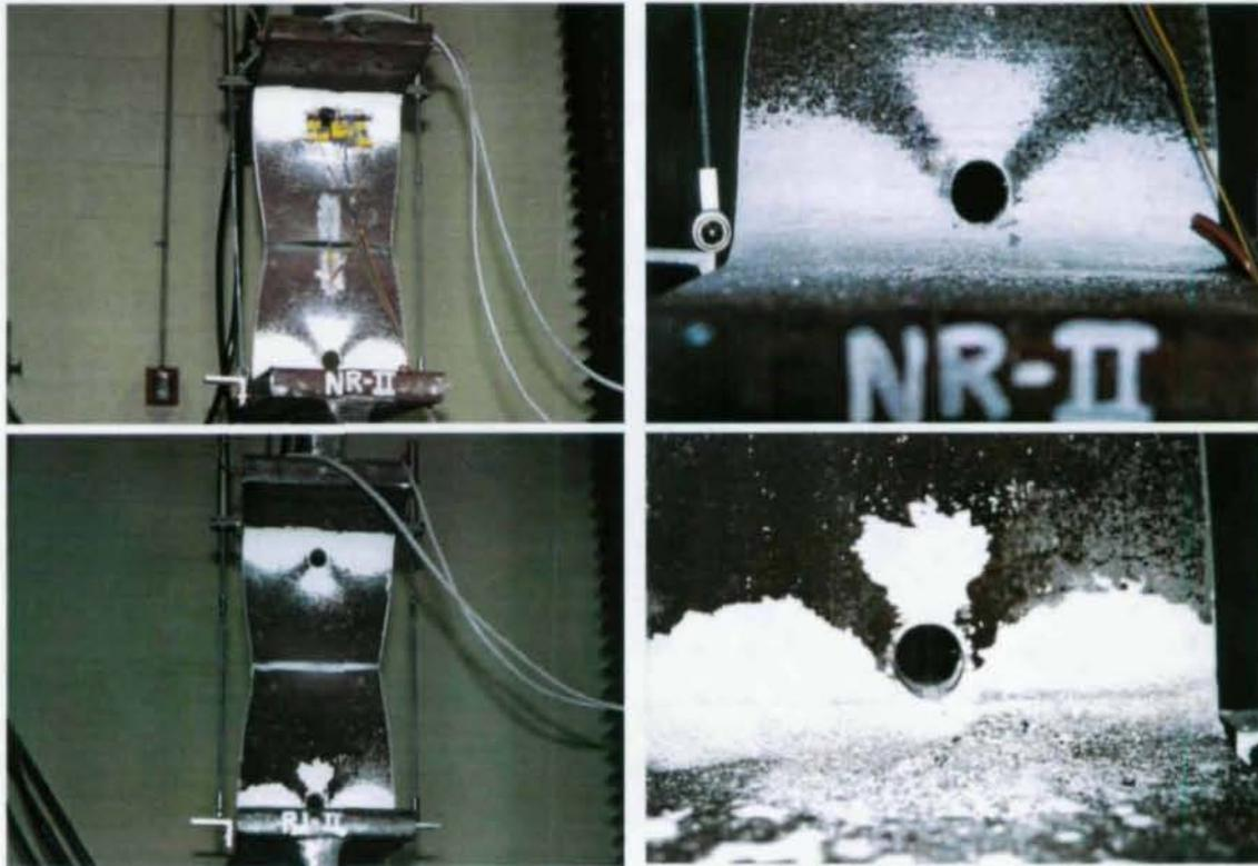
Figure 11 Ductile Web Fracture of As-Rolled (NR-II) and Rotary Straightened (R1-II) Type II Specimens. Note Large Elongation of Drilled Hole in NR-II and Lesser Deformation in R1-II.
