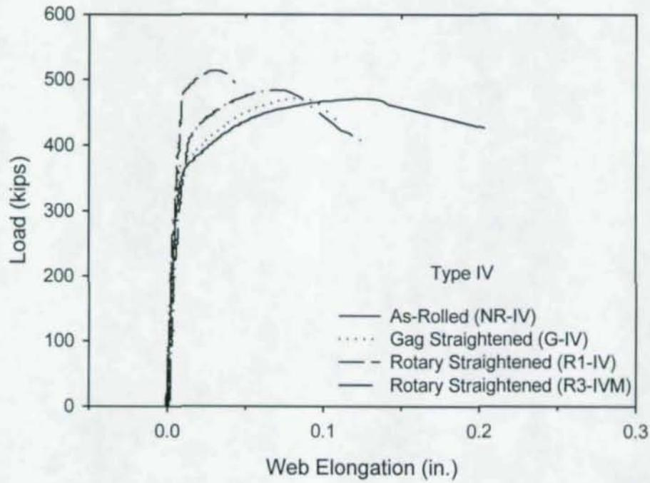
**Figure 22** Load vs. Web Elongation Behavior of Modified Type IV Rotary Straightened Specimen (R3-IVM) With Larger Web Gap in Comparison to Standard Type IV Specimens.
