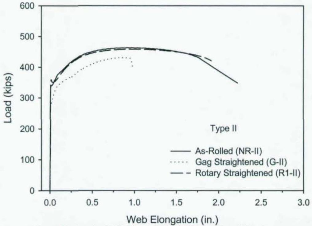
Figure 10 Load vs. Web Elongation Behavior for Type II Specimens.
