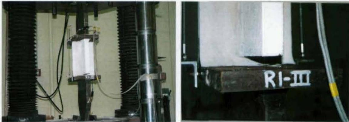
**Figure 14** Type III Specimen Configuration Showing Stiffener Weld Terminating in the K-area (Approx. 3/4 in. From Flange Inside Face).
