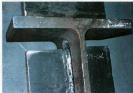
**Figure 5e** Type IV Web Gap Detail.
