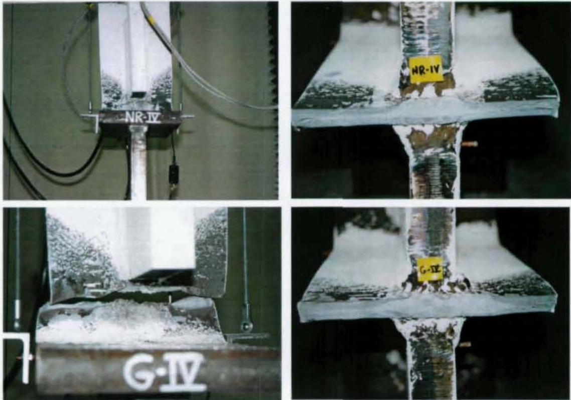
Figure 19 Fully Ductile Fracture of As-rolled (NR-IV) and Gag Straightened Type IV Specimens.
