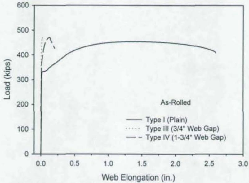
**Figure 23** Effect of Stiffener Web Gap on As-Rolled Section Behavior.
