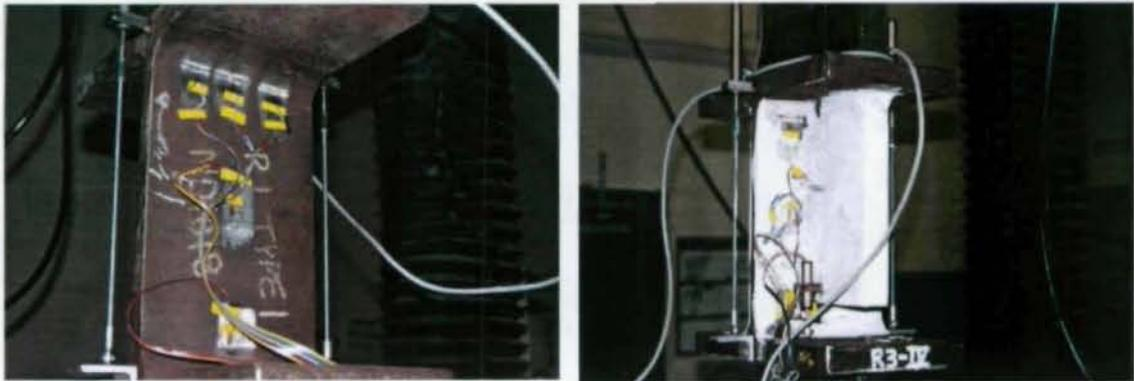
**Figure 7** LVDT Sensor Positions for Measurement of Web and Web Gap Displacements.
